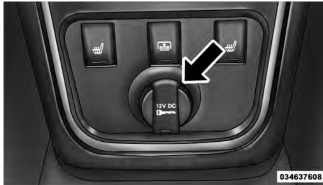
Center Console Power Outlet
