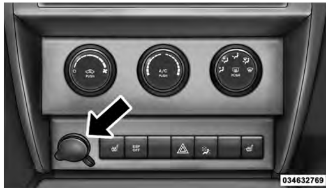
Front Power Outlet
