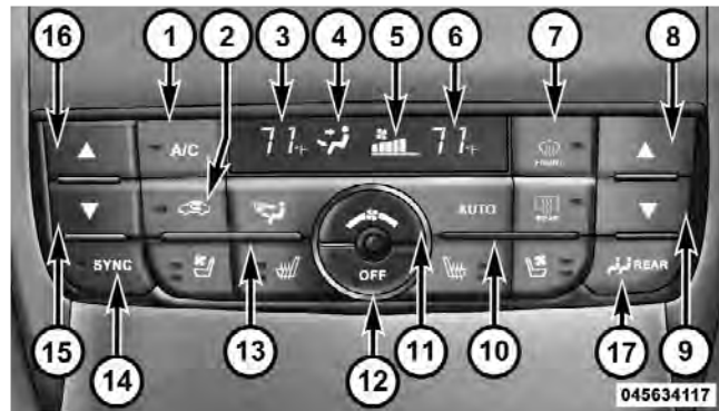
Automatic Temperature Control (ATC) Panel
