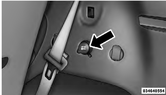
Rear Power Outlet
