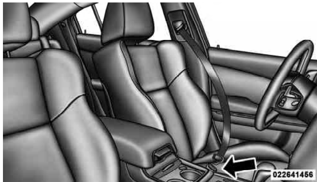
Inserting Latch Plate Into Buckle
