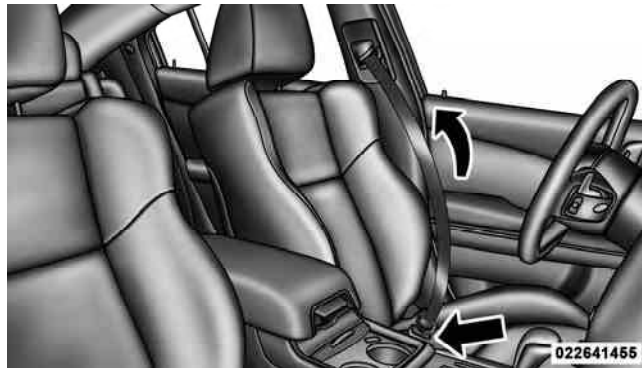
Removing Slack From Belt
