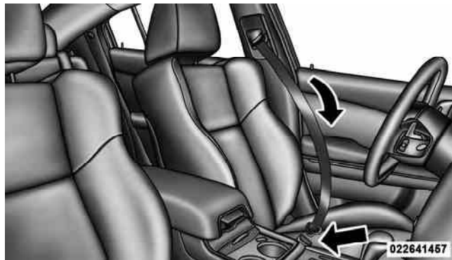
Pulling Out The Lap/Shoulder Belt Latch Plate
