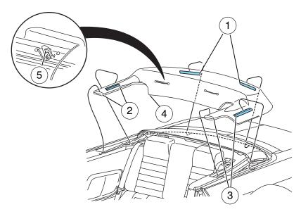
1. Install the boot on the vehicle by hooking the boot retaining clips on the back panel.
