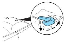
**Note:** If the top has not been lowered for some time and sticks to the windshield header, push the front of the top up slightly with your hand to loosen it.
