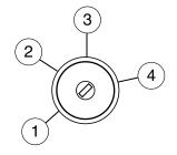
The battery saver will shut off the interior lamps 10 minutes after the ignition has been turned to the 1 (OFF/LOCK) position and a door is left open, and in 30 minutes if the dome lamp control is left on and the ignition has been turned to the 1 (OFF/LOCK) position. The battery saver will also shut off the trunk lamps in 30 minutes if the trunk is left open.
