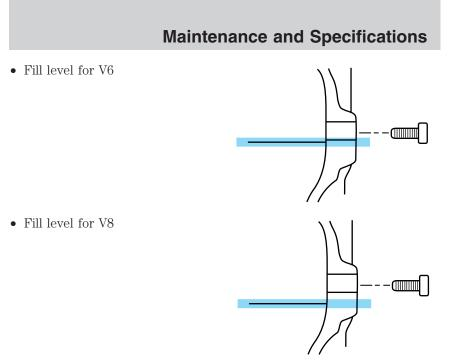
4. Add enough fluid through the filler opening to bring the fluid up to the recommended levels.
