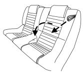
When raising the seatback(s), make sure you hear the seat latch into place. Pull on the seatback to ensure that it has latched.
