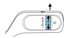
For normal or low speed wiper operation, move control up two positions from OFF.
