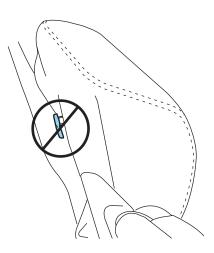
4. Access tether anchors located behind the seatback under the vinyl tag marked with the child tether anchor symbol.
