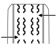
the same height as these "wear bars", the tire is worn out and must be replaced.
