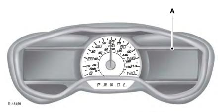
The display is located on the right side of your instrument cluster (A). You can use your steering wheel controls to view and make minor adjustments to active modes without taking your hands off the wheel. For example:
