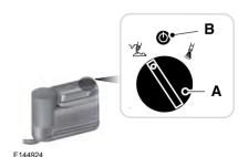
7. Push and turn dial (A) counterclockwise to the sealant position. Turn on the kit by pressing the on and off button (B).
