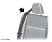
When in use, the rear safety belts should be placed in the belt guides on the outboard seat backs.
