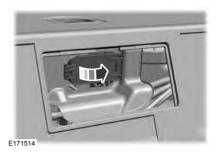
If equipped, pull the end of the outer lever toward the front of the vehicle and remove the outer lever from the service disconnect.
