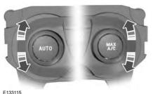
You can set the temperature between 60°F (15.5°C) and 85°F (29.5°C) in steps of 1°F (0.5°C). In position **LO**, 59°F (15°C), the system switches to permanent cooling. In position **HI**. 86°F (30°C), the system switches to permanent heating.
