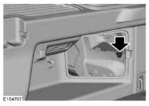
4. Pull the manual override mechanism.
