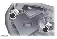
Lift the air cleaner assembly (A) from the mounting studs, then rotate and pull it towards the front of the vehicle.
