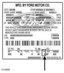
The transmission code is on the Safety Compliance Certification Label. The following table shows the transmission code along with the transmission description.
