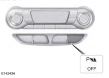
Press the button to switch the system off. It will remain off for the entire ignition cycle. The system can also be switched off through the information display.
