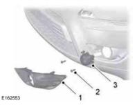
Remove the screws from the splash shield at the wheel well to gain access to the lamp assembly.
