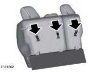
2. Locate the correct anchor on the back panel of the rear seat for the selected seating position. The anchors are labeled with the tether strap symbol and are partially covered by the gap panel. Pull the panel back to fully expose the anchors.
