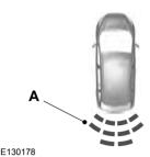
A Coverage area of up to 6 feet (1.8 meters) from the rear bumper. There is decreased coverage area at the outer corners of the bumper.
