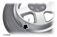
**Note:** Each road tire is equipped with a tire pressure sensor located inside the wheel and tire assembly cavity. The pressure sensor is attached to the valve stem. The pressure sensor is covered by the tire and is not visible unless the tire is removed. Take care when changing the tire to avoid damaging the sensor
