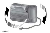
Unwrap the clear tube from the compressor housing.
