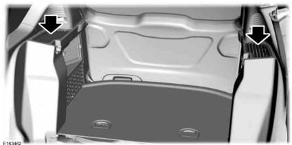
**Note:** The high-voltage battery is equipped with air vents in the package tray that help to regulate its temperature. It is important to keep these openings free of obstructions. Do not block the flow of cabin air to this area.
