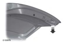
A handle is located inside the liftgate to help with closing.
