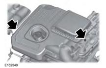
4. Install and tighten the bolts to each side of the air cleaner assembly (A) as shown with arrows.
