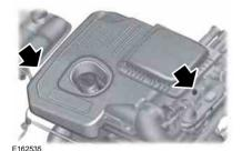
Remove the bolts from each side of the air cleaner assembly (A) as shown with arrows
