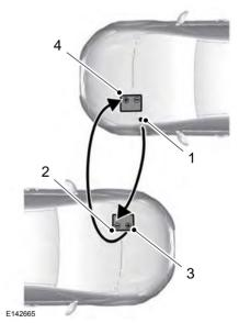
Remove the jumper cable from the ground metal surface or connecting point, if available.
