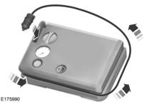
5. Wrap the power cord around the housing and stow the accessory power plug into its storage area.
