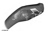
To operate the washers and spray the windshield, pull the lever toward you.
