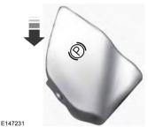
You can release the electric parking brake either manually by pressing the switch or automatically.
