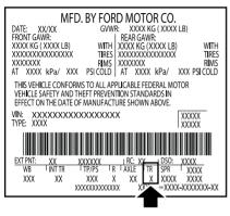
The transmission code is on the Safety Compliance Certification Label. The following table shows the transmission code along with the transmission description.
