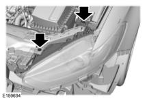
Remove the two screws securing the headlamp using a flat-bladed screwdriver.
