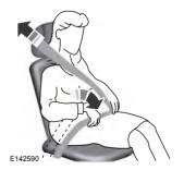
Pregnant women should always wear their safety belt. The lap belt portion of a combination lap and shoulder belt should be positioned low across the hips below the belly and worn as tight as comfort will allow. The shoulder belt should be positioned to cross the middle of the shoulder and the center of the chest.
