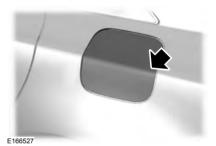
Press the center-rear edge of the fuel filler door and release to open.
