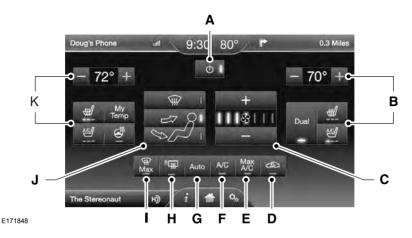
A **Power:** Touch the button to switch the system on and off. Switching off the climate control system prevents outside air from entering the vehicle.
