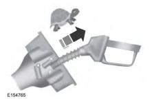
**Note:** Allow about five to ten seconds after pumping fuel before removing the fuel filler nozzle. This allows residual fuel to drain back into the fuel tank and not spill onto the vehicle.
