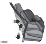
10. Before placing the child in the seat, forcibly move the seat forward and back to make sure the seat is securely held in place. To check this, grab the seat at the belt path and attempt to move it side to side and forward and back. There should be no more than 1 inch (2.5 centimeters) of movement for proper installation.
