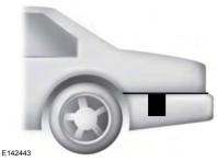
The system uses radar sensors which are located behind the bumper fascia on each side of your vehicle. Do not allow mud, snow or bumper stickers to obstruct these areas, this can cause degraded system performance.
