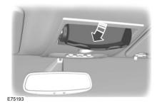
Press near the rear edge of the door to open it.
