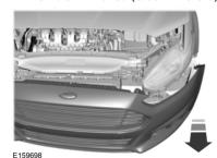
9. From the front of the vehicle, gently pull the front bumper cover forward 4 inches (10 centimeters) by grasping it next to the headlamp to be serviced and in the lower front of the wheel opening.
