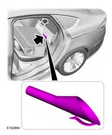
Locate the portable funnel that comes with your vehicle. The funnel is located behind the left-hand side rear seat, under the carpet. Fold down the left-hand side rear seat back. Pull back the piece of carpet to access the funnel.
