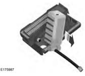
Rotate the sealant canister up 90 degrees and pull away from casing/housing to remove.
