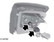
2. Remove the bulb from the bulb holder.
