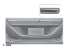
Press the release button above the license plate to unlatch the trunk. Your vehicle must be unlocked or have an intelligent access transmitter within 3 feet (1 meter) of the trunk.
