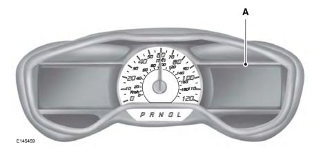
The display is located on the right side of your instrument cluster (A). You can use your steering wheel controls to view and make minor adjustments to active modes without taking your hands off the wheel. For example:
