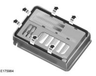
Unwrap the dual purpose hose (black tube) from the compressor housing.
