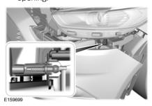
10. Gently pull the headlamp assembly outward to disengage it from the lower fixing point.
