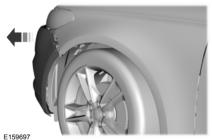
8. Separate the front bumper cover from the fender by gently pulling the front bumper cover to the outside of the vehicle 1.2 inches (3 centimeters).
