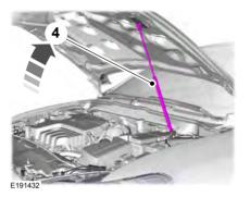
4. Open the hood. The hood strut automatically supports the hood.
