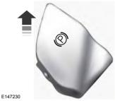
Pull the switch up to apply the electric parking brake.
