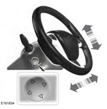
Use the control on the side of the steering column to adjust the position.
