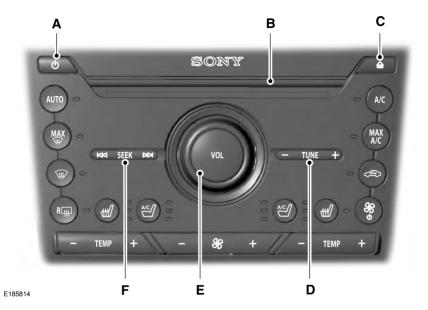
A **Power:** Press this button to switch the system off and on.
