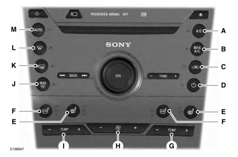
A **A/C:** Press the button to turn air conditioning compressor on or off. Use air conditioning with recirculated air to improve cooling performance and efficiency.
