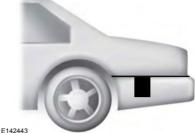
The system uses radar sensors which are located behind the bumper fascia on each side of your vehicle. Do not allow mud, snow or bumper stickers to obstruct these areas, this can cause degraded system performance.
