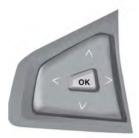
Press the OK button to acknowledge and remove some messages from the information display. The information display will automatically remove other messages after a short time.
