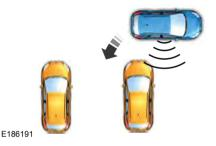
When you shift the transmission into reverse (R), with your hands off the wheel (and nothing obstructing its movement), your vehicle steers itself into the space. The system displays instructions to move your vehicle back and forth in the space.
