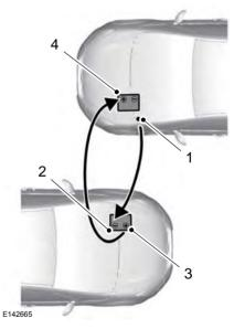
1. Remove the jumper cable from the ground metal surface or connecting point. if available.
