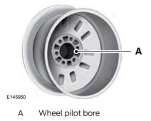
Inspect the wheel pilot hole and mounting surface prior to installation. Remove any visible corrosion or loose particles.
