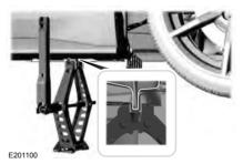
Position the jack so that the vehicle 10. downward flange rests in the jack saddle flange as shown above. Raise the vehicle by using the lug wrench to turn the jack nut clockwise. Once the flat tire is raised above the ground, remove the lug nuts with the lug wrench.
