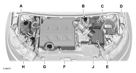
A Engine coolant reservoir. See **Engine Coolant Check** (page 263).
