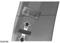
Slide the clip away from the tongue so there is no loose webbing when an occupant or child seat is buckled up. You can also use the sliding clip to raise the tongue and prevent it from rattling or to ease access to the tongue.
