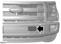
A message displays if something obstructs the radar signals from the sensor. The sensor is behind a cover near the driver side of the lower grille. The system cannot detect a vehicle ahead and does not function when something obstructs the radar signals. The following table lists possible causes and actions for this message displaying.
