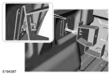
Hook the top of the ramp holder over the mounting plate and rotate the ramp holder into position.
