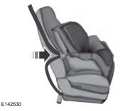
While holding both shoulder and lap portions next to the tongue, route the tongue and webbing through the child seat according to the child seat manufacturer's instructions. Be sure that the belt webbing is not twisted.
