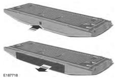
3. Pull the step out fully. Lower the step to its lowest position.
