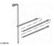
Use your key to remove the lock cylinder from the access hole of the bumper to allow access to the guide tube. Assemble the jack handle as shown in the illustration.
