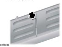
5. Make sure to insert the latch rod into the tailgate hole. Make sure to engage both sides of the locking pins into their holes in the pick-up box.
