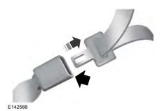
To unfasten, press the release button and remove the tongue from the buckle.
