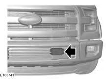
If a blocked sensor message appears in the information display, dirt, water, or an object is blocking the sensor. The sensor is located behind a cover near the driver side of the lower grille. If anything blocks the sensor, your vehicle cannot see through the sensor, and the collision warning system will not work. Possible causes for the blocked sensor message and corrective actions are listed below.
