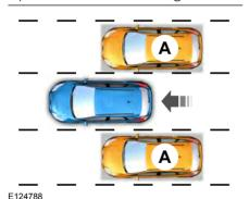
The Blind Spot Information System is designed to aid you in detecting vehicles that may have entered the blind spot zone (A). The detection area is on both sides of your vehicle, extending rearward from the exterior mirrors to approximately 13 ft (4 m) beyond the bumper. The system is designed to alert you if certain vehicles enter the blind spot zone while driving.
