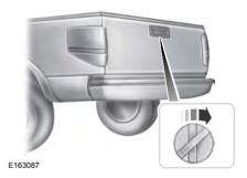
Insert the ignition key into the tailgate lock. Turn it clockwise to lock the tailgate. Turn it counterclockwise to unlock the tailgate.
