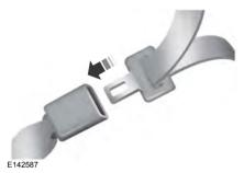
Insert the belt tongue into the proper buckle (the buckle closest to the direction the tongue is coming from) until you hear a snap and feel it latch. Make sure you securely fasten the tongue in the buckle.
