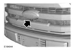
The front video camera, located in the grille, provides a video image of the area in front of your vehicle. It adds assistance to the driver while driving forward at low speeds. To use the front video camera system, place the transmission in any gear except reverse (R). An image will display once the camera enable button is pressed. The area displayed on the screen may vary according to your vehicle's orientation and/or road condition.
