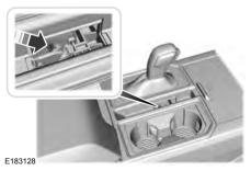
Apply the brake pedal. Using light finger pressure move the white lever forward while pulling the gearshift lever out of the park (P) position and into the neutral (N) position.
