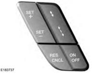
The controls for using your cruise control are located on the steering wheel.
