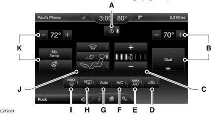
A **Power:** Touch the button to turn the system on and off. Switching off the climate control system prevents outside air from entering the vehicle.
