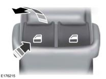
Press the switch to open the window. Lift the switch to close the window.
