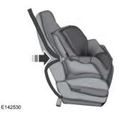
3. While holding the shoulder and lap belt portions together, route the tongue through the child seat according to the child seat manufacturer's instructions. Be sure the belt webbing is not twisted.
