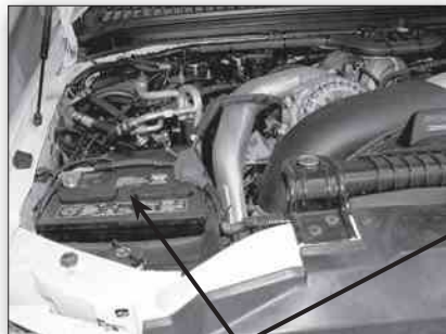
F-550 Primary Battery Location
