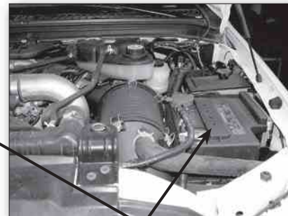
F-550 Primary Battery Location
