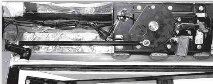
Electric door motor with control arm
