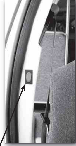
Secondary Entry Door Switch - used on air operated door systems, located on passenger door post
