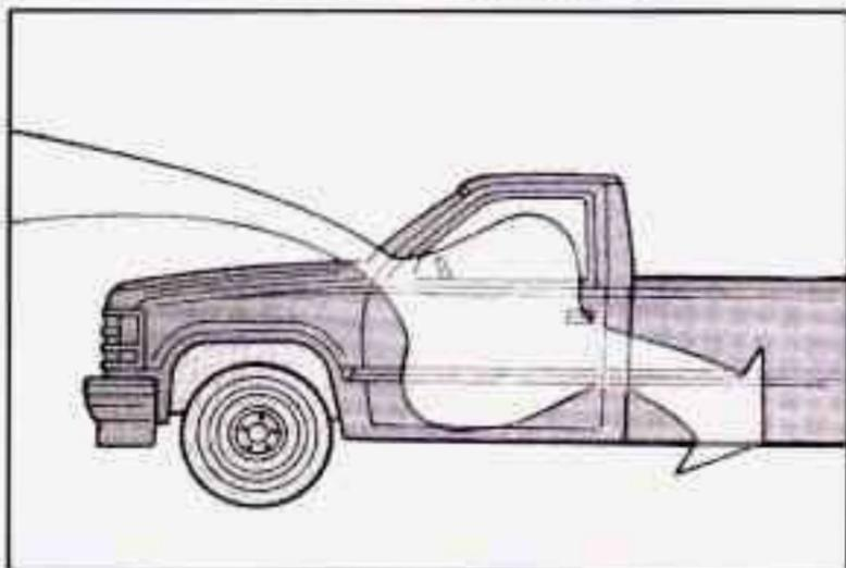
With the side windows closed, air will flow into the front air inlet grilles, through the vehicle and out the rear air exhaust valves.
