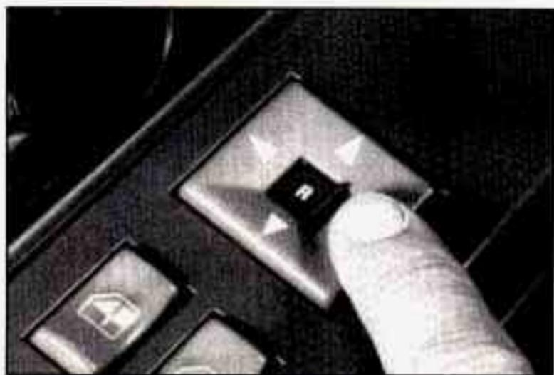
Select the mirror you want to move by moving the center of the switch, located on the driver's door armrest, to **R** (right) or **L** (left). Then, adjust the mirror angle by pressing the outer arrows on the switch until the mirror is adjusted where you want it.
