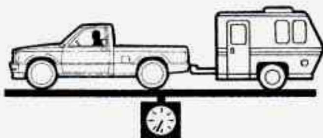
If your vehicle comes with the Trailer Package, there is also a load rating which includes the weight of the vehicle **and** the trailer it tows. This rating is called the Gross Combination Weight Rating (GCWR).
