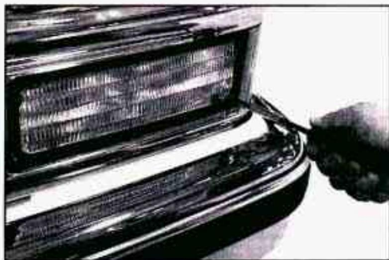
1. Remove the screws and take out the parking/turn signal light assembly.
