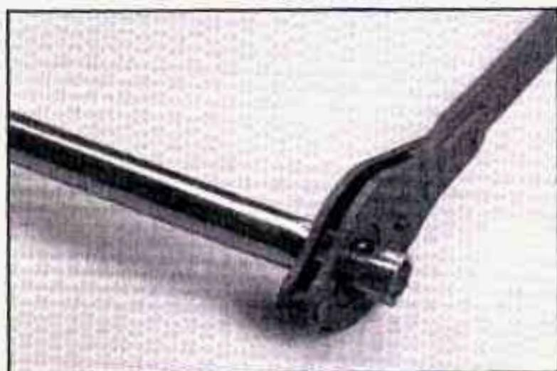
Attach the ratchet, with the **DOWN** marking facing you, to the wheel wrench.
