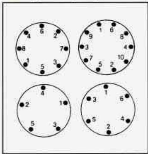
Tighten the nuts firmly in a criss-cross sequence as shown. Rotate the ratchet to the right with the **UP** marking facing you.
