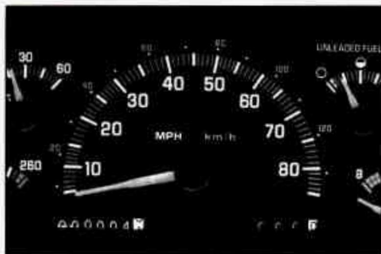
Your speedometer lets you see your speed in both miles per hour (mph) and kilometers per hour (km/h). Your odometer shows how far your vehicle has been driven, in either miles (used in the U.S.) or kilometers (used in Canada).
