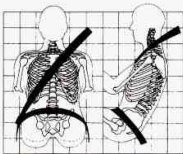
The driver has a lap-shoulder belt. Here's how to wear it properly.
