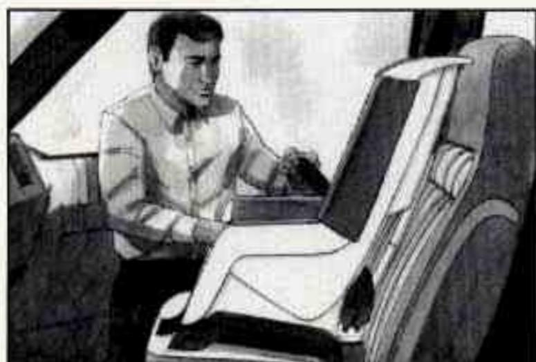
5. Pull the rest of the lap belt all the way out of the retractor to set the lock.
