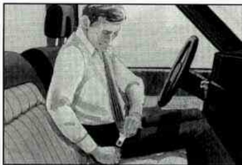
3. Pick up the latch plate and pull the belt across you. (On some models, you may hear a clicking sound as the belt is pulled out. The clicking sound is the shoulder belt tension feature operating properly.) Don't let the belt get twisted.
