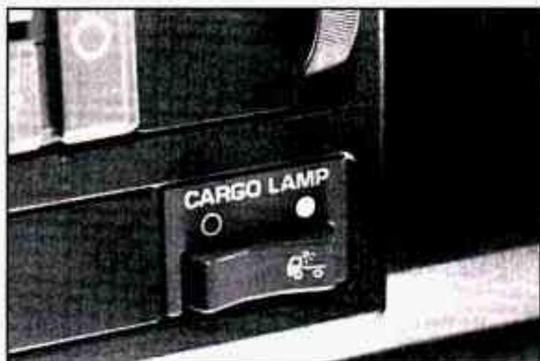
To turn your optional cargo lamp on, push the side of the switch with the cargo lamp symbol on it.
