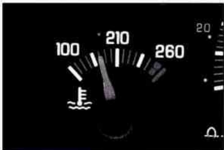
This gage shows the engine coolant temperature. If the gage pointer moves into the red area, about 260° F (145° C) or more, your engine is too hot! It means that your engine coolant has overheated. If you have been operating your vehicle under normal operating conditions, you should pull off the road, stop your vehicle, and turn off the engine as soon as possible.
