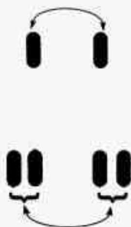
Use this pattern if your front and rear tires are different sizes or load ranges. The dual rear tires are rotated as a pair and the inside rear tires become the outside rear tires.
