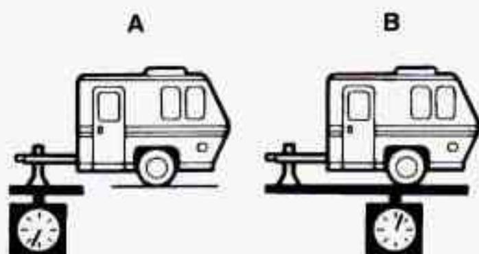
If you’re using a “dead-weight” hitch, the trailer tongue (A) should weigh 10% of the total loaded trailer weight (B). If you have a “weight-distributing” hitch, the trailer tongue (A) should weigh 12% of the total loaded trailer weight (B).
