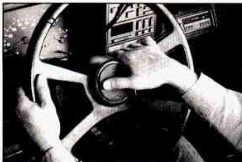
To sound the horn, press the pad in the center of the steering wheel. The pad has a horn symbol on it.
