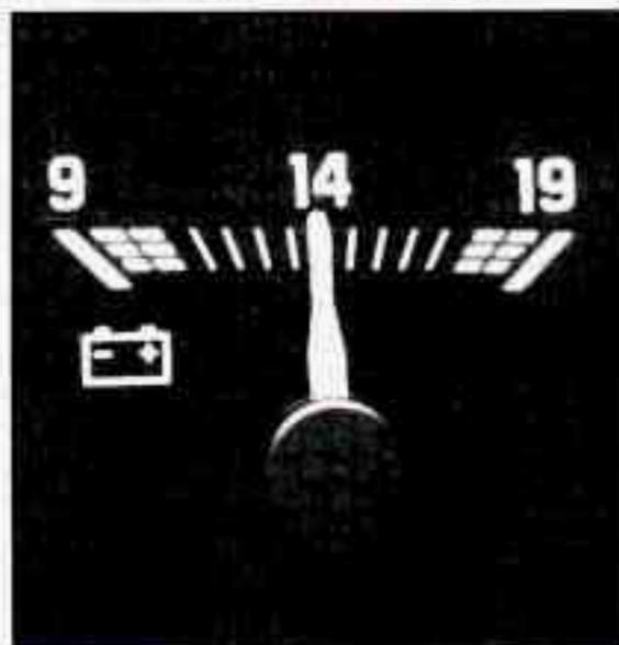
When your engine is not running, but the ignition is on (in the **RUN** Position), this gage shows your battery's state of charge in DC volts. When the engine is running, the gage shows the condition of the charging system. Readings between the low and high warning zones indicate the normal operating range.
