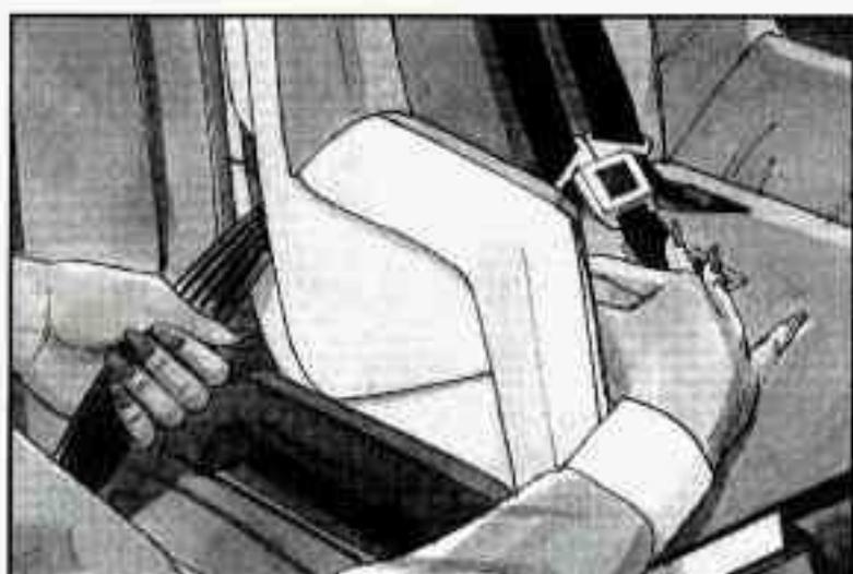
6. To tighten the belt, feed the lap belt back into the retractor while you push down on the child restraint.
