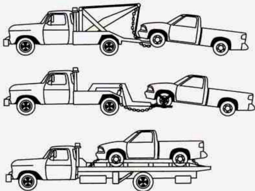
If you have a two-wheel drive vehicle, don't have your vehicle towed on the rear wheels, unless you must. If the vehicle must be towed on the rear wheels, don't go more than 35 mph (56 km/h) or farther than 50 miles (80 km) or your transmission will be damaged. If these limits must be exceeded, then the rear wheels have to be supported on a dolly.
