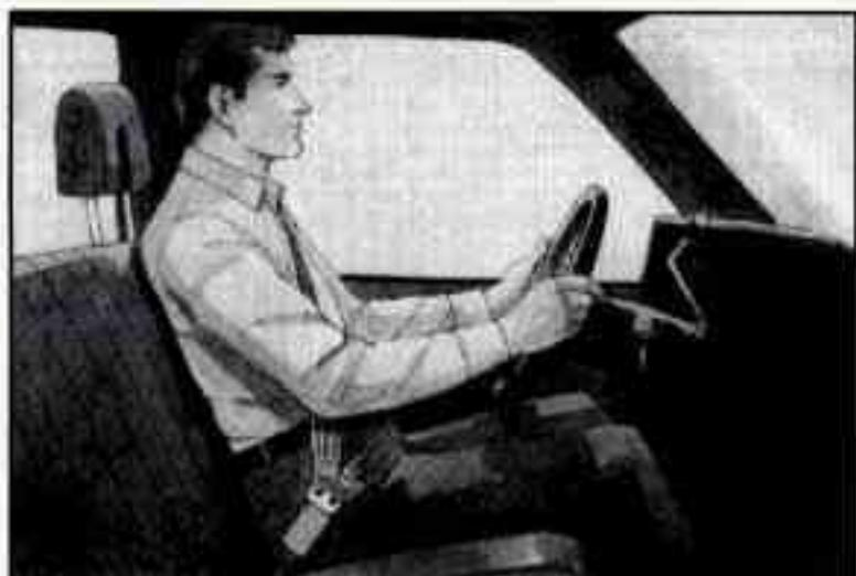
Slide the head restraint up or down so that the top of the restraint is closest to the top of your ears.
