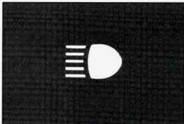
When the high beams are on, this blue light on the instrument panel also will be on.
