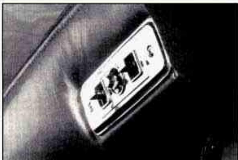
If your vehicle has a power seat on the driver's side, you can adjust it with this switch at the front of the seat.
