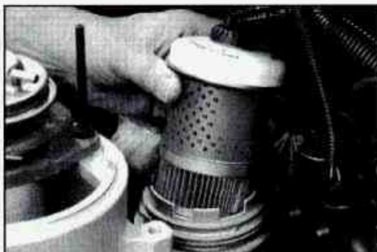
5. Lift the element out of the filter head.
