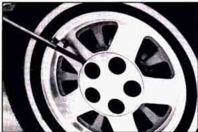
If the wheel has a smooth center piece or a center piece with recessed nuts, place the flat end of the wheel wrench in the slot on the wheel and pry out gently.
