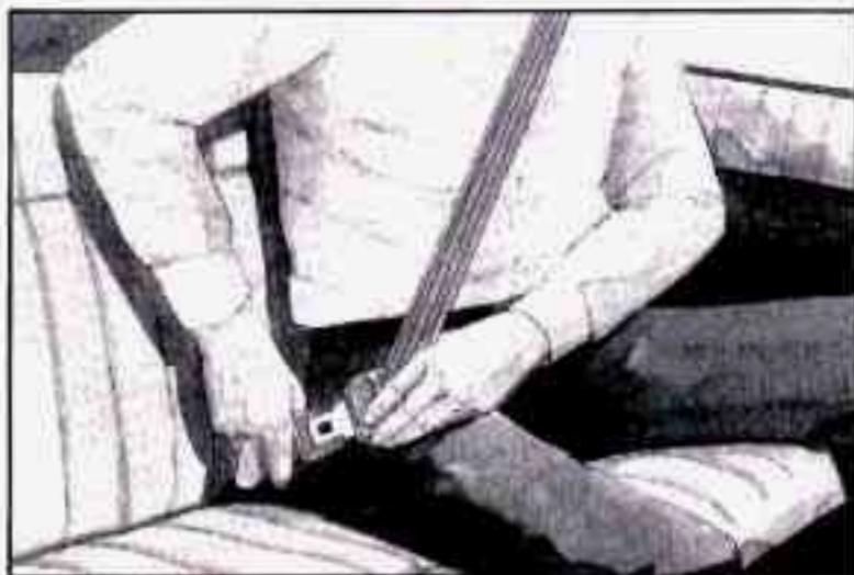
1. Pick up the latch plate and pull the belt across you. (On some models, you may hear a clicking sound as the belt is pulled out. The clicking sound is the shoulder belt tension feature operating properly.) Don't let the belt get twisted.
