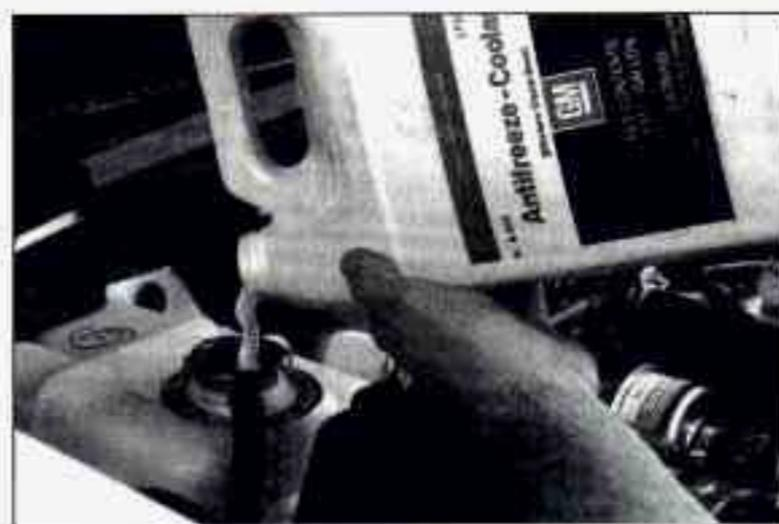
4. Fill the coolant surge tank with the proper mix, up to the **COLD** mark.
