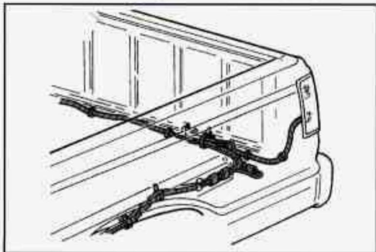
An optional 7-wire harness is stored under your vehicle along the rear frame crossmember. The harness has a 30 amp. in-line fused battery feed wire and no connector, and should be wired by a qualified electrical technician.
