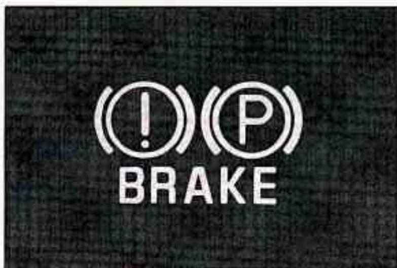
The red brake system warning light is located at the bottom right corner of the instrument cluster
