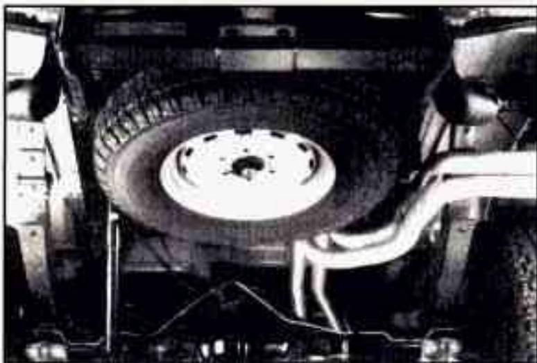
Your spare tire may be mounted underneath the rear of the vehicle.
