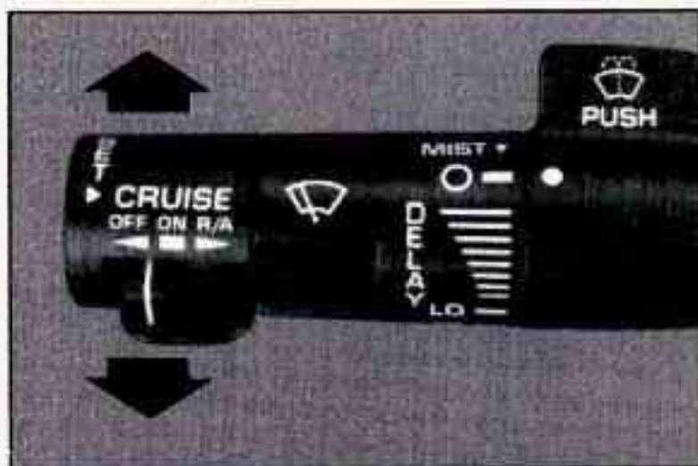
The turn signal has two upward (for right signal) and two downward (for left signal) positions. These positions allow you to signal a turn or a lane change.
