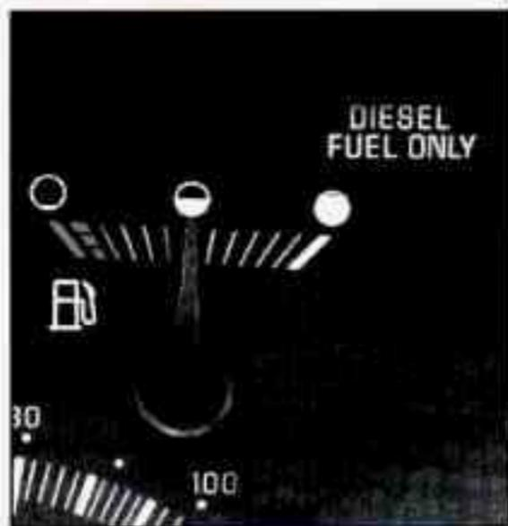
The fuel gage, when the ignition is on, tells you about how much fuel you have left in your tank. The gage will first indicate empty before you are out of fuel, and you should get more fuel as soon as possible.
