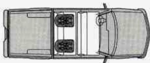
You'll be using the lap-shoulder belt. See the earlier section about the top strap if the child restraint has one.
