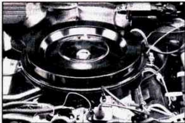
To remove the air cleaner filter on a gas engine or a 6.5 liter naturally aspirated diesel, turn the wing nuts to the left. Remove the cover and change the filter.
