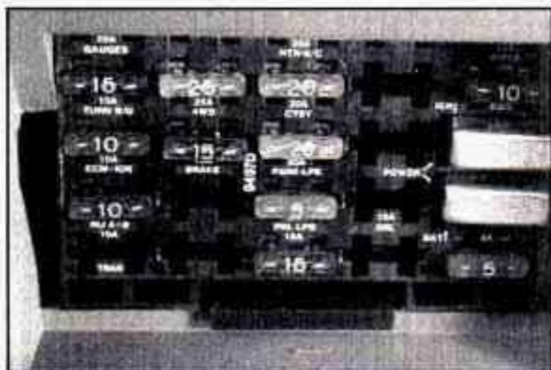
The fuse block is behind an access door at the bottom of the instrument panel, next to the parking brake release lever.
