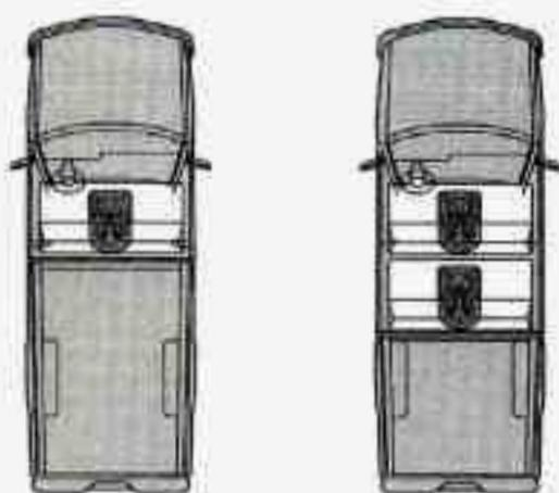
When you secure a child restraint in a center seating position, you'll be using the lap belt.
