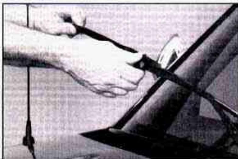
To replace the windshield wiper blade insert, lift the wiper arm and rotate the blade until it is facing away from the windshield.
