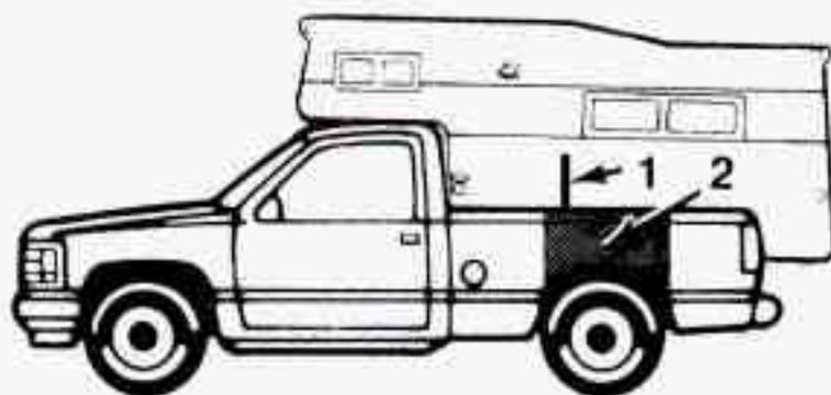
The camper's center of gravity should fall within the center of gravity zone for your vehicle's cargo load.
