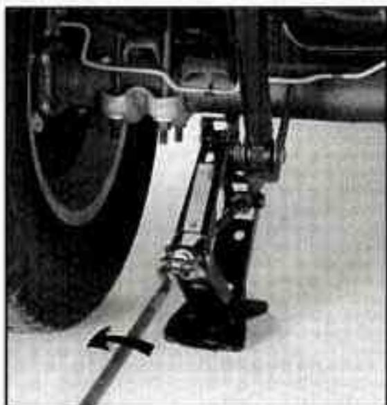
Lower the vehicle by rotating the ratchet to the left. Lower the jack completely.
