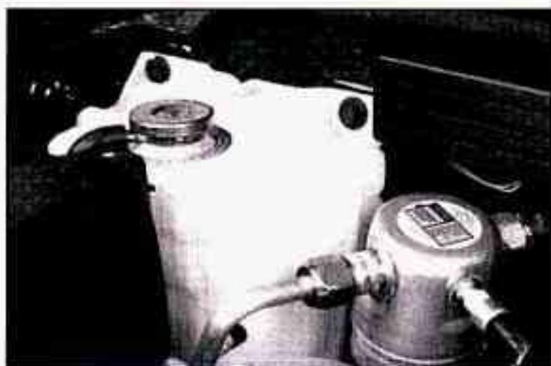
The coolant level should be slightly above the **COLD** mark. If it isn't, you may have a leak in the radiator hoses, heater hoses, radiator, water pump or somewhere else in the cooling system.
