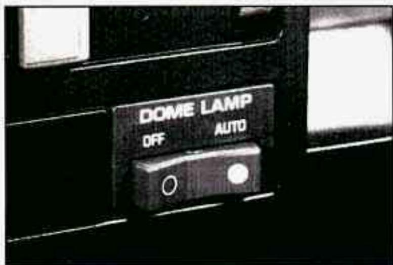
If you have a Crew Cab, you can use the dome lamp switch, located below the headlight switch, to set the dome lamps to come on automatically or remain off.
