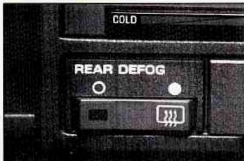
To turn on the rear window defogger, find the switch marked **REAR DEFOG** on your instrument panel, just below the heater system. Press the right side of the switch, with the defog symbol on it, until the light in the switch comes on, then release it.
