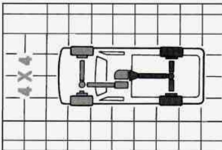
The front axle portion of the indicator diagram will light up when you shift into four-wheel drive.
