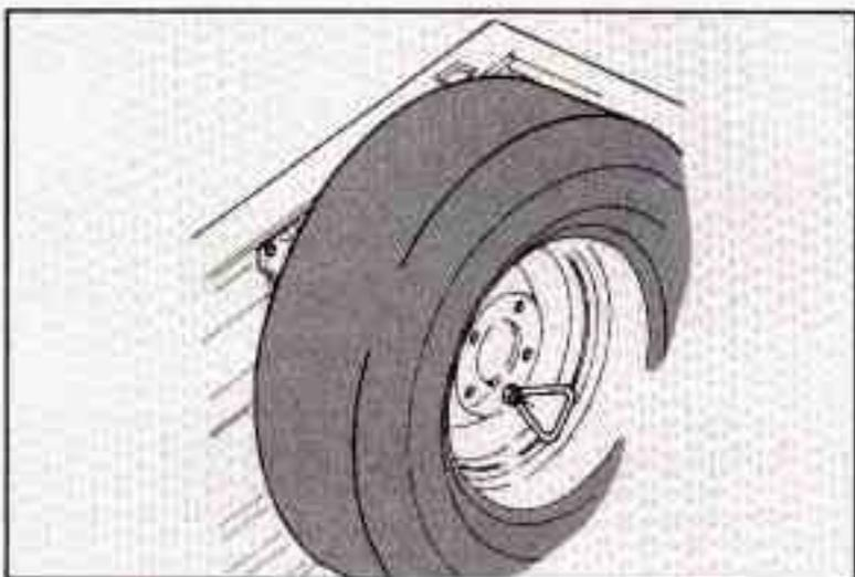
it may be mounted to the inside of the truck bed on the driver's side.
