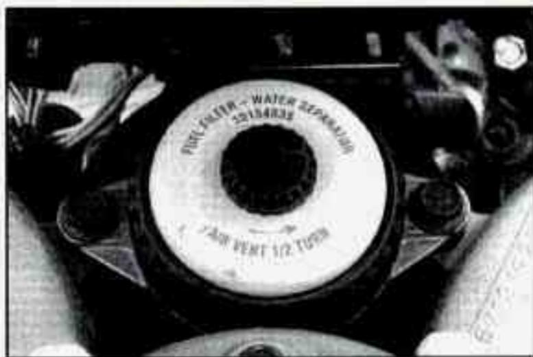
7. Line up the writing on the top of the filter so it faces (is readable from) the front of the vehicle. Push the element in until the mating surfaces touch.
