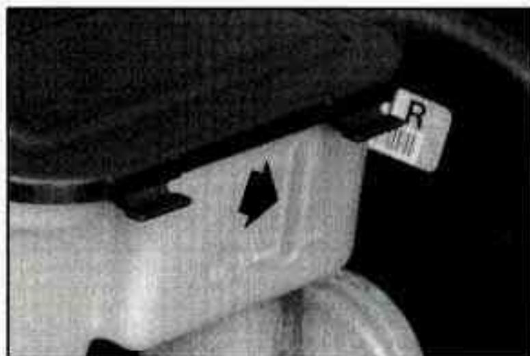
You can check the brake fluid without taking off the cap. Just look at the windows on the brake fluid reservoir. The fluid levels should be above "MIN." If they aren't, have your brake system checked to see if there is a leak.
