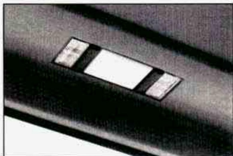
If your vehicle has reading lights, press the bar next to the light to turn the light on. Press the bar again to turn the light off.
