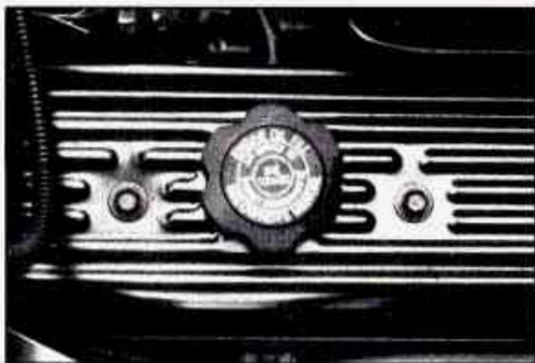
The engine oil filler cap is located on the driver's side engine valve cover.
