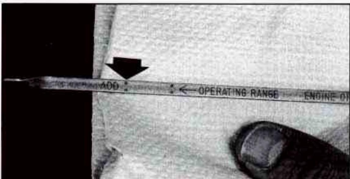
Pull out the dipstick and clean it with a paper towel or cloth, then push it back in all the way. Remove it again, keeping the tip lower.
