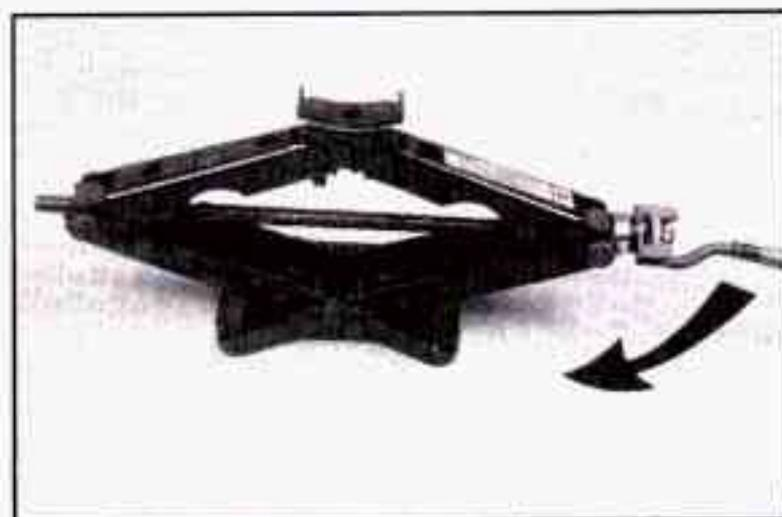
With the **UP** marking on the ratchet facing you, rotate the ratchet to the right.
