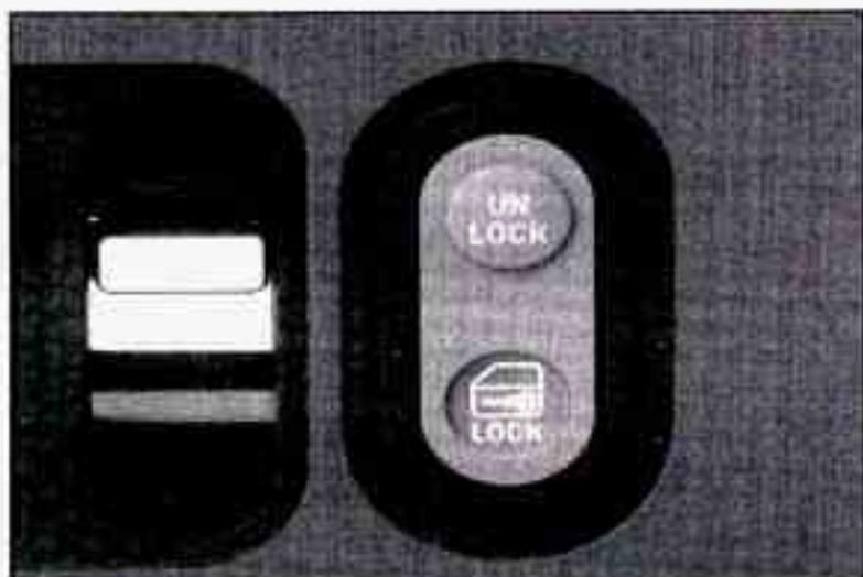
Press the bottom of the power door lock switch, marked **LOCK**, on either front door to lock all the doors at once. Press the switch marked **UNLOCK** to unlock all the doors at once.
