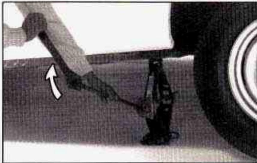
5. Raise the vehicle by rotating the ratchet clockwise. Make sure the UP mark faces you. Raise the vehicle far enough off the ground so there is enough room for the spare tire to fit.
