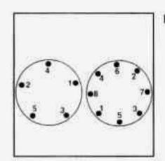
Tighten the nuts firmly in a criss-cross sequence as shown. Rotate the wheel wrench clockwise.
