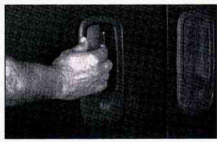
To open the sliding side door from outside, pull the handle toward the rear of the vehicle. Then, slide the door toward the rear of the vehicle to open.
