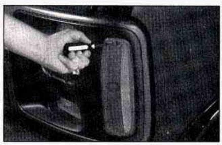
1. Remove the screw from the top of the lens.
