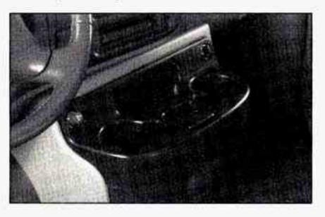
Your front storage compartment is at the center of the instrument panel extension, by the floor. To open the compartment, squeeze and pull the handle at the top.
