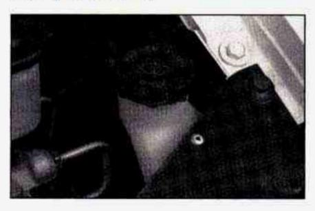
Open the cap labeled WASHER FLUID. Add washer fluid until the tank is full.
