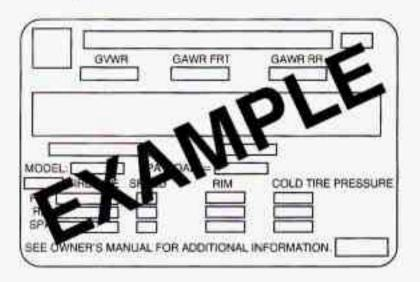
The Certification/Tire label is found on the rear edge of the driver's door. The label shows the size of your original tires and the inflation pressures needed to obtain the gross weight capacity your vehicle. This is called GVWR (Gross Vehicle Weight Rating). The GVWR includes the weight of the vehicle, all occupants, fuel and cargo.
