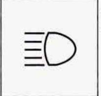
When the high beams are on, this light on the instrument panel also will be on.
