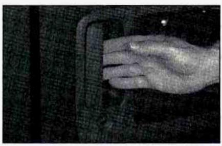
To open the rear doors from the outside, open the passenger side rear door first. Pull the the handle toward you to open the door.
