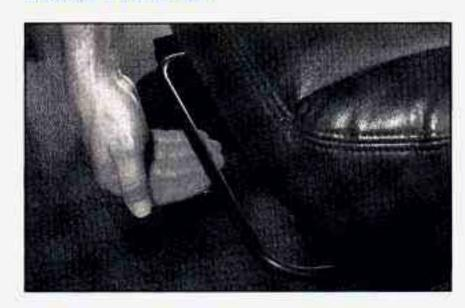
The bucket seats can be adjusted forward or rearward with the lever at the front of the seat.
