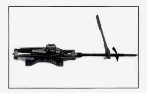
The jack has a bolt on the end. Attach the socket end of the extension to the jack bolt.
