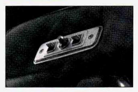
If your vehicle has a power seat on the driver or passenger's side, you can adjust it with this switch at the front center cushion of the seat. You can use the center knob to move the seat where you want it. To raise the seat, move the center knob up. To lower the seat, move the center knob down. To move the seat forward, move the center knob toward the front of the vehicle. To move the seat rearward, move the center knob toward the rear of the vehicle.
