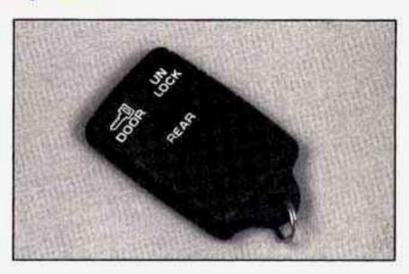
To unlock the driver's door, press the UNLOCK button. If you press this button again within five seconds, all the doors will unlock. Press the REAR button to unlock the rear door only. When the UNLOCK or REAR button is pressed, the interior dome lamps are turned on for 40 seconds or until the ignition switch is activated.
