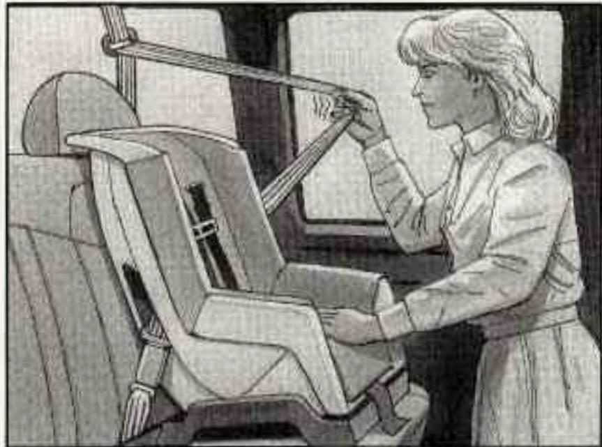
5. Pull the rest of the shoulder belt all the way out of the retractor to set the lock.
