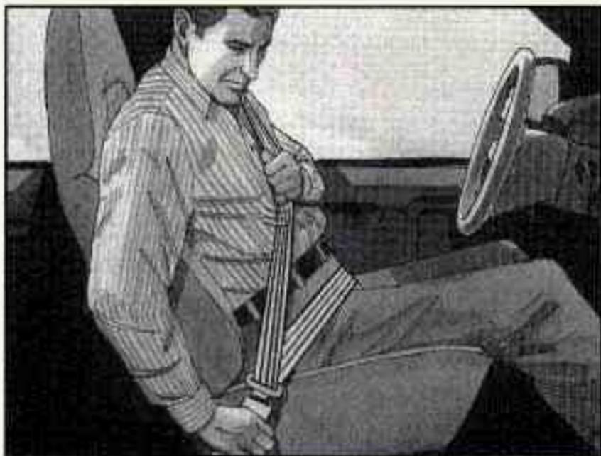
5. To make the lap part tight, pull down on the buckle end of the belt as you pull up on the shoulder belt.
