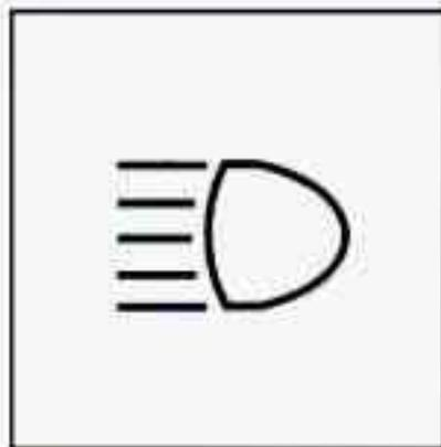
When the high beams are on, this light on the instrument panel also will be on.
