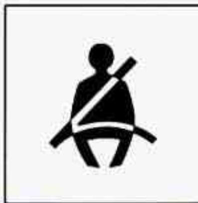
The safety belt light will also come on and stay on for about 20 seconds, then it will flash for about 55 seconds. If the driver's belt is already buckled, neither the tone nor the light will come on.
