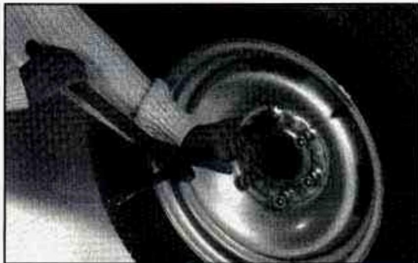
1. With the DOWN side facing you, use the ratchet and socket to loosen all the wheel nuts. Don't remove them yet.
