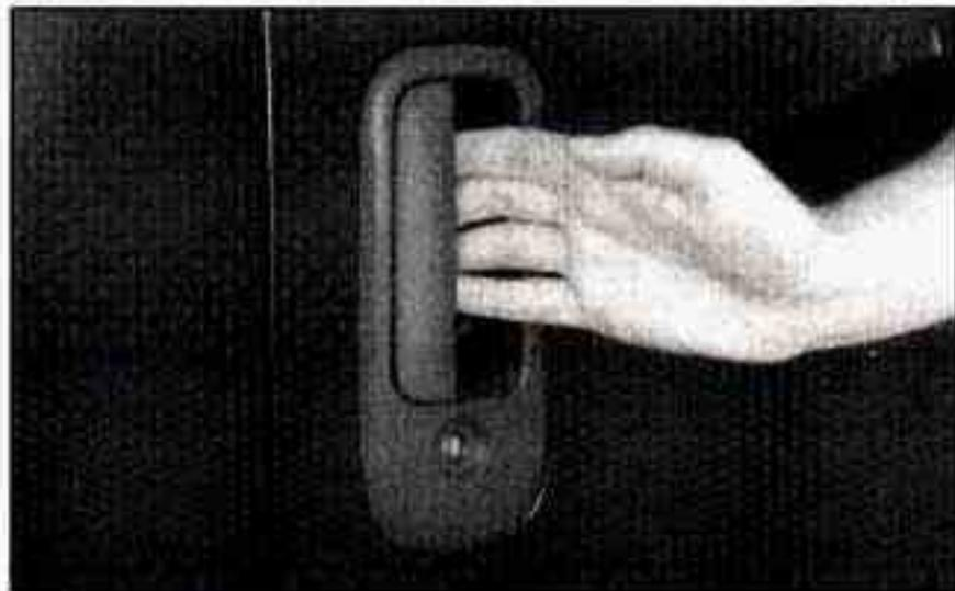
To open the "60" (front) portion of a 60/40 door from the outside, pull up on the handle and pull the handle toward you.
