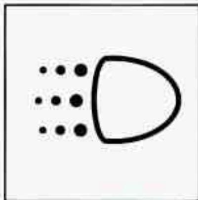
You may have this light on the instrument panel. It will light whenever the DRL are on. It is also a reminder to turn on your headlamps when driving at night. For more details about DRL, see "Headlamps and Vehicle Lighting" in this section.
