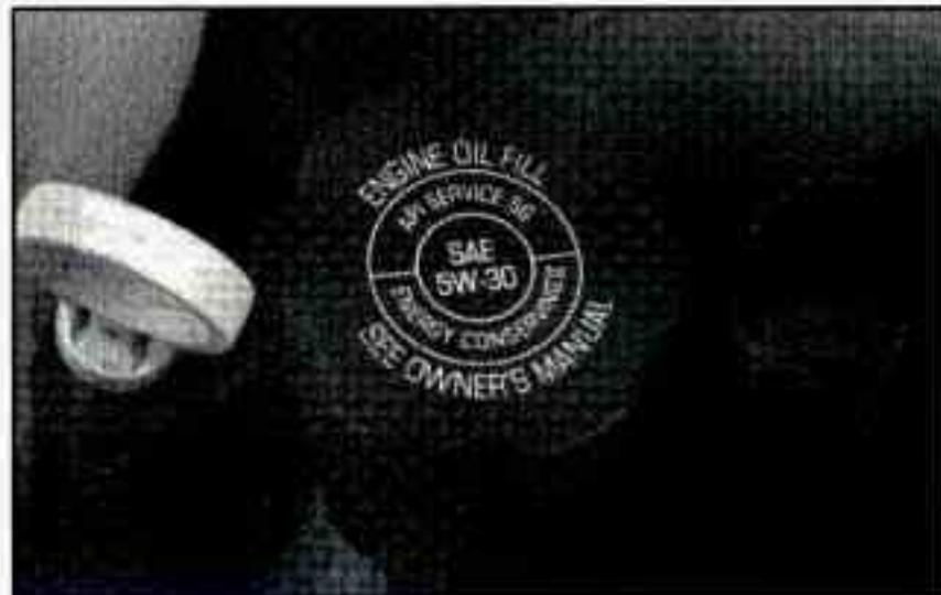
The engine oil filler cap is located between the air cleaner and engine oil dipstick.
