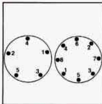
10. Tighten the nuts firmly in a criss-cross sequence as shown. Rotate the wheel wrench clockwise.
