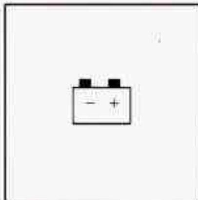
This light should come on briefly when you turn on the ignition, before starting the engine, as a check to show you it is working.
