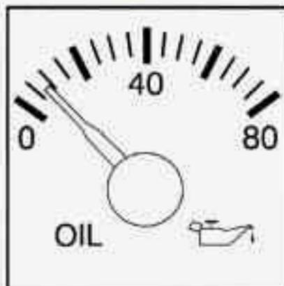
The oil pressure gage shows the engine oil pressure in psi (pounds per square inch) when the engine is running. Canadian vehicles indicate pressure in kPa (kilopascals).
