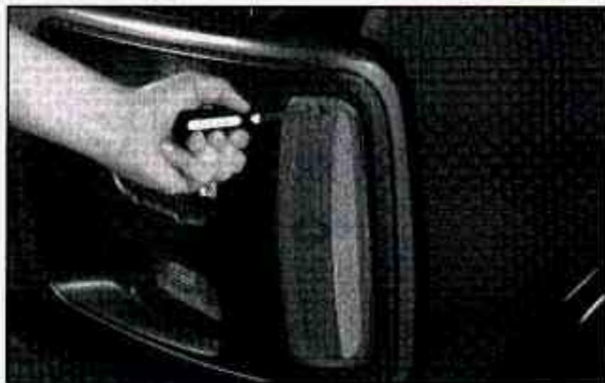
1. Remove the screw from the top of the lens.
