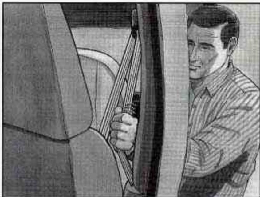
7. To tighten the belt, feed the shoulder belt back into the retractor while you push down on the child restraint.
