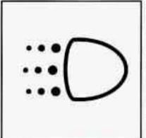
You may have this light on the instrument panel. It will light whenever the DRL are on. It is also a reminder to turn on your headlamps when driving at night. For more details about DRL, see "Headlamps and Vehicle Lighting" in this section.
