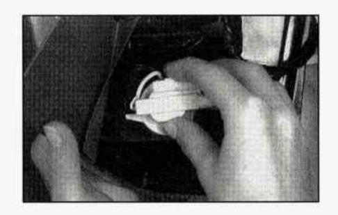
6. Turn the sockets counterclockwise to remove.
