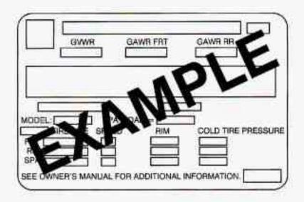
The Certification/Tire label is found on the rear edge of the driver's door. The label shows the size of your original tires and the inflation pressures needed to obtain the gross weight capacity of your vehicle. This is called GVWR (Gross Vehicle Weight Rating). The GVWR includes the weight of the vehicle, all occupants, fuel and cargo.
