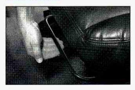
The buckets seats can be adjusted forward or rearward with the lever at the front of the seat. To adjust the seat, pull the lever up to release the seat bottom and slide the seat where you want it. Then release the lever and try to move the seat with your body, to make sure the seat is locked into place.
