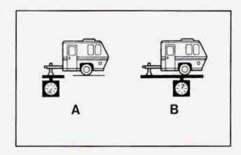
If you're using your platform hitch as a weight-carrying hitch, the trailer tongue (A) should weigh 10 percent of the total loaded trailer weight (B). If you're using your platform hitch as a weight-distributing hitch, the trailer tongue (A) should weigh 12 percent of the total loaded trailer weight (B).
