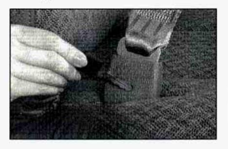
Disconnect the quick release latch plates for the lap shoulder belts on the bench seat to be removed. To do this, press the tip of a key into the release hole of the safety belt buckle while pulling up on the safety belt.
