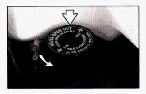
You can remove the radiator pressure cap when the cooling system, including the radiator pressure cap and upper radiator hose, is no longer hot. Turn the pressure cap slowly counterclockwise until it first stops. (Don't press down while turning the pressure cap.)
