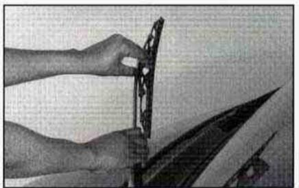
See "Normal Maintenance Replacement Parts" in the Index for the proper type of replacement blade.
