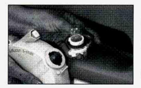
Remove the bulb assembly from the back of the lens and replace the bulb.
