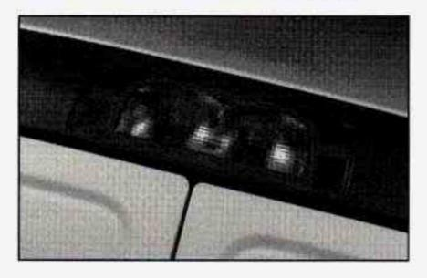
Your vehicle's center high-mounted stoplamp is located above the rear doors at the center of the vehicle. If items are loaded on the roof of the vehicle, as in a luggage carrier, care should be taken not to block or damage the center high-mounted stoplamp unit.
