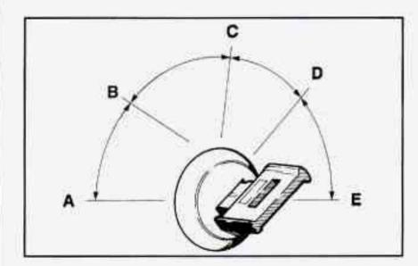
ACCESSORY (A): ACCESSORY lets you use things like the radio, power windows and the windshield wipers when the engine is off. To get into ACCESSORY, push in the key and turn it toward you. Your steering wheel will remain locked, just as it was before you inserted the key. LOCK (B): This position locks your ignition, steering wheel and transmission. It's a theft-deterrent feature. You will only be able to remove your key when the ignition is turned to LOCK.
