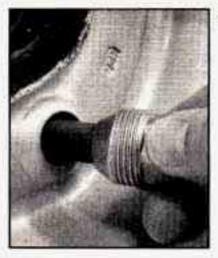
8. Replace the wheel nuts with the rounded end of the nuts toward the wheel. Tighten each wheel nut by hand until the wheel is held against the hub.
