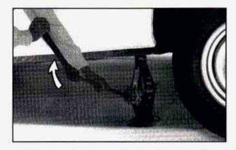
Raise the vehicle by rotating the ratchet clockwise. Make sure the UP mark faces you. Raise the vehicle far enough off the ground so there is enough room for the spare tire to fit.
