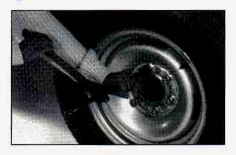
With the DOWN side facing you, use the ratchet and socket to loosen all the wheel nuts. Don't remove them yet.
