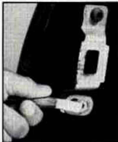
1. Raise the tailgate slightly and release both retaining cable clips. To release the cable clips, lift the cable so it points straight out and push the cable clips forward.
