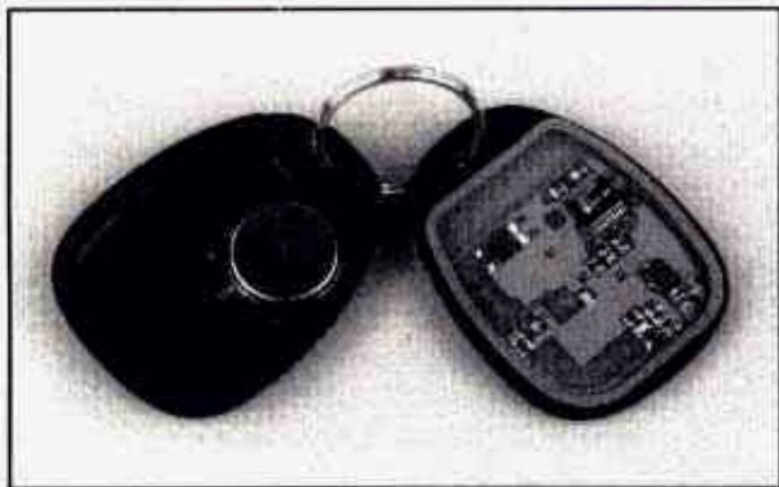
1. Insert a small coin, or flathead screwdriver, to separate the bottom of the transmitter from the top.
