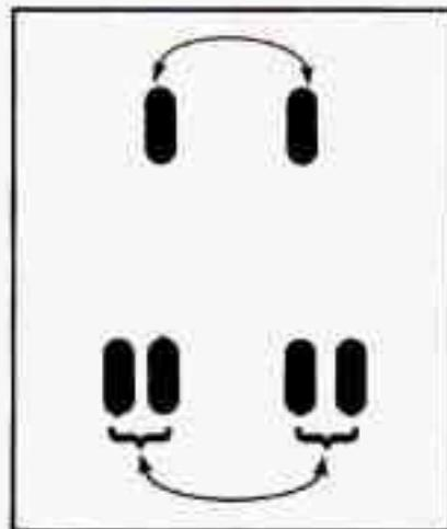
If your vehicle has dual rear wheels and the load range or tread design for your front tires is different from your rear tires, always use the correct rotation pattern shown here when rotating your tires.
