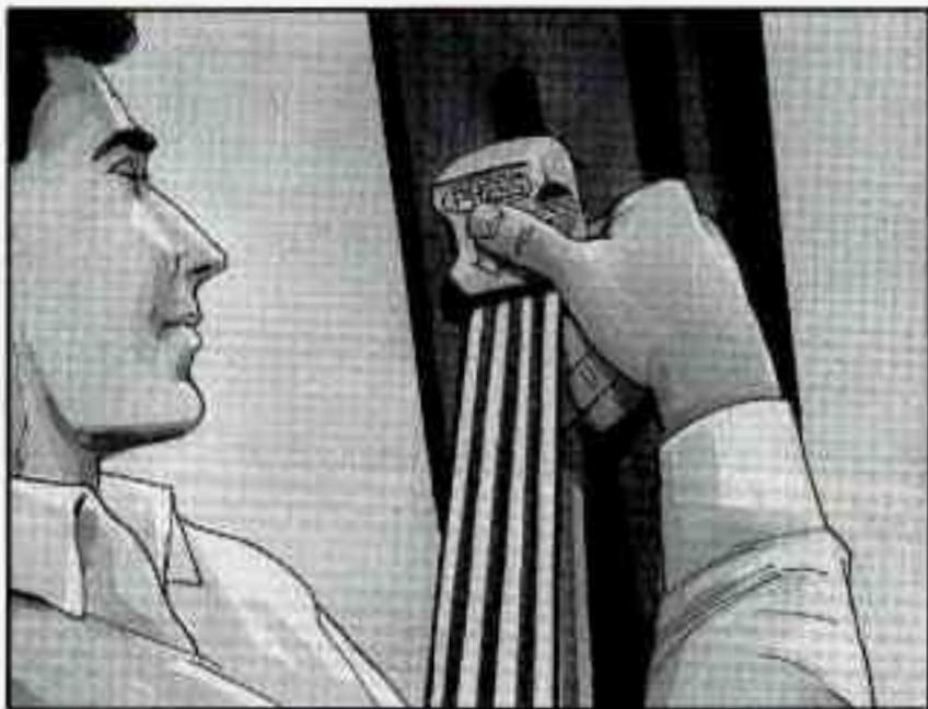
To move it down, push in at the word **PRESS** and move the height adjuster to the desired position. You can move the adjuster up just by pushing up on the shoulder belt guide. After you move the adjuster to where you want it, try to move it down without pushing in to make sure it has locked into position.
