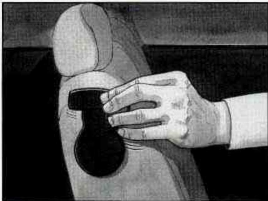
1. Remove the guide from its storage clip on the side of the seatback.
