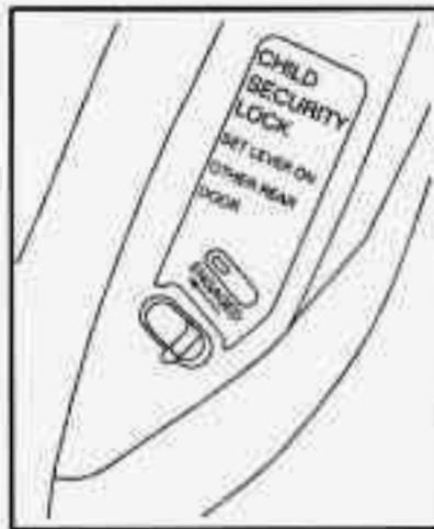
With this feature, you can lock the rear doors so they can't be opened from the inside by the passengers.
