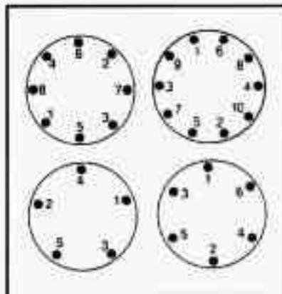
8. Tighten the nuts firmly in a criss-cross sequence as shown by rotating the wheel wrench clockwise.
