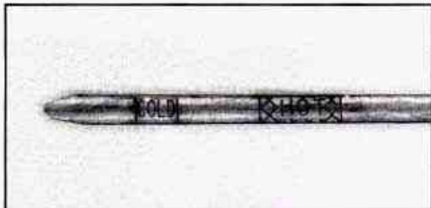
3. Check both sides of the dipstick, and read the lower level. The fluid level must be in the COLD area for a cold check or in the HOT area or cross-hatched area for a hot check.
