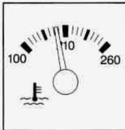
This gage shows the engine coolant temperature.
