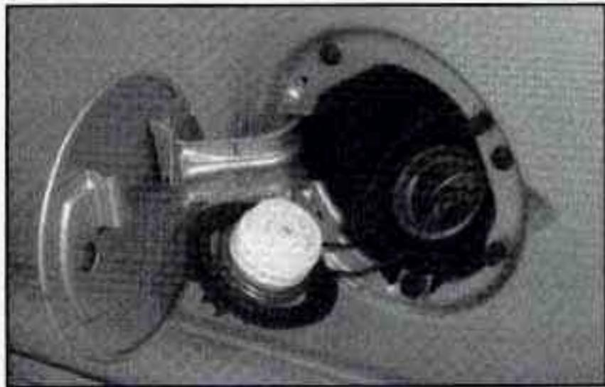
While refueling vehicles equipped with the "VORTEC" 4300 engine, let the cap hang by the tether below the fuel filler neck.
