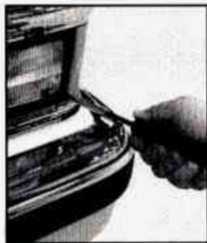
1. Remove the screws and take out the parking/turn signal lamp assembly.
