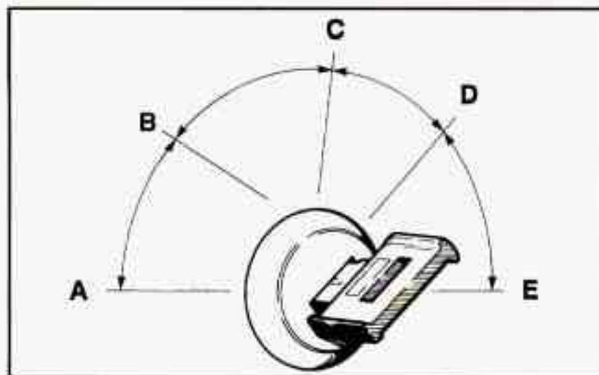
**ACCESSORY (A):** ACCESSORY lets you use things like the radio, power windows and the windshield wipers when the engine is off. Push in the key and turn it towards you. Your steering wheel will remain locked, just as it was before you inserted the key.
