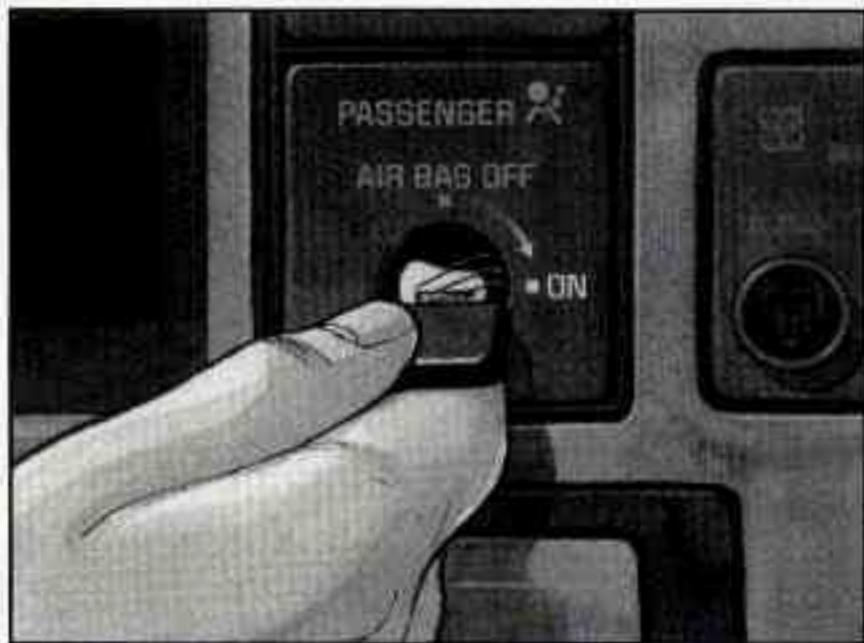
To turn the air bag on again, insert your ignition key into the switch, push in, and move the switch to the ON position.
