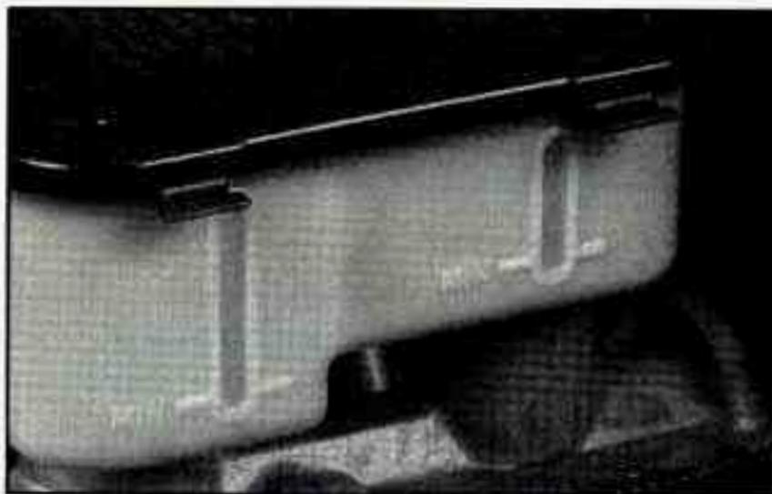
You can check the brake fluid without taking off the cap. Just look at the window on the brake fluid reservoir. The fluid level should be above MIN. If it isn't, have your brake system checked to see if there is a leak.
