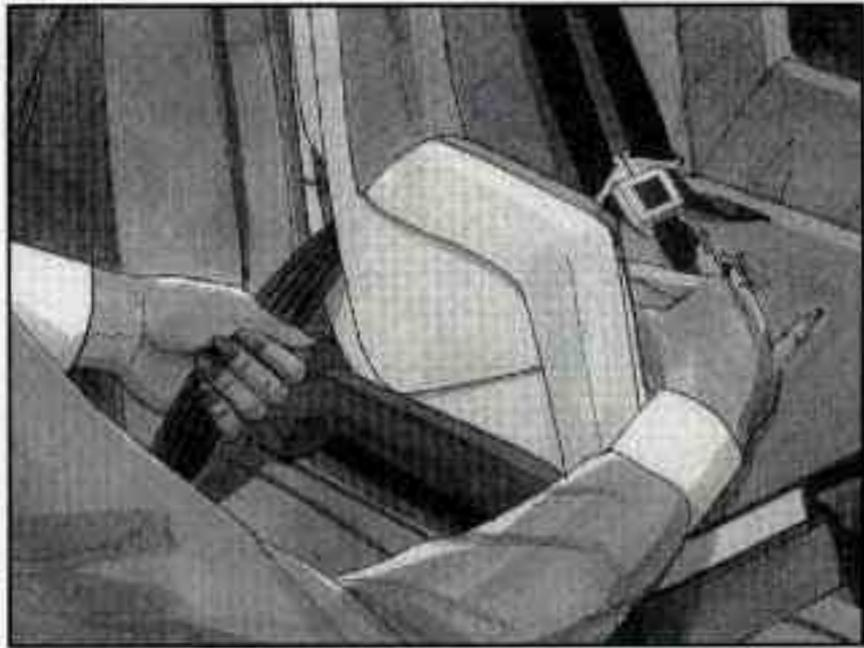
6. To tighten the belt, feed the lap belt back into the retractor while you push down on the child restraint.
