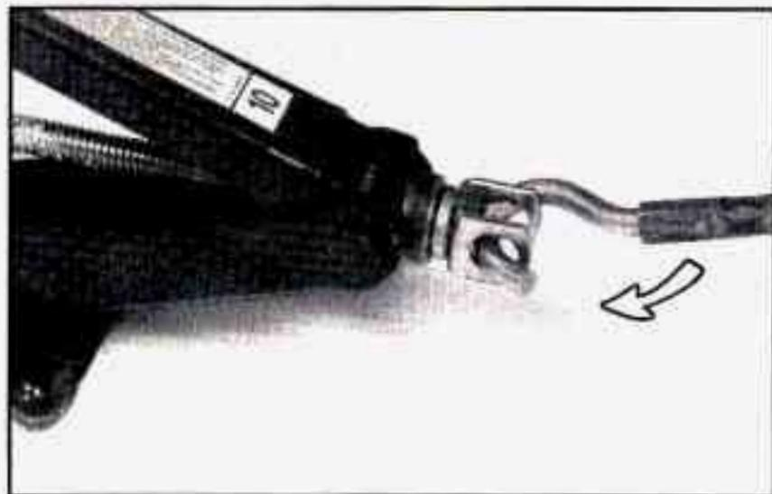
With the UP marking on the ratchet facing you, rotate the ratchet clockwise. That will lift the jack head a little.
