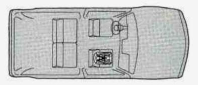
Your vehicle has a right front passenger air bag. Never put a rear-facing child restraint in this seat. Here's why:
