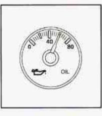
The oil pressure gage shows the engine oil pressure in psi (pounds per square inch) when the engine is running.
