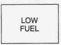
This light comes on when the fuel tank is low on fuel.
