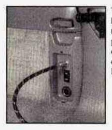
Then attach that end of the hose to the object you wish to inflate. Remove the protective cap covering the outlet. Attach the other end of the hose to the outlet. Press the ON switch. If the air inflator system does not turn on, the fuse may be blown or installed incorrectly. See "Fuses and Circuit Breakers" in the Index or see your dealer for service.
