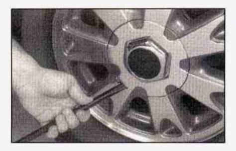
Position the chisel end of your wheel wrench in the notch of the hub cap and pry off the hub cap.
