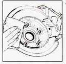
Remove any rust or dirt from the wheel bolts, mounting surfaces and spare wheel.
