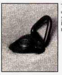
There are four cargo tie downs in the rear that allow you to strap cargo in and keep it from moving inside the vehicle.
