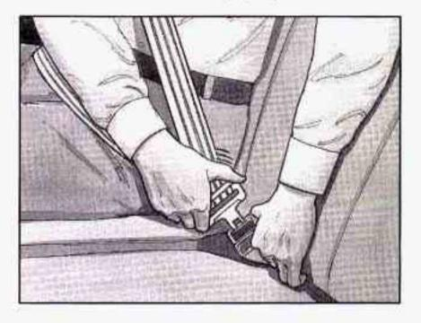
Pick up the latch plate and pull the belt across you. Don't let it get twisted. The shoulder belt may lock if you pull the belt across you very quickly. If this happens, let the belt go back slightly to unlock it. Then pull the belt across you more slowly. Push the latch plate into the buckle until it clicks.
