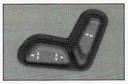
Horizontal Control: Raise the front of the seat by raising the forward edge of the button. Lower the front of the seat by lowering the forward edge of the button. Move the seat forward by moving the whole button toward the front of the vehicle.
