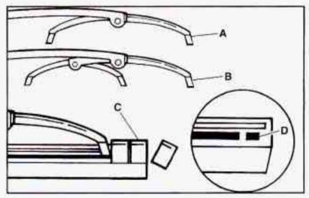
To install the new wiper insert, slide the insert (D), notched end last, into the end with two blade claws (A). Slide the insert all the way through the blade claws at the opposite end (B). The plastic caps (C) will be forced off as the insert is fully inserted. Be sure that the notches are locked by the bottom claws. Make sure that all other claws are properly locked on both sides of the insert slots.
