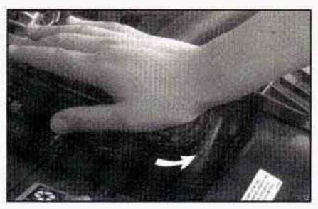
Then keep turning the pressure cap, but now push down as you turn it. Remove the pressure cap.
