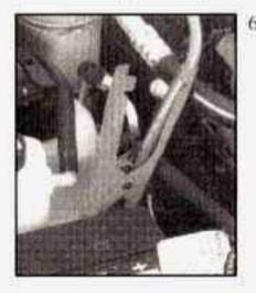
Connect the red positive (+) cable to the positive (+) terminal of the vehicle with the dead battery.
