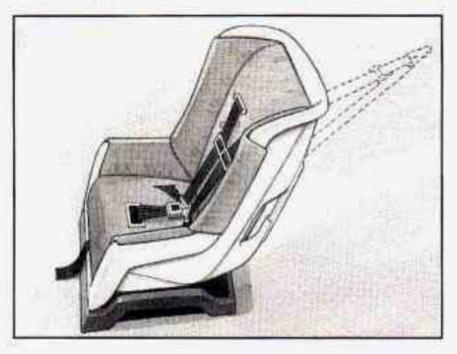
If your child restraint has a top strap, it should be anchored. Anchor brackets for the rear outside seat positions are located on the floor in the cargo area.
