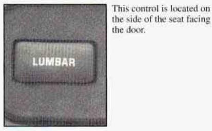
Press and hold the front of the control until you have the desired lumbar support. To decrease lumbar support, press and hold the rear of the control.
