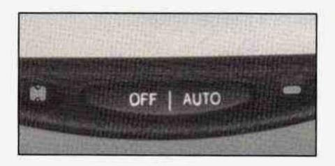
Press the OFF AUTO button at the base of the mirror to turn on the automatic feature. The button has an indicator light to show it is on. Press the OFF AUTO button to turn the automatic feature off.
