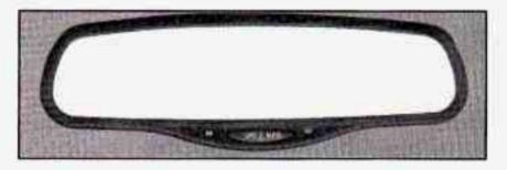
This mirror automatically changes to reduce glare from headlamps behind you. A photocell on the back of the mirror senses when it is becoming dark outside. Another photocell built into the mirror surface senses when headlamps are behind you.
