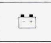
The charging system light will come on briefly when you turn on the ignition, but the engine is not running, as a check to show you it is working.
