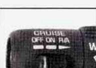
With cruise control, you can maintain a speed of about 25 mph (40 km/h) or more without keeping your foot on the accelerator. This can really help on long trips. Cruise control does not work at speeds below about 25 mph (40 km/h).
