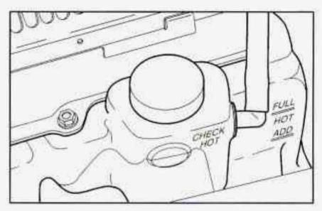
The coolant level should be at least up to the ADD mark.
