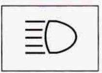
When the high beams are on, this indicator light on the instrument panel will also be on.
