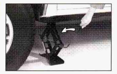
Lower the vehicle by turning the jack handle to the left. Lower the jack completely.
