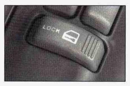
The power door lock switch is located on the armrest. Remove the ignition key and press LOCK to lock all the doors at once.
