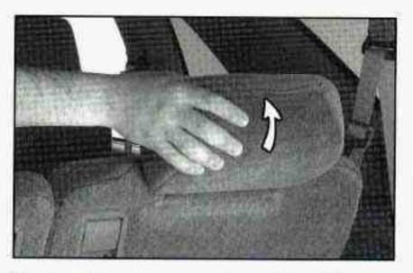
To return the head restraints to the upright position, reach behind the seats and pull the head restraint up until it locks into position.
