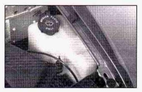
Open the cap labeled WASHER FLUID ONLY with the washer symbol on it. Add washer fluid until the tank is full.
