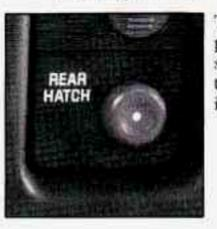
This button on the passenger's side of the steering column allows you to release the liftglass from inside the vehicle.
