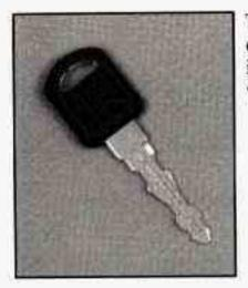
This vehicle has one double-sided key for the ignition and door locks. It will fit with either side up.
