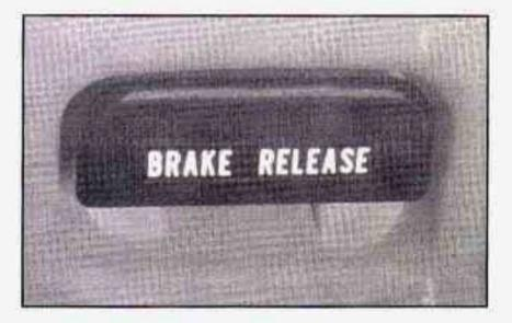
Pull the BRAKE RELEASE lever. It is located on the bottom of the driver's side of the instrument panel.
