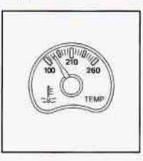
This gage shows the engine coolant temperature. If the gage pointer moves into the red area, your engine is too hot!
