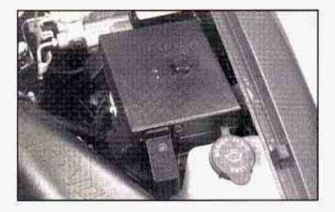
The fuse block is under the hood at the driver's side of the engine compartment.
