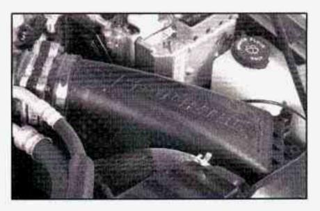
To remove the air cleaner, remove the wing nuts that hold the cover on. Remove the cover and lift out the air filter.
