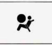
There is an air bag readiness light on the instrument panel, which shows the air bag symbol.
