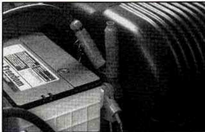
6. Connect the red positive (+) cable to the positive (+) terminal of the vehicle with the dead battery.
