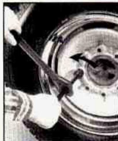
1. Use the ratchet and wheel wrench to loosen all the wheel nuts. Turn the wheel wrench to the left, with DOWN facing you, to loosen the wheel nuts. Don't remove the wheel nuts yet.
