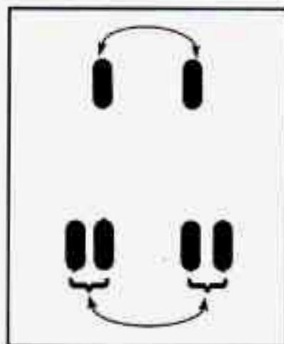
If your vehicle has dual rear wheels and the load range or tread design for your front tires is different from your rear tires, always use the correct rotation pattern shown here when rotating your tires. The dual tires are rotated as a pair, and the inside rear tires become the outside rear tires.
