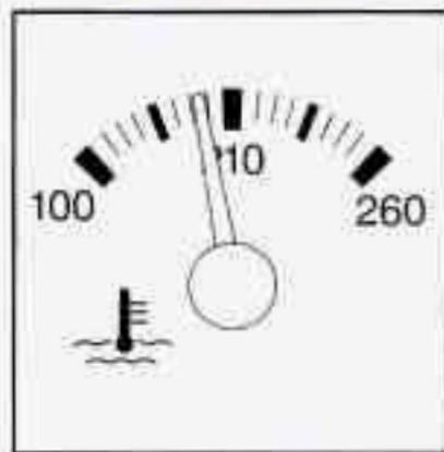
This gage shows the engine coolant temperature.
