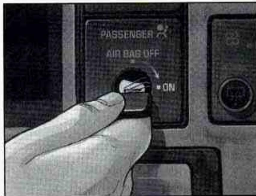
To turn the air bag on again, insert your ignition key into the switch, push in, and move the switch to the ON position.
