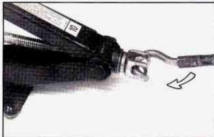
With the UP marking on the ratchet facing you, rotate the ratchet to the right. That will lift the jack head a little.
