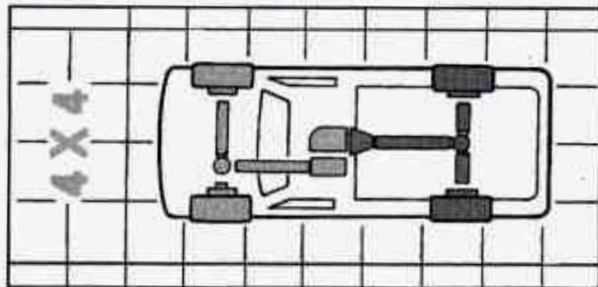
The front axle portion of the indicator diagram will light up when you shift into four-wheel drive and the front axle engages.
