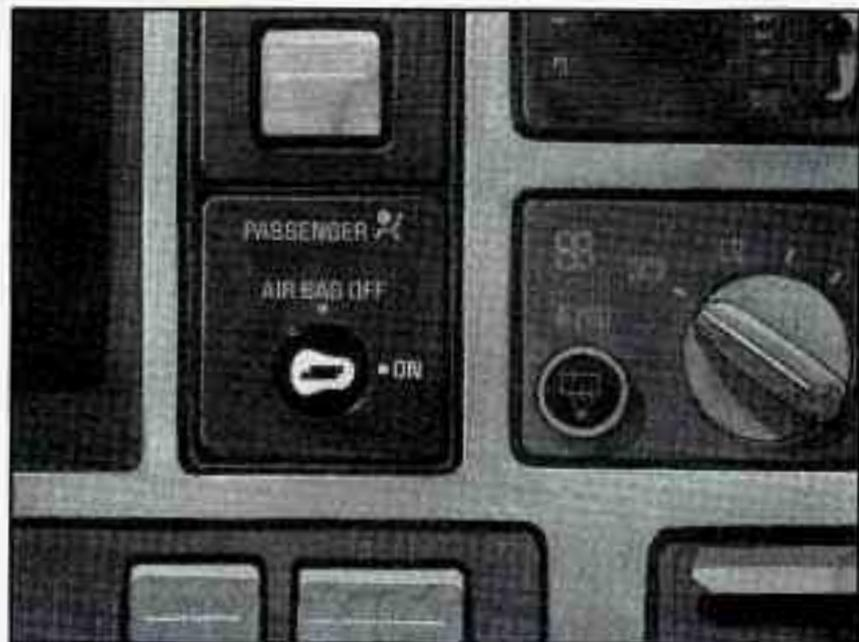
If your vehicle has air bags, there is a switch on the instrument panel that you can use to turn off the right front passenger's air bag. But use this switch only when you want to secure a rear-facing child restraint at the right front passenger's position.
