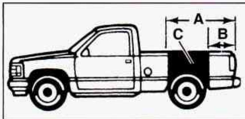
Use the rear edge of the load floor for measurement purposes. The recommended location for the cargo center of gravity is at point C for the CWR. It is the point where the mass of a body is concentrated and, if suspended at that point, would balance the front and rear.
