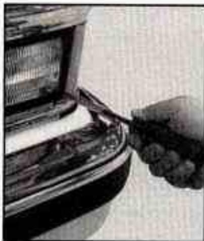
1. Remove the four screws and take out the parking/turn signal lamp assembly.
