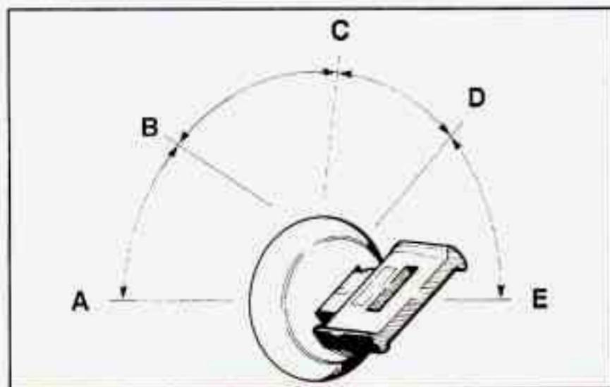
**ACCESSORY (A):** ACCESSORY lets you use things like the radio, power windows and the windshield wipers when the engine is off. Push in the key and turn it toward you. Your steering wheel will remain locked, just as it was before you inserted the key.
