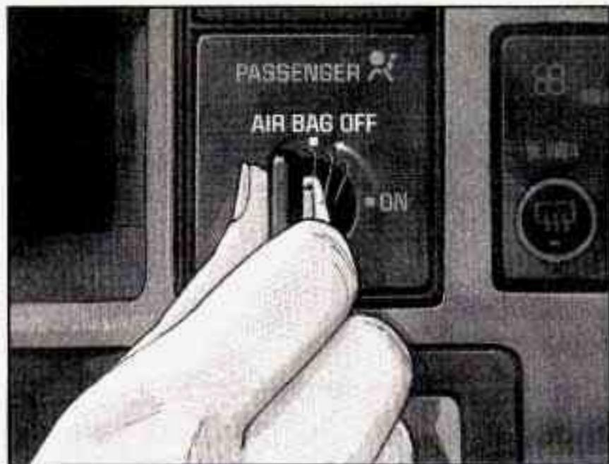
To turn off the right front passenger's air bag, insert your ignition key into the switch, push in, and move the switch to AIR BAG OFF.
