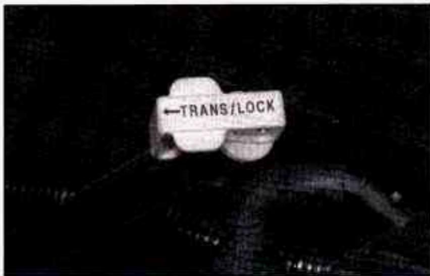
1. The red transmission dipstick handle is located at the rear of the engine compartment, on the passenger's side. Flip the handle up and then pull out the dipstick and wipe it with a clean rag or paper towel.
