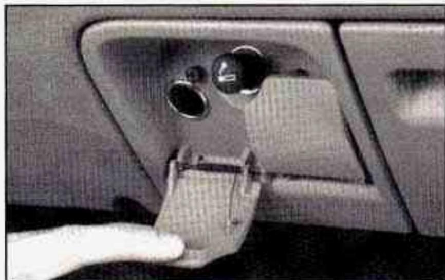
Two auxiliary power outlets are located near the cigarette lighter. Use these outlets to power mobile telephones or other devices designed to operate with vehicle electrical systems.
