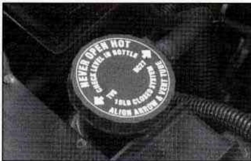
The radiator pressure cap must be tightly installed with the arrows on the cap lined up with the overflow tube on the radiator filler neck.
