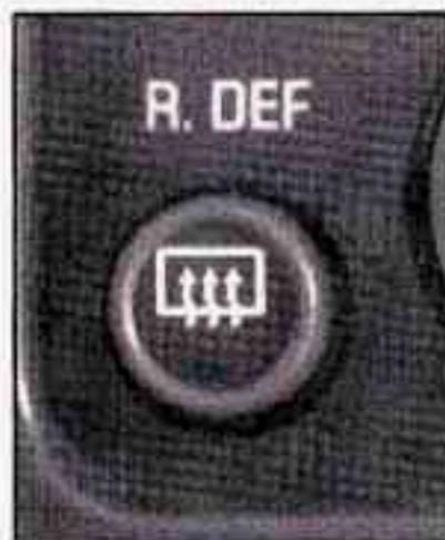
To turn on the rear window defogger, press this button next to the fan control knob. The rear window defogger will only work if the ignition switch is turned to RUN. For best results, clear the window of as much snow or ice as possible first.
