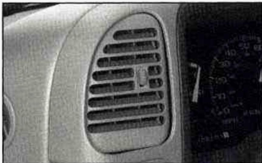
Your vehicle has air outlets in the center and on the sides of your instrument panel. You can move the outlets from side-to-side or up and down to direct the flow of air, or close the outlets altogether. When you close an outlet, it will increase the flow of air coming out of any outlets that are open. These outlets do not completely shut off airflow when in the closed position.
