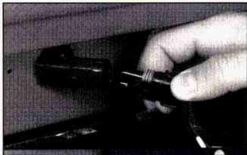
1. Remove the screws and lamp assembly.
