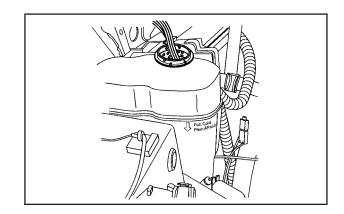
Fill the coolant surge tank with the proper mixture to the FULL COLD mark.  With the coolant surge tank pressure cap off, start the engine and let it run until the engine coolant temperature gage indicates approximately 195°F (90°C).
