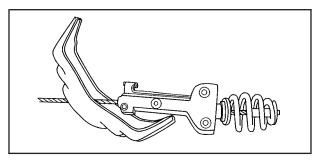
Separate the tire/wheel retainer (D) from the guide pin. Pull the pin through the center of the wheel. Tilt the retainer down and through the center wheel opening.
