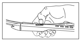
Squeeze the grooved areas on each side of the blade and turn the blade assembly away from the arm connector.
