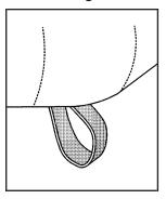
Pull up on the front of the seat cushion while pulling down on the release strap, located under the seat cushion.
