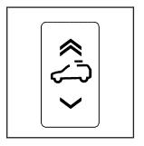
If your vehicle is an extended cab, the sunroof switch is located on the headliner above the rearview mirror.
