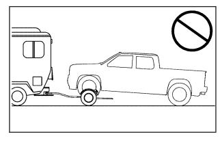
Notice: If a two-wheel-drive vehicle is towed with the rear wheels on the ground, the transmission could be damaged. The repairs would not be covered by the vehicle warranty. Never tow the vehicle with the rear wheels on the ground.
