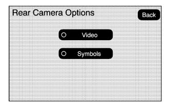
Select the Video screen button. When the Video screen button is highlighted the RVC system is on.
