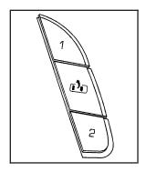
The controls for this feature are located on the driver's door panel, and are used to program and recall memory settings for the driver's seat, outside mirrors, and the adjustable throttle and brake pedal.
