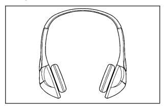
The RSE includes two 2-channel wireless headphones that are dedicated to this system. Channel 1 is dedicated to the video screen, while Channel 2 is dedicated to RSA selections. These headphones can used to listen to the radio, CDs, DVDs, MP3s, DVDAs, any auxiliary source connected to A/V jacks, or the auxiliary input jack, if the vehicle has this feature. The wireless headphones have an On/Off button, channel 1/2 switch, and a volume control.
