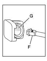
Insert the hoist end (F) through the hole (G) in the rear bumper and onto the hoist shaft.
