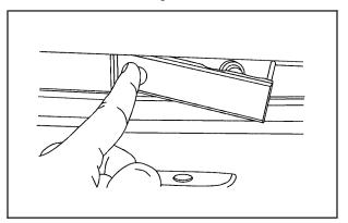
Press and hold the driver side of the handle in and pull out on the exposed portion of the handle to access the storage area.
