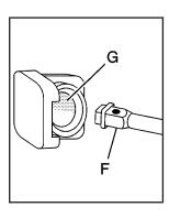
Insert the hoist end (open end) (F) of the extension through the hole (G) in the rear bumper.
