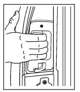
To open a rear access door from the outside, first open the front door. Then, use the handle located on the front edge of the rear access door to open it.
