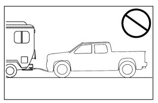
Notice: If the vehicle is towed with all four wheels on the ground, the drivetrain components could be damaged. The repairs would not be covered by the vehicle warranty. Do not tow the vehicle with all four wheels on the ground.
