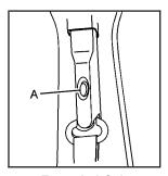
On the extended cab, push down on the release button (A) and move the height adjuster to the desired position.
