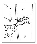
Raise the tailgate slightly and release both retaining cable clips. To release the retaining cable clips, lift the cable so it points straight out. Lift the clip over the bolt, and push the cable forward then rotate down.
