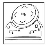
Vehicles with outside power mirrors have controls located on the driver door.
