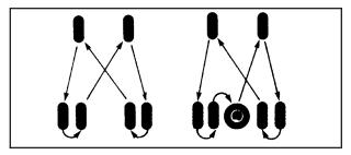
If your vehicle has dual rear wheels and the tread design for the front tires is the same as the rear tires, always use one of the correct rotation patterns shown here when rotating the tires.
