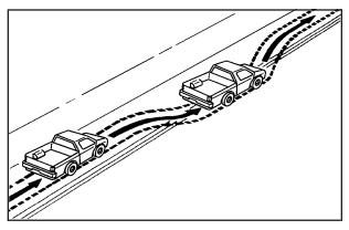
If the level of the shoulder is only slightly below the pavement, recovery should be fairly easy. Ease off the accelerator and then, if there is nothing in the way, steer so that the vehicle straddles the edge of the pavement. Turn the steering wheel 3 to 5 inches, 8 to 13 cm, (about one-eighth turn) until the right front tire contacts the pavement edge. Then turn the steering wheel to go straight down the roadway.
