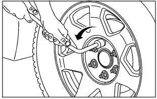
3. Use the wheel wrench and turn it counterclockwise to loosen the wheel nuts. Do not remove the wheel nuts yet.
