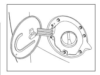
The tethered fuel cap is located behind a hinged fuel door on the driver side of the vehicle. If the vehicle has E85 fuel capability, the fuel cap will be yellow and state that E85 or gasoline can be used. See *Fuel E85 (85% Ethanol) on page 5-9*.
