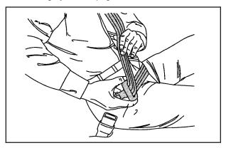
If the belt stops before it reaches the buckle, when using the lap-shoulder belt in a rear center seating position of a crew-cab, tilt the latch plate and keep pulling the safety belt until it can be buckled.
