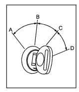
The ignition switch has four different positions.
