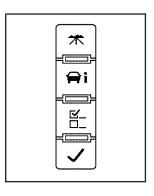
The buttons are the trip/fuel, vehicle information, customization, and set/reset buttons. The button functions are detailed in the following pages.
