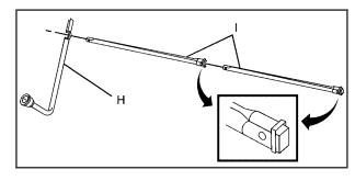
3. Attach the wheel wrench (H) and extensions (I) together, as shown.
