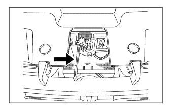
Then go to the front of the vehicle and locate the secondary hood release. This is located under the hood, near the center of the grille.
