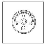
For vehicles with a voltmeter gage, this gage indicates the battery voltage when the ignition is turned on.
