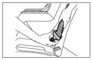
For crew cab second row seatings positions, tilt the latch plate to adjust the belt if needed.
