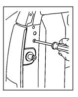
Remove the two rear lamp assembly screws near the tailgate latch strikerpost and pull out the lamp assembly.
