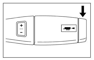
Vehicles with an Allison or Hydra-Matic® 6-speed automatic transmission® have a tow/haul mode. The tow/haul mode adjusts the transmission shift pattern to reduce shift cycling, providing increased performance, vehicle control, and transmission cooling when towing or hauling heavy loads.
