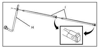
2. Assemble the wheel wrench (H) and the two jack handle extensions (I) as shown.
