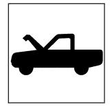
Pull the handle with this symbol on it. It is located inside the vehicle to the left of the brake pedal.
