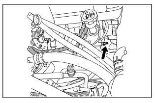
The remote negative (–) terminal is a stud located on the right front passenger side of the engine, where the negative battery cable attaches.
