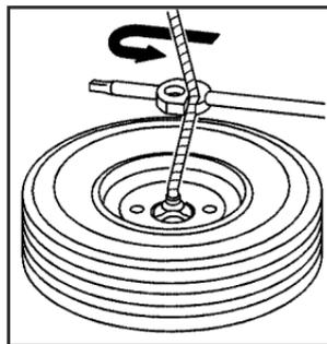
5. Use the wheel wrench hook which allows you to pull the hoist cable towards you to assist in reaching the spare tire.
