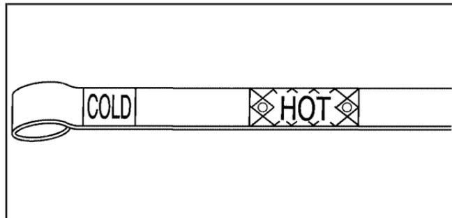
4. Check both sides of the dipstick, and read the lower level. The fluid level must be in the COLD area, below the cross-hatched area, for a cold check or in the HOT or cross-hatched area for a hot check. Be sure to keep the dipstick pointed down to get an accurate reading.
