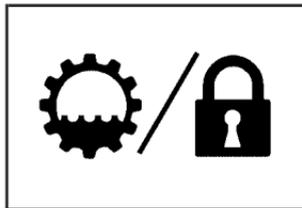
1. Locate the transmission dipstick handle with this graphic which is located at the rear of the engine compartment, on the passenger side of the vehicle.
