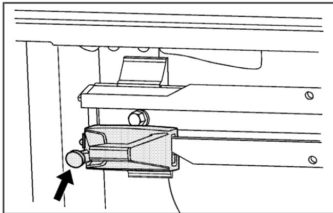
To adjust a tie-down, pull the locator pin out and move the tie-down to another location making sure the locator pin lines up with a locator hole on the rail. The tie-down pin may not be installed correctly if the pin
