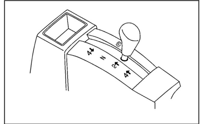
The transfer case shift lever is on the floor to the right of the driver. Use this lever to shift into and out of Four-Wheel Drive.
