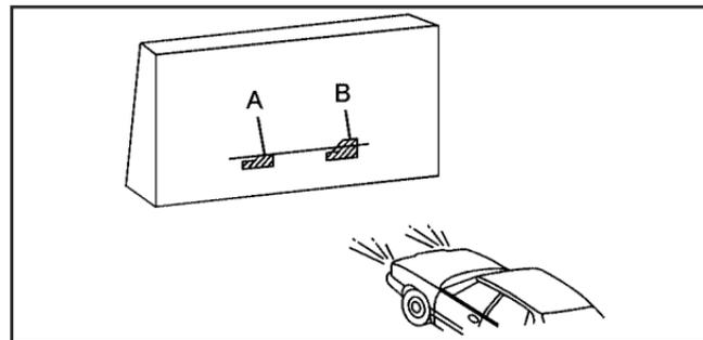
7. Locate the vertical headlamp aiming screws, which are under the hood near each headlamp assembly. The adjustment screw can be turned with a E8 Torx<sup>®</sup> socket.
