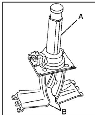
7. Place the bottom edge of the jack (A) on the wheel blocks (B), separating them so that the jack is balanced securely.
