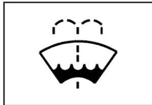
Open the cap with the washer symbol on it. Add washer fluid until the tank is full. See *Engine Compartment Overview on page 5-16* for reservoir location.
