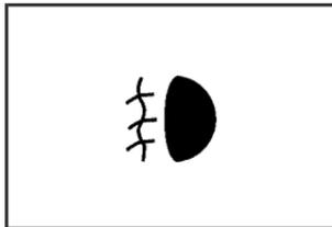
The fog lamp light comes on when the fog lamps are in use.
