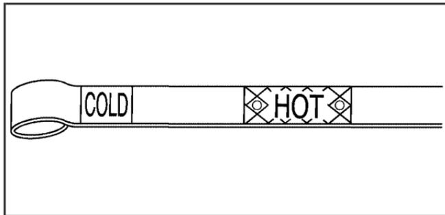
5. If the fluid level is below the COLD check band, add only enough fluid as necessary to bring the level into the COLD band. It does not take much fluid, generally less than one pint (0.5L). Do not overfill.
