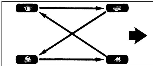
If your vehicle has single rear wheels and the tread design for the front tires is the same as the rear tires, use the rotation pattern shown here when rotating the tires.
