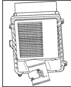
1. Locate the air cleaner/filter assembly. See *Engine Compartment Overview* on page 5-16.
