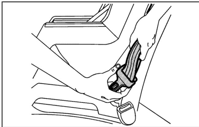
For crew cab second row seatings positions, tilt the latch plate to adjust the belt if needed.
