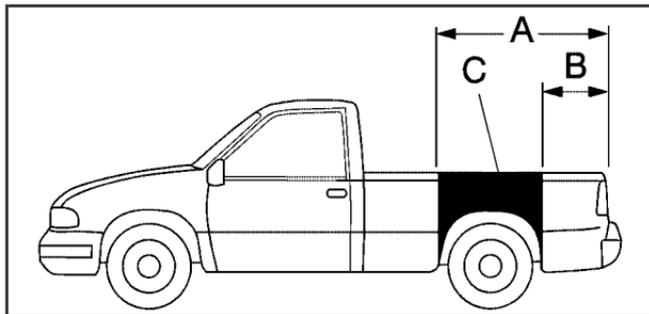
Use the rear edge of the load floor for measurement purposes. The recommended location for the cargo center of gravity is at point C for the CWR. It is the point where the mass of a body is concentrated and, if suspended at that point, would balance the front and rear.
