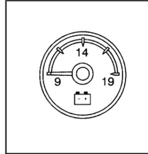
For vehicles with a voltmeter gage, this gage indicates the battery voltage when the ignition is turned on.
