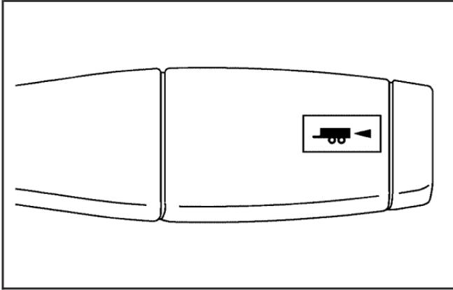
The selector button is located on the end of the shift lever. Turn the tow/haul on and off by pressing the button. When the tow/haul is on, a light on the instrument panel cluster will come on.
