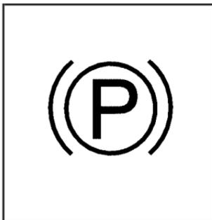
A parking brake symbol is located next to the N (Neutral) symbol as a reminder to set the parking brake before shifting the transfer case into N (Neutral).
