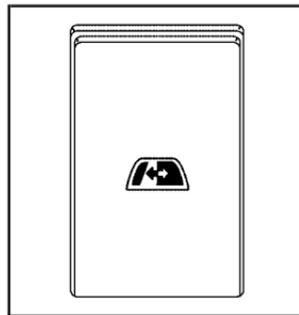
On vehicles with a power sliding rear window, the switch is located in the overhead console.
