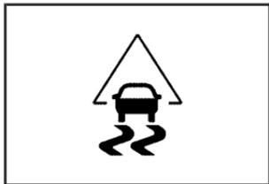
For vehicles with the StabiliTrak<sup>®</sup> system, this light comes on briefly while starting the engine.
