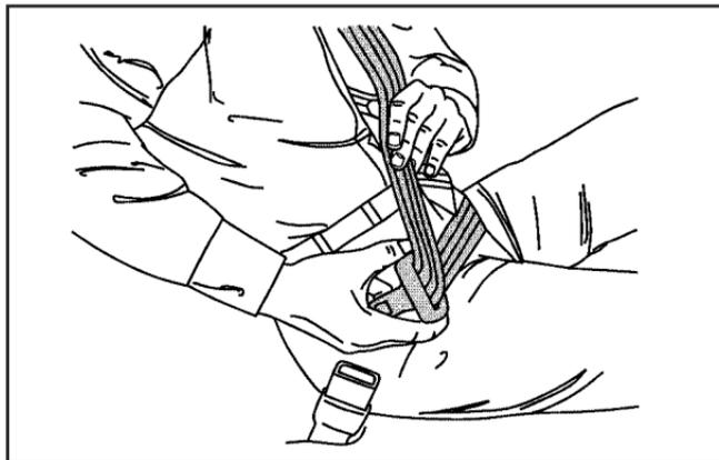
If the belt stops before it reaches the buckle, when using the lap-shoulder belt in a rear center seating position of a crew-cab, tilt the latch plate and keep pulling the safety belt until it can be buckled.
