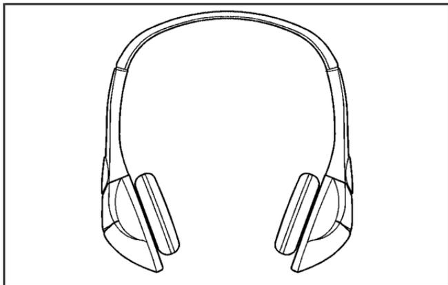
The RSE includes two 2-channel wireless headphones that are dedicated to this system. Channel 1 is dedicated to the video screen, while Channel 2 is dedicated to RSA selections. These headphones can be used to listen to the radio, CDs, DVDs, MP3s, DVDA's, any auxiliary source connected to A/V jacks, or the auxiliary input jack, if the vehicle has this feature. The wireless headphones have an On/Off button, channel 1/2 switch, and a volume control.
