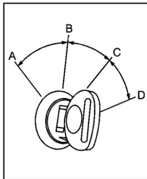
The ignition switch has four different positions.
