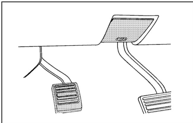
For vehicles with a release handle, set the parking brake by holding the regular brake pedal down, then pushing down the parking brake pedal.
