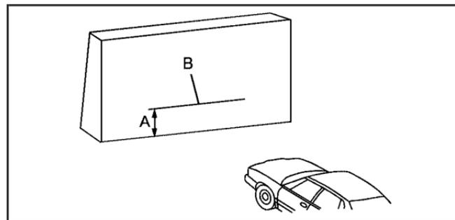
4. At a wall, measure from the ground upward (A) to the recorded distance from Step 3 and mark it.
