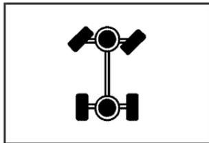
The four-wheel-drive light comes on when a vehicle with a manual transfer case is shifted into four-wheel drive and the front axle engages.
