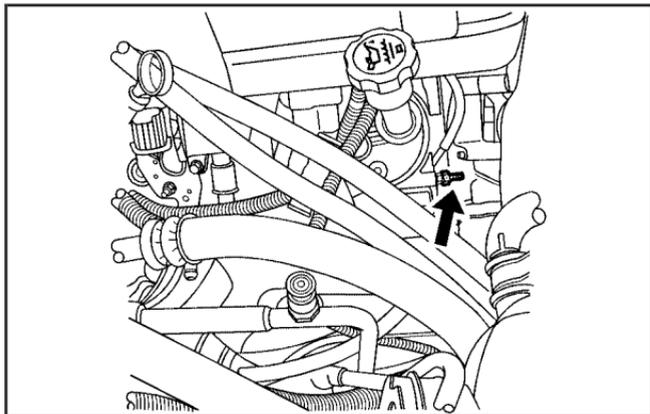
The remote negative (-) terminal is a stud located on the right front passenger side of the engine, where the negative battery cable attaches. See *Engine Compartment Overview* on page 5-16.
