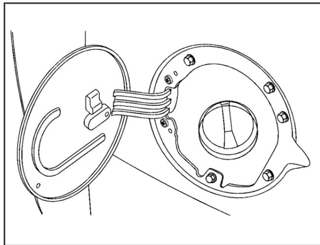
The tethered fuel cap is located behind a hinged fuel door on the driver side of the vehicle. If the vehicle has E85 fuel capability, the fuel cap will be yellow and state that E85 or gasoline can be used. See *Fuel E85 (85% Ethanol)* on page 5-9.
