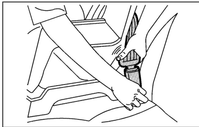
3. Push the latch plate into the buckle until it clicks. Position the release button on the buckle so that the safety belt could be quickly unbuckled if necessary.
