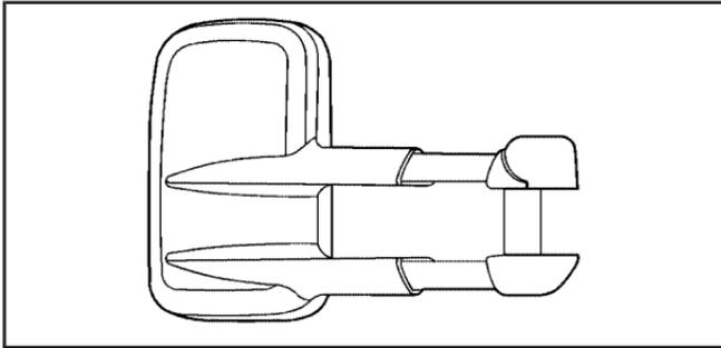
If the vehicle has towing mirrors, they can be adjusted for a clearer view of the objects behind you. Manually pull out the mirror head to extend it for better visibility when towing a trailer.
