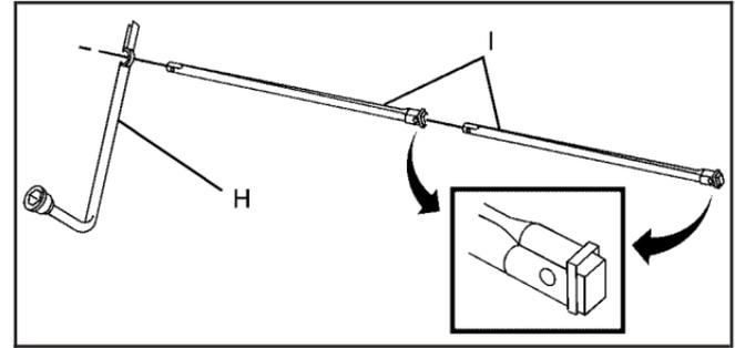
3. Attach the wheel wrench (H) and extensions (I) together, as shown.
