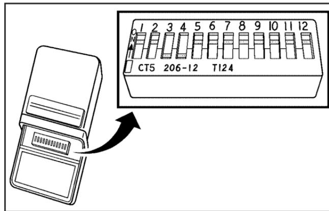
1. To verify that the garage door opener is a Fixed Code unit, remove the battery cover on the hand held transmitter supplied by the manufacturer of the garage door opener motor. If there are a row of dip switches similar to the graphic above, the garage door opener is a Fixed Code unit.
