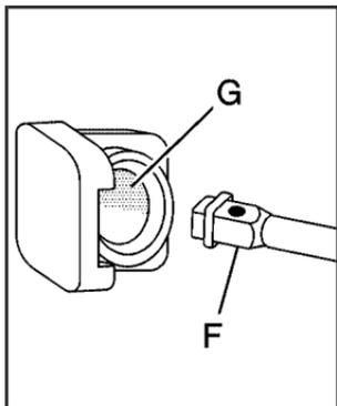
4. Insert the hoist end (F) through the hole (G) in the rear bumper and onto the hoist shaft.
