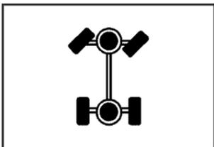
A Four-Wheel Drive indicator light comes on when you shift into four-wheel drive and the front axle engages. See *Four-Wheel-Drive Light* on page 3-51.
