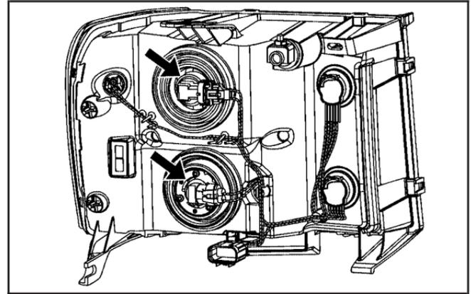
4. Turn the bulb socket counterclockwise to remove it from the headlamp assembly and pull it straight out.
