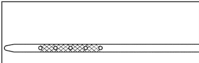
If the oil is below the cross-hatched area at the tip of the dipstick, add at least one quart/liter of the recommended oil. This section explains what kind of oil to use. For engine oil crankcase capacity, see *Capacities and Specifications on page 5-131*.
