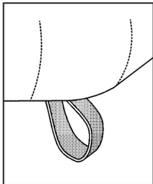
1. Pull up on the front of the seat cushion while pulling down on the release strap, located under the seat cushion.
