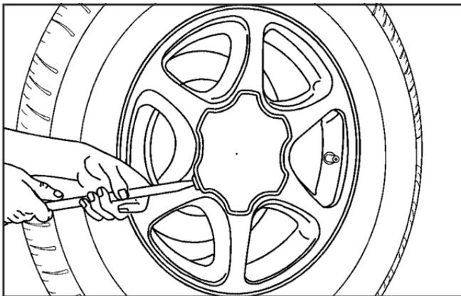
If the wheel has a smooth center cap, place the chisel end of the wheel wrench in the slot on the wheel, and gently pry it out.
