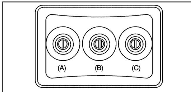
The A/V jacks, located on the rear of the floor console, allow audio or video signals to be connected from an auxiliary device such as a camcorder or a video game unit to the RSE system. Adapter connectors or cables (not included) may be required to connect the auxiliary device to the A/V jacks. Refer to the manufacturer's instructions for proper usage.
