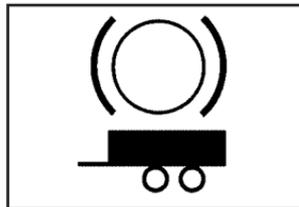
The vehicle may have an Integrated Trailer Brake Control (ITBC) system for electric trailer brakes.
