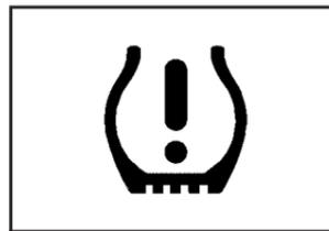
When a low tire pressure condition is detected, the TPMS will illuminate the low tire pressure warning symbol located on the instrument panel cluster.
