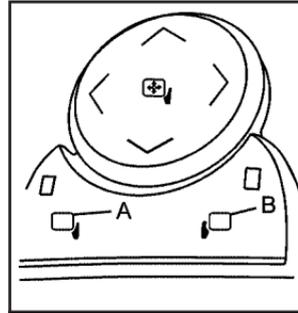
Vehicles with outside power mirrors have controls located on the driver door.
