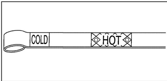
5. Safe operating level is within the HOT cross hatch band on the dipstick. If the fluid level is not within the HOT band, and the transmission temperature is between 160°F and 200°F (71°C and 93°C), add or drain fluid as necessary to bring the level into the HOT band. If the fluid level is low, add only enough fluid to bring the level into the HOT band. It does not take much fluid, generally less than one pint (0.5L). Do not overfill.
