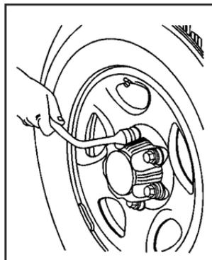
2. If your vehicle has wheel nut caps, loosen them by turning the wheel wrench counterclockwise.
