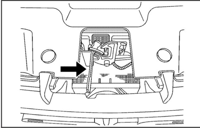
2. Then go to the front of the vehicle and locate the secondary hood release. This is located under the hood, near the center of the grille.
