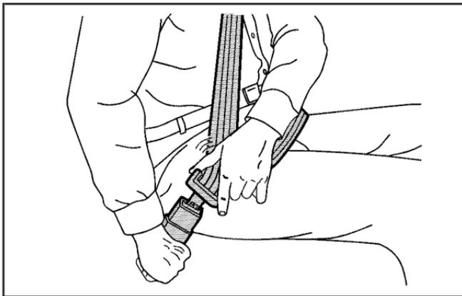
3. Push the latch plate into the buckle until it clicks. Pull up on the latch plate to make sure it is secure. If the belt is not long enough, see *Safety Belt Extender on page 1-37*.
