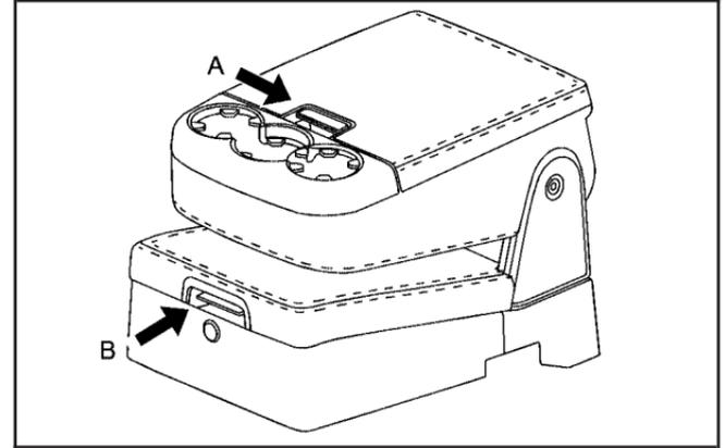
Pull the lever (A) up to access the upper storage area. Raise the upper storage bin, then pull the lever (B) up to access the lower storage area. Use the key to lock and unlock the lower storage area.
