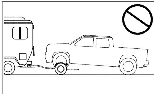
**Notice:** If a two-wheel-drive vehicle is towed with the rear wheels on the ground, the transmission could be damaged. The repairs would not be covered by the vehicle warranty. Never tow the vehicle with the rear wheels on the ground.
