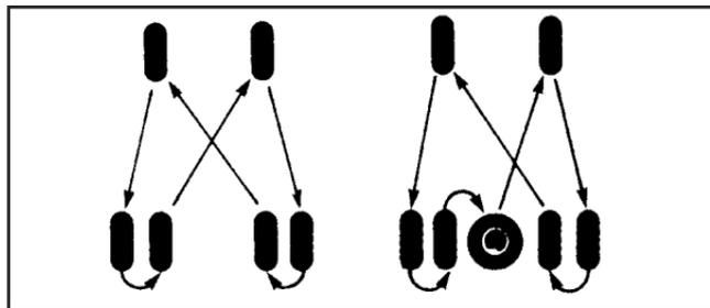
If your vehicle has dual rear wheels and the tread design for the front tires is the same as the rear tires, always use one of the correct rotation patterns shown here when rotating the tires.
