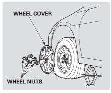
On LX and LX-V6 models Do not attempt to forcibly pry the wheel cover off with a screwdriver or other tool. The wheel cover cannot be removed without first removing the wheel nuts.
