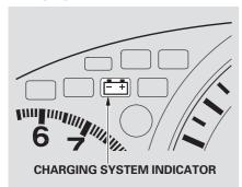
If the charging system indicator comes on brightly when the engine is running, the battery is not being charged.
