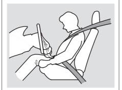
After inflating, the front airbags will immediately deflate, so they won't interfere with the driver's visibility, or the ability to steer or operate other controls.
