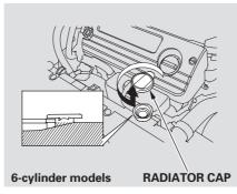
3. The coolant level should be up to the base of the filler neck. Add coolant if it is low.
