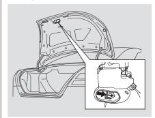
As a safety feature, your vehicle has a release lever on the trunk latch so the trunk can be opened from the inside. To open the trunk, push the release lever to the left.
