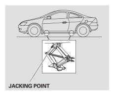
9. Place the jack under the jacking point nearest the tire you need to change. Turn the end bracket clockwise until the top of the jack contacts the jacking point. Make sure the jacking point tab is resting in the jack notch.
