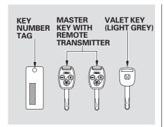
The master key fits all the locks on your vehicle. The valet key works only in the ignition and the driver's door lock. You can keep the trunk release handle, rear seat trunk access, and glove box locked when you leave your vehicle and the valet key at a parking facility.
