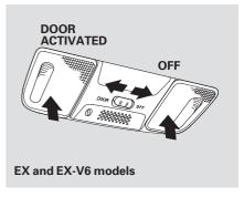
On EX and EX-V6 models The spotlights have a two-position switch. In the DOOR position, the lights come on when you open either door. In the OFF position, the lights do not come on.
