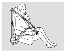
For added protection, the front seat belts are equipped with automatic seat belt tensioners. When activated, the tensioners immediately tighten the belts to help hold the driver and a front passenger in place. The tensioners are designed to activate primarily in frontal collisions, and they should activate in any collision severe enough to cause front-airbag inflation.
