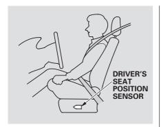
The driver's advanced front airbag system includes a seat position sensor under the seat. If the seat is positioned too far forward, the airbag will inflate sequentially, regardless of the severity of the impact.
