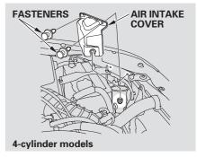
1. Open the hood. To change a bulb on the passenger's side, undo the two fasteners and remove the air intake cover.
