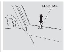
The lock tab on the passenger's door lock and unlock only that door. Pulling up on the driver's door lock tab only unlocks the driver's door.
