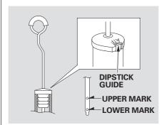
3. Insert the dipstick all the way into the transmission securely as shown in the illustration. Make sure the notch in the rubber cap fits in the dipstick guide and that you push the dipstick in all the way.
