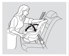
5. Push and pull the child seat forward and from side to side to verify that it is firmly secured. If the child seat is not secure, unlatch the belt, allow it to retract fully, then repeat these steps.
