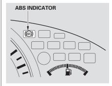
If the ABS indicator comes on, the anti-lock function of the braking system has shut down. The brakes still work like a conventional system, but without anti-lock. You should have the dealer inspect your vehicle as soon as possible.
