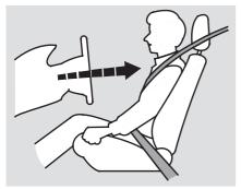
Adjust the steering wheel, if needed, so that the wheel points toward your chest, not toward your face. This provides optimal protection from the front airbag.
