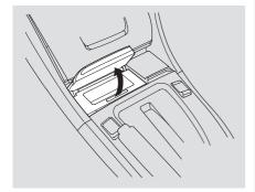
To open the coin pocket, pull the lid up. To close it, push the lid down until it latches. The compartment cannot be used as an ashtray.
