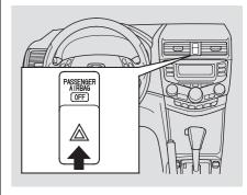
Push the button between the center vents to turn on the hazard warning lights (four-way flashers). This causes all four outside turn signals and both turn indicators in the instrument panel to flash. Use the hazard warning lights if you need to park in a dangerous area near heavy traffic, or if your vehicle is disabled.
