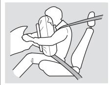
If you ever have a moderate to severe frontal collision, sensors will detect the vehicle's rapid deceleration. If the rate of deceleration is high enough, the control unit will instantly inflate the driver's and front passenger's front airbags, at the appropriate time and with the force needed.
