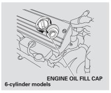
Install the engine oil fill cap and tighten it securely. Wait a few minutes and recheck the oil level. Do not fill above the upper mark; you could damage the engine.
