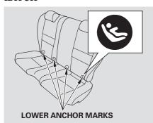
Your vehicle is equipped with LATCH (Lower Anchors and Tethers for Children) at the outer rear seats. The lower anchors are located between the seat-back and seat bottom, and are to be used only with a child seat designed for use with LATCH.
