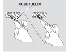
4. Check the smaller fuses in the under-hood fuse box and all the fuses in the interior fuse box by pulling out each fuse with the fuse puller provided in the under-hood fuse box.
