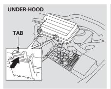
The under-hood fuse box is located on the driver's side. To open it, push the tabs as shown
