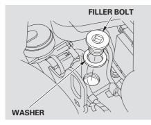
If no fluid comes out, remove the filler bolt. Slowly add Honda Manual Transmission Fluid (MTF) until it starts to run out of the check bolt hole. Let the fluid run out until it stops, then reinstall the check bolt and the filler bolt.
