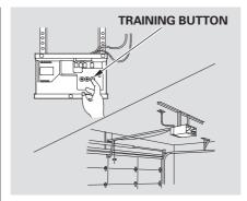
3. Press the Training button on the garage door opener unit until the light next to the button comes on, then release it. The light may blink, or come on and stay on. You then have approximately 30 seconds to complete the following steps.
