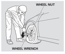
8. Loosen each wheel nut 1/2 turn with the wheel wrench.
