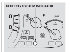
Once the security system is set, opening either door without using the key or the remote transmitter, the hood, or the trunk will cause it to sound. It also sounds if the radio is removed from the dashboard or the wiring is cut.
