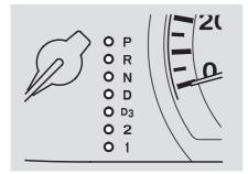
These indicators between the tachometer and speedometer show which position the shift lever is in.
