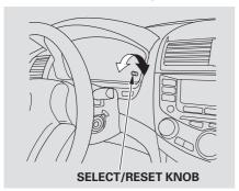
The Select/Reset knob on the instrument panel controls the brightness of the instrument panel lights. Turn the knob to adjust the brightness.
