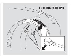
2. Use a flat-tipped screwdriver to remove the two holding clips from the inner fender.
