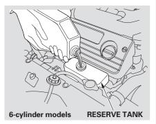
Do not add any rust inhibitors or other additives to your vehicle's cooling system. They may not be compatible with the coolant or engine components.
