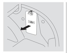
6. The jack is behind a cover in the right fender. Remove the cover by turning the handle counterclockwise, then pulling on the cover.
