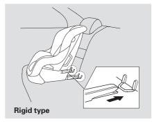
3. Place the child seat on the vehicle seat, and attach the seat to the lower anchors according to the child seat maker's instructions.
