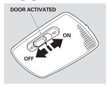
The ceiling light has a three-position switch; ON, Door Activated, and OFF. In the Door Activated (center) position, the light comes on when you:
