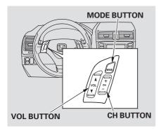
On all EX and V6 models Three controls for the audio system are mounted in the steering wheel hub. These let you control basic functions without removing your hand from the wheel.
