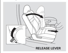
To get into the rear seat on the passenger's side, push downward on the release lever at the base of the seat-back. The seat-back will tilt forward and the entire seat will move forward to allow easier entry to the rear seat.
