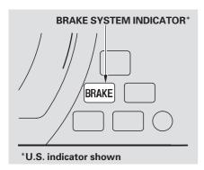
The brake system indicator normally comes on when you turn the ignition switch to ON (II) and as a reminder to check the parking brake. It will stay lit if you do not fully release the parking brake.
