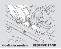
5. Pour coolant into the reserve tank. Fill it to halfway between the MAX and MIN marks. Put the cap back on the reserve tank.
