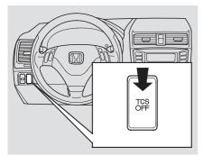
This switch is under the side vent. It lets you turn the Traction Control System on and off. You cannot turn off the TCS while the TCS Activation indicator is flashing.
