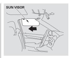
On vehicles with side curtain airbags In this position, the sun visor can be adjusted by moving it on its slider. Do not use the sun visor extension over the rear view mirror.
