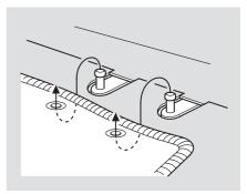
The driver's floor mat that came with your vehicle hooks over the floor mat anchors. This keeps the floor mat from sliding forward and possibly interfering with the pedals or making the front passenger's weight sensors ineffective.
