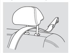
1. After securing the child seat in the desired position (see page 43), lift the head restraint, then route the tether strap over the top of the seat-back and through the head restraint legs.
