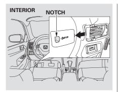
The vehicle's fuses are located in two fuse boxes.
