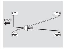
The hydraulic system that operates the brakes has two separate circuits. Each circuit works diagonally across the vehicle (the left-front brake is connected with the right-rear brake,
