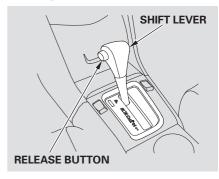
To shift from any position, press firmly on the brake pedal and press the release button on the side of the shift lever. You cannot shift out of Park when the ignition switch is in LOCK (0) or ACCESSORY (I).
