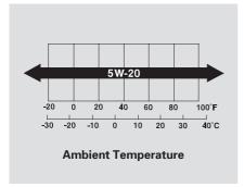
The oil viscosity or weight is provided on the container's label. 5W-20 oil is formulated for year-round protection of your Honda to improve cold weather starting and fuel economy.
