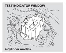
Check the condition of the battery monthly by looking at the test indicator window. The label on the battery explains the test indicator's colors.
