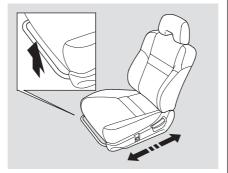
To adjust the seat forward and backward, pull up on the bar under the seat cushion's front edge. Move the seat to the desired position and release the bar. Try to move the seat to make sure it is locked in position.
