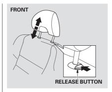
The head restraints adjust for height. You need both hands to adjust the restraint. Do not attempt to adjust it while driving. To raise it, pull upward. To lower the restraint, push the release button sideways, and push the restraint down.
