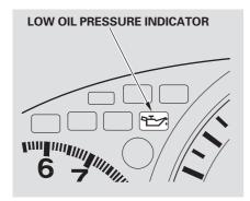
This indicator should never come on when the engine is running. If it starts flashing or stays on, the oil pressure has dropped very low or lost pressure. Serious engine damage is possible and you should take immediate action.
