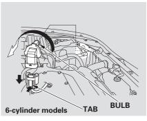
Push the electrical connector back onto the bulb. Make sure it is on all the way.
