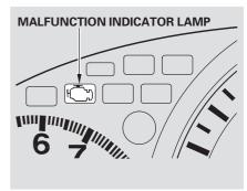
If the indicator comes on while driving, it means one of the engine's emissions control systems may have a problem. Even though you may feel no difference in your vehicle's performance, it can reduce your fuel economy and cause increased emissions. Continued operation may cause serious damage.
