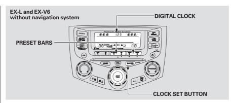
clock back to the previous hour. If the displayed time is after the half hour, the clock sets forward to the beginning of the next hour.
