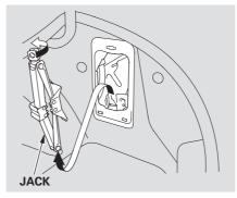
7. Turn the jack's end bracket counterclockwise to loosen it, then remove the jack.
