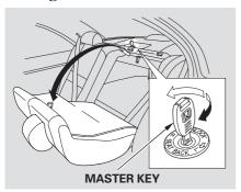
The left and right halves can be folded separately from inside the vehicle or inside the trunk. To fold down the seat-back from inside the vehicle, insert the master key in the lock on the rear shelf. To fold down the driver's side, turn the key clockwise, pull down the top of the seat-back, then release the key. To fold down the passenger's side, turn the key counterclockwise and perform the same procedure.
