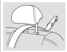
5. Route the tether strap through the legs of the head restraint, then attach the hook to the anchorage point as shown.
