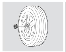
16. EX and EX-V6 models Remove the center cap before storing the flat tire in the trunk well.
