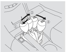
1. With the clutch pedal pressed, move the shift lever to the First/ Second gear side of the Neutral gate, then shift to Reverse.
