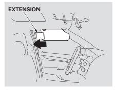
On vehicles without side curtain airbags In this position, the sun visor can be extended by sliding out the extension. Do not use the sun visor extension over the rear view mirror.
