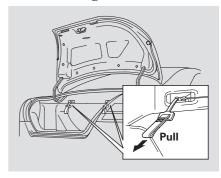
To lock the seat-back upright, push it firmly against the trunk panel. Make sure it is latched in place by pulling on the top of the seat.
