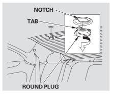
5. Insert the moonroof wrench securely into the socket behind this plug. Hold the longer handle as shown and turn the wrench slowly until the moonroof is fully closed.
