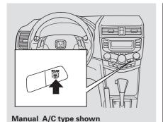
The rear window defogger will clear fog, frost, and thin ice from the window. Push the defogger button to turn it on and off. The indicator above/in the button lights to show the defogger is on. It also shuts off when you turn off the ignition. You have to turn it on again when you restart the vehicle.
