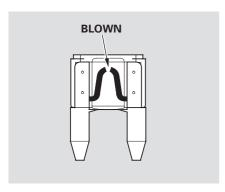
5 Look for a burned wire inside the fuse. If it is burned, replace it with one of the spare fuses of the same rating or lower.
