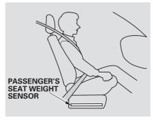
The passenger's advanced front airbag system has weight sensors under the seat. If the sensors detect a total weight on the seat of about 65 lbs (30 kg) or less, the system will automatically turn the passenger's front airbag off.
