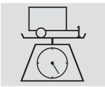
• Total Trailer Weight: The total weight of the trailer and everything loaded in it must not exceed 1,000 lbs (450 kg). Towing a load that is too heavy can seriously affect your vehicle's handling and performance. It can also damage the engine and drivetrain.
