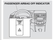
This indicator alerts you that the passenger's front airbag has been shut off. It does not mean there is a problem with the airbag.
