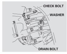
Remove the check bolt and look for transmission fluid coming out of the bolt hole. If a small amount of fluid drips out of the bolt hole, reinstall the check bolt.
