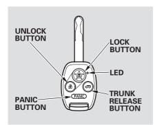
LOCK — Press this button once to lock both doors. Some exterior lights will flash once. When you push LOCK twice within 5 seconds, you will hear a beep to verify that the doors are locked and (if equipped) that the security system has set. You cannot lock it if either door is not fully closed or the key is in the ignition switch.
