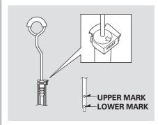
3. Insert the dipstick all the way into the transmission securely as shown in the illustration.
