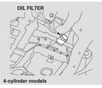
4. Install a new oil filter according to the instructions that come with it. Make sure to clean off any dirt and dust on the connecting surface of a new oil filter.
