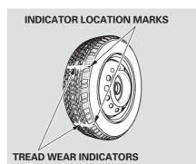
Your vehicle's tires have wear indicators molded into the tread. When the tread wears down to that point, you will see a 1/2 inch (12.7 mm) wide band running across the tread. This shows there is less than 1/16 inch (1.6 mm) of tread left on the tire. A tire that is this worn gives very little traction on wet roads. You should replace the tire if you can see the tread wear indicator in three or more places around the tire.
