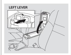
You can put small items in the tray located in the console compartment lid. To use the tray, pull up on the left lever and lift up the armrest.
