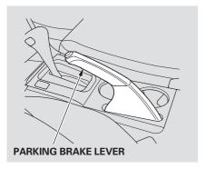
To apply the parking brake, pull the lever up fully. To release it, pull up slightly, push the button, and lower the lever. The parking brake indicator on the instrument panel should go out when the parking brake is fully released with the engine running (see page 59).
