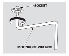
6. Remove the wrench. Reinstall the round plug.
