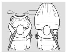
Your vehicle has a Supplemental Restraint System (SRS) with front airbags to help protect the heads and chests of the driver and a front seat passenger during a moderate to severe frontal collision (see page 22 for more information on how your front airbags work).
