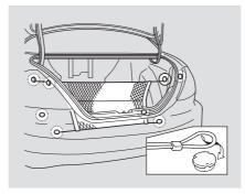
On all EX and EX-V6 models The cargo net can be used to help hold down items stored in the trunk. To use the cargo net, hook it to the buttons on the floor and sides of the trunk. You can use the cargo net in several configurations by hooking it to different buttons.
