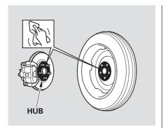
12. Before mounting the spare tire, wipe any dirt off the mounting surface of the wheel and hub with a clean cloth. Wipe the hub carefully; it may be hot from driving.
