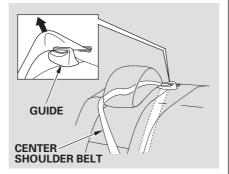
When storing cargo, you can move the rear center shoulder belt out of the way by removing the belt from the guide. To release the seat-back from inside the trunk, pull the release under the trunk panel. Push the seat-back down, then let go of the release.
