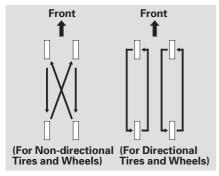
To help increase tire life and distribute wear more evenly, rotate the tires every 10,000 miles (16,000 km) on 4-cylinder models and 7,500 miles (12,000 km) on 6-cylinder models. Move the tires to the positions shown in the chart each time they are rotated. If you purchase directional tires, rotate only front-to-back.
