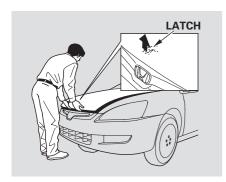
2. Reach in between the hood and the front grille with your finger. The hood latch handle is above and to the left of the "H" logo. Push this handle up until it releases the hood. Lift the hood.
