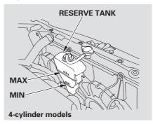
Look at the coolant level in the radiator reserve tank. Make sure it is between the MAX and MIN lines. If it is below the MIN line, see Adding **Engine Coolant** on page 221 for information on adding the proper coolant.
