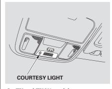
On EX and EX-V6 models The courtesy light between the spotlights comes on when you turn the parking lights on. To adjust its brightness, turn the Select/Reset knob on the instrument panel.
