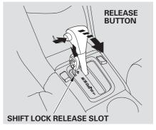
6. Remove the key from the Shift Lock Release slot, then reinstall the cover. Make sure the notch on the cover is on the left side. Press the brake pedal, and restart the engine.
