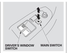
The driver's armrest has a master power window control panel. To open the passenger's window, push down on the switch and hold it down until the window reaches the desired position. To close the window, pull back on the window switch. Release the switch when the window gets to the position you want.
