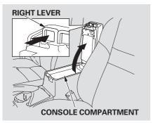
To open the console compartment, pull up on the right lever and lift the armrest.
