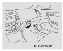
Open the glove box by pulling the handle to the left. Close it with a firm push. Lock or unlock the glove box with the master key.
