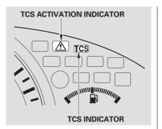
When starting out or driving on a loose or slippery road surface, you may notice that the vehicle does not respond to the accelerator in the same way it does at other times. This is a sign TCS is activating. You will see the TCS Activation indicator flash.
