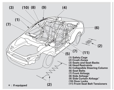
Your vehicle is equipped with many features that work together to protect you and your passengers during a crash.
