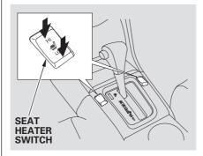
On EX-V6 model and EX-L model Both front seats are equipped with seat heaters. Because of the sensors for the side airbag system, there is no heater in the passenger's seatback. The ignition switch must be ON (II) to use the heaters.
