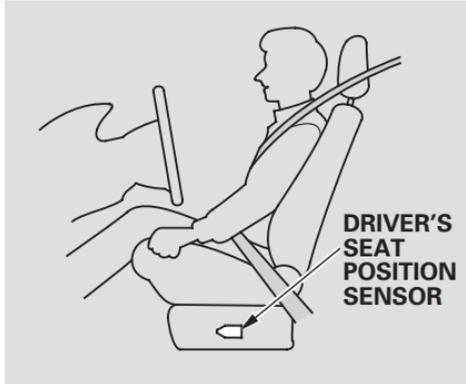
The driver's advanced front airbag system includes a seat position sensor under the seat. If the seat is positioned too far forward, the airbag will inflate sequentially, regardless of the severity of the impact.
