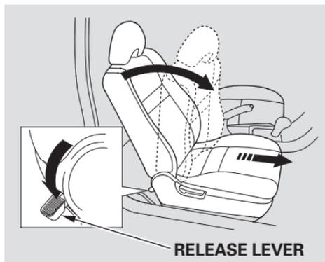
To get into the rear seat on the passenger's side, push downward on the release lever at the base of the seat-back. The seat-back will tilt forward and the entire seat will move forward to allow easier entry to the rear seat.
