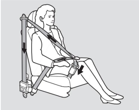
For added protection, the front seat belts are equipped with automatic seat belt tensioners. When activated, the tensioners immediately tighten the belts to help hold the driver and a front passenger in place.
