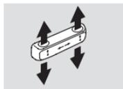
Moves the front of the seat up or down and the rear of the seat up or down.
