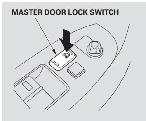
To lock both doors, push the top of the master door lock switch on either door, or press the lock tab down on the driver's door, or use the key on the outside lock on the driver's door.
