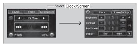
Select Clock/Screen to adjust the clock and screen settings.
