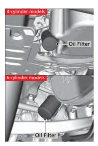
**4.** Remove the oil filter and dispose of the remaining oil.
