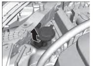
If the level is low, fill the washer reservoir.
