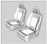
The ignition switch must be in ON  $\overline{\rm II}^{*1}$  to use the seat heaters. The  ${\bf HI}$  setting heats the seats faster than the  ${\bf LO}$  setting.
