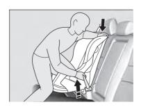
A child seat that is not properly secured will not adequately protect a child in a crash and may cause injury to the child or other vehicle occupants.
