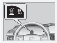
Even though adaptive cruise control has been automatically canceled, you can still resume the prior set speed. Wait until the condition that caused ACC to cancel improves, then press the **RES/+** button.
