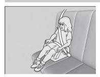
If a lap/shoulder seat belt cannot be used properly, position the child in a booster seat in a rear seating position. For the child's safety, check that the child meets the booster seat manufacturer's recommendations.
