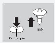
Push the central pin back to lock the clip. Then, insert the clip into the hole and press on the central pin until it is flat.
