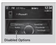
Certain manual functions are disabled or inoperable while the vehicle is in motion. You cannot select a grayed-out option until the vehicle is stopped.
