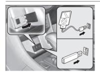
Install the iPod® dock connector or the USB flash drive to the USB port.
