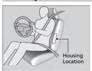
The side airbags are housed in the outside edge of the driver's and passenger's seatbacks.
