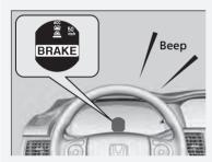
Depress the brake pedal, and keep an appropriate distance from the vehicle ahead.
