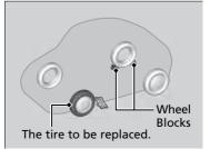
**4.** Place a wheel block or rock in front and rear of the wheel diagonal to the flat tire.
