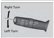
The turn signals can be used when the ignition switch is in ON III \*1.
