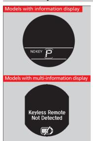
Warning buzzers may sound from inside or/ and outside the vehicle to remind you that the smart entry remote is out of the vehicle. If the buzzer continues even after the remote is put back inside, place it to be within its operational range.
