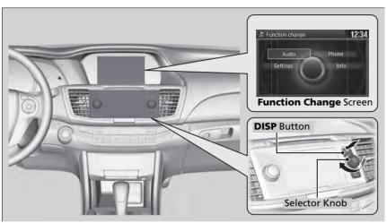
Press the **DISP** button to go to the **Function Change** screen. Rotate ♥ to select **Audio**, **Phone**, **Info** or **Setting** and press ८.
