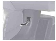
2 Locate the hood latch lever, pull the lever up, and lift up the hood.
