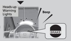
When the lights flash at any setting: The **BRAKE** message appears until a possible collision is avoided.
