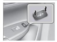
The ignition switch must be in ON [II]\*1 to use the seat heaters. The **HI** setting heats the seats faster than the **LO** setting.
