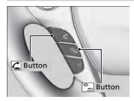
Press the (pick-up) button on the steering wheel to receive a call when *Bluetooth* Audio is playing.
