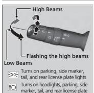
Rotating the light switch turns the lights on and off, regardless of the position of the ignition switch\*1.
