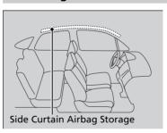
The side curtain airbags are located in the ceiling above the side windows on both sides of the vehicle.
