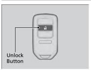
**To open:** Press the unlock button twice within 10 seconds and hold it down for the second time. If the windows stop midway, repeat the procedure.
