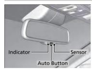
When driving after dark, the automatic dimming rearview mirror reduces the glare from headlights behind you. Press the auto button to turn this function on and off. When activated, the auto indicator comes on.
