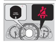
Your vehicle monitors front seat belt use. If the ignition switch is turned to ON  $\boxed{II}^{*1}$  before the driver's seat belt is fastened, a beeper will sound and the indicator will blink. If the driver does not fasten the belt before the beeper stops, the indicator will remain on.
