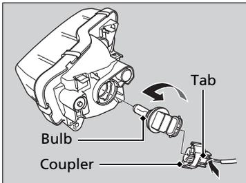
4. Push the tab to remove the coupler.
