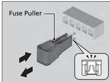
4. Inspect the small fuses in the engine compartment and the vehicle interior.
