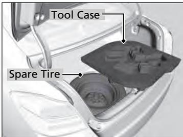
2. Take the tool case out of the trunk. Take the jack and wheel nut wrench out of the tool case.
