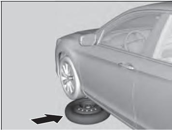
**5.** Place the compact spare tire (wheel side up) under the vehicle body, near the tire that needs to be replaced.
