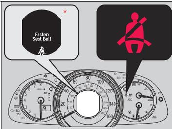
Your vehicle monitors front seat belt use. If the ignition switch is turned to ON **II**<sup>\*1</sup> before the driver's seat belt is fastened, a beeper will sound and the indicator will blink. If the driver does not fasten the belt before the beeper stops, the indicator will remain on.
