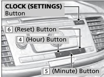
1. Press and hold the **CLOCK (SETTINGS)** button until the clock display blinks.
