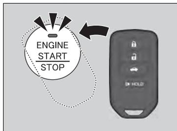
1. Touch the center of the **ENGINE START/STOP** button with the **H** logo on the smart entry remote while the indicator on the **ENGINE START/STOP** button is flashing. The buttons on the smart entry remote should be facing you.
