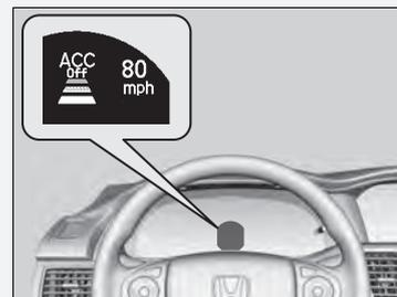
Even though adaptive cruise control has been automatically canceled, you can still resume the prior set speed. Wait until the condition that caused ACC to cancel improves, then press the **RES/+** button.
