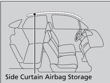
The side curtain airbags are located in the ceiling above the side windows on both sides of the vehicle.
