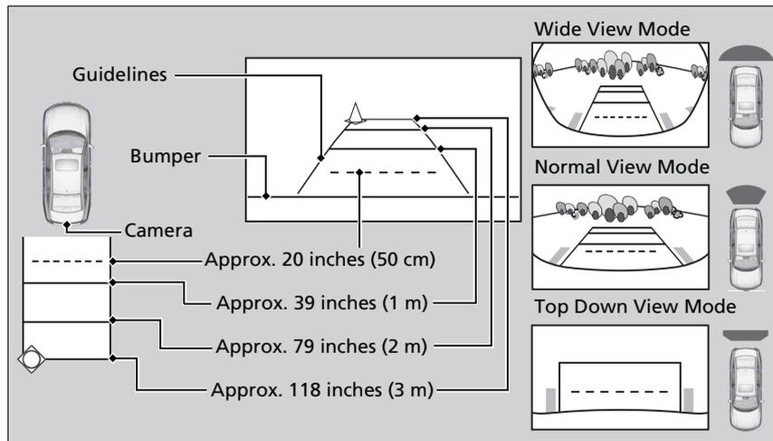
You can view three different camera angles on the rearview display. Press the selector knob to switch the angle.
