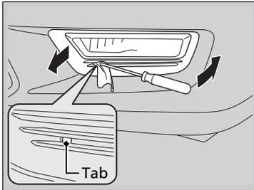
2. Insert a flat-tip screwdriver into the tab on the cover, then pull straight out as indicated to remove the cover.
