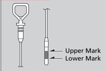
4. Remove the dipstick again, and check the level. It should be between the upper and lower marks. Add oil if necessary.
