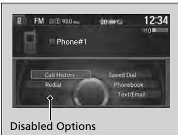
Certain manual functions are disabled or inoperable while the vehicle is in motion. You cannot select a grayed-out option until the vehicle is stopped.
