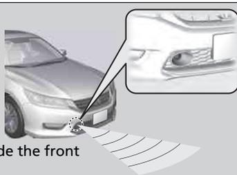
The radar sensor is inside the front grille on the right side.
