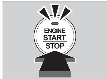
2. Depress the brake pedal (automatic transmission) or clutch pedal (manual transmission) and press the **ENGINE START/STOP** button within 10 seconds after the beeper sounds and the indicator stays on.
