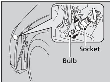
1. Turn the socket to the left and remove it, then remove the old bulb.
