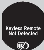
Warning buzzers may sound from inside or/ and outside the vehicle to remind you that the smart entry remote is out of the vehicle. If the buzzer continues even after the remote is put back inside, place it to be within its operational range.
