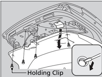
1. Remove the holding clips using a flat-tip screwdriver, then pull the lining back.
