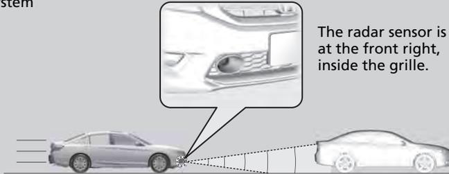
The radar sensor is at the front right, inside the grille.
