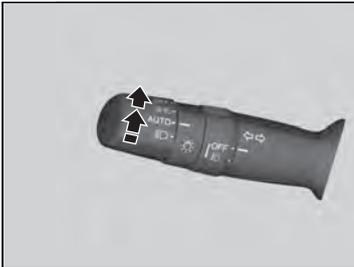
Automatic lighting control can be used when the ignition switch is in ON
