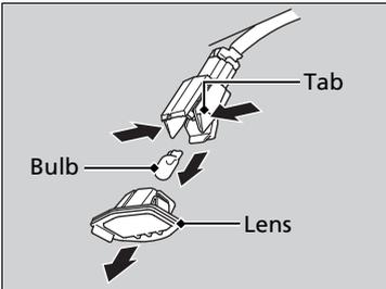
2. Remove the lens by pushing the tabs.
