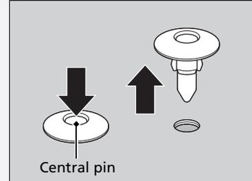
Push the central pin back to lock the clip. Then, insert the clip into the hole and press on the central pin until it is flat.
