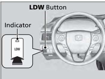
Press the **LDW** button to turn the system on and off.
