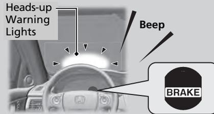
When the lights flash at any setting: The **BRAKE** message appears until a possible collision is avoided.
