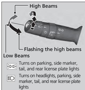
Rotating the light switch turns the lights on and off, regardless of the position of the ignition switch\*1.
