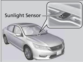
The automatic climate control system is equipped with a sunlight sensor and an interior temperature sensor. Do not cover or spill any liquid on them.
