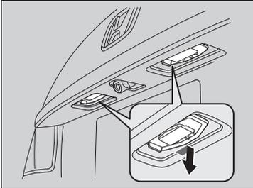
1. Remove the license plate light assembly by pushing the left edge of the lens toward the right and pulling the assembly out.
