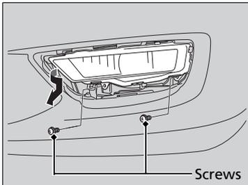
3. Remove the screws using a Phillips-head screwdriver and carefully pull the fog light assembly out of the bumper.
