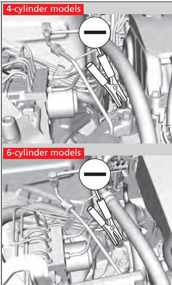
4. Connect the other end of the second jumper cable to the engine mounting bolt as shown. Do not connect this jumper cable to any other part.
