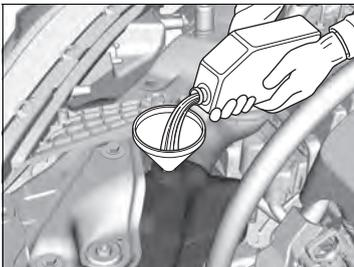
2. If the coolant level is below the **MIN** mark, add the specified coolant until it reaches the **MAX** mark.
