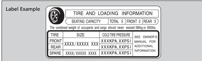
This figure includes the total weight of all occupants, cargo, and accessories, and the tongue load if you are towing a trailer.
