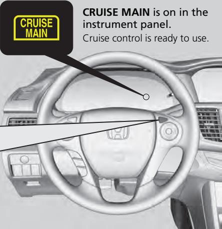
**CRUISE MAIN** is on in the instrument panel. Cruise control is ready to use.
