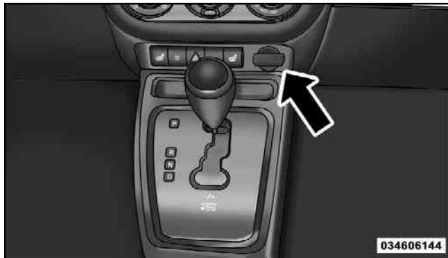
Power Outlet 12-Volts
