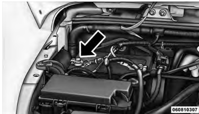
Positive Battery Post
