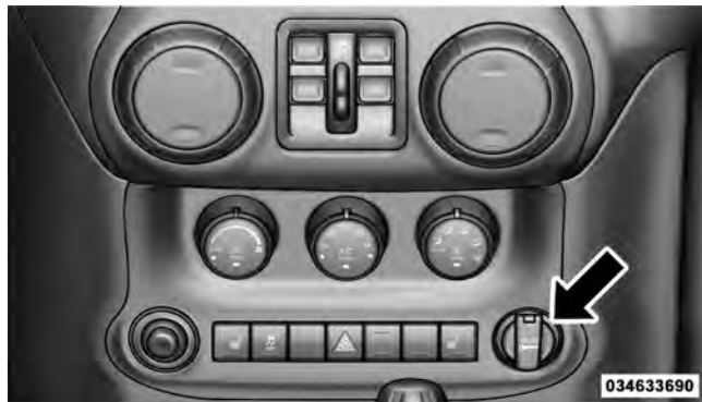
Front Power Outlet
