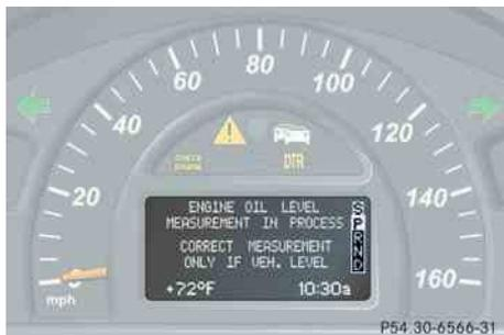
After about three seconds this message is displayed: ENGINE OIL LEVEL - MEASURING NOW
