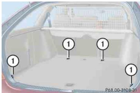
Four rings **1** are located in the cargo compartment.
