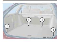
Four rings 1 are located in the cargo compartment.
