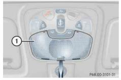
Pry off lens 1 using a flat blade screwdriver.
