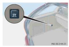
An electrical outlet is located on the left side of the cargo compartment.
