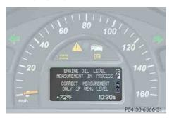
After about three seconds this message is displayed: ENGINE OIL LEVEL - MEASURING NOW
