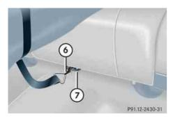
Connect snap hook 6 of front strap to eye 7 located on center tunnel in front of rear seat bench.
