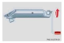
Turn the crank handle clockwise until it engages (operational position).
