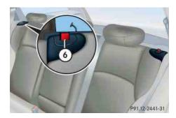
If the backrest is not locked into position, a red indicator (6) will be visible.
