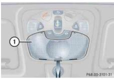
► Pry off lens ① using a flat blade screwdriver.
