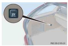
An electrical outlet is located on the left side of the cargo compartment.
