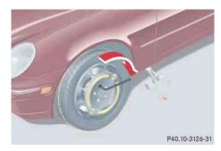
► Unscrew the alignment bolt, install last wheel bolt and tighten slightly.
