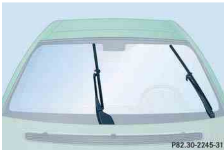
Wiper blades in vertical position
