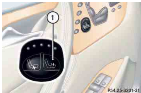
① Seat heating switch
