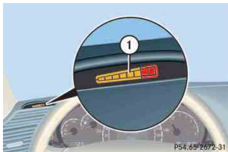
① Left front area warning indicator
