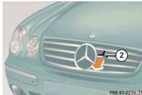
② Handle for opening the hood
