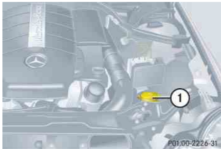
① Washer fluid reservoir
