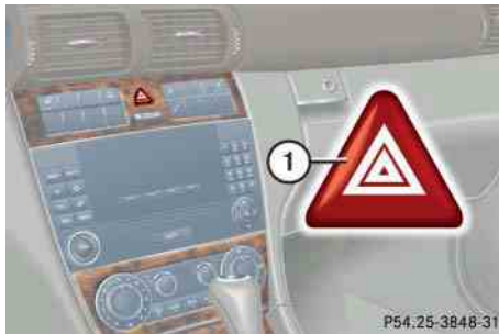
① Hazard warning flasher switch
