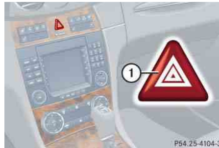
① Hazard warning flasher switch
