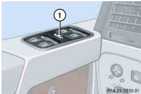
① Override switch
