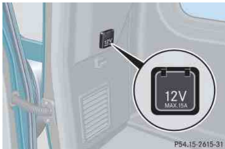
Electrical outlet on the left side (driver's side) of the cargo compartment
