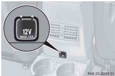
Electrical outlet in the rear passenger footwell
