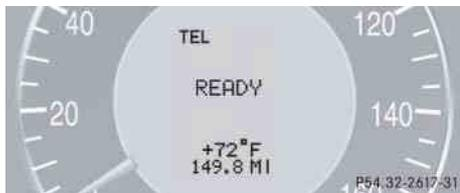
This standby message indicates that your telephone is ready for use and you can operate it using the control system.
