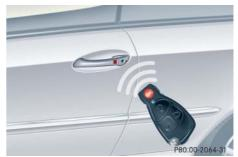
Aim transmitter eye of the SmartKey or SmartKey with KEYLESS-GO\* at the driver's outside door handle. The SmartKey or SmartKey with KEYLESS-GO\* must be in close proximity to the driver's outside door handle.
