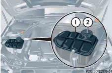
(1) Coolant expansion tank (2) Cap
