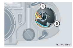
④ Bulb holder for high beam flasher bulb
