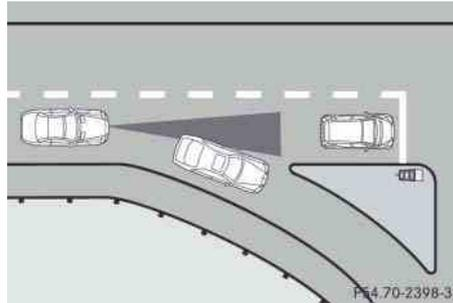
DISTRONIC Plus does not brake for obstacles or stationary vehicles. If, for example, the vehicle detected in front of you changes lanes to bypass an obstacle or stationary vehicle in front of it, DISTRONIC Plus will not brake for the obstacle or stationary vehicle.
