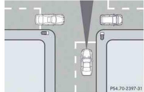
DISTRONIC Plus may inadvertently detect crossing vehicles. If you switch on DISTRONIC Plus, for example, at a traffic light with cross-traffic, the vehicle may suddenly start to drive off.
