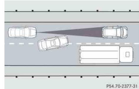
DISTRONIC Plus has not yet detected the vehicle changing lanes. There will be insufficient distance to the lane-changing vehicle.
