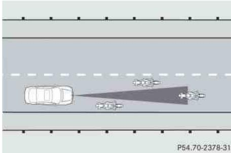
Because of their narrow profile, the vehicles traveling near the outer edge of the lane have not yet been detected by DISTRONIC Plus. There will be insufficient distance to the vehicles ahead.
