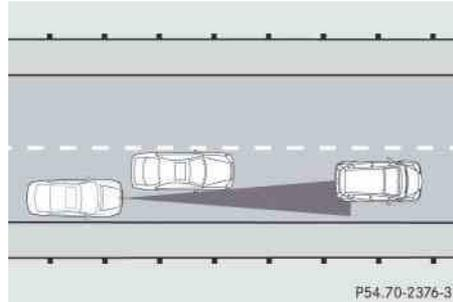
A vehicle traveling in your lane but offset from your direct line of travel may not be detected by DISTRONIC Plus. There will be insufficient distance to the vehicle ahead.
