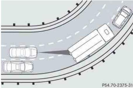
In turns or bends, DISTRONIC Plus may not detect a moving vehicle in front, or it may detect one too soon. This may cause your vehicle to brake late or unexpectedly.
