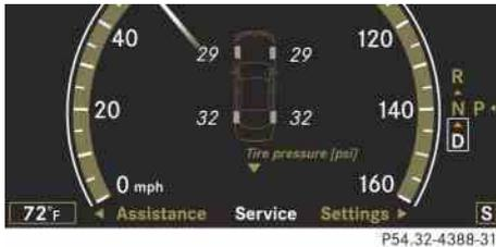
**i** When the message “Tire pressures displayed after driving a few minutes” appears in the display, the individual inflation pressure values are matched with the tires. The individual values are displayed after a few minutes driving.
