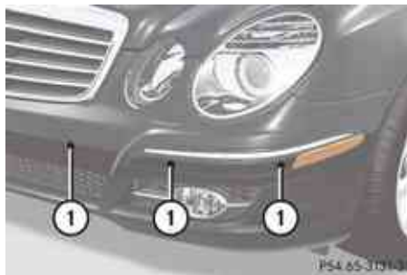
① Sensors in the front bumper
