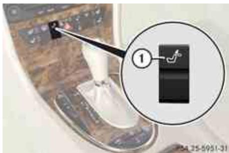
① Head restraint release switch
