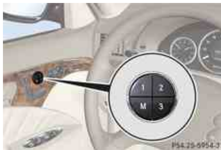
M Memory button 1, 2, 3 Memory position button
