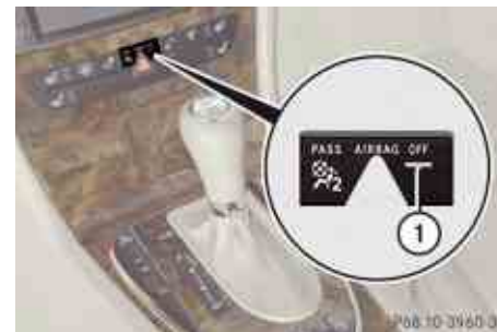
① Front passenger front air bag off indicator lamp
