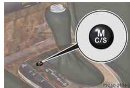
Program mode selector switch on E 63 AMG
