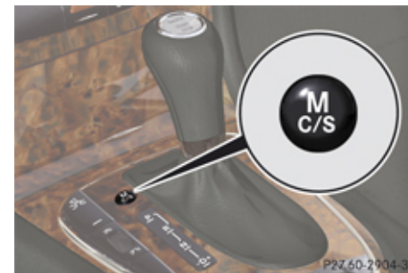
Program mode selector switch
