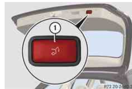
Example illustration: Wagon without KEYLESS-GO ① Tailgate closing switch
