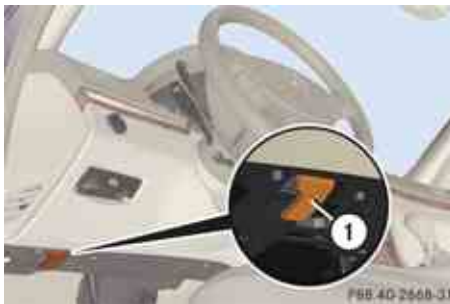
① Hood lock release lever
