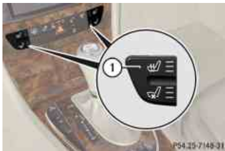
① Front seat heating switch
