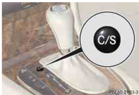
Program mode selector switch
