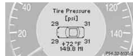
Display in vehicles with Advanced TPMS
