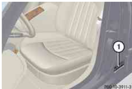
① Certification label (on driver's door B-pillar)
