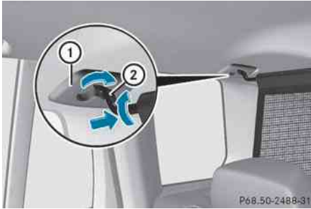
Cargo net attached behind the C-pillar
