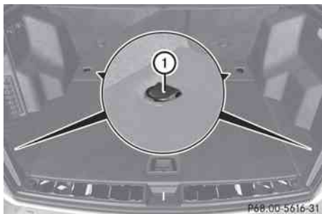
① Cargo tie down rings in the cargo compartment
