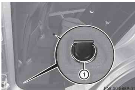
① Cargo tie down rings in the rear-compartment footwell (Canada only)
