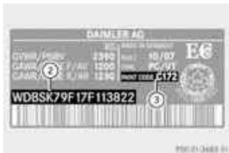
Example: vehicle identification plate (Canada only)
