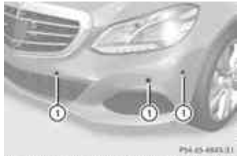
① Sensors in the front bumper, left-hand side (example)
