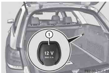
Power socket in the cargo compartment (Wagon)
