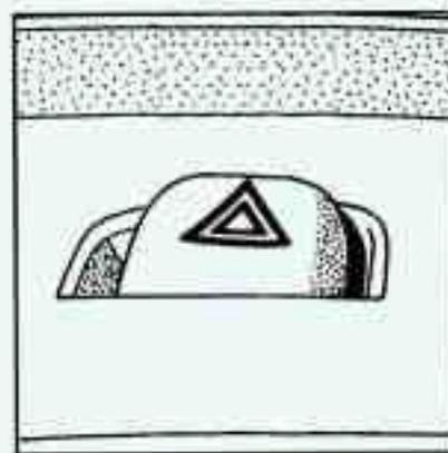
Press down on the button located on top of the steering column, then release it to turn on the hazard warning flashers.
