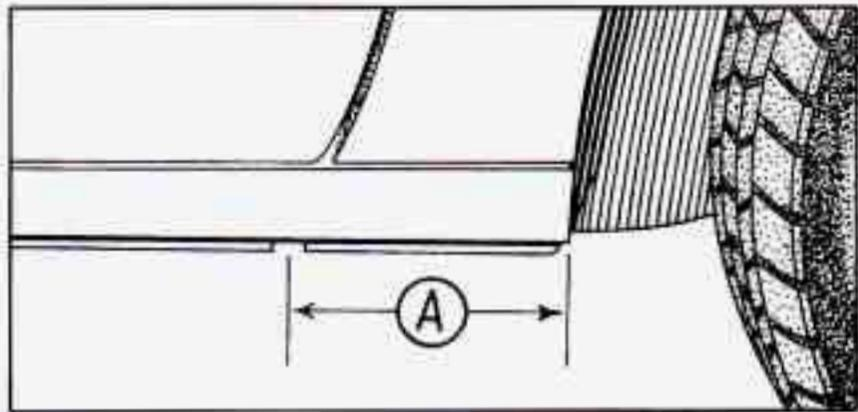
8. Near each wheel well is a notch on the frame to position the jack head. The front notch is 11 inches (28 cm) back from the front wheel well. The rear notch is 7.5 inches (19 cm) forward from the rear wheel well. You'll find the word JACK and an arrow stamped into the plastic near each notch.
