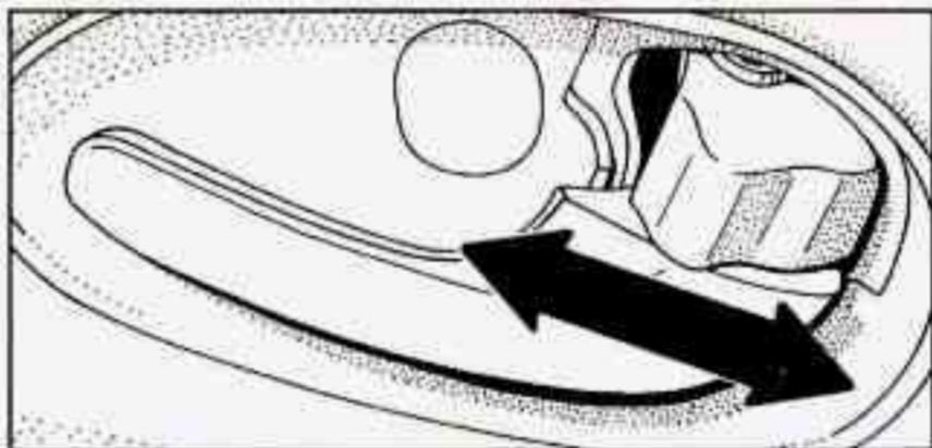
From the inside, to lock the door, rotate the locking lever forward.
