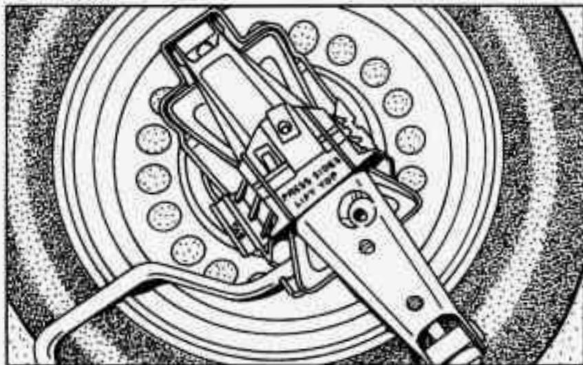
16. Store the flat tire as far forward in the trunk as possible. Store the jack and wheel wrench in their compartment in the trunk.
