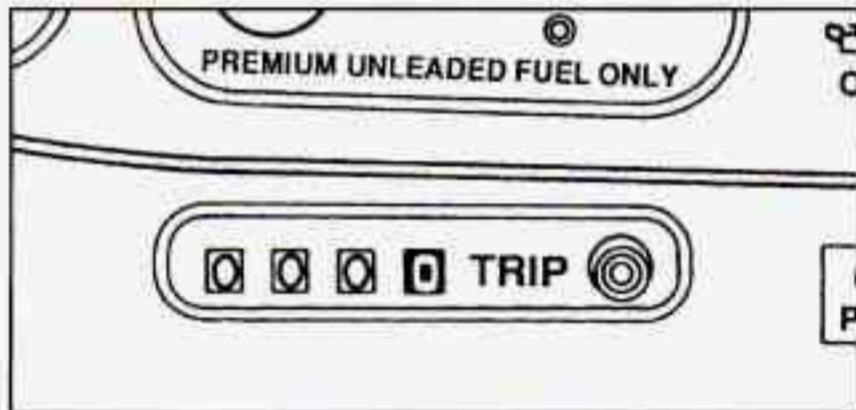
Your trip odometer tells you how far you have driven since you last reset it. Press the trip button located next to the trip odometer, below the fuel gage.
