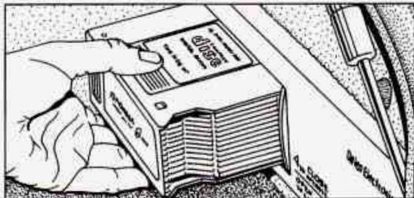
Once you have loaded the discs in the cartridge, slide open the door of the CD changer. Push the cartridge into the changer in the direction of the arrow marked on the top of the cartridge.
