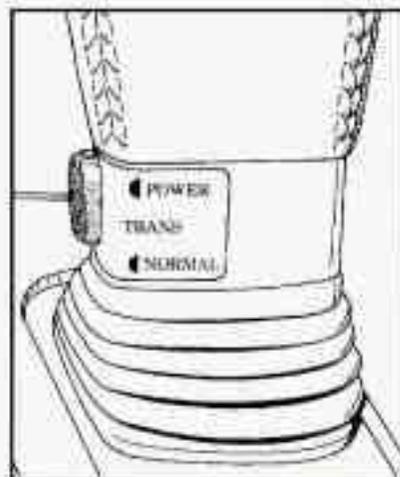
This button lets you change from a normal driving mode to a power mode. For general driving conditions, use the normal mode.
