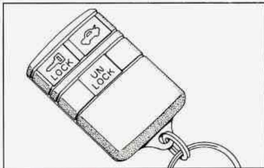
You can lock and unlock your doors or unlock your trunk from up to 30 feet (9 m) away using the key chain transmitter supplied with your vehicle.
