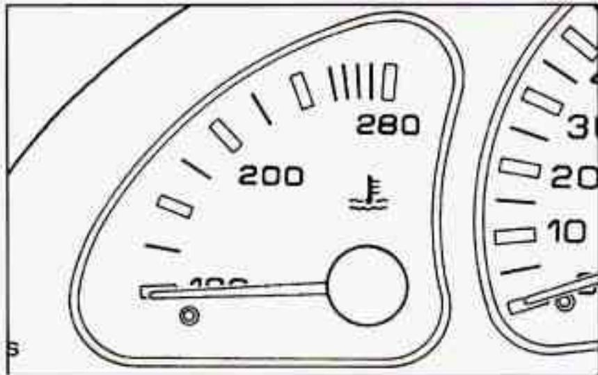
This gage shows the engine coolant temperature.
