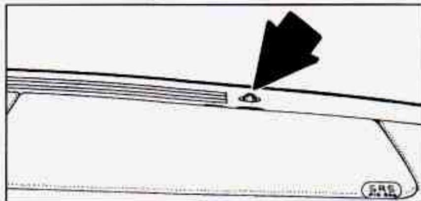
Your system has two sun sensors on top of the instrument panel that detect direct sunlight and the increased warming caused by it. To keep you comfortable, the sensors may reduce the interior temperature by as much as 5°F (3°C) below the setting on the digital screen, if necessary. Be careful not to put anything over these sun sensors. If you do, the system will think it's night and warm up the vehicle.
