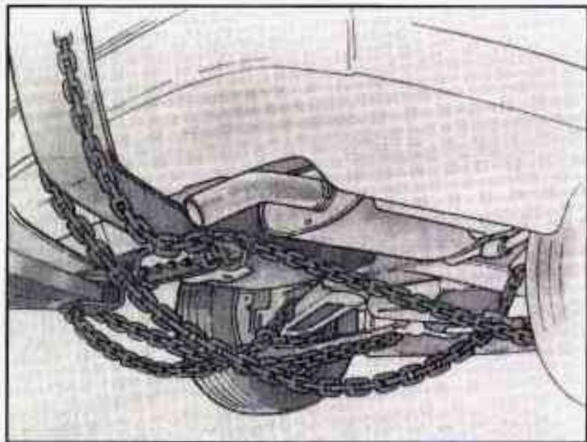
2. Position the lower sling crossbar directly under the rear bumper.
