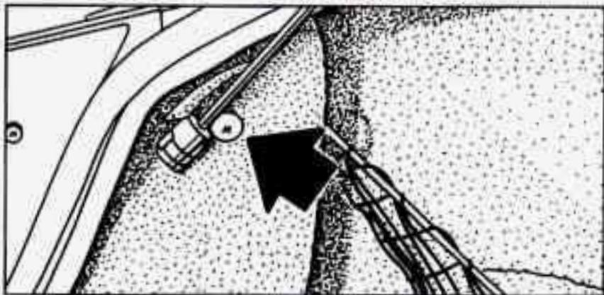
1. In the trunk, remove the convenience net from the hooks. Next remove the plastic screws holding the carpeting in place and pull back the carpeting.
