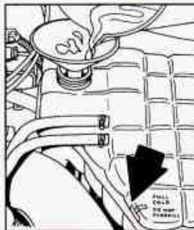
3. Fill the coolant surge tank with the proper mix, up to **FULL COLD**.
