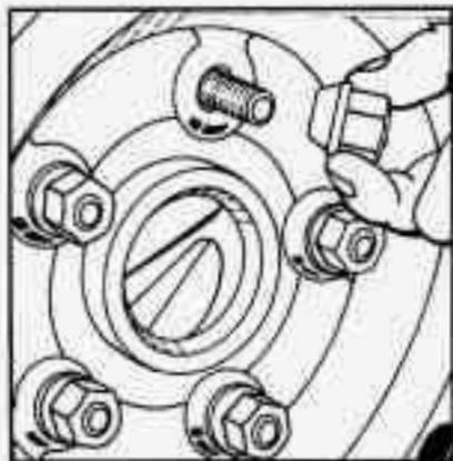
13. Replace the wheel nuts with the rounded end of the nuts toward the wheel. Tighten each nut by hand until the wheel is held against the hub.
