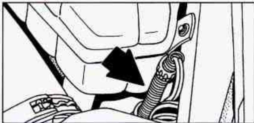
In very cold weather, 0°F (-18°C) or colder, the engine coolant heater can help. You'll get easier starting and better fuel economy during engine warm-up. Usually, the coolant heater should be plugged in a minimum of four hours prior to starting your vehicle.
