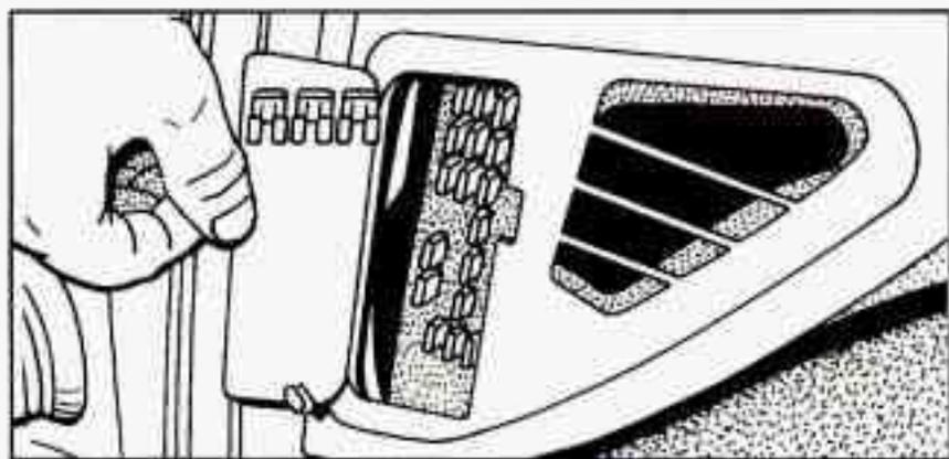
The third fuse panel is located on the left side of the instrument panel. To open it, simply pull on the latch and the door will open.
