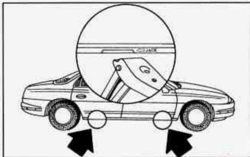
9. Position the jack and raise the jack head until it fits firmly against the sheet metal next to the word **JACK**. Do not raise the vehicle yet. Put the compact spare near you.
