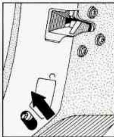
2. Move the lever on the door all the way up to the ENGAGED position.
