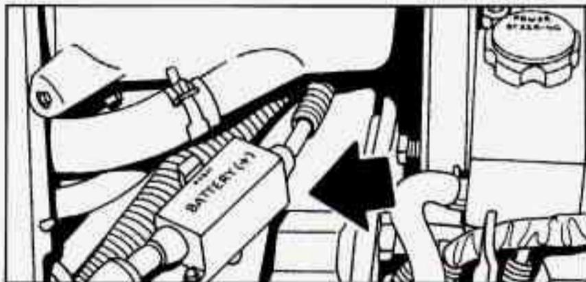
4. Open the hoods and locate the other vehicle's battery and the Aurora's remote positive (+) jump starting terminal.
