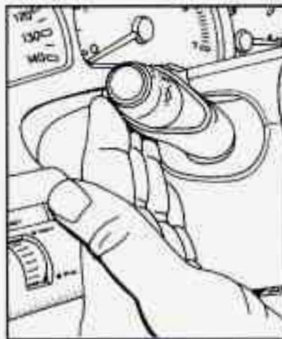
To change the headlamps from low beam to high or high to low, pull the turn signal lever all the way toward you. Then release it.
