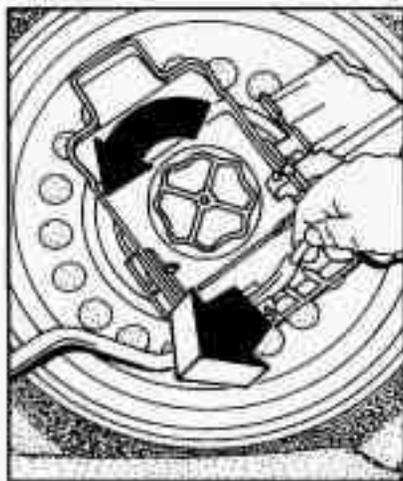
3. Turn the spare tire retainer bolt counterclockwise until it's loose and remove the retainer assembly.
