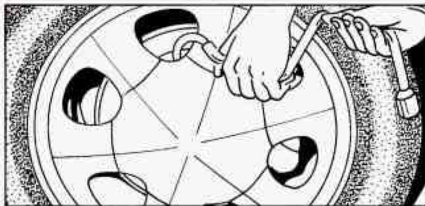
5. Insert the hooked end of the wheel wrench in one of the two small notches in the center cover and pry the cover off. Do not drop the cover or lay it face down, as it could be scratched or damaged.
