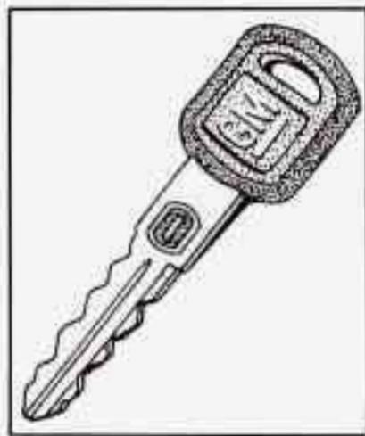
Your vehicle is equipped with the PASS-Key® II (Personalized Automotive Security System) theft deterrent system. PASS-Key® II is a passive theft deterrent system. This means you don't have to do anything different to arm or disarm the system. It works when you insert or remove the key from the ignition. PASS-Key® II uses a resistor pellet in the ignition key that matches a decoder in your vehicle.
