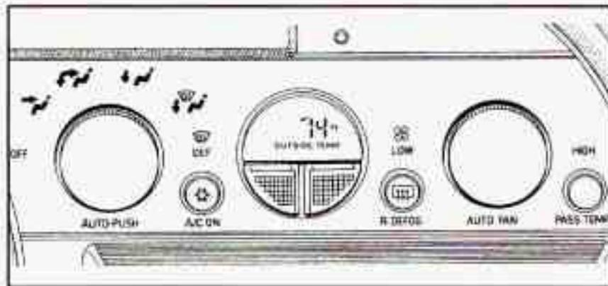
With this system, you can control the ventilation, heating and air conditioning in your vehicle, or you can use the automatic setting. Your vehicle also has the flow-through ventilation system described later in this section.
