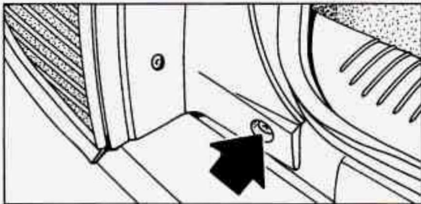
4. Remove the taillamp filler screw located to the side of the taillamp filler panel.
