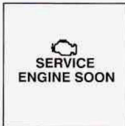
A computer monitors operation of your fuel, ignition and emission controls systems. This light should come on when you start your engine as a check to show you it is working.
