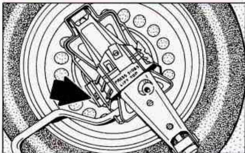
2. The jack container is labeled PRESS SIDES LIFT TOP. Do this, then remove the jack and wrench.
