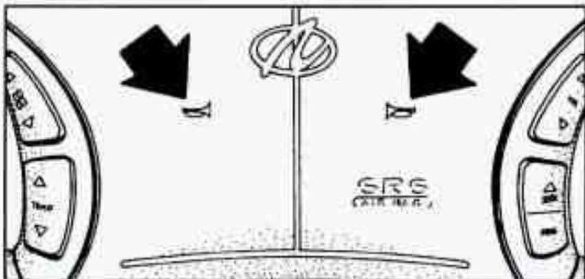
You can sound the horn by pressing the horn symbols on your steering wheel.
