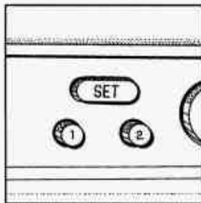
The memory function controls both the driver's seat and outside mirror positions. First position the seat and mirrors where you want them. Next, press the SET button. Within five seconds, press either the 1 or 2 button.
