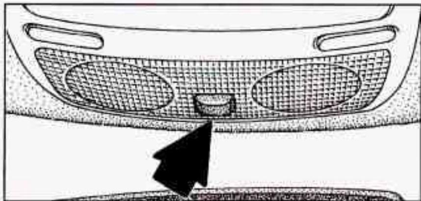
To open the sunroof, press the control switch rearward and release it to open the glass panel and sunshade.
