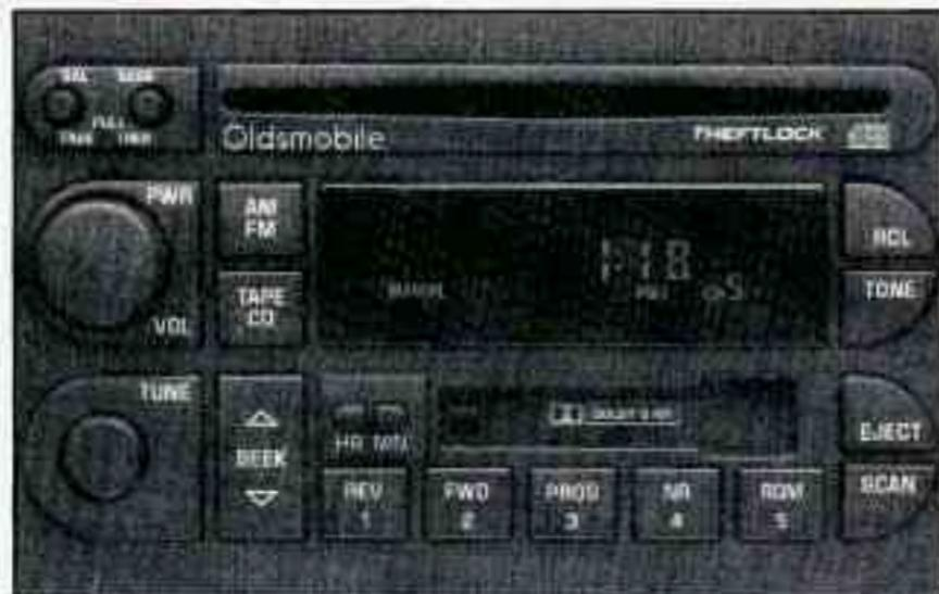
The digital display indicates information on time or radio station frequency, the AM or FM radio band, whether the station is in stereo, and other audio system functions.
