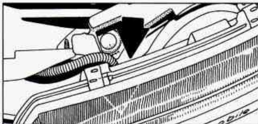
2. Now you can reach in behind the lamp housing and pull out the bulb.
