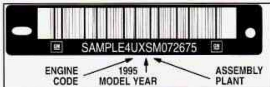
This is the legal identifier for your Aurora. It appears on a plate in the front corner of the instrument panel, on the driver's side. You can see it if you look through the windshield from outside your vehicle. The VIN also appears on the Vehicle Certification and Service Parts labels and the certificates of title and registration.
