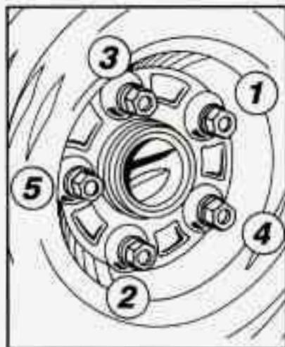
15. In a crisscross sequence, tighten the wheel nuts firmly.
