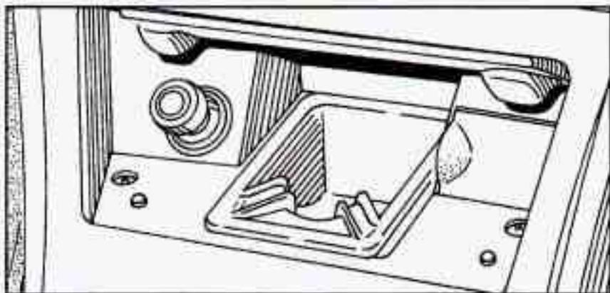
Push and release the cover to reveal the front ashtray, lighter and accessory power outlet.
