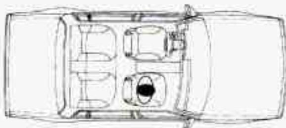
Your vehicle has a right front passenger air bag. *Never* put a rear-facing child restraint in this seat. Here's why:
