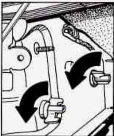
3. Remove the two wing nuts now exposed
