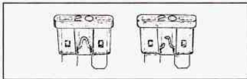
Look at the silver-colored band inside the fuse. If the band is broken or melted, replace the fuse. Be sure you replace a bad fuse with a new one of the correct amp rating.
