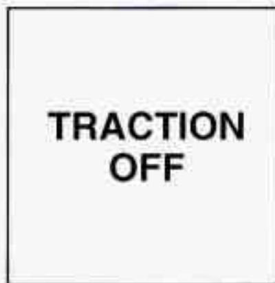
When the system is on, the TRACTION OFF warning light will come on to let you know if there's a problem with your traction control system. See "Traction Control System Warning Light" in the Index. When this warning light is on, the system will not limit wheel spin. Adjust your driving accordingly.
