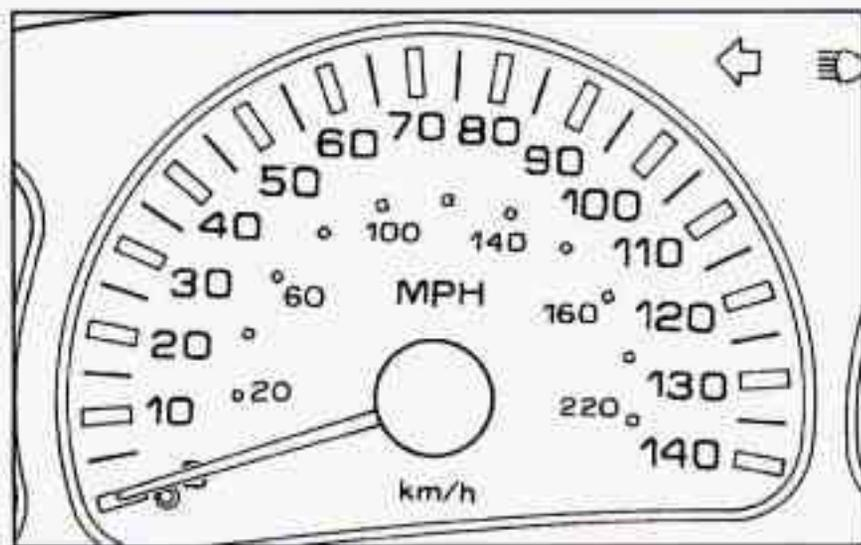
Your speedometer lets you see your speed in both miles per hour (mph) and kilometers per hour (km/h).
