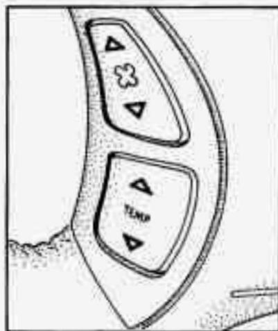
Some heating and cooling controls can be adjusted at the steering wheel. Other touch controls also operate some audio controls. See “Steering Wheel Touch Controls for Audio System” later in this section.
