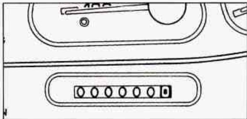
Your odometer shows how far your vehicle has been driven in either miles (used in the United States) or kilometers (used in Canada).
