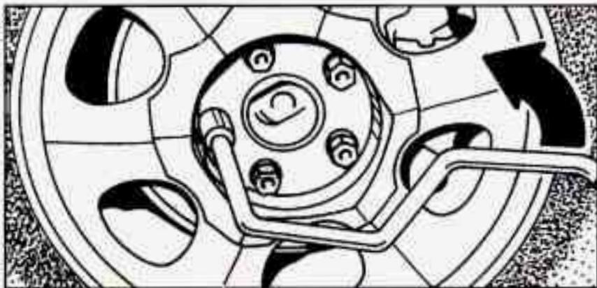
6. Use the wheel wrench to loosen the wheel nuts, but don't remove them.
