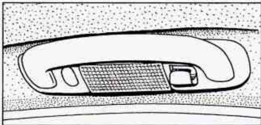
Use the hook marked with the coat hanger symbol to hang garments and coats during trips.
