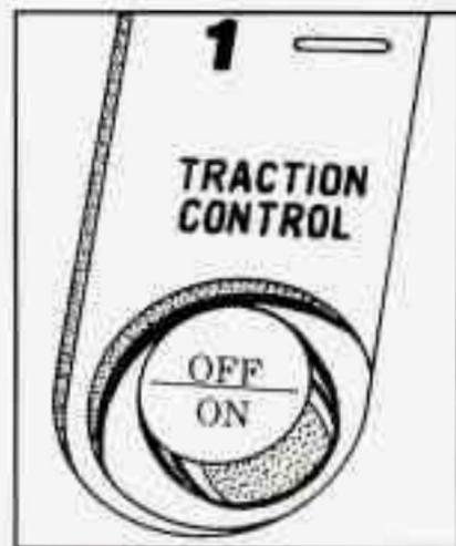
To turn the system off, press the TRACTION CONTROL button on the center console.
