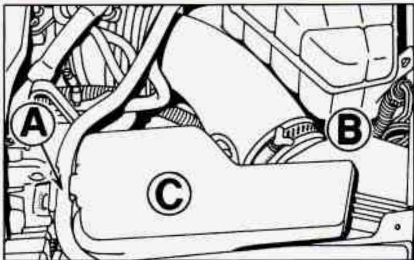
1. Remove hose (A) from resonator channel.
