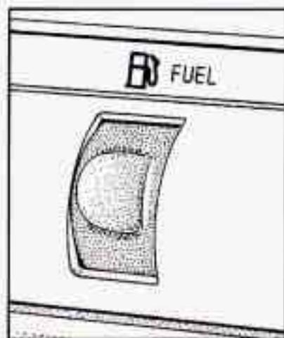
To open the fuel door (on the left of the vehicle), press the button next to the trunk release button, to the right of the steering column. The ignition need not be on. The remote fuel door release will work in all transaxle positions.
