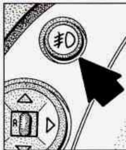
To turn on the fog lamps, first turn on the parking lamps or headlamps. Then press the fog lamp switch. A light will glow on the switch when the switch is on. To turn off the fog lamps, press it again. The fog lamps will also switch off when you turn on your high beam headlamps, but will turn on again when you switch to low beams.
