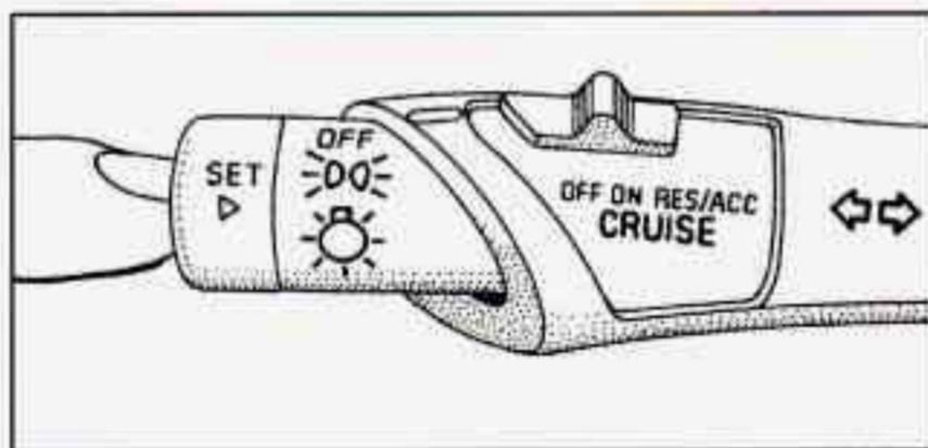
3. Push in the SET button at the end of the lever and release it. The CRUISE light on your instrument panel will come on.
