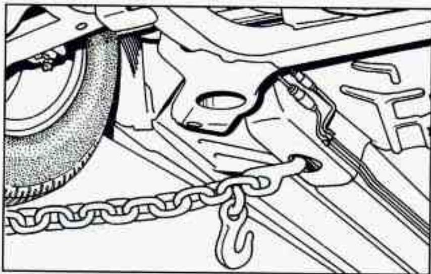
1. Attach T-hook chains into the bottom slots in the cradle behind the front wheels, on both sides.
