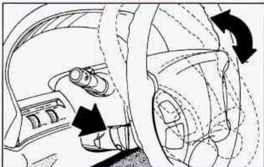
A tilt steering wheel allows you to adjust the steering wheel before you drive. You can also raise it to the highest level to give your legs more room when you exit or enter the vehicle.
