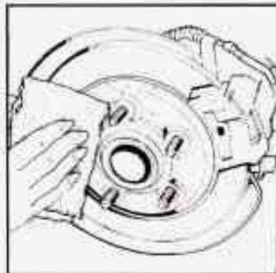
12. Remove any rust or dirt from the wheel bolts, mounting surfaces and spare wheel. Place the spare on the wheel mounting surface.
