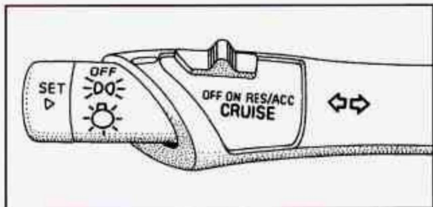
With cruise control, you can maintain a speed of about 25 mph (40 km/h) or more without keeping your foot on the accelerator. This can really help on long trips.
