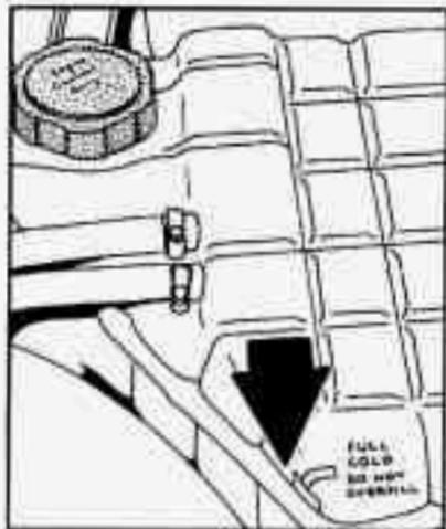
The coolant level should be at or above **FULL COLD**. If it isn't and the **LOW ENGINE COOLANT** message appears on the Driver Information Center, you may have a leak in the radiator hoses, heater hoses, radiator, water pump or somewhere else in the cooling system.
