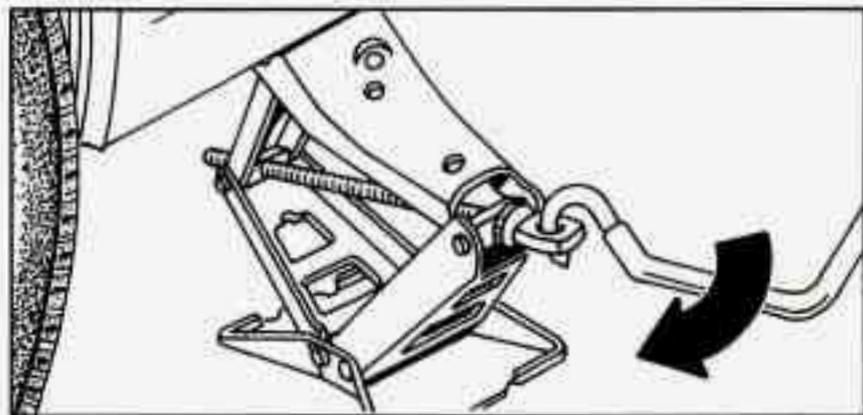
10. Raise the vehicle by rotating the wheel wrench clockwise in the jack. Raise the jack far enough so there's enough room for the spare tire to fit.
