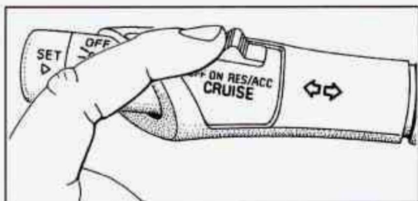
Suppose you set your cruise control at a desired speed and then you apply the brake. This, of course, shuts off the cruise control. But you don't need to reset it. Once you're going about 25 mph (40 km/h) or more, you can move the cruise control switch from ON to RES/ACC (Resume/Accelerate) for about half a second.
