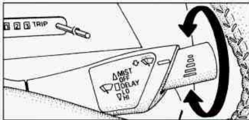
You can set the wiper speed for a long or short delay between wiper cycles. This can be very useful in light rain or snow. Push the lever down to the first detent, DELAY. Turn the band closer to the short lines for fewer wiper passes per minute. As you turn the band toward the long lines, the wiper cycles per minute will increase.
