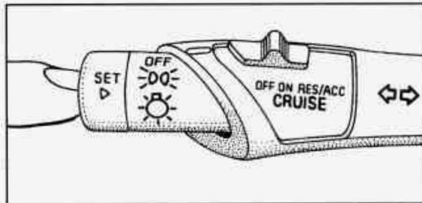
1. Move the cruise control switch to ON.
