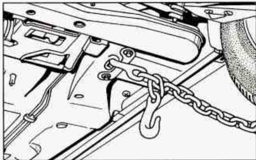
1. Attach T-hook chains on both sides in the slotted holes in the floor pan support rails just ahead of the rear wheels.
