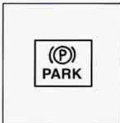
This light will come on when you set your parking brake, and it will stay on if your parking brake doesn't release fully. If you try to drive off with the parking brake set, a chime will also come on until you release the parking brake.
