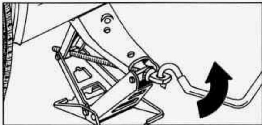
14. Lower the vehicle by rotating the wheel wrench counterclockwise on the jack. Lower the jack completely.
