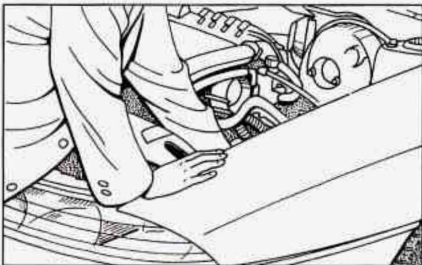
2. Twist the bulb assembly  $1/6$  turn and pull out the bulb assembly.
