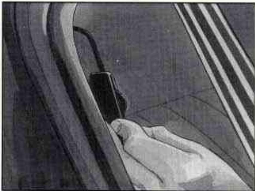
There is one guide for each outside passenger position in the rear seat. You will find them tucked in between the seatback and the interior body, about half-way down the
