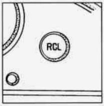
When you press the RCL button, the system scrolls through any currently active warning messages, then returns to the mode the system was in before you pressed RCL.
