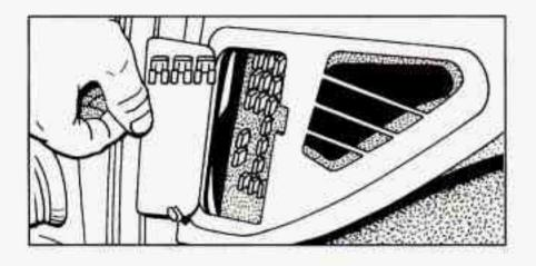
The third fuse panel is located on the left side of the instrument panel. To open it, simply pull on the latch and the door will open.
