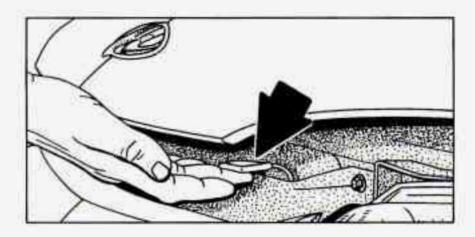
Then go to the front of the vehicle and pull up on the underhood release. Lift the hood.
