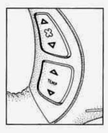
Some heating and cooling controls can be adjusted at the steering wheel. Other touch controls also operate some audio controls. See "Steering Wheel Touch Controls for Audio System" later in this section. Press the upper part of the fan symbol to increase the fan speed; press the lower part of the control to reduce the fan speed.
