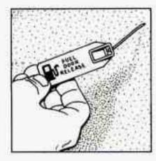
The fuel door can be opened manually in case of an electrical power failure. To do so, first open the trunk. The release mechanism is on the driver's side of the vehicle, at the top of the trunk compartment. Pull the tab toward you to release the fuel door.
