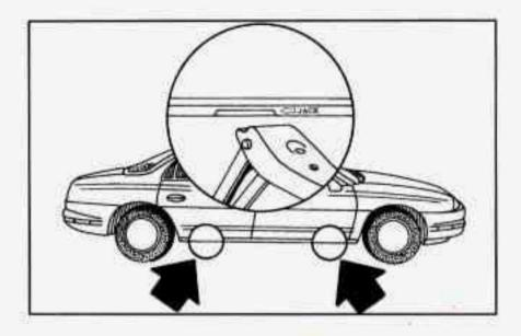
Position the jack and raise the jack head until it fits firmly against the sheet metal next to the word JACK. Do not raise the vehicle yet. Put the compact spare near you.
