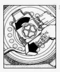
Turn the spare tire retainer bolt counterclockwise until it's loose and remove the retainer assembly.
