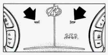
You can sound the horn by pressing the horn symbols on your steering wheel.
