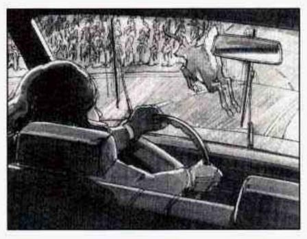
You can steer around the obstacle while braking hard. As you brake, your computer keeps receiving updates on wheel speed and controls braking pressure accordingly. Remember: Anti-lock doesn't change the time you need to get your foot up to the brake pedal. If you get too close to the vehicle in front of you, you won't have time to apply your brakes if that vehicle suddenly slows or stops. Always leave enough room up ahead to stop, even though you have anti-lock brakes.
