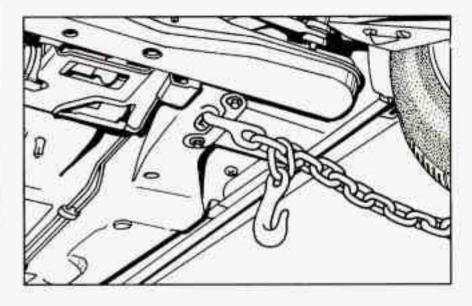
Attach T-hook chains on both sides in the slotted holes in the floor pan support rails just ahead of the rear wheels.
