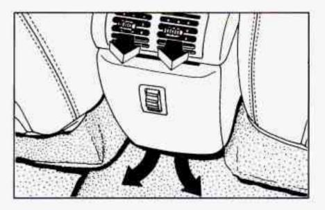
Rotate the control between the outlets up to direct air through the upper outlets. Rotate the control down to direct air through the lower outlets. Adjust the direction of air flow from side to side with the controls in each outlet.
