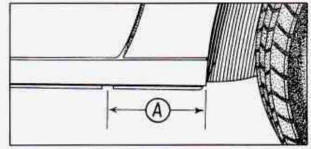
Near each wheel well is a notch on the frame to position the jack head. The front notch is 11 inches (28 cm) back from the front wheel well. The rear notch is 7.5 inches (19 cm) forward from the rear wheel well. You'll find the word JACK and an arrow stamped into the plastic near each notch.
