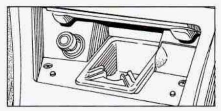
Push and release the cover to reveal the front ashtray, lighter and accessory power outlet.
