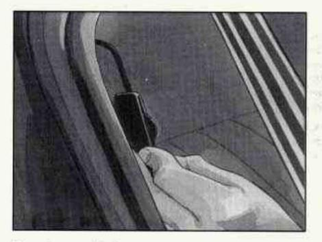
There is one guide for each outside passenger position in the rear seat. You will find them tucked in between the seatback and the interior body, about half-way down the edge of the seatback. Here is how you should install the comfort guides on the shoulder belts:
