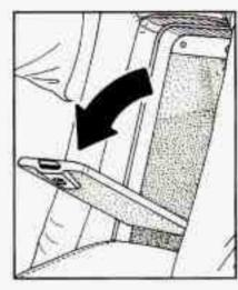
You have a trunk access panel for storing long objects such as skis. Pull the rear armrest down. Then push down on the latch on the trunk access panel to open the panel.
