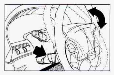
A tilt steering wheel allows you to adjust the steering wheel before you drive. You can also raise it to the highest level to give your legs more room when you exit or enter the vehicle.
