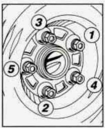
In a crisscross sequence, tighten the wheel nuts firmly.
