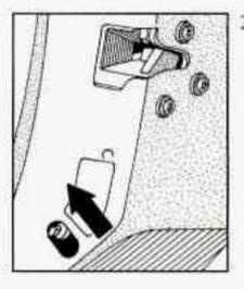
Move the lever on the door all the way up to the ENGAGED position.
