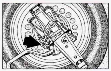
The jack container is labeled PRESS SIDES LIFT TOP. Do this, then remove the jack and wrench.
