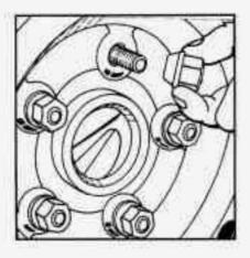
13. Replace the wheel nuts with the rounded end of the nuts toward the wheel. Tighten each nut by hand until the wheel is held against the hub.
