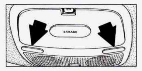
These lamps and the interior courtesy lamps will come on when you open a door. They will turn off when you turn on the ignition. If the door is left open, they will turn off after about 10 minutes.
