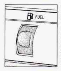
To open the fuel door (on the left of the vehicle), press the button next to the trunk release button, to the right of the steering column. The ignition need not be on. The remote fuel door release will work in all transaxle positions.
