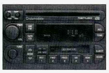
The digital display indicates information on time or radio station frequency, the AM or FM radio band, whether the station is in stereo, and other audio system functions.
