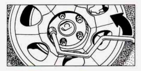
Use the wheel wrench to loosen the wheel nuts, but don't remove them.
