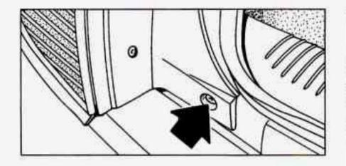
Remove the taillamp filler screw located to the side of the taillamp filler panel.
