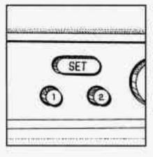
The memory function controls both the driver's seat and outside mirror positions. First position the seat and mirrors where you want them. Next, press the SET button. Within five seconds, press either the 1 or 2 button.
