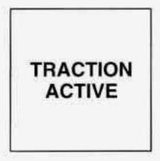
When your traction control system is limiting wheel spin, the TRACTION ACTIVE light will come on. Slippery road conditions may exist if this light comes on, so adjust your driving accordingly. The light will stay on for a few seconds after the traction control system stops limiting wheel spin.
