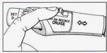
Suppose you set your cruise control at a desired speed and then you apply the brake. This, of course, shuts off the cruise control. But you don't need to reset it. Once you're going about 25 mph (40 km/h) or more, you can move the cruise control switch from ON to RES/ACC (Resume/Accelerate) for about half a second.
