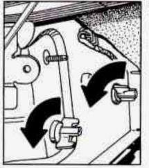
Remove the two wing nuts now exposed
