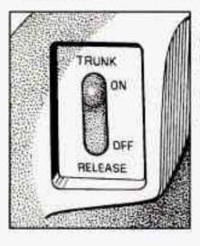
Inside the glove box is an override switch that is useful if you want to leave valuables in the trunk when using a commercial parking lot.
