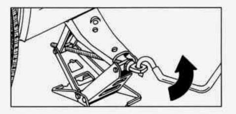
Lower the vehicle by rotating the wheel wrench counterclockwise on the jack. Lower the jack completely.
