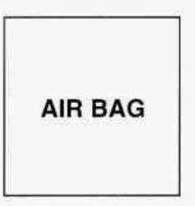
There is an air bag readiness light on the instrument panel, which shows AIR BAG. The system checks the air bag's electrical system for malfunctions. The light tells you if there is an electrical problem. See "Air Bag Readiness Light" in the Index for more information.
