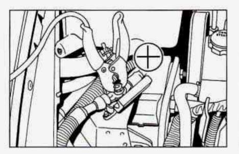
Connect the red positive (+) cable to the remote positive (+) terminal of the vehicle with the dead battery.
