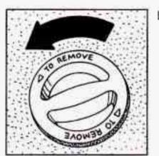
Turn the center retainer bolt on the spare tire cover counterclockwise to remove it, then lift the tire cover.
