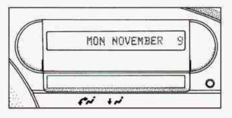
You will need to open the cover to access the control buttons. To open the cover, push the button located to the right of the cover.
