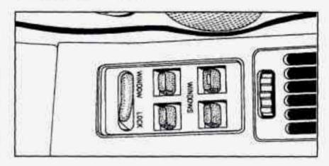
Switches on the driver's armrest control each of the windows when the ignition is on. In addition, each passenger door has a switch for its own window.
