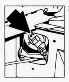
Unclip the bulb assembly from the wiring harness and replace the bulb assembly.
