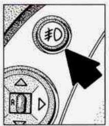
To turn on the fog lamps, first turn on the parking lamps or headlamps. Then press the fog lamp switch. A light will glow on the switch when the switch is on. To turn off the fog lamps, press it again. The fog lamps will also switch off when you turn on your high beam headlamps, but will turn on again when you switch to low beams.
