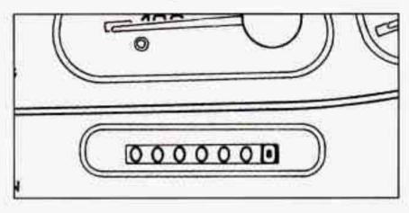
Your odometer shows how far your vehicle has been driven in either miles (used in the United States) or kilometers (used in Canada).
