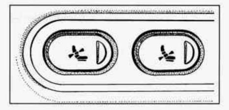
The rear lumbar control adjusts upper lumbar support; the front control adjusts lower lumbar support.
