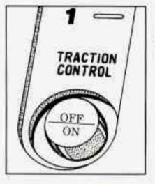
To turn the system off, press the TRACTION CONTROL button on the center console. The TRACTION OFF warning light will come on and stay on. If the system is limiting wheel spin when you press the button, the system won't turn off right away. It will wait until there's no longer a current need to limit wheel spin.
