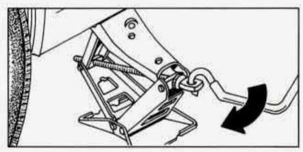
Raise the vehicle by rotating the wheel wrench clockwise in the jack. Raise the jack far enough so there's enough room for the spare tire to fit.
