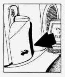
To open the hood, first pull the hood release handle inside the vehicle, located to the left of the steering wheel under the instrument panel.
