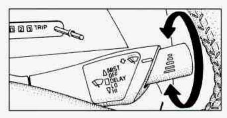
You can set the wiper speed for a long or short delay between wiper cycles. This can be very useful in light rain or snow. Push the lever down to the first detent. DELAY. Turn the band closer to the short lines for fewer wiper passes per minute. As you turn the band toward the long lines, the wiper cycles per minute will increase.
