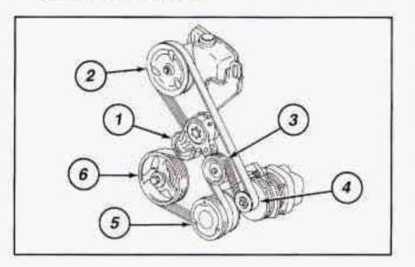
The 4.0L Aurora engine uses an engine accessory belt. This diagram shows the features connected by the belt routing. See "Maintenance Schedule" in the Index for when to check the belt.
