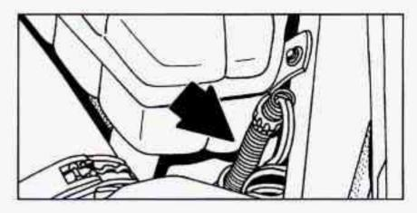
In very cold weather, 0°F (-18°C) or colder, the engine coolant heater can help. You'll get easier starting and better fuel economy during engine warm-up. Usually, the coolant heater should be plugged in a minimum of four hours prior to starting your vehicle.
