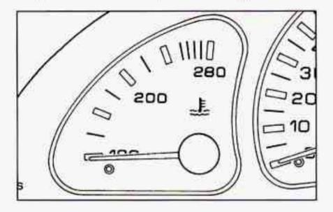
This gage shows the engine coolant temperature.
