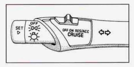
With cruise control, you can maintain a speed of about 25 mph (40 km/h) or more without keeping your foot on the accelerator. This can really help on long trips.
