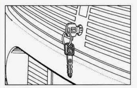
To unlock the trunk from the outside, insert the door key and turn it.
