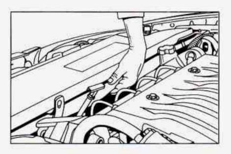
With the coolant surge tank pressure cap off, start the engine and let it run until you can feel the upper radiator hose getting hot. Watch out for the engine fans. By this time, the coolant level inside the coolant surge tank may be lower. If the level is lower, add more of the proper mix to the coolant surge tank until the level reaches FULL COLD.
