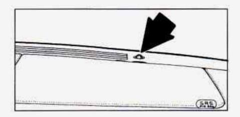
Your system has two sun sensors on top of the instrument panel that detect direct sunlight and the increased warming caused by it. To keep you comfortable, the sensors may reduce the interior temperature by as much as 5°F (3°C) below the setting on the digital screen, if necessary. Be careful not to put anything over these sun sensors. If you do, the system will think it's night and warm up the vehicle.
