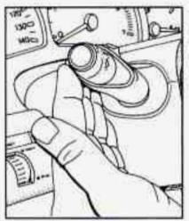
To change the headlamps from low beam to high or high to low, pull the turn signal lever all the way toward you. Then release it.
