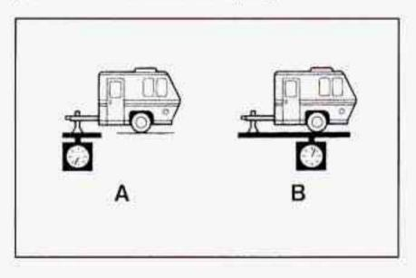
If you're using a "dead-weight" hitch, the trailer tongue (A) should weigh 10% of the total loaded trailer weight (B). If you have a "weight-distributing" hitch, the trailer tongue (A) should weigh 12% of the total loaded trailer weight (B).
