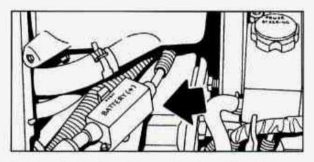
Open the hoods and locate the other vehicle's battery and the Aurora's remote positive (+) jump starting terminal.
