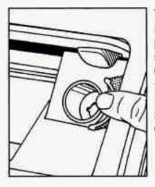
The power outlet inside the front ashtray can be used to plug in electrical equipment such as a cellular telephone. CB radio, etc. Follow the proper installation instructions that are included with any electrical equipment you install.
