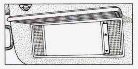
When you open the cover to either visor vanity mirror, the lamps will come on. You can adjust the brightness of the lamps with the switch.
