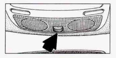
To open the sunroof, press the control switch rearward and release it to open the glass panel and sunshade.
