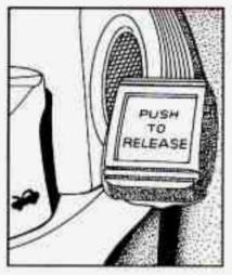
To set the parking brake, hold the regular brake pedal down with your right foot. Push down the parking brake pedal with your left foot. If the ignition is on, the parking brake indicator light will come on.
