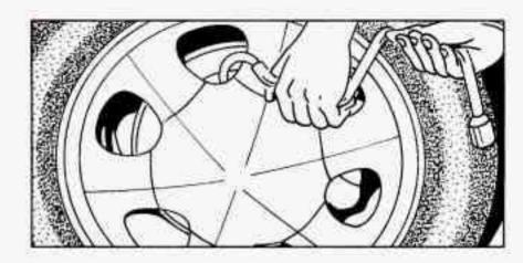
Insert the hooked end of the wheel wrench in one of the two small notches in the center cover and pry the cover off. Do not drop the cover or lay it face down, as it could be scratched or damaged.
