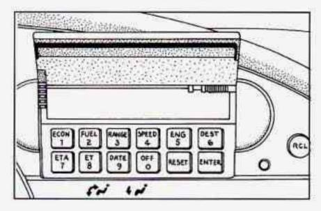
The Driver Information Center (DIC) displays information in either English or metric. When the system is on or off, hold the OFF button down for five seconds to change the display between English and metric. This will also change the digital screen for the climate control system between English and metric.
