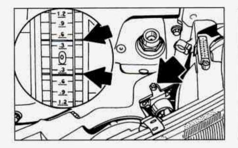
Check the vertical aim for each headlamp and adjust it as necessary. Turn the vertical aiming screw until the bubble in the level is centered at 0 (zero).
