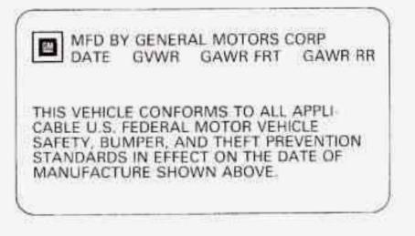
The other label is the Certification label, found on the rear edge of the driver's door. It tells you the gross weight capacity of your vehicle, called the GVWR (Gross Vehicle Weight Rating). The GVWR includes the weight of the vehicle, all occupants, fuel and cargo. Never exceed the GVWR for your vehicle, or the Gross Axle Weight Rating (GAWR) for either the front of rear axle.
