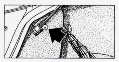
In the trunk, remove the convenience net from the hooks. Next remove the plastic screws holding the carpeting in place and pull back the carpeting.
