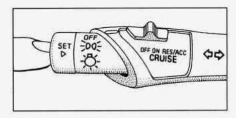
1. Move the cruise control switch to ON.
