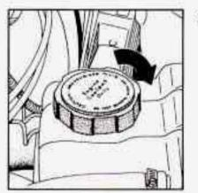
Then replace the pressure cap. Be sure the pressure cap is tight.
