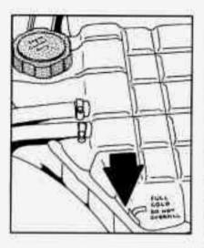
The coolant level should be at or above FULL COLD. If it isn't and the LOW ENGINE COOLANT message appears on the Driver Information Center, you may have a leak in the radiator hoses, heater hoses, radiator, water pump or somewhere else in the cooling system.
