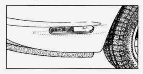
The cornering lamps are designed to come on when you signal a turn. This will provide more light for cornering at night.
