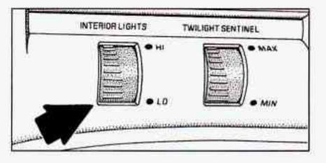
You can brighten or dim your instrument cluster, radio and climate control displays and control lights by rotating the INTERIOR LIGHTS control between LO and HI when your lights are on. Rotate the control all the way to HI and you will turn on the interior courtesy lamps.
