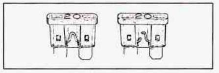
Look at the silver-colored band inside the fuse. If the band is broken or melted, replace the fuse. Be sure you replace a bad fuse with a new one of the correct amp rating.
