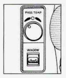
With this feature, the right front seat passenger can control the temperature of heated air for his/her own zone. To turn on the system, adjust the control on the passenger side armrest to the temperature setting desired. The system can also be turned on and off by pressing the PASS TEMP button on the comfort control system on the instrument panel.
