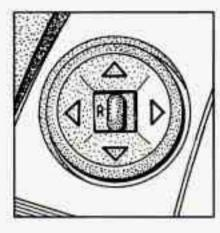
The controls on the far left of the instrument panel control both outside rearview mirrors. Move the center switch to the left to select the driver's side rearview mirror, or to the right to select the passenger's side rearview mirror.
