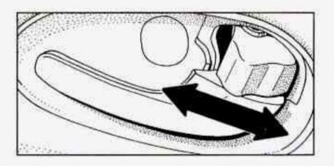
From the inside, to lock the door, rotate the locking lever forward.
