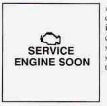
A computer monitors operation of your fuel, ignition and emission controls systems. This light should come on when you start your engine as a check to show you it is working. **Oil Pressure Warning Light**
