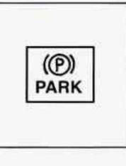
This light will come on when you set your parking brake, and it will stay on if your parking brake doesn't release fully. If you try to drive off with the parking brake set, a chime will also come on until you release the parking brake.
