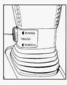
This button lets you change from a normal driving mode to a power mode. For general driving conditions, use the normal mode.
