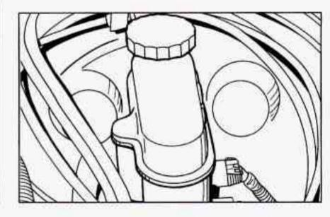
There are only two reasons why the brake fluid level in your master cylinder might go down. The first is that the brake fluid goes down to an acceptable level during normal brake lining wear. When new linings are put in, the fluid level goes back up. The other reason is that fluid is leaking out of the brake system. If it is, you
