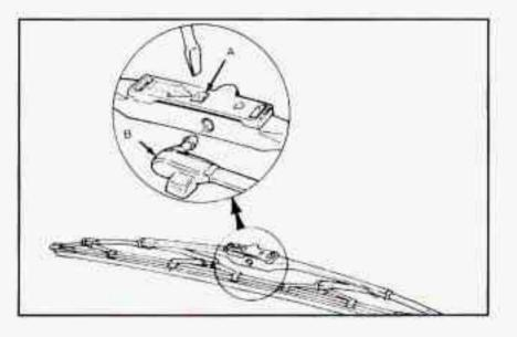
Replacement blades come in different types and are removed in different ways. Here's how to remove the type with a release hole:
