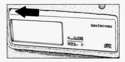
Close the door by sliding it all the way to the left. If the door is left partially open, the changer will not operate and an error will occur.
