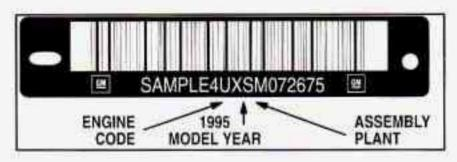
This is the legal identifier for your Aurora. It appears on a plate in the front corner of the instrument panel, on the driver's side. You can see it if you look through the windshield from outside your vehicle. The VIN also appears on the Vehicle Certification and Service Parts labels and the certificates of title and registration.
