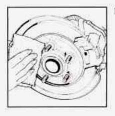
Remove any rust or dirt from the wheel bolts, mounting surfaces and spare wheel. Place the spare on the wheel mounting surface.
