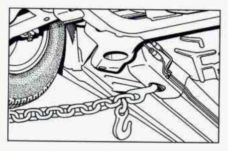
Attach T-hook chains into the bottom slots in the cradle behind the front wheels, on both sides.
