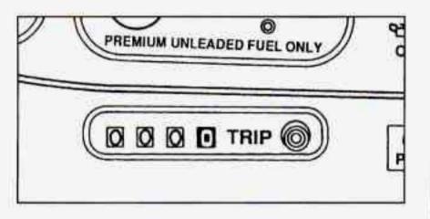
Your trip odometer tells you how far you have driven since you last reset it. Press the trip button located next to the trip odometer, below the fuel gage.
