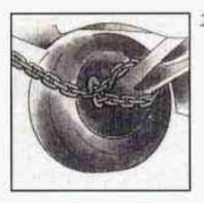
Attach a separate safety chain around the outboard end of each control arm.
