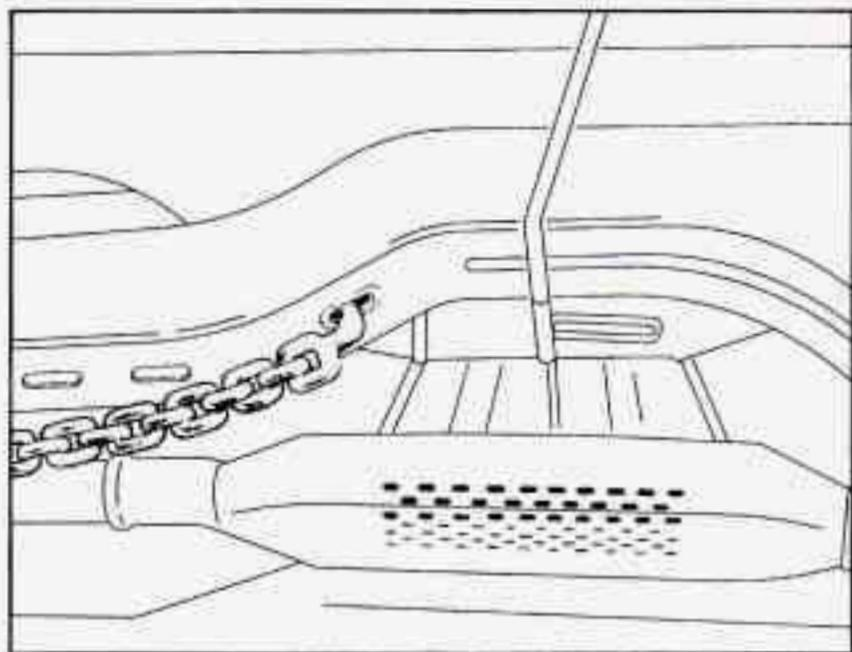
1. Attach T-hook chains on both sides, in the slotted holes in the bottom of the frame rails, about two feet behind the front wheels.
