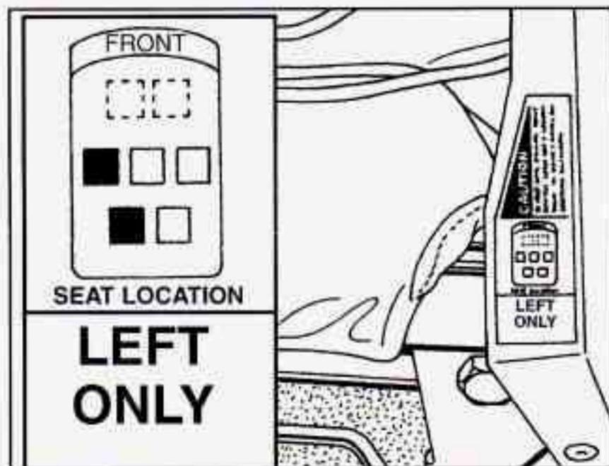
There are three types of rear bucket seats: **RIGHT ONLY**, **CENTER OR LEFT** and **LEFT ONLY**. **RIGHT ONLY** and **LEFT ONLY** seats may be equipped with the built-in child restraint option.
