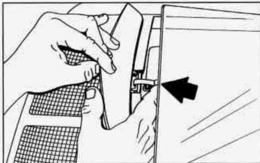
9. Attach the spring clips to the taillamp housing and secure them.
