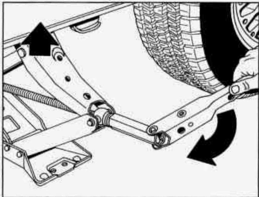
11. Raise the vehicle by rotating the folding wrench clockwise in the jack. Raise the vehicle far enough off the ground so there is enough room for the spare tire to fit.
