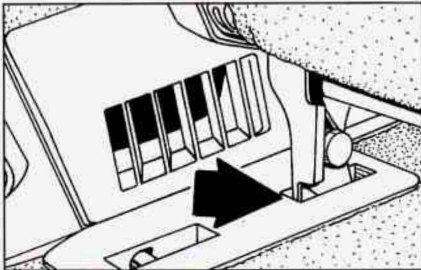
**Rear Air Vents:** To maximize airflow through the rear heater outlet, place the left second row bucket seat in the forward position (see "Adjusting Rear Seats" in the Index).
