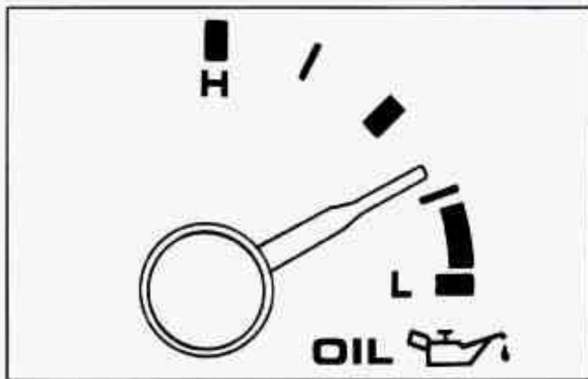
Your vehicle is equipped with an oil pressure indicator rather than an oil pressure gage. Your oil pressure indicator lets you know when you may have a problem with your engine oil pressure.
