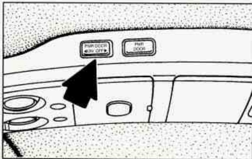
With this option, you can open and close the sliding door with switches inside your vehicle. If you have the optional Remote Lock Control system, you can also operate the sliding door with your remote transmitter. See "Remote Lock Control" in the Index.
