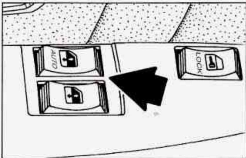
With power windows, switches on the driver's door armrest control the front windows (when the ignition is on). The left switch controls the driver's window. The right switch controls the passenger's window.
