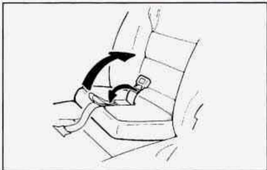
1. Make sure that the crotch strap is held flush to the child restraint cushion with the fastener strip. Also be sure the shoulder harness adjustment strap (gray) is folded up in the seat. This will allow the cushion to fold completely into the seatback. Raise the cushion.
