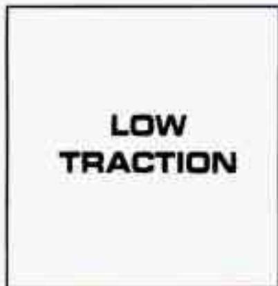
If your vehicle has the traction control system, there will be a LOW TRACTION light on the instrument panel.
