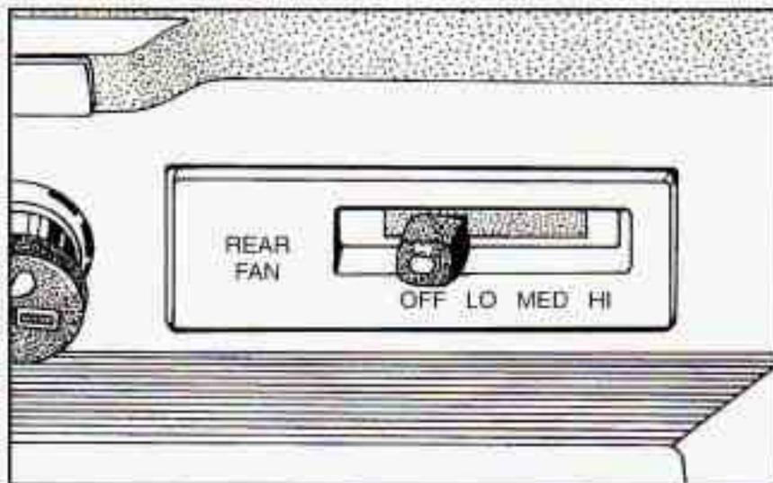
Your vehicle will have a rear air outlet and a rear fan. To maximize airflow to the rear of your vehicle, place the left second row bucket seat in the forward position (see "Adjusting Rear Seats" in the Index). This uncovers the rear air outlet.
