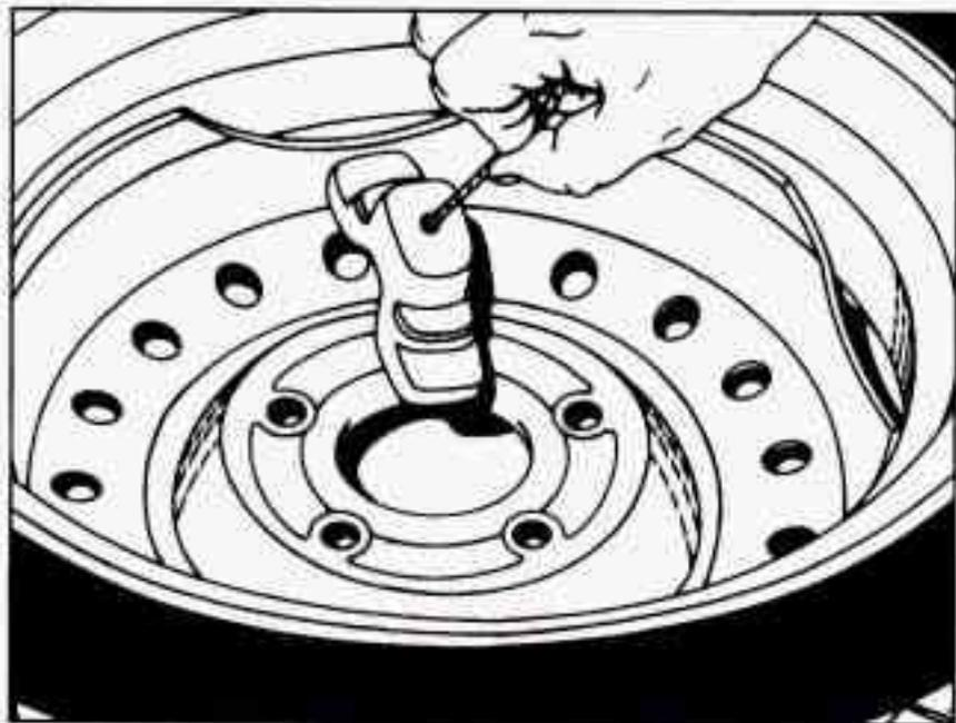
6. Slide the cable retainer through the center of the spare, then place the compact spare tire near the flat tire.
