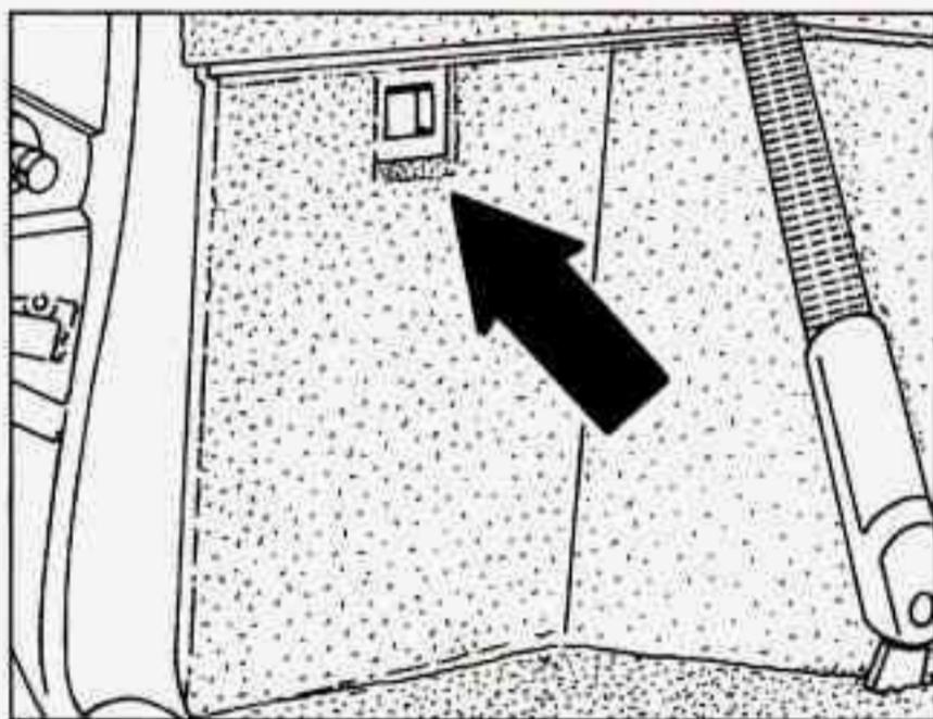
The power outlet is located in the rear compartment on the driver's side. To open, slide the latch down and remove the cover.
