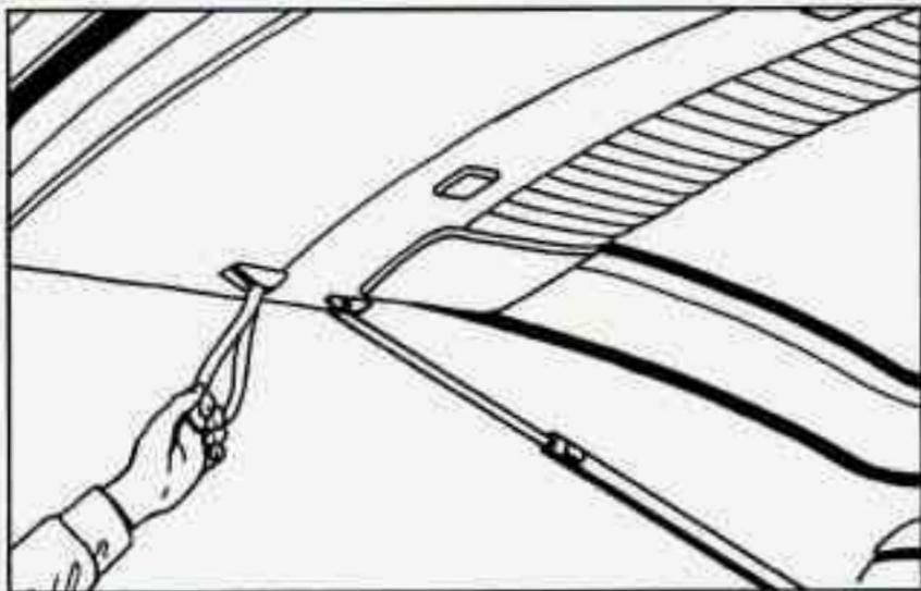
To close the liftgate, pull down on the strap, then firmly shut the liftgate. Don't drive with the liftgate open, even slightly. See "Exhaust" in the Index.
