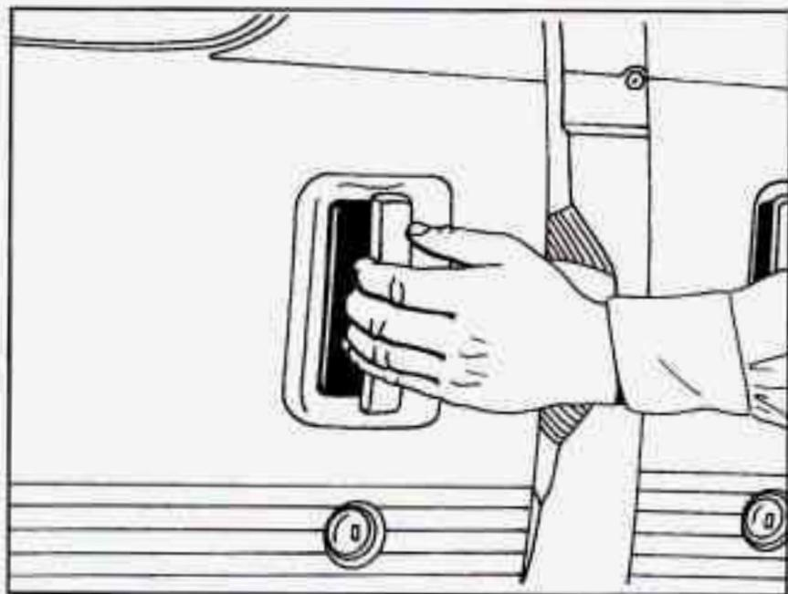
To move the door forward, you must first pull the inside or outside latch release out and then forward, or the door will remain latched in the open position.
