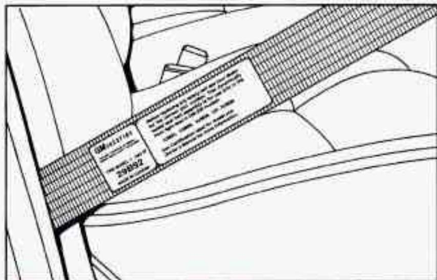
The model number on the replacement belt must be listed on the safety belt you want to replace. Pull the shoulder belt all the way out to see this label.
