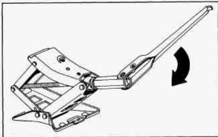
9. Attach the folding wrench to the jack, and rotate the wrench clockwise to raise the jack head a few inches.
