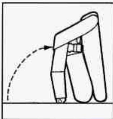
The second and third row bucket seats have been designed to allow them to fold fully upward and forward when the seats are anchored in the rear-most position. This design improves both luggage/cargo capacity and rear seat entry/exit.
