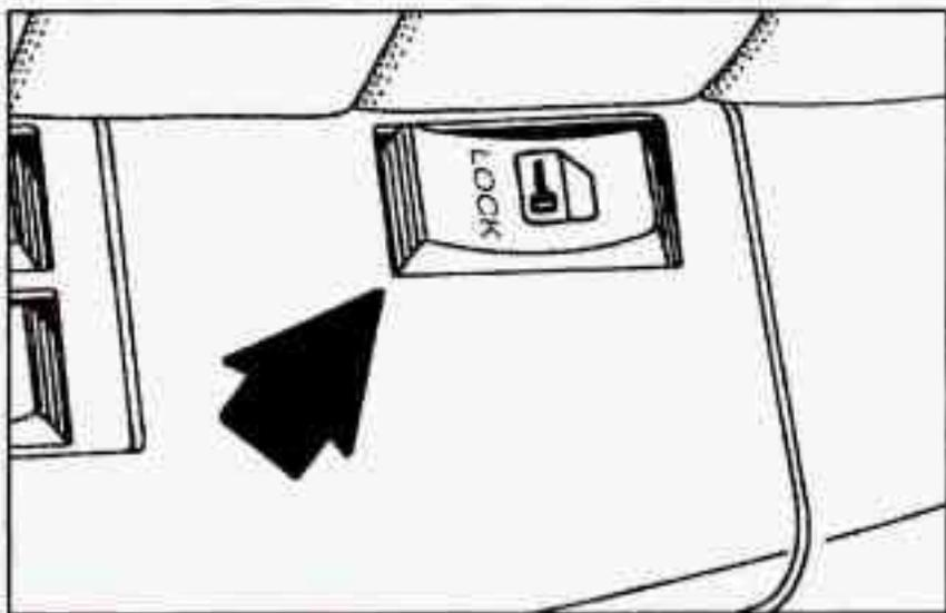
From the inside, press the front of the power door lock switch (on either front door), to unlock all doors and the liftgate.
