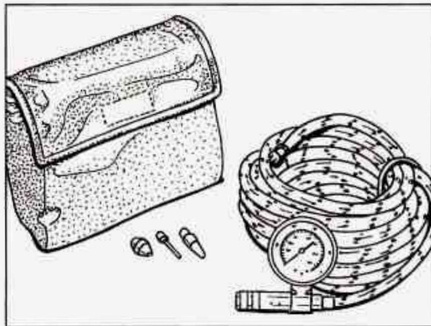
The air inflator kit is stored in a pouch in the glove box. It includes a 20-foot (6 m) hose with an air pressure gage, nozzle adapters and instructions.
