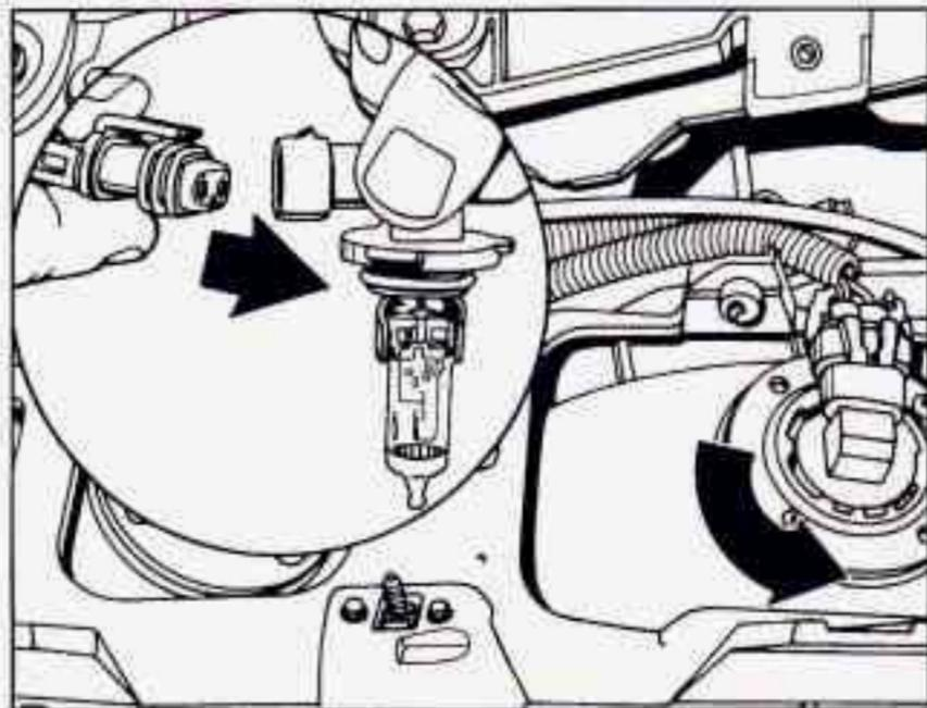
3. Twist the L-shaped bulb assembly counterclockwise 1/6 turn until the flanges align with the slots in the retainer ring.
