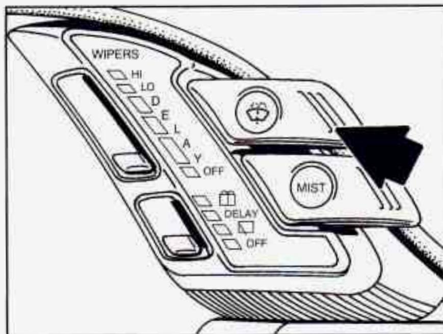
To wash your windshield, press and hold the windshield washer switch. The washers and wipers will operate. When you release the switch, the washers will stop, and the wipers will continue to operate for two cycles, unless your wipers had already been on. In that case, the wipers will resume the wiper speed you had selected earlier.
