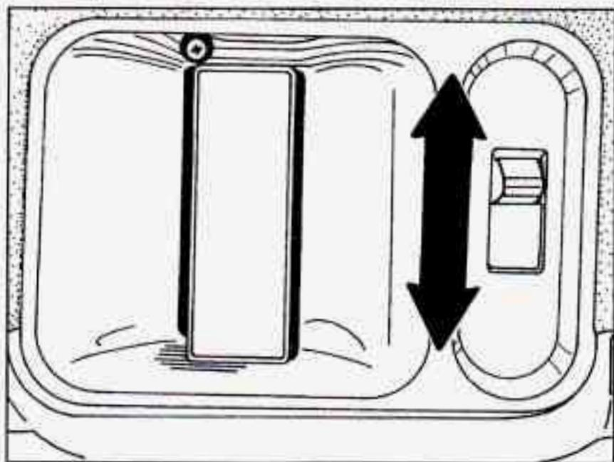
Lock the sliding door from the inside by sliding the manual locking lever down. Unlock it by sliding the lever up.
