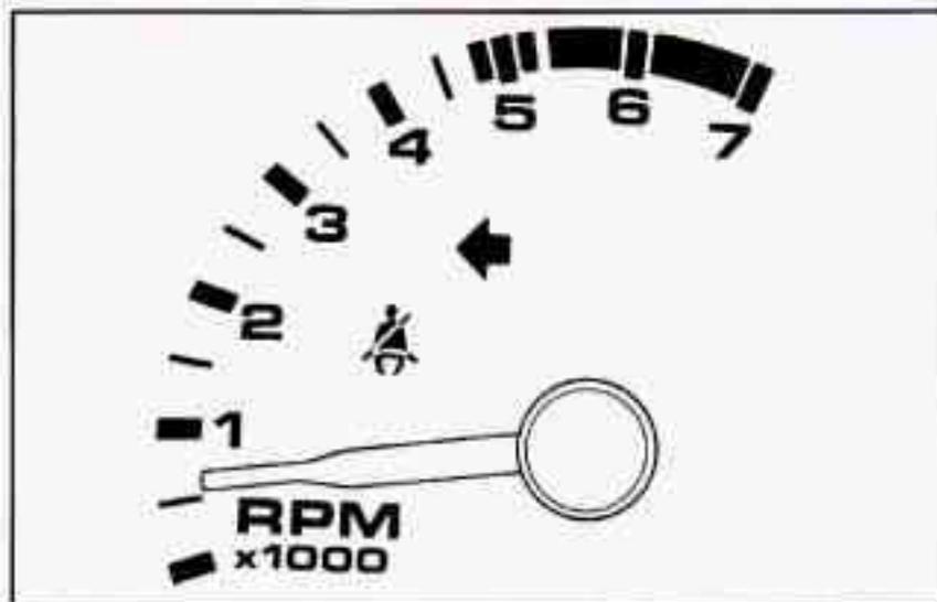
The tachometer displays the engine speed in revolutions per minute (rpm).
