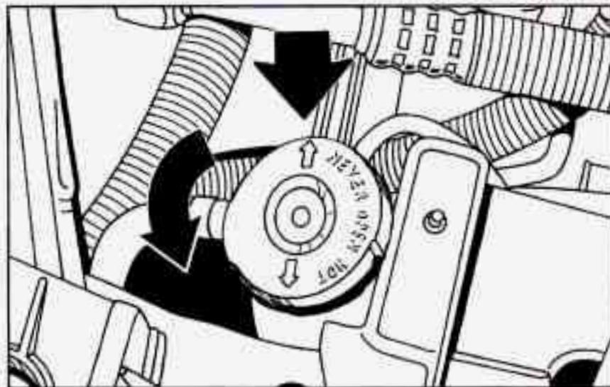
**3.1L V6: Removing the Pressure Cap**
