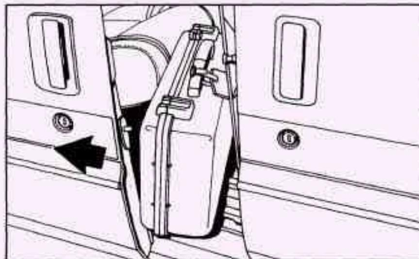
If anything obstructs the power sliding door while it is closing, the door will automatically reverse to the open position, provided it meets sufficient resistance. Resistance must be as strong as the force of the closing door, or stronger. The force of the closing door increases significantly as the door approaches the latch position.
