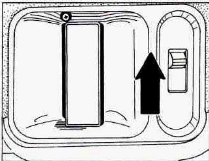
If you have the optional power sliding door, slide the power sliding door enable switch to the ON position. Press either PWR DOOR switch.
