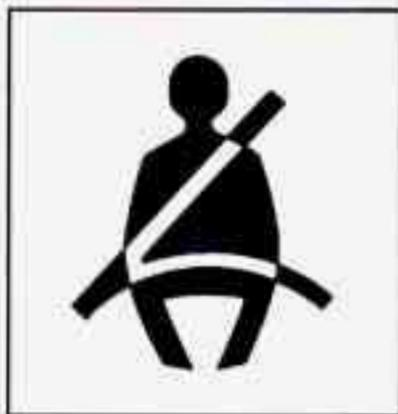
When the key is turned to RUN or START, a chime will come on for about eight seconds to remind people to fasten their safety belts, unless the driver's safety belt is already buckled. The safety belt light will also come on and stay on until the driver's belt is buckled.
