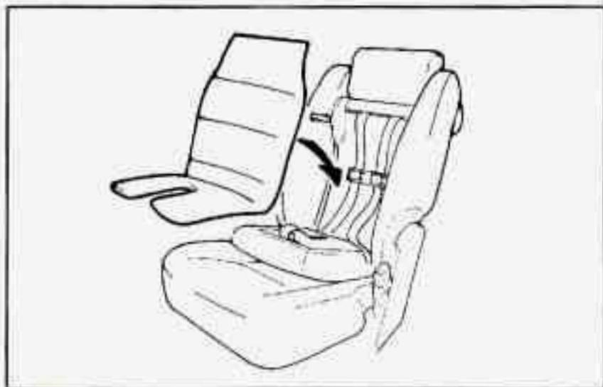
3. Store the 5-point child restraint harness behind the removable pad. The pad is held in place by fastener strips.
