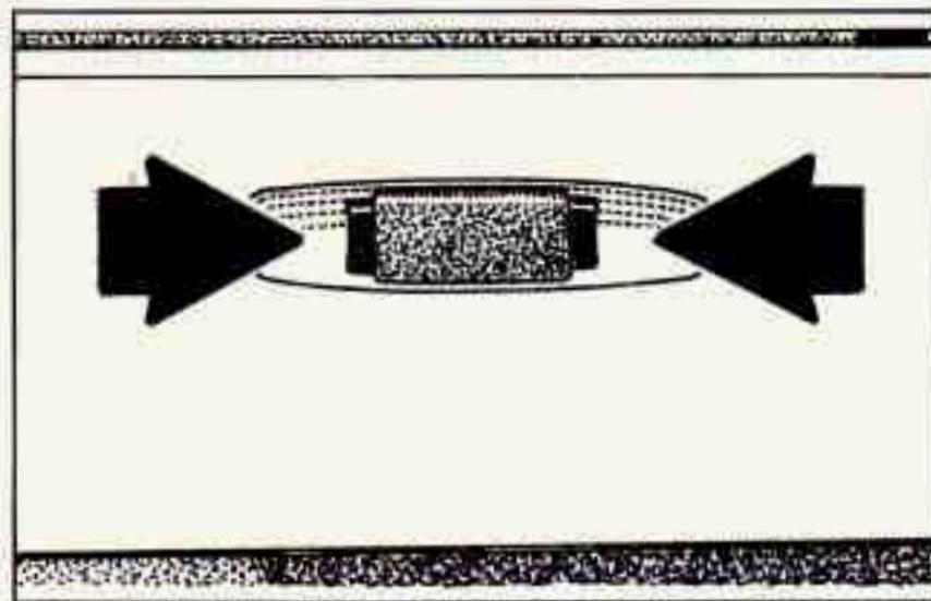
To open the glove box, pinch the latch release.
