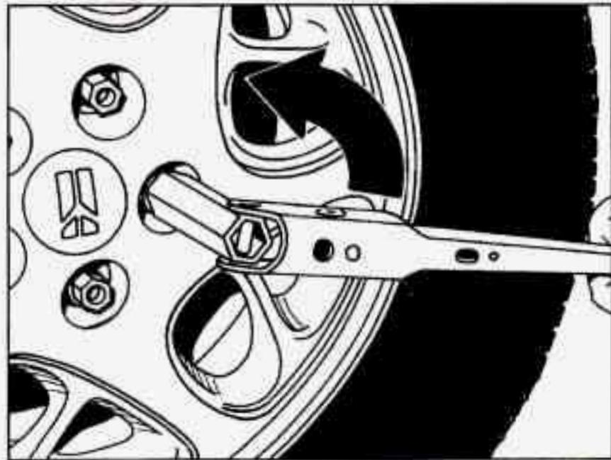
8. Loosen the wheel nuts -- but do not remove them -- using the folding wrench.
