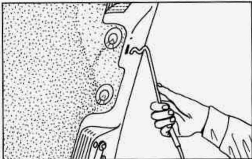
The hood prop rod may be hot due to increased engine temperatures under the hood, so be careful when handling it. Use your hood prop sleeve when handling the prop.
