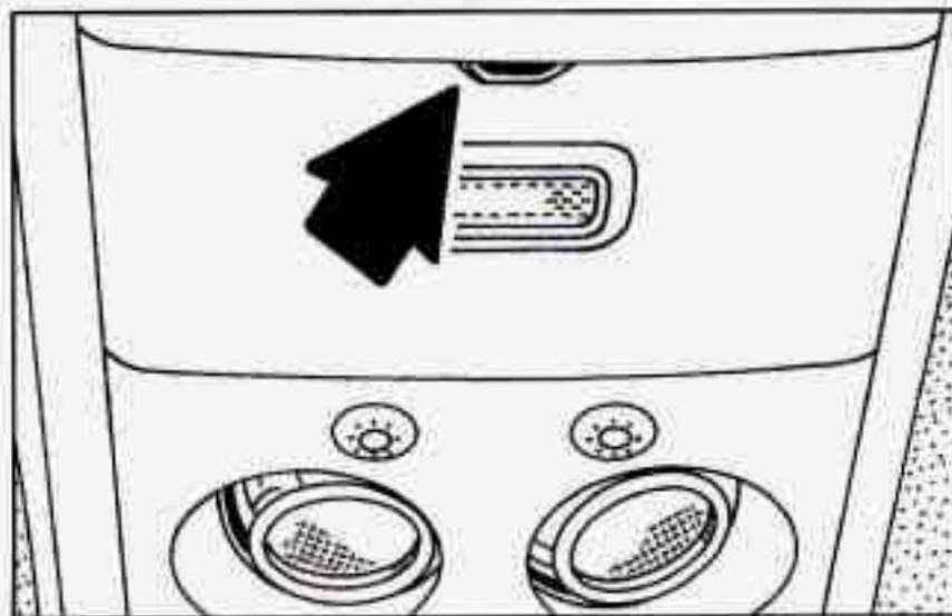
**GARAGE DOOR OPENER COMPARTMENT:** You can store your garage door opener in the front compartment of your overhead console, and operate it from this position. To install your garage door opener, follow these instructions:
