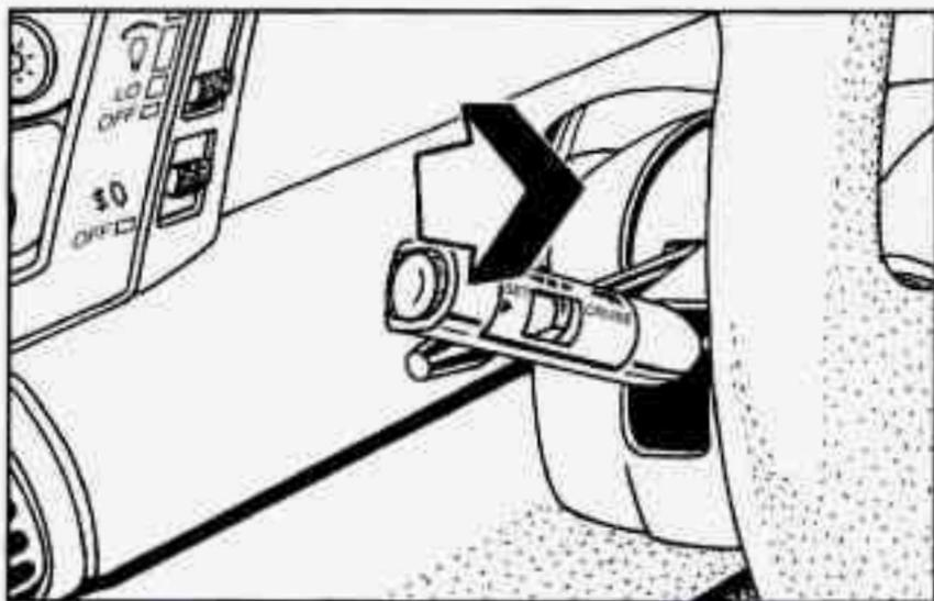
To change the headlamps from high to low beam, or low to high, simply pull the turn signal lever all the way toward you. Then release it.
