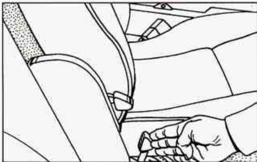
The **RIGHT ONLY** seats have a lower lever to tilt the seat forward. To get into third row seats, push back the lower lever on the **RIGHT ONLY** seat (nearest the sliding door) and tilt the seat forward completely. To return the seat to its normal position, pull the seat back, holding the lower lever back. Once the seat is in place, release the lower lever. Push and pull on the seat to be sure that it is locked.
