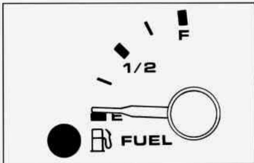
When there is between 3 gallons (11 liters) and 0.5 gallon (1.8 liters) of fuel left in the tank, the warning light next to the fuel symbol will go on.
