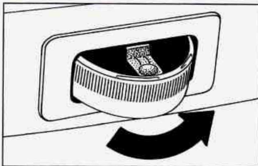
To open the ashtray, press the right side and turn it open. To remove the ashtray for cleaning, press the snuffer as you lift up the bottom of the ashtray.
