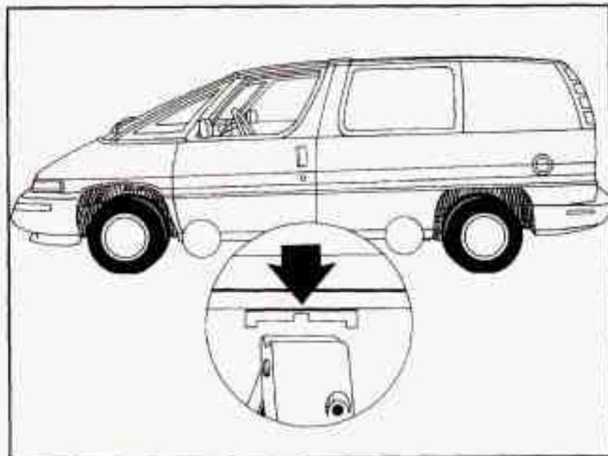
10. Near each wheel, there is a notch in the vehicle's frame. Position the jack and raise the jack head until it fits firmly into the notch in the vehicle's frame (nearest the flat tire). Do not raise the vehicle yet. Put the compact spare tire near you.
