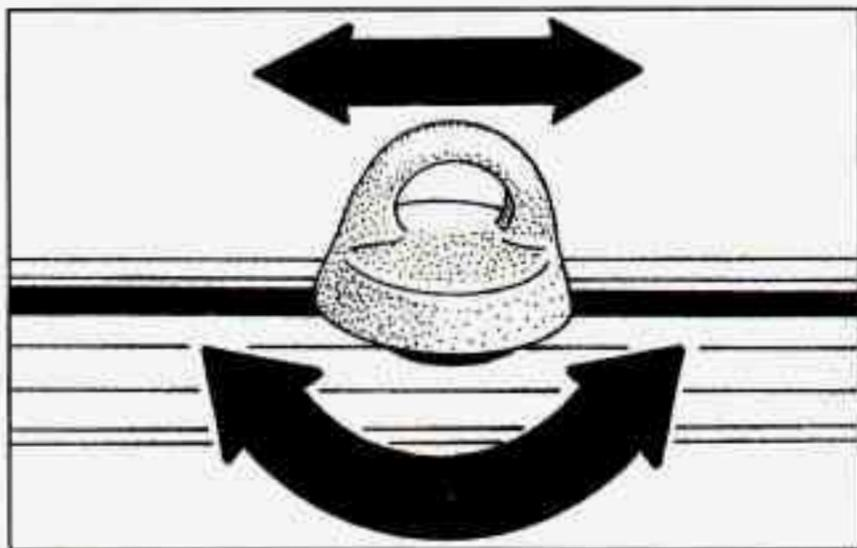
Use the adjustable tiedown loops in the side rails to help secure large loads. Reposition the tiedowns by turning them counterclockwise, then slide them along the side rail. Turn the tiedowns clockwise to tighten them in place.
