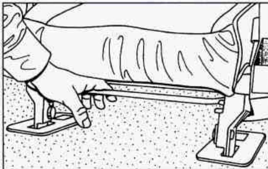
To get out of the third row seats, push down on the rear release bar under the seat ahead of you to tilt the entire seat forward.
