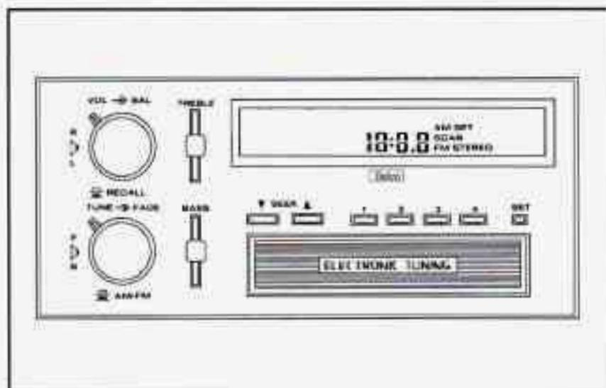
The digital display indicates information on time or radio station frequency, the AM or FM radio band, whether the station is in stereo, and other radio functions.
