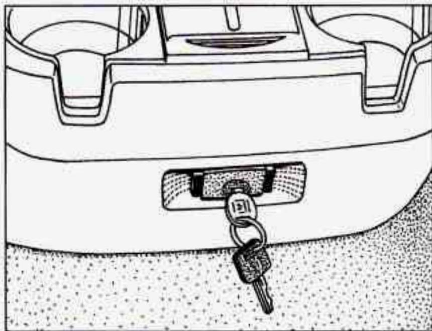
At the base of the center instrument panel console is a storage bin. Use the door key to lock and unlock it. To open the bin, pinch the latch release. Inside the storage bin will find a coinholder.
