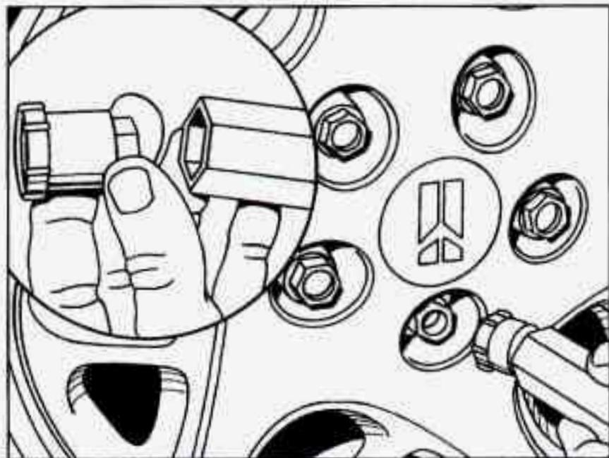
7. Each wheel nut is covered with a nylon cap. Use the folding wrench to remove the nylon caps from the wheel nuts before you loosen the nuts.
