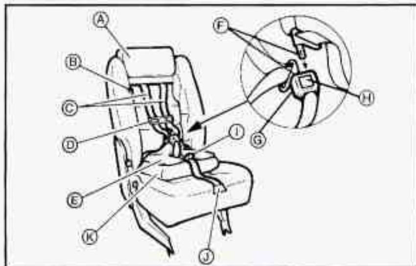
If you have a rear seat with the optional built-in child restraint, refer to this picture to become familiar with the parts of each child seat and 5-point harness listed next.
