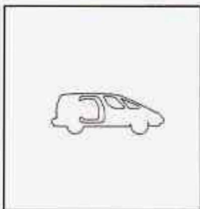
With the optional power sliding door, the sliding door ajar symbol on your instrument panel will come on if your sliding door is not completely closed.
