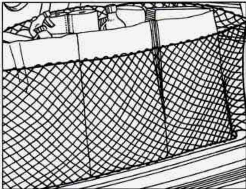
The optional convenience net is designed to help keep small loads, like grocery bags, from falling over during sharp turns or quick stops and starts.
