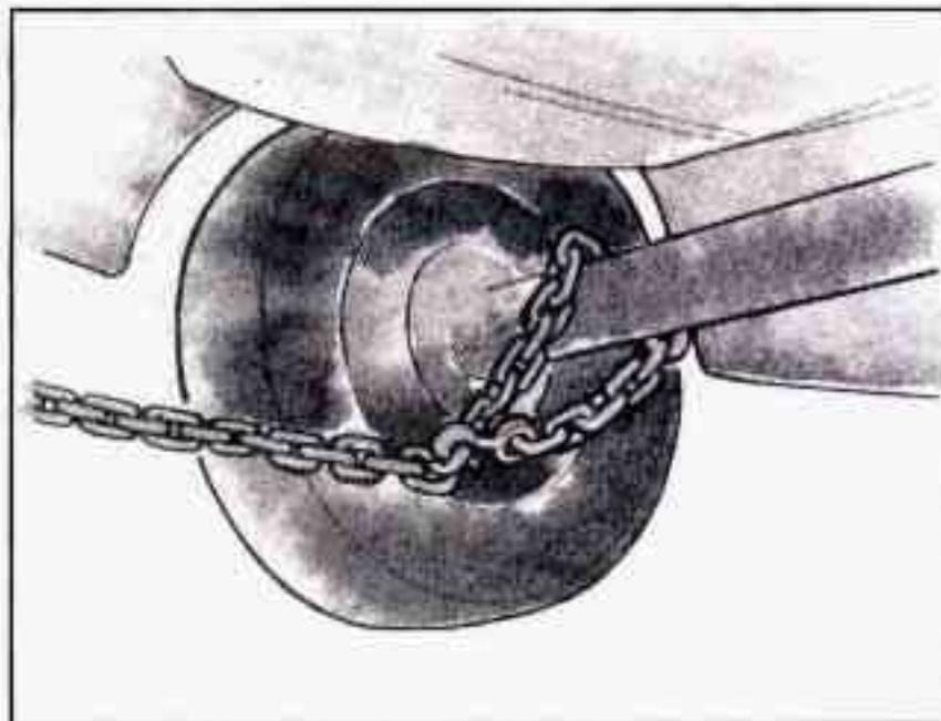
3. Attach a separate safety chain around the end of each axle inboard of the spring.
