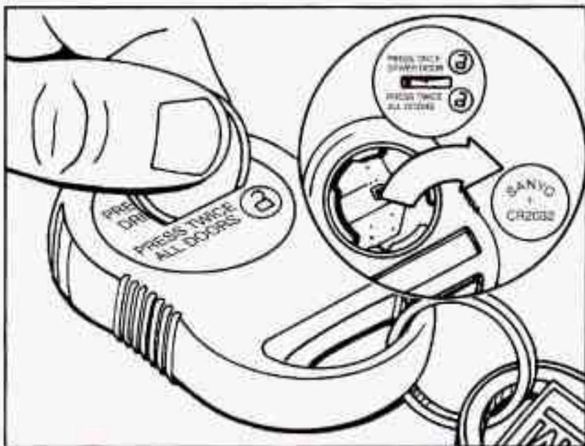
1. Insert a coin into the slot in the back of the transmitter, and turn it counterclockwise to open the cover.
