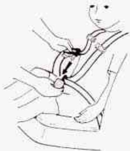
5. Place the child in the child restraint and put a shoulder harness strap over each shoulder. Insert both seat belt latch plates into the buckle and pull up on them to make sure they are firmly latched.
