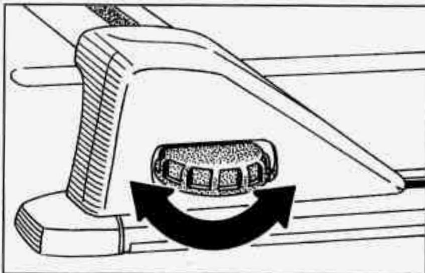
Your luggage carrier has release knobs set in the ends of each crossrail. Turn the release knobs counterclockwise to unlock the crossrails. Slide the crossrails forward or back, as needed, to accommodate loads of varying size.
