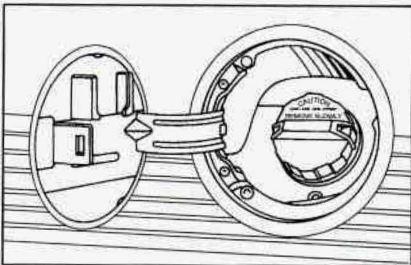
The cap is behind a hinged door on the driver's side of your vehicle. You will notice that on the inside of the hinged door there is a place to hold the gas cap while you are adding fuel.
