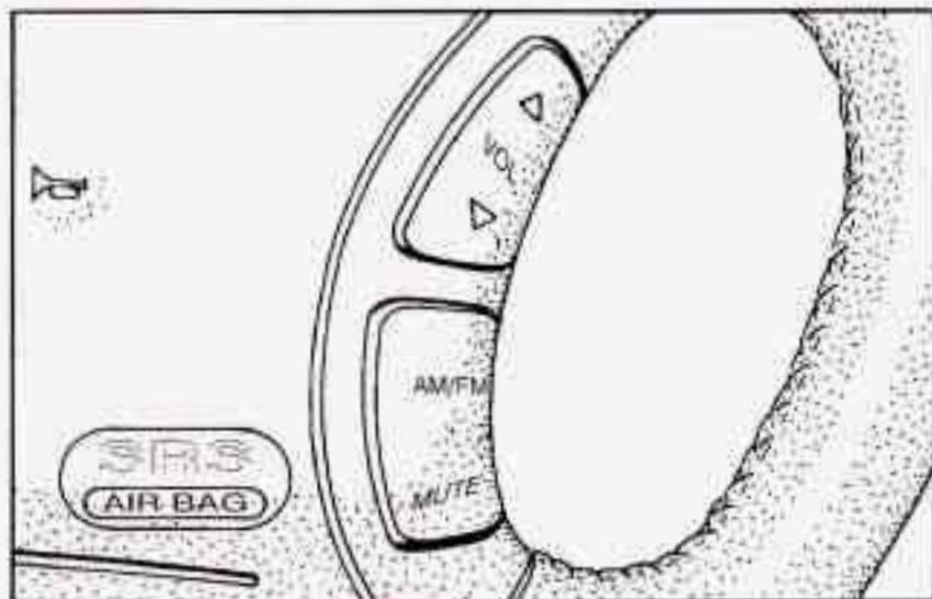
**▲ VOL ▼:** Press the up VOL arrow to increase volume; press the down VOL arrow to decrease volume.
