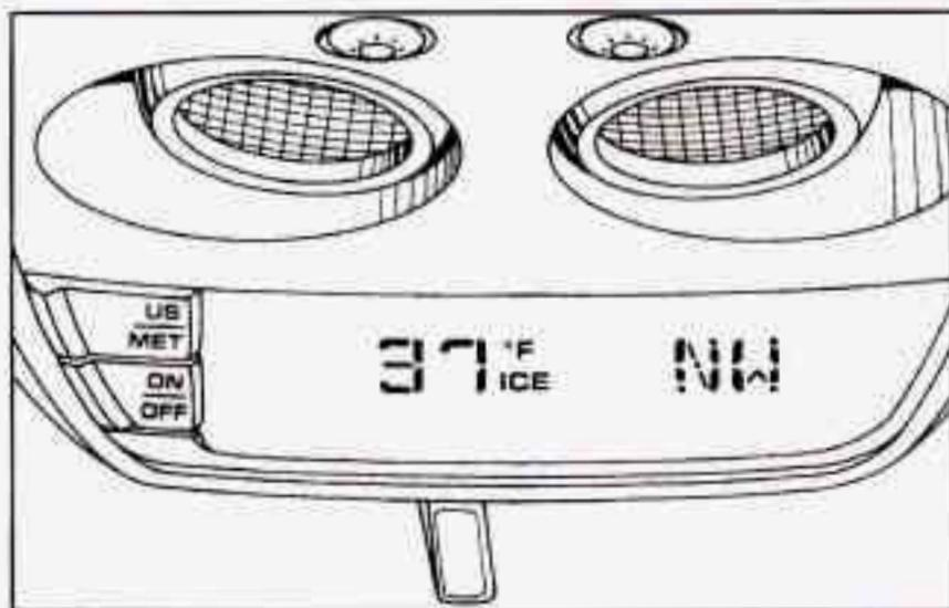
**TEMPERATURE AND COMPASS DISPLAY:** The outside air temperature and the compass are displayed at the front of the overhead console. The control switches are located to the left of the display.
