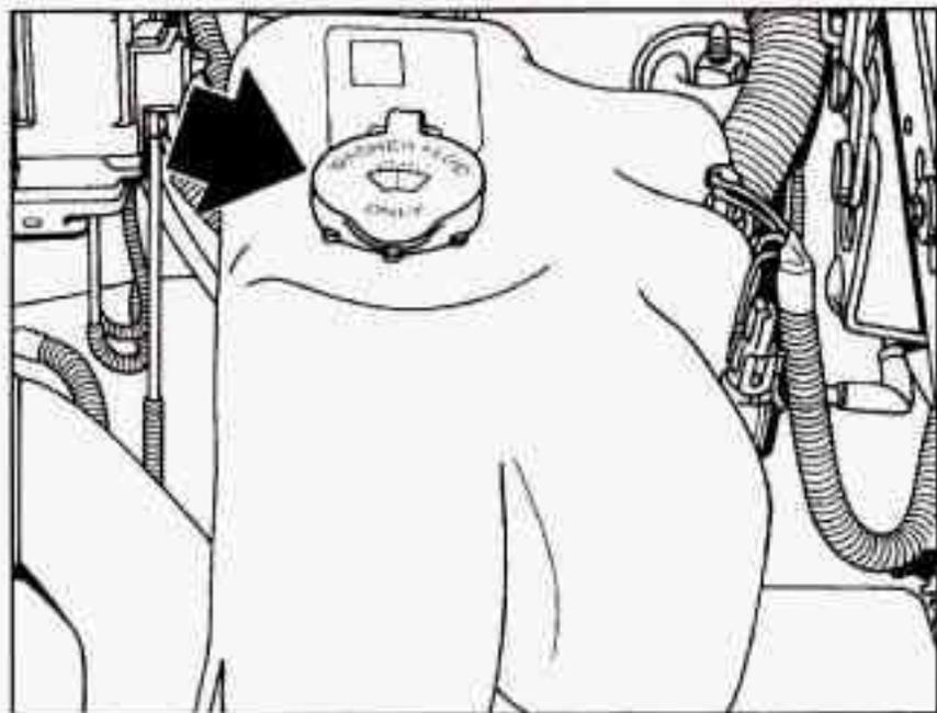
The windshield washer fluid reservoir is located on the driver's side of the vehicle, toward the front of the engine compartment.
