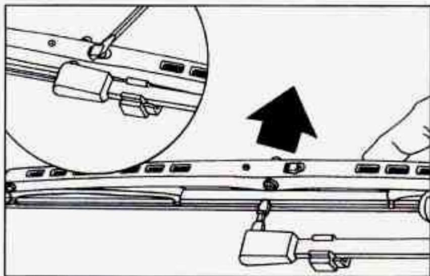
Replacement blades for your vehicle are 24 inches in length. They come in different types and are removed in different ways. Here's how to remove the type with a release clip:
