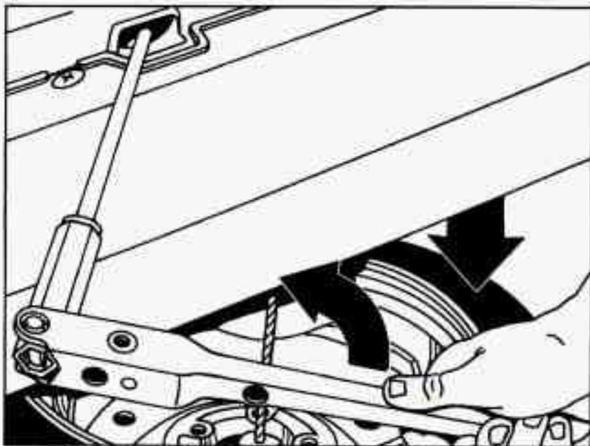
4. The compact spare tire is located under the vehicle, behind the rear bumper. Insert the narrow end of the shaft into the hole above the rear bumper. Then attach the folding wrench to the shaft.
