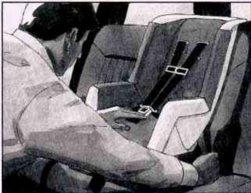
6. To tighten the belt, feed it back into the retractor while you push down on the child restraint.
