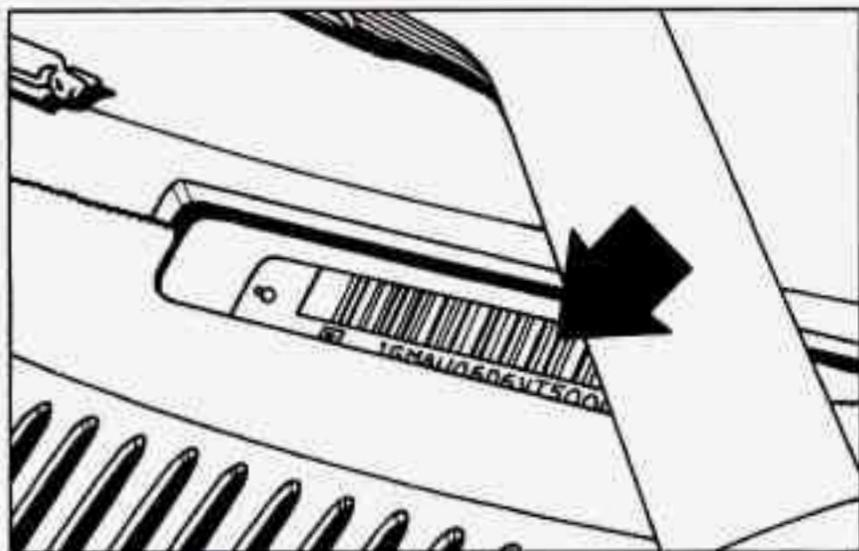
This is the legal identifier for your Oldsmobile. It appears on a plate in the front corner of the instrument panel, on the driver's side. You can see it if you look through the windshield from outside your vehicle. The VIN also appears on the Vehicle Certification and Service Parts labels and the certificates of title and registration.
