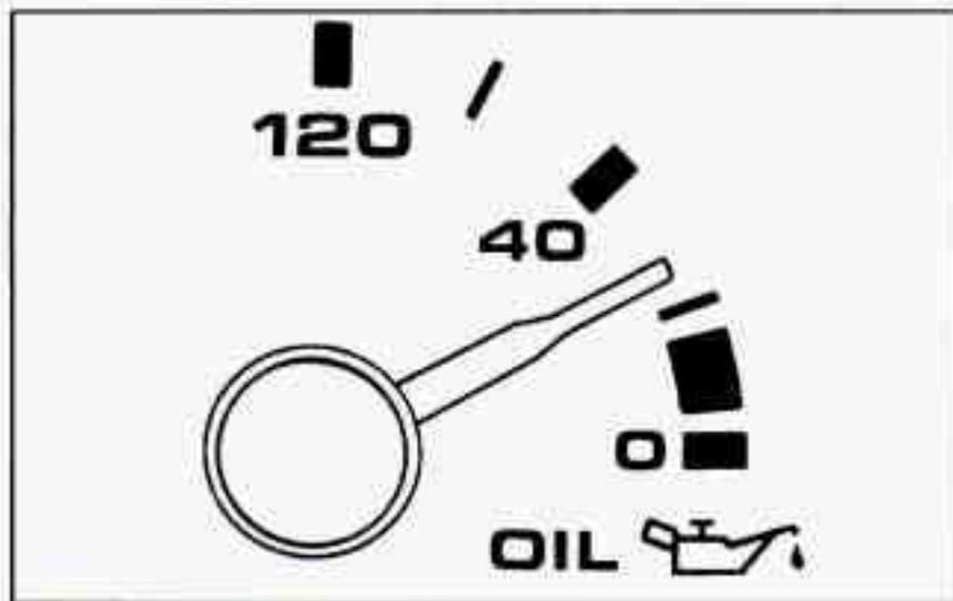
Your oil pressure gage shows the oil pressure in psi (pounds per square inch) when the engine is running. Oil pressure may vary with engine speed, outside temperature and oil viscosity. In fact, while the engine is warming up, the oil pressure will be higher than at the normal operating temperature. Readings above the red warning zone indicate the normal operating range.
