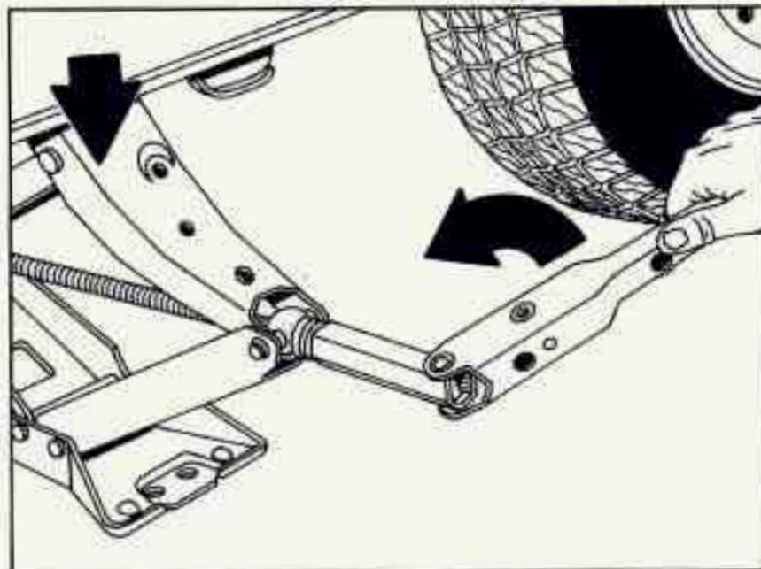
15. Lower the vehicle by attaching the folding wrench to the jack and rotating the wrench counterclockwise. Lower the jack completely.
