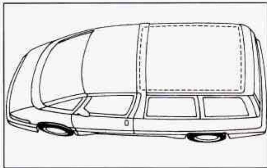
Your state-of-the-art integrated roof antenna is not visible. It is located between the roof and headliner of your vehicle, covering the entire roof area from the rear edge of the front doors to the liftgate.
