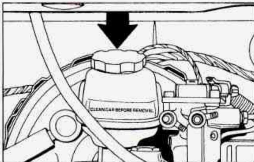
There are only two reasons why the brake fluid level in your master cylinder might go down. The first is that the brake fluid goes down to an acceptable level during normal brake lining wear. When new linings are put in, the fluid level goes back up. The other reason is that fluid is leaking out of the brake system. If it is, you
