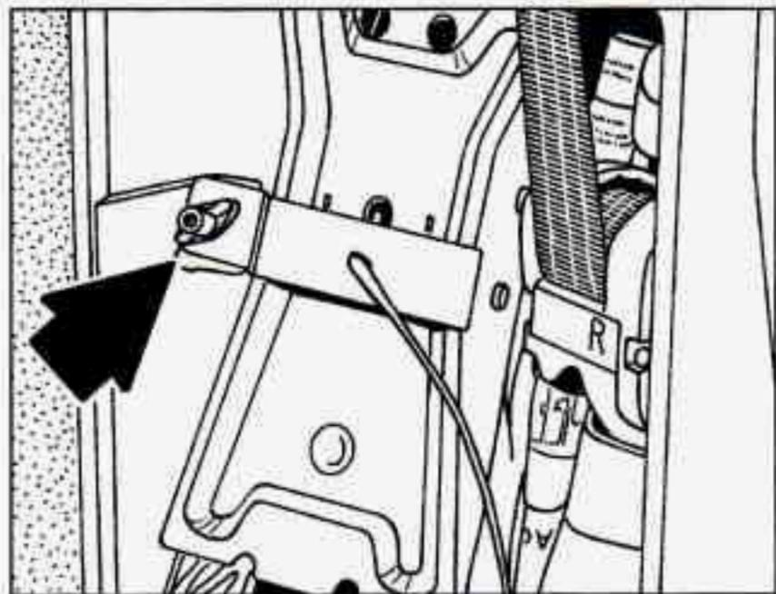
2. Remove the jack and jacking tools by loosening the wing nut and retainer bar.
