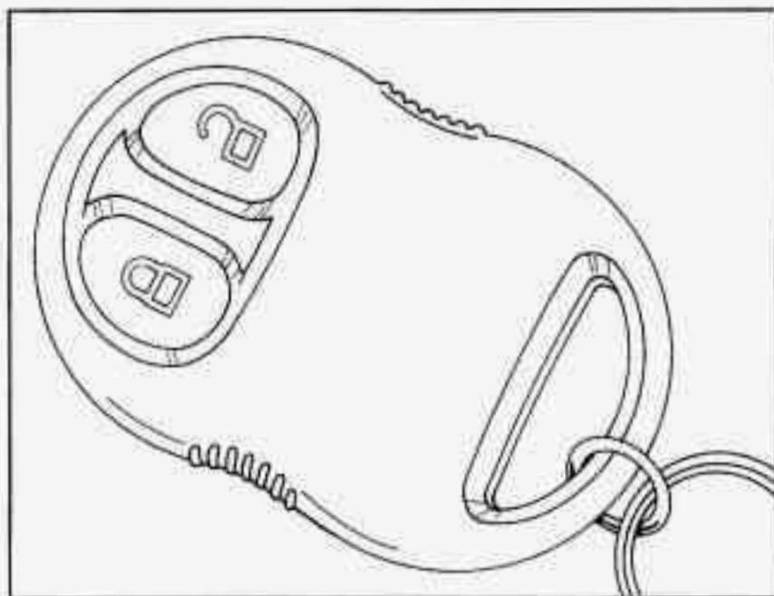
If your Oldsmobile has this option, you can lock and unlock your doors and liftgate from up to 30 feet (9 m) away using the key chain transmitter supplied with your vehicle.
