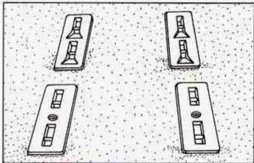
Each rear seat location has two sets of floor pins. Seats equipped with the built-in child restraint option must be secured in the rear set of floor pins. Seats that don't have the built-in child restraint option can be secured in either set of floor pins. Move the position of these seats up or back to provide a little more room behind or in front of a seat.
