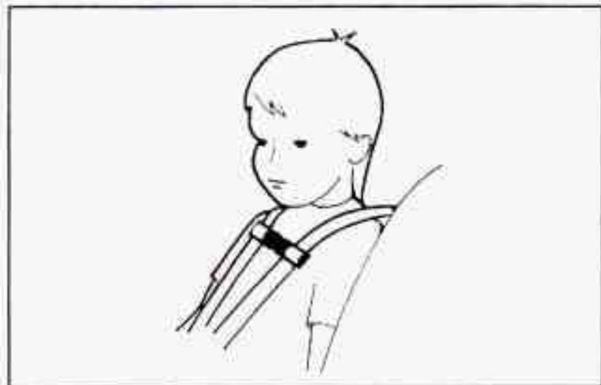
6. Fasten the two halves of the shoulder harness clip together and put it two to three inches (5-8 cm) below the child's chin. The purpose of the clip is to keep the shoulder harness straps positioned correctly on the shoulders.
