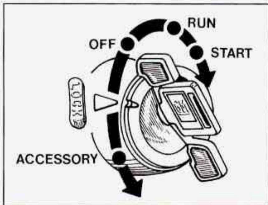
With the ignition key in the ignition switch, you can turn the switch to five positions.
