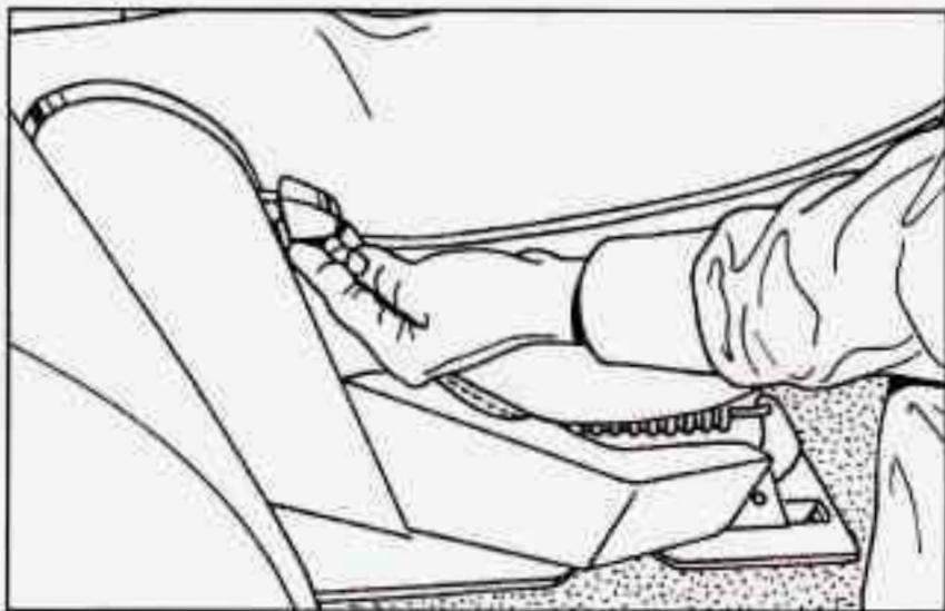
1. With the entire seat tilted forward, place the front hooks of the seat latch onto the front floor pins.
