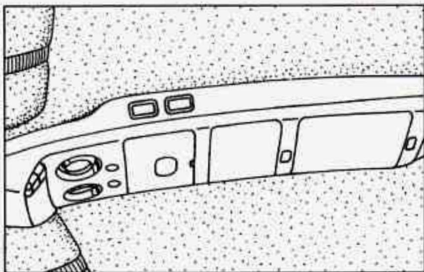
The front overhead console has reading lamps, two switches for the optional power sliding door, storage compartments (including one for your garage door opener and one for sunglasses), a compass and an outside temperature display. The features of the overhead console are explained on the following pages.
