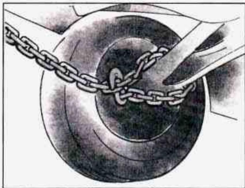
2. Attach a separate safety chain around the outboard end of each control arm.
