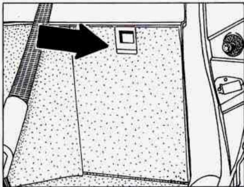
1. Open the jack storage compartment by sliding the latch down and removing the compartment cover.
