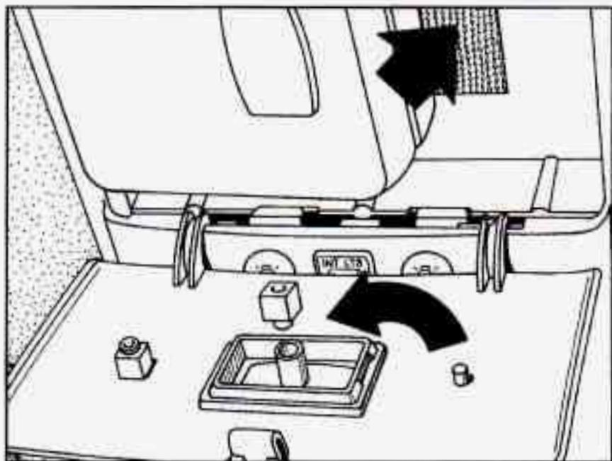
3. To make sure the button on your garage door opener is centered above the button on the compartment door, use the intersecting lines on the Velcro<sup>®</sup> inside the compartment as a guide. Center the control button of your garage door opener over the point where the lines intersect, and press the opener firmly into place. Make sure the button is facing down.
