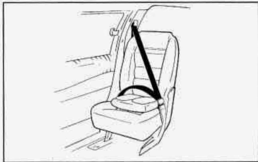
The booster seat can be used by children over 40 pounds (18 kg) or whose shoulders are above the shoulder belt anchorages of the 5-point child restraint harness. The vehicle lap-shoulder belt is used instead of the 5-point harness system. If a child's shoulders are higher than the shoulder belt anchorages while using the 5-point harness, the spine could be injured in a collision.
