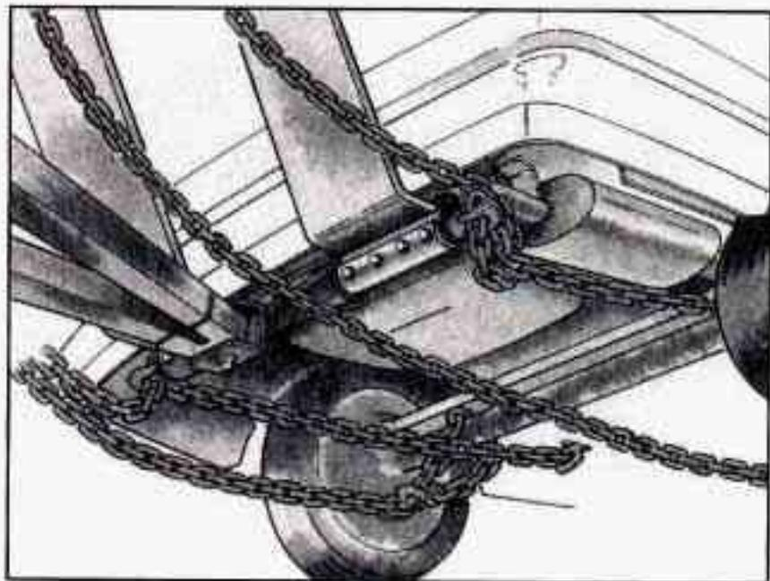
2. Position the lower sling crossbar directly under the rear bumper. No 4x4 wood beam is needed.
