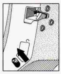
Move the lever on the door all the way up to the ENGAGED position.
