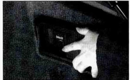
Close the door by sliding it all the way to the left. If the door is left partially open the changer will not operate and an error will occur. When the door is closed, the changer will begin checking for discs in the magazine. This will continue for up to 1 1/2 minutes depending on the number of discs loaded.
