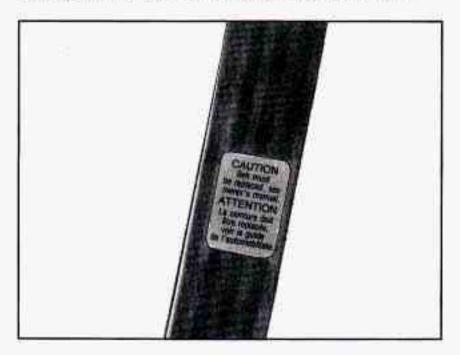
If you ever see a label on the driver's or the right front passenger's safety belt that says to replace the belt, be sure to do so. Then the new belt will be there to help protect you in a collision. You would see this label on the belt near the latch plate.
