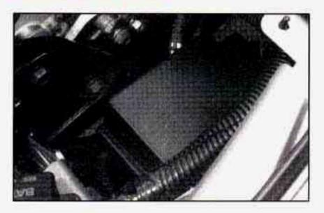
It's easy to check the fuses in this underhood relay center. There are two locking arms on either side of the base of the cover. Reach down and unsnap each one by pulling the cover toward you, then pushing it away while pulling up. Remove the cover. The inside of the cover has a chart that explains the features and controls governed by each fuse and relay.
