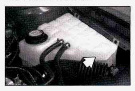
If the message LOW ENGINE COOLANT is displayed on your message center, it means you're low on engine coolant.
