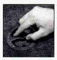
Turn the center retainer bolt on the spare tire cover counterclockwise to remove it, then lift and remove the tire cover.
