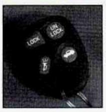
You can lock and unlock your doors or unlock your trunk from up to 30 feet (9 m) away using the key chain transmitter supplied with your vehicle.
