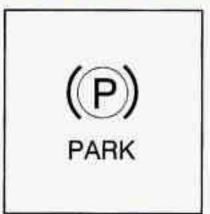
Vehicles with hydraulic brakes have a parking brake indicator light. When the ignition is on, this light will come on when you set your parking brake. The light will stay on if your parking brake doesn't release fully. If you try to drive off with the parking brake set, a chime will also come on until you release the parking brake.
