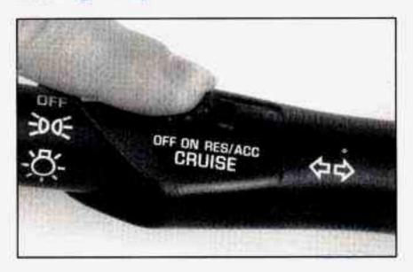
Setting the cruise control at a desired speed and then applying the brake will end the cruise control function.
