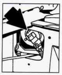
Unclip the bulb assembly from the wiring harness and replace the bulb assembly.
