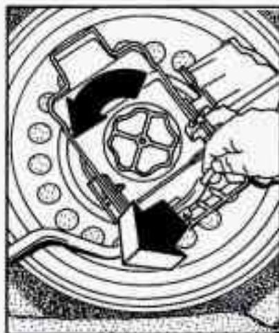
Turn the spare tire retainer bolt counterclockwise and remove the retainer assembly.
