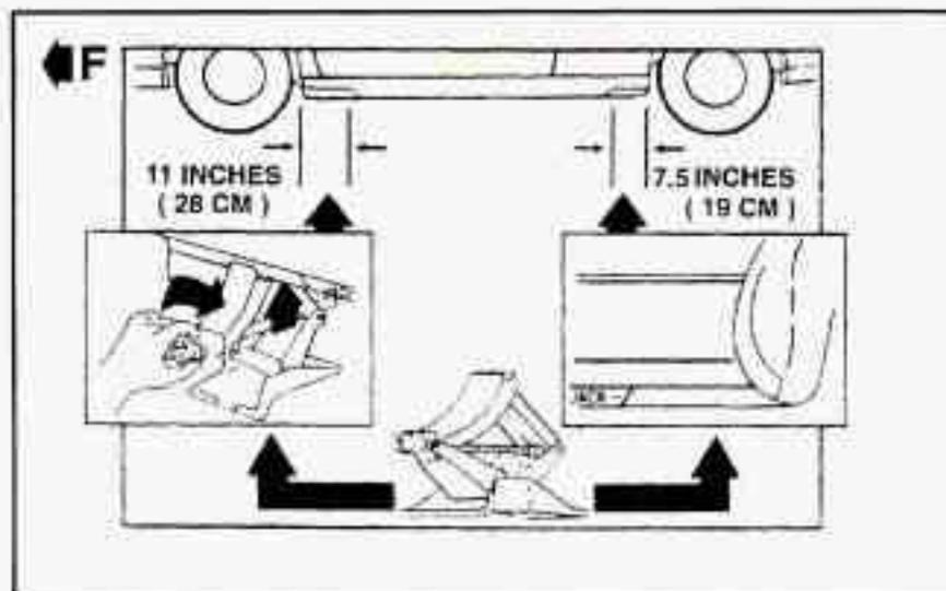
4. Near each wheel well is a notch in the frame to position the jack head. You'll find the word **JACK** and an arrow stamped into the plastic near each notch. Position the jack under the vehicle and raise the jack head until it fits firmly against the sheet metal next to the word **JACK**. Do not raise the vehicle yet. Put the compact spare near you.
