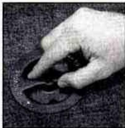
Turn the center retainer bolt on the spare tire cover counterclockwise to remove it, then lift and remove the tire cover.
