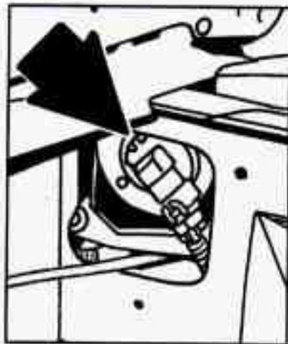
6. Unclip the bulb assembly from the wiring harness and replace the bulb assembly.
