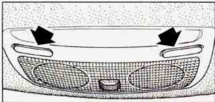
These lamps and the interior courtesy lamps will come on when you open a door. They will turn off when you turn on the ignition. If the door is left open, they will turn off after about 10 minutes.
