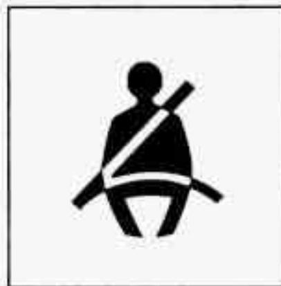
The safety belt light will also come on and stay on for about 70 seconds. If the driver's belt is already buckled, neither the chime nor the light will come on.
