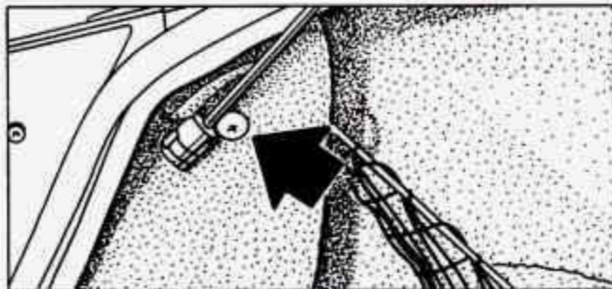
1. In the trunk, remove the convenience net from the hooks. Next remove the plastic screws holding the carpeting in place and pull back the carpeting.
