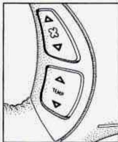
Some heating and cooling controls can be adjusted at the steering wheel. Other touch controls also operate some audio controls. See "Steering Wheel Controls for Audio System" later in this section.
