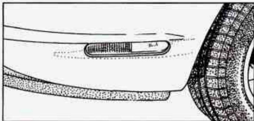
The cornering lamps are designed to come on when you signal a turn. This will provide more light for cornering at night.
