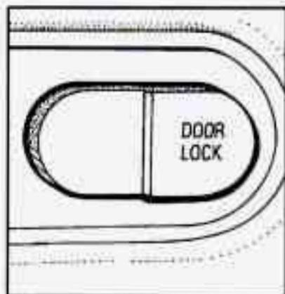
With power door locks, you can lock or unlock all doors of your vehicle from the driver or front passenger door lock switch.
