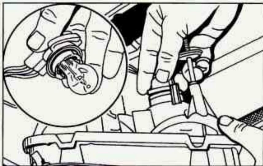
5. Pull out the lamp to reach the bulb. Pull out the bulb. To replace, push the bulb back in.
