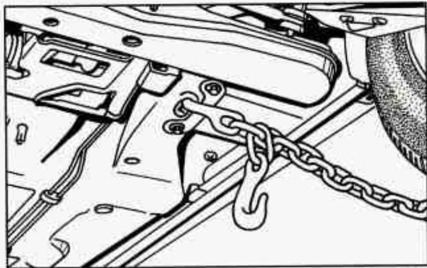
Attach T-hook chains to the T-hook slots in the floor pan support rails just ahead of the rear wheels on both sides.
