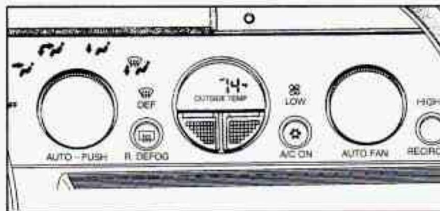
Your Aurora is equipped with a Dual Zone Automatic Electronic Climate Control System. You can use the automatic setting or override the automatic setting by using the manual controls. Your vehicle also has the flow-through ventilation system described later in this section.
