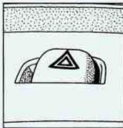
Press down on the button located on top of the steering column, then release it to turn on the hazard warning flashers.
