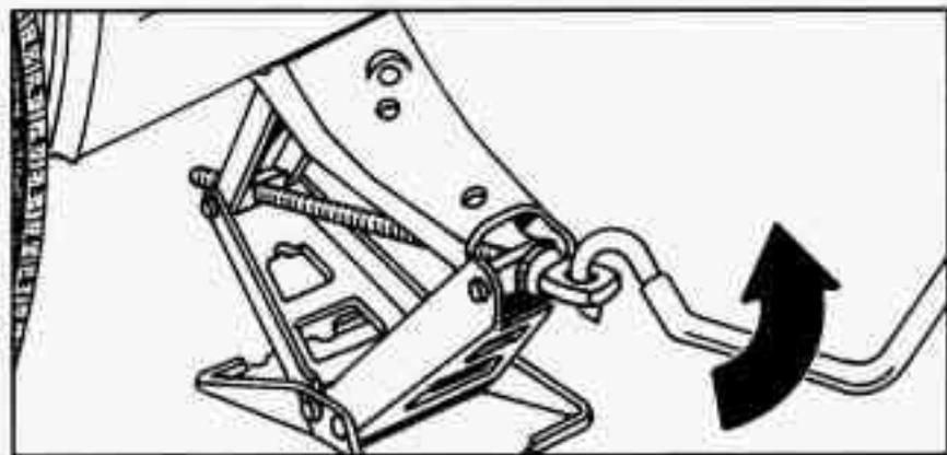
10. Lower the vehicle by rotating the wheel wrench counterclockwise on the jack. Lower the jack completely.
