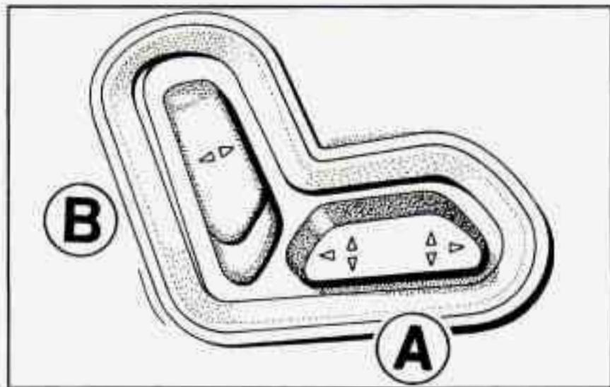
**Horizontal Control (A):** Raise the front of the seat by raising the forward edge of the button. Lower the front of the seat by lowering the forward edge of the button. Move the seat forward by moving the whole button toward the front of the vehicle.
