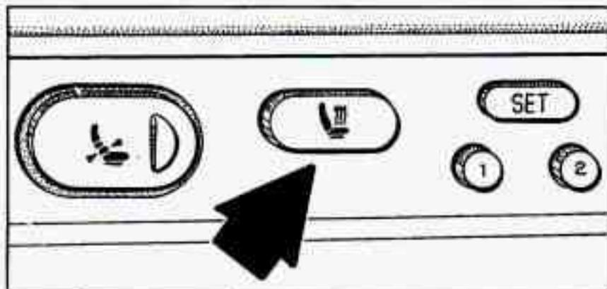
This feature will quickly heat the lower cushions and lower back of the driver and front passenger seats for added comfort.
