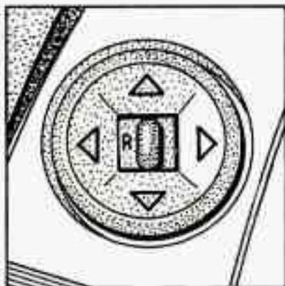
The controls on the far left of the instrument panel control both outside rearview mirrors. Move the center switch to the left to select the driver's side rearview mirror, or to the right to select the passenger's side rearview mirror.
