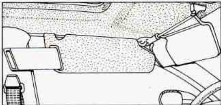
To block out glare, you can swing down the visors. You can also remove them from the center mount and swing them to the side, while the auxiliary visor remains to block glare from the front.
