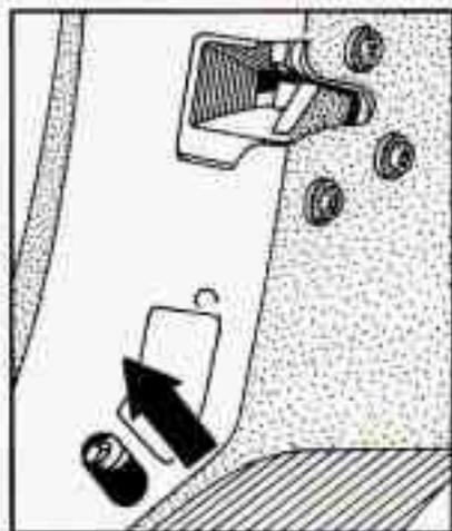
2. Move the lever on the door all the way up to the ENGAGED position.
