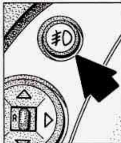
To turn on the fog lamps, first turn on the parking lamps or headlamps. Then press the fog lamp switch. A light will glow on the switch when the switch is on. To turn off the fog lamps, press it again.
