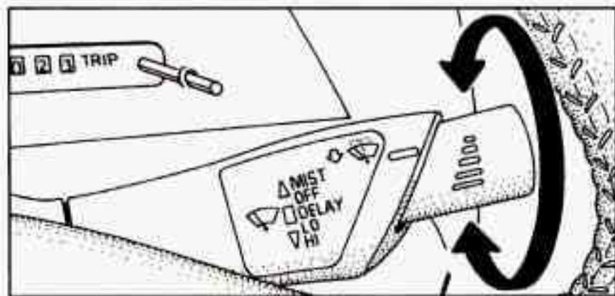
You can set the wiper speed for a long or short delay between wiper cycles. This can be very useful in light rain or snow. Push the lever down to the first detent, DELAY. Turn the band closer to the short lines for fewer wiper passes per minute. As you turn the band toward the long lines, the wiper cycles per minute will increase.
