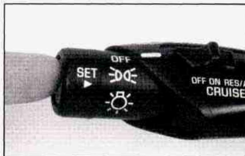
3. Push in the button at the end of the lever and release it. The CRUISE light on the instrument panel will come on.
