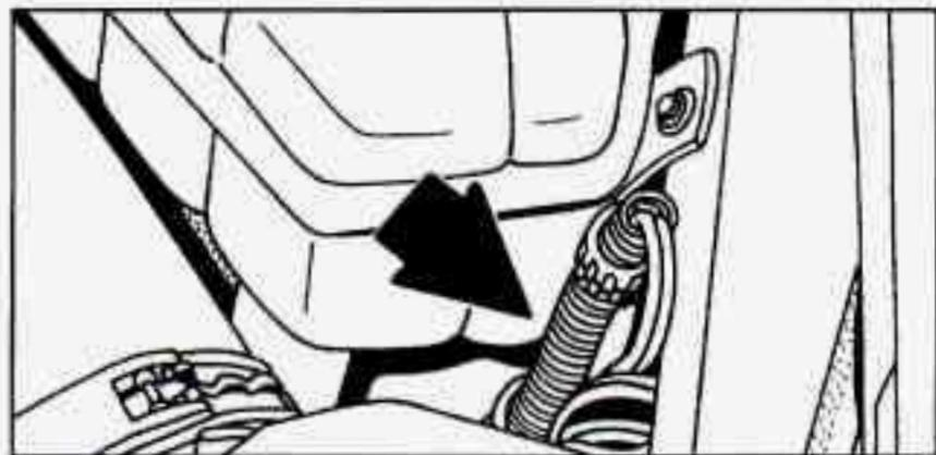
In very cold weather, 0°F (-18°C) or colder, the engine coolant heater can help. You'll get easier starting and better fuel economy during engine warm-up. Usually, the coolant heater should be plugged in a minimum of four hours prior to starting your vehicle.
