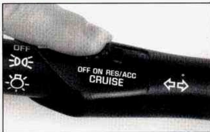
Setting the cruise control at a desired speed and then applying the brake will end the cruise control function.
