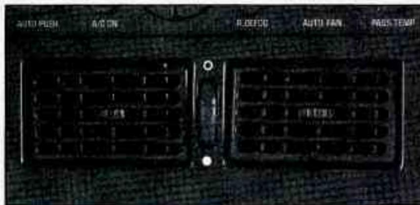
The direction of the air can be controlled by adjusting or closing the outlets in the instrument panel. Rotate the control between the front outlets upward to open the outlets and downward to close the outlets. Adjust the direction of airflow from side to side with the controls in each outlet.
