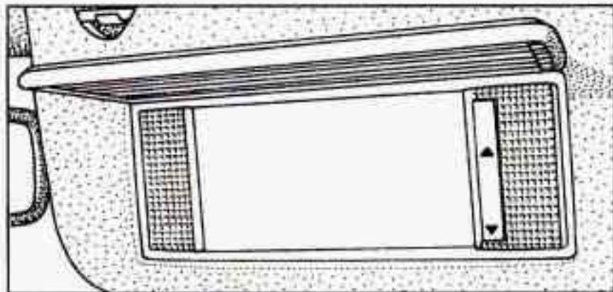
When you open the cover to the driver or passenger side visor vanity mirror, the lamps will come on. You can adjust the brightness of the lamps with the switch by sliding the lever up or down.
