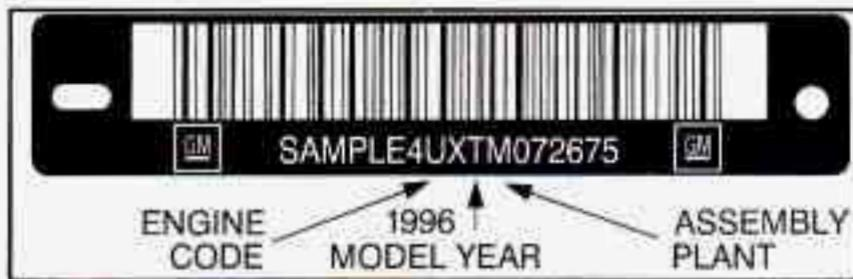
This is the legal identifier for your Aurora. It appears on a plate in the front corner of the instrument panel, on the driver's side. You can see it if you look through the windshield from outside your vehicle. The VIN also appears on the Vehicle Certification and Service Parts labels and the certificates of title and registration.
