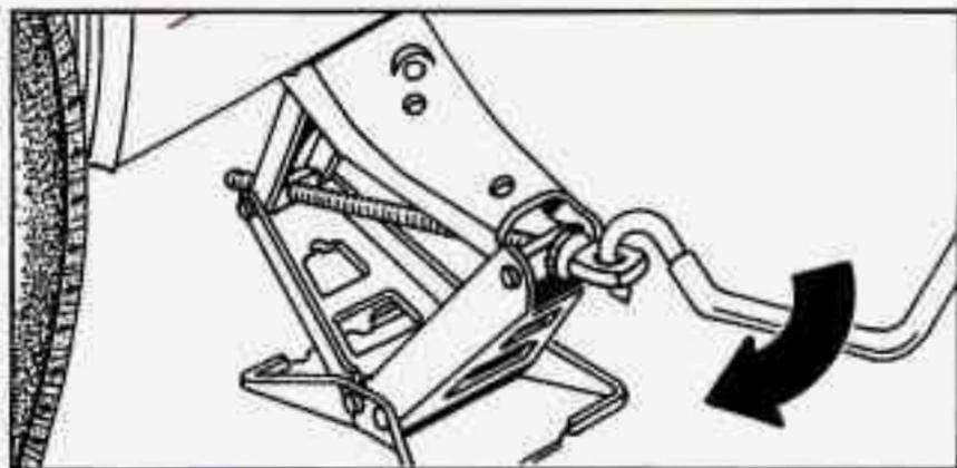
5. Raise the vehicle by rotating the wheel wrench clockwise in the jack. Raise the vehicle far enough off the ground so there's enough room for the spare tire to fit.
