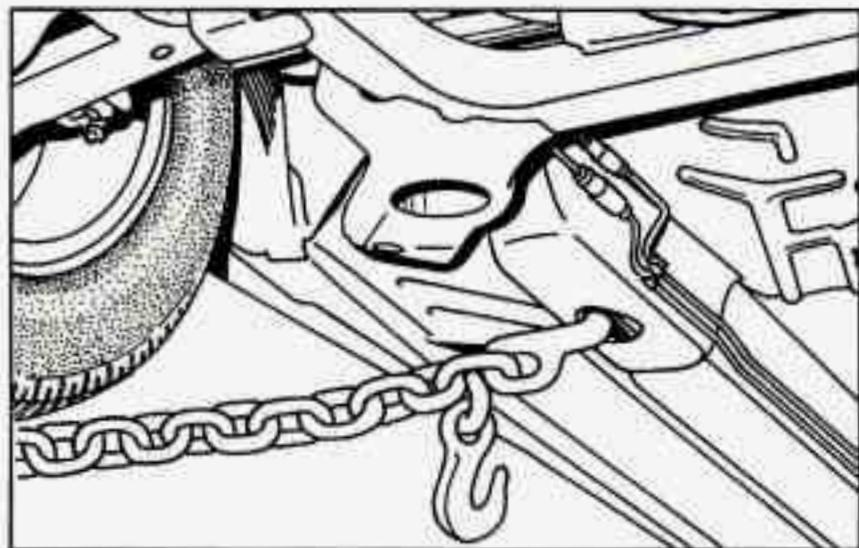
Attach T-hook chains on both sides, in the slotted holes in the bottom of the body rail, behind the front wheels and cradle.
