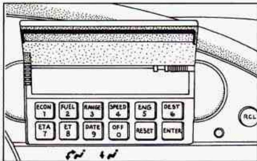
The Driver Information Center (DIC) displays information in either English or metric. When the system is on or off, hold the OFF button down for five seconds to change the display between English and metric. This will also change the digital screen for the climate control system between English and metric.
