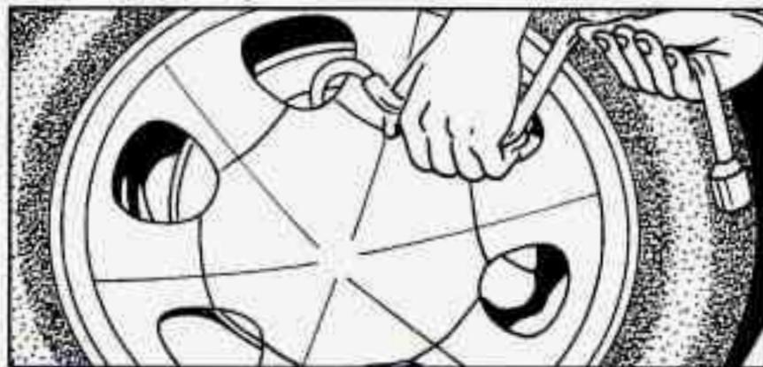
Insert the hooked end of the wheel wrench in one of the two small notches in the center cover and pry the cover off. Do not drop the cover or lay it face down, as it could be scratched or damaged.
