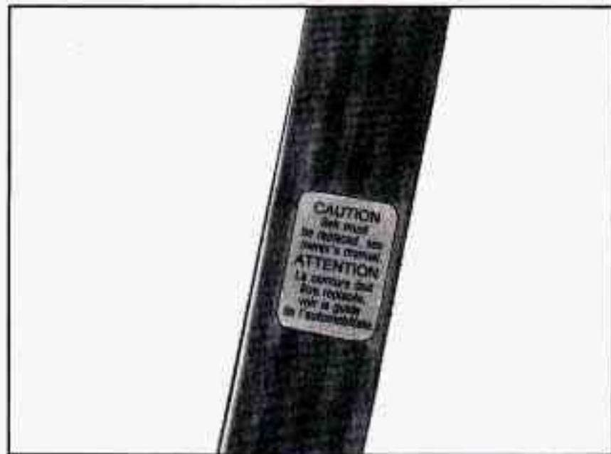
If you ever see a label on the driver's or the right front passenger's safety belt that says to replace the belt, be sure to do so. Then the new belt will be there to help protect you in a collision. You would see this label on the belt near the latch plate.
