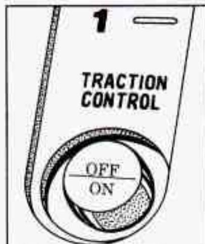
To turn the system off, press the **TRACTION CONTROL** button on the center console.
