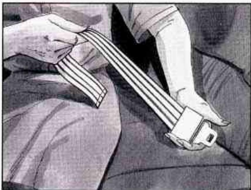
1. Make the belt as long as possible by tilting the latch plate and pulling it along the belt.
