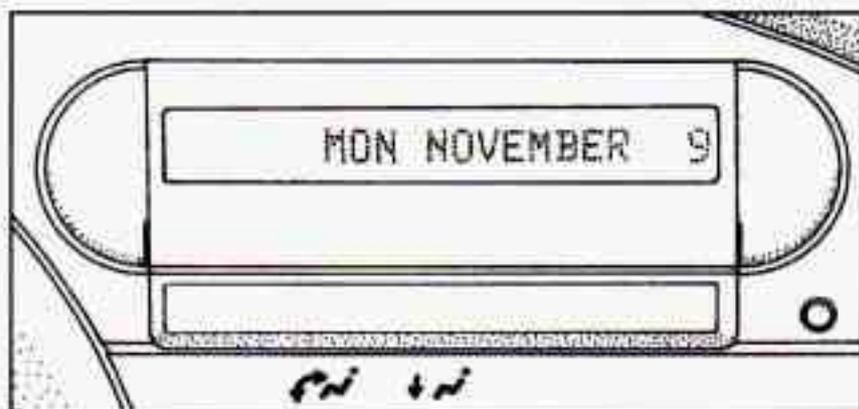
You will need to open the cover to access the control buttons. To open the cover, push the button located to the right of the cover.
