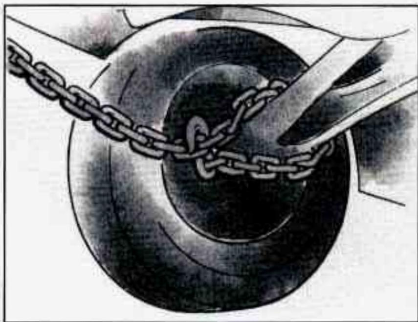
Attach a separate safety chain around the outboard end of each lower control arm.
