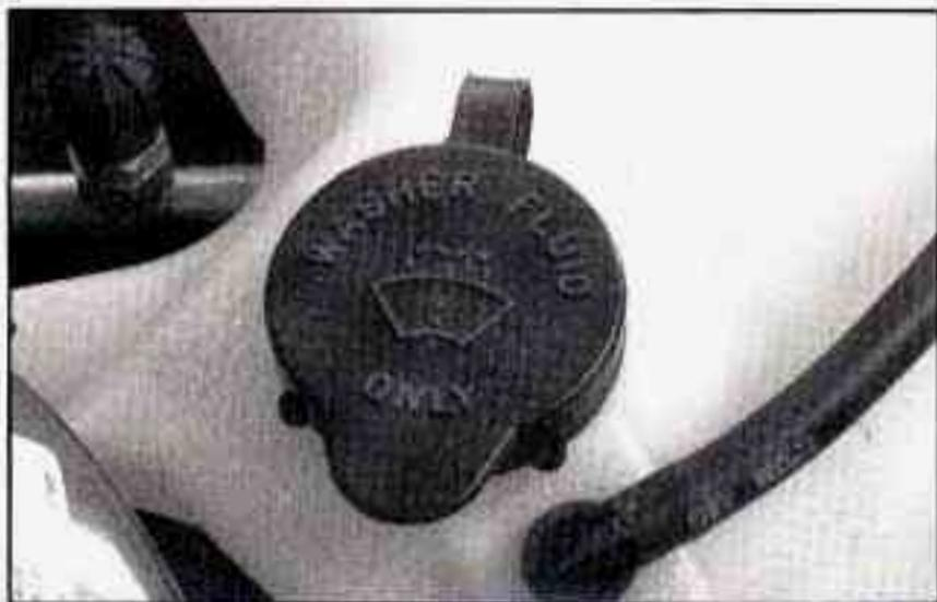
There are two windshield washer fluid tanks. The upper tank (shown above) will empty first. When the lower tank contains 0.5 quarts (0.5 liters) or less, the message LOW WASHER FLUID will be displayed on the Driver Information Center.
