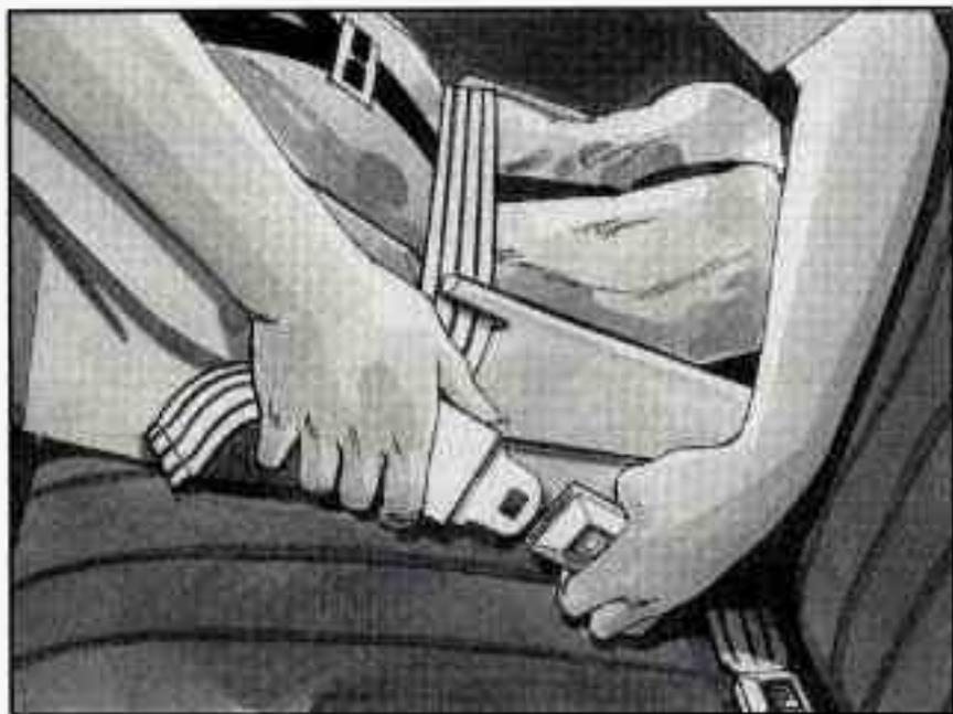
4. Run the vehicle's safety belt through or around the restraint. The child restraint instructions will show you how.
