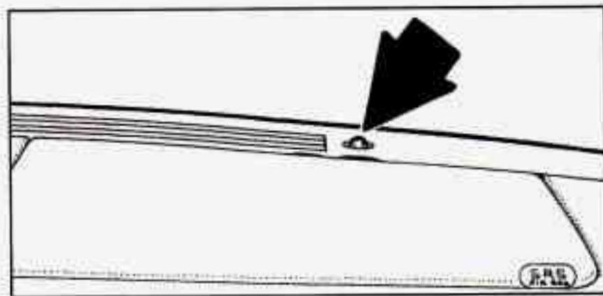
Your automatic electronic climate control system has two sun sensors located on the top of the instrument panel that detect direct sunlight. To keep you and your passengers comfortable, the system may supply cooler air to the side towards the sun. Be careful not to put anything over these sun sensors. The automatic electronic climate control system may not operate correctly if these sensors are covered.
