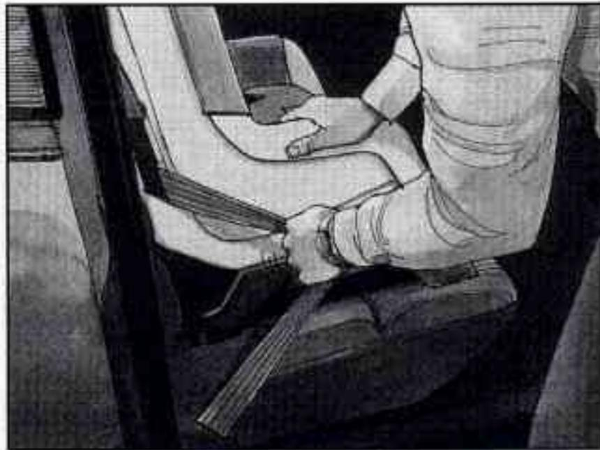
6. Pull the rest of the lap belt all the way out of the retractor to set the lock.
