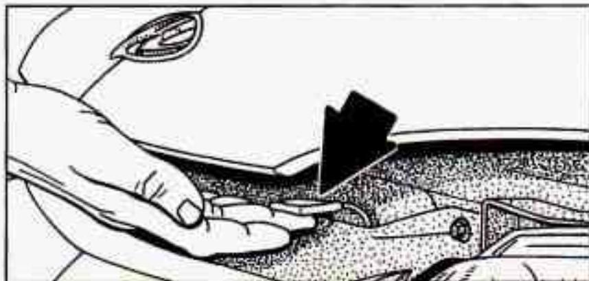
Then go to the front of the vehicle and pull up on the underhood release.
