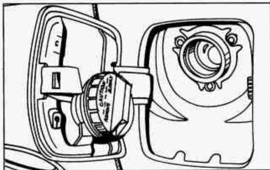
While refueling, hang the cap inside the fuel door. Twist it clockwise to secure it, if necessary.
