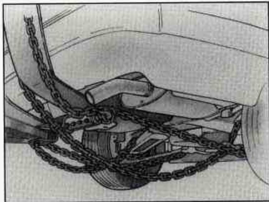
Position the lower sling crossbar just ahead of the front edge of the rear bumper.
