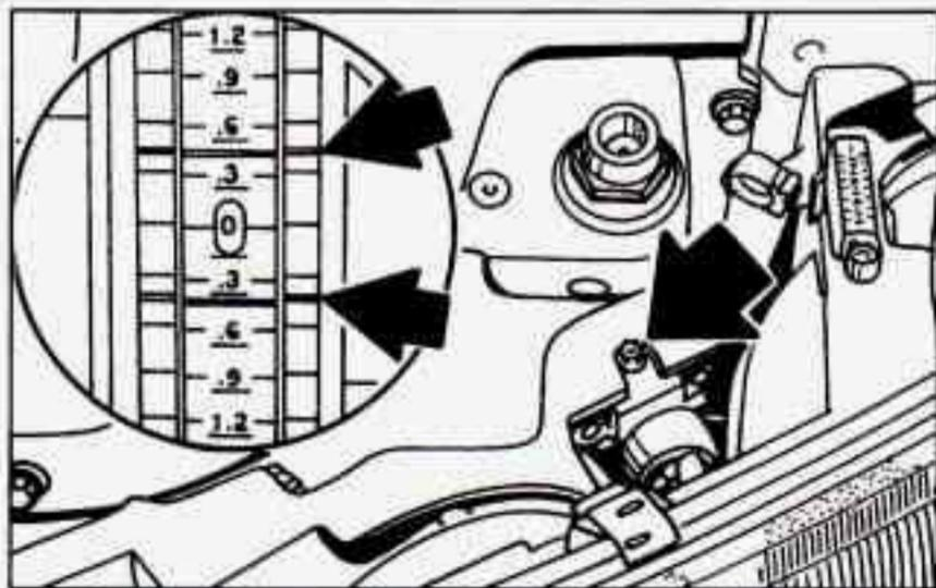
1. Check the vertical aim for each headlamp and adjust it as necessary. Turn the vertical aiming screw until the bubble in the level is centered at 0 (zero).
