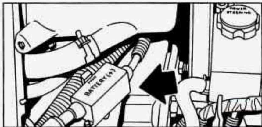
4. Open the hoods and locate the other vehicle's battery and the Aurora's remote positive (+) jump starting terminal in the box on the passenger side of the engine compartment. (Your Aurora's battery isn't under the hood.)
