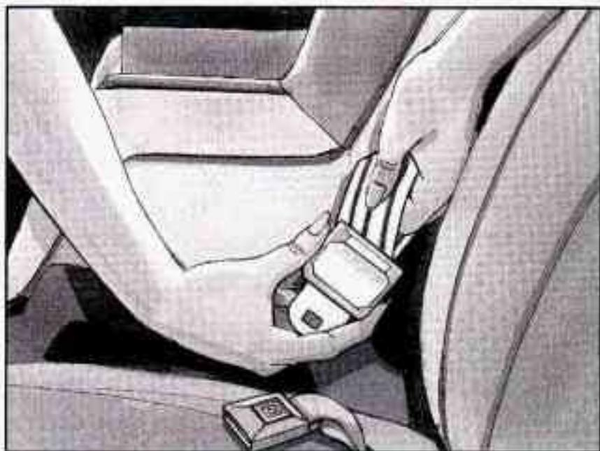
4. Tilt the latch plate to adjust the belt if needed.
