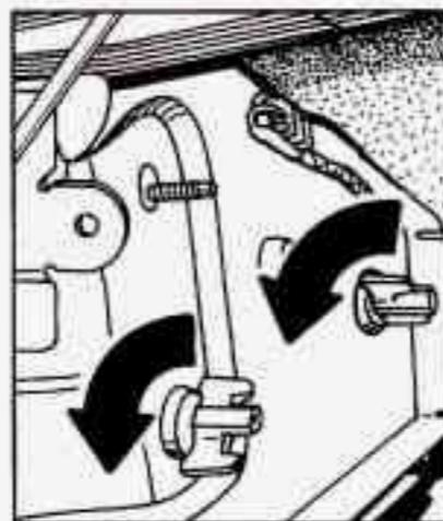
3. Remove the two wing nuts now exposed.
