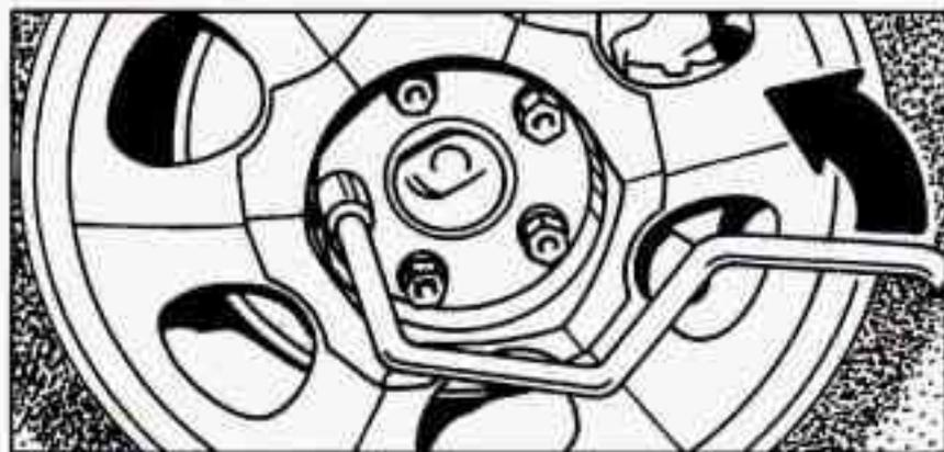
1. Use the wheel wrench to loosen the wheel nuts, but don't remove them.
