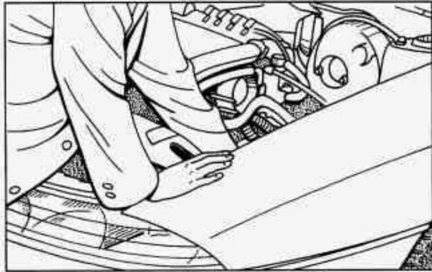
3. Release tension of the wing screw clamp on the air intake duct where it attaches to the air cleaner cover near the top of the engine. Turn the wing screw counterclockwise, then detach the hose from the air cleaner cover.
