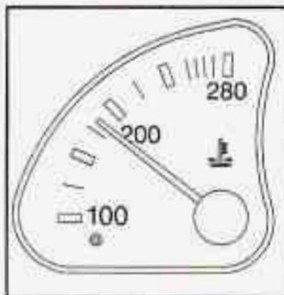
This gage shows the engine coolant temperature.
