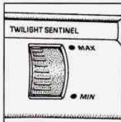
Twilight sentinel turns your headlamps, taillamps and parking lamps on and off by sensing how dark it is outside.
