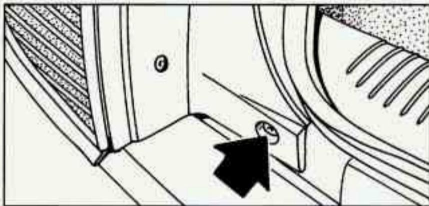
4. Remove the taillamp filler screw located to the side of the taillamp filler panel.
