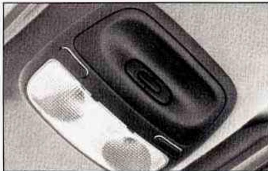
This transmitter allows you to consolidate the functions of up to three individual hand-held transmitters. It will operate garage doors and gates, or with the accessory package, other devices controlled by radio frequency such as home/office lighting systems and security systems.
