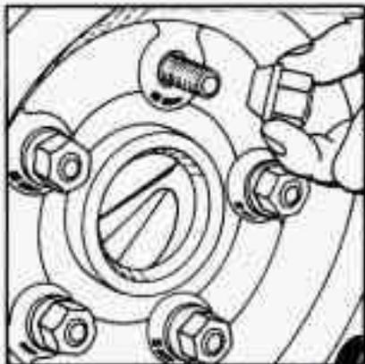
9. Replace the wheel nuts with the rounded end of the nuts toward the wheel. Tighten each nut by hand until the wheel is held against the hub.
