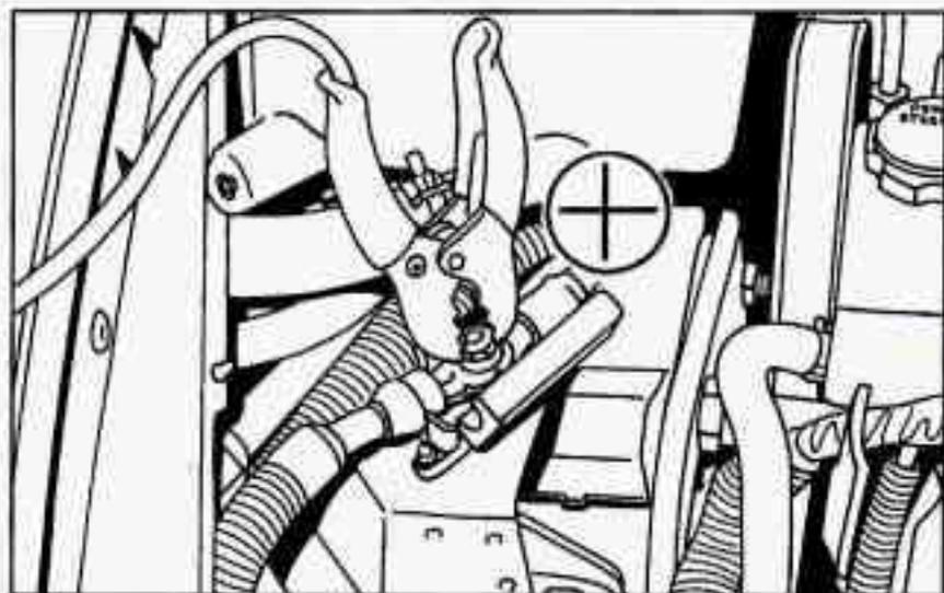
7. Connect the red positive (+) cable to the remote positive (+) terminal of the vehicle with the dead battery.
