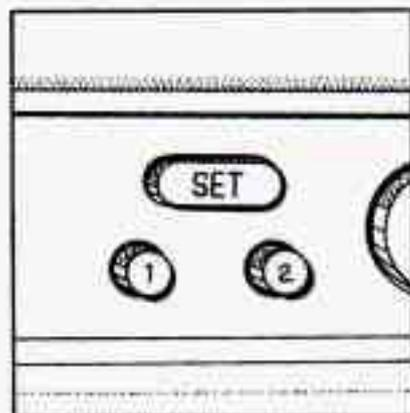
The memory function controls both the driver's seat and outside mirror positions. First, position the seat and mirrors where you want them. Next, press the SET button. You will hear one beep. Within five seconds, press either the 1 or 2 button. You will hear two beeps.
