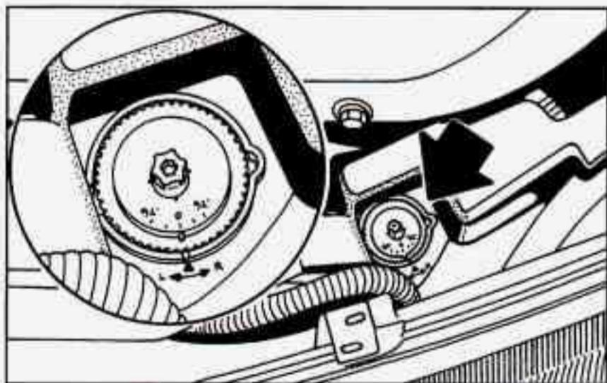
2. Now adjust the horizontal aim. Check the horizontal aim for each headlamp and adjust it as necessary. Turn the horizontal aiming screw until the pointer is lined up with the 0 (zero).
