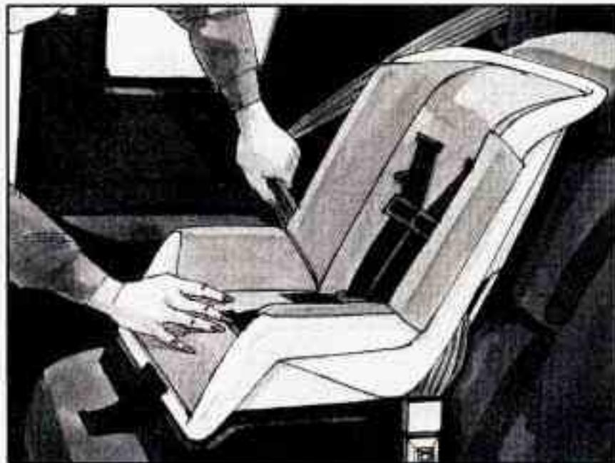
6. To tighten the belt, pull up on the shoulder belt while you push down on the child restraint.
