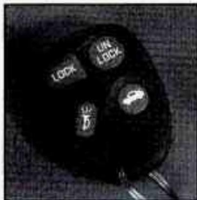
You can lock and unlock your doors or unlock your trunk from up to 30 feet (9 m) away using the key chain transmitter supplied with your vehicle.
