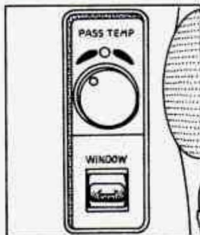
With this feature, the right front seat passenger can control the comfort setting for their own zone. To use this feature, adjust the control on the passenger side armrest to the desired comfort level.
