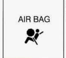
There is an air bag readiness light on the instrument panel, which shows the words AIR BAG.
