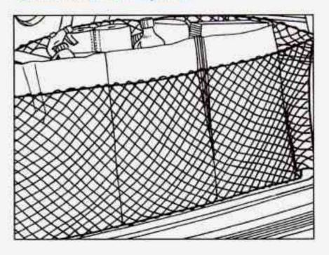
The optional convenience net is designed to help keep small loads, like grocery bags, from falling over during sharp turns or quick stops and starts. Install the convenience net at the rear of your vehicle, just inside the liftgate. Attach the upper loops to the posts on either side of the liftgate opening (the label on the net should be in the upper right-hand corner). Attach the lower loops to the hooks on the floor.
