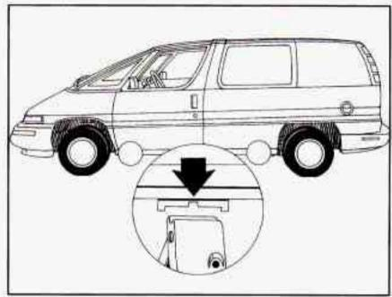
4. Near each wheel, there is a notch in the vehicle's frame. Position the jack and raise the jack head until it fits firmly into the notch in the vehicle's frame (nearest the flat tire). Do not raise the vehicle yet. Put the compact spare tire near you.
