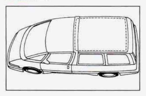
Your state-of-the-art integrated roof antenna is not visible. It is located between the roof and headliner of your vehicle, covering the entire roof area from the rear edge of the front doors to the liftgate.
