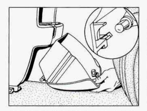
To replace the bin, set the hinge pins (one on each side of the bin, at the bottom) into the hinge guides (one at each side of the console opening, at the base), then close the bin. If the hinge pins are placed properly in the guides, the bin will close easily.
