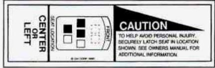
The center position bucket seat is a CENTER OR LEFT type seat. Because it is the only bucket seat with a lap belt, and has a buckle on only one side, there are certain places a CENTER OR LEFT type bucket seat should, and should not, be used. See "Seats" in the Index. If the CENTER OR LEFT bucket seat is used on the left side of the vehicle, the person sitting there should use the lap-shoulder belt. It works the same way as the driver's safety belt. See "Driver Position" in the Index.
