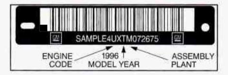
This is the legal identifier for your Oldsmobile. It appears on a plate in the front corner of the instrument panel, on the driver's side. You can see it if you look through the windshield from outside your vehicle. The VIN also appears on the Vehicle Certification and Service Parts labels and the certificates of title and registration.
