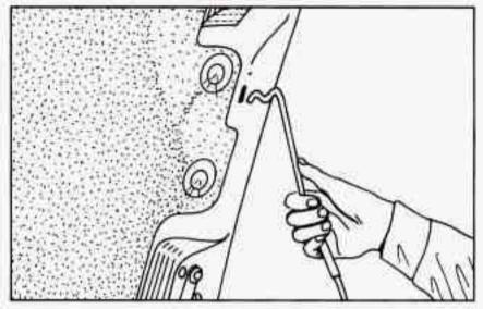
The hood prop rod may be hot due to increased engine temperatures under the hood, so be careful when handling it. Use your hood prop sleeve when handling the hood prop.
