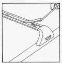
If you wish to attach the luggage tiedowns or other equipment, you will need to remove the outboard bumper strips to access the tapped plates on the crossbar.
