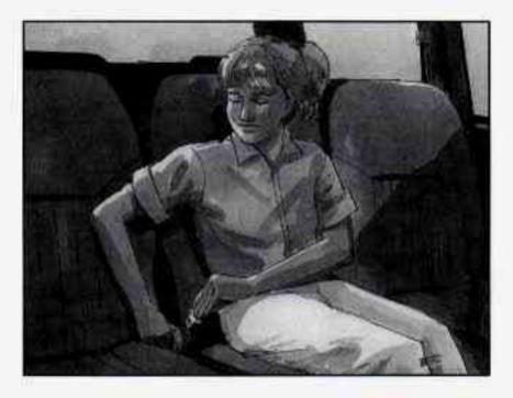
When you sit in the center position bucket seat, you have a lap safety belt which has a retractor.
