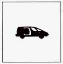
With the optional power sliding door, the sliding door ajar symbol on your instrument panel will come on if your sliding door is not completely closed.
