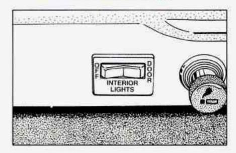
This switch is located to the left of the cigarette lighter in the center instrument panel console. It has two positions, DOOR (on) and OFF, and overrides all interior lamps except the reading lamps.
