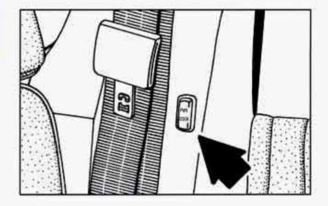
To open or close the sliding door, press and release one of two PWR DOOR switches. There is one mounted on the wall, just in front of the sliding door; the other is the rear-most switch on the side of the overhead console. (If you have the compact overhead console, this switch is located between the reading lamps.)
