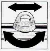
Use the adjustable tie-down loops in the side rails to help secure large loads.
