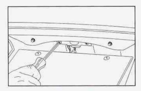
2. Remove the lamp lens from the liftgate.
