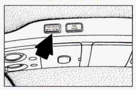
With this option, you can open and close the sliding door with switches inside your vehicle. If you have the optional Remote Lock Control system, you can also operate the sliding door with your remote transmitter. See "Remote Lock Control" in the Index.
