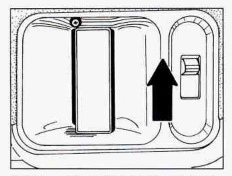
If you want to open the sliding door when the security lock is on, unlock the sliding door from the inside and open the door from the outside.
