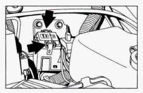
You'll find this fuse under the hood in the ABS junction block, located next to the remote positive jump starting terminal.
