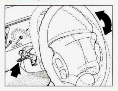
A tilt steering wheel allows you to adjust the steering wheel before you drive. You can also raise it to the highest level to give your legs more room when you exit and enter the vehicle.
