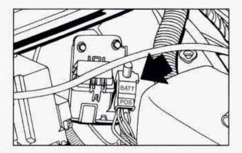
Your Oldsmobile has a remote positive (+) jump starting terminal. The terminal is in the red box on the same side of the engine compartment as your battery. You should always use the remote positive (+) terminal instead of the positive (+) terminal on your battery.
