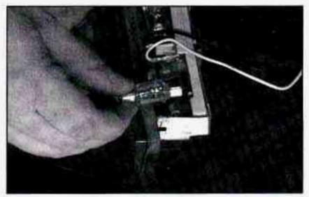
Reinstall the lamp assembly into the liftgate and secure with the screws.
