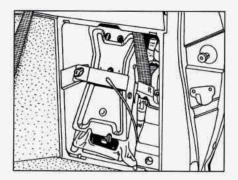
Replace all jacking tools as they were stored in the storage compartment and replace the compartment cover. Be sure to also store the nylon nut caps.
