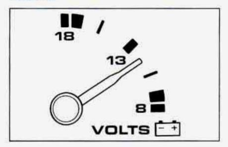
Your charging system gage will show the rate of charge when the engine is running.
