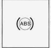
With the anti-lock brake system, this light will come on when you start your engine and it will stay on for three seconds. That's normal.
