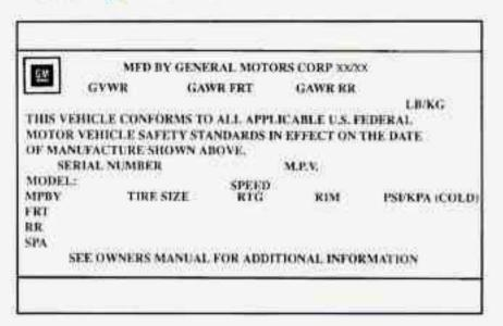
The Certification/Tire label is found on the rear edge of the driver's door. The label shows the size of your original tires and the inflation pressures needed to obtain the gross weight capacity of your vehicle. This is called the GVWR (Gross Vehicle Weight Rating). The GVWR includes the weight of the vehicle, all occupants, fuel and cargo.
