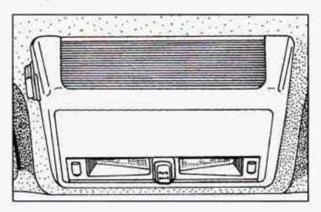
The overhead console includes two reading lamps and a storage compartment.
