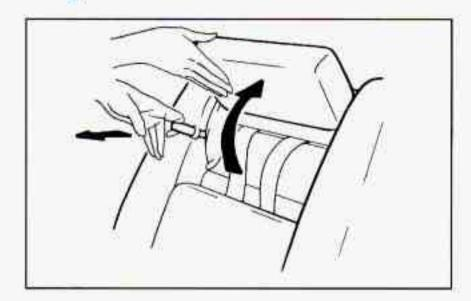
Pull the child head restraint release strap and raise the head restraint until you hear the latch click.
