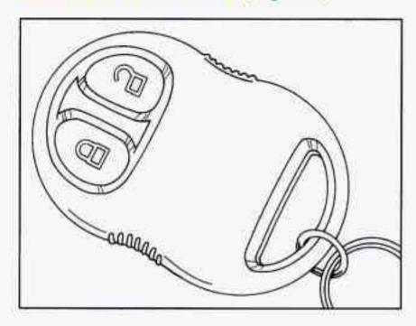
If your Oldsmobile has this option, you can lock and unlock your doors and liftgate from up to 30 feet (9 m) away using the key chain transmitter supplied with your vehicle. Your Remote Lock Control operates on a radio frequency subject to Federal Communications Commission (FCC) Rules.
