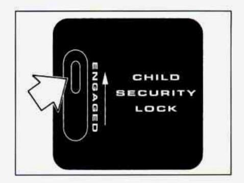
To use the security lock, move the security lock lever all the way up and close the door.
