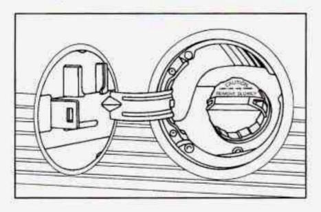
The cap is behind a hinged door on the driver's side of your vehicle. You will notice that on the inside of the hinged door there is a place to hold the gas cap while you are adding fuel.
