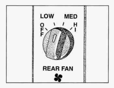
Rear Fan -- Rear Control: This feature allows passengers riding in the rear seats to control the flow of air to the rear area of the vehicle.
