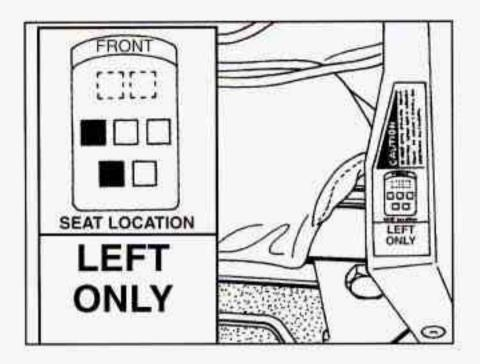
There are three types of rear bucket seats: RIGHT ONLY, CENTER OR LEFT and LEFT ONLY. RIGHT ONLY and LEFT ONLY seats may be equipped with the built-in child restraint option.
