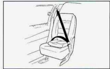
To make sure that the child is tall enough, compare the child's standing height to the top surface of the bucket seat, which is about 29 inches (74 cm) from the floor.
