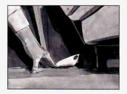
There's a vinyl sleeve there; to get to the bracket, push this vinyl sleeve aside slightly. Anchor the top strap to the bracket. If you need to have an anchor bracket installed for any additional passenger seat position, you can ask your Oldsmobile retailer to put it in for you. If you want to install an anchor bracket yourself, your retailer can tell you how to do it.
