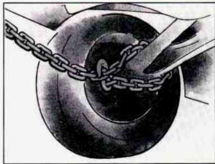
Attach T-hook chains on both sides, in the slotted holes in the bottom of the frame rails behind the front wheels.
