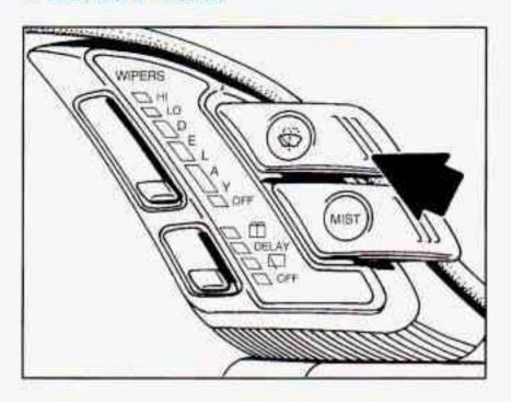
To wash your windshield, press and hold the windshield washer switch. The washers and wipers will operate. When you release the switch, the washers will stop, and the wipers will continue to operate for two cycles, unless your wipers had already been on. In that case, the wipers will resume the wiper speed you had selected earlier.
