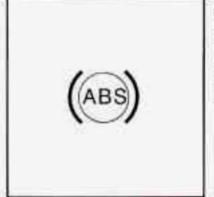
If there's a problem with the anti-lock brake system, this warning light will stay on or flash. See "Anti-Lock Brake System Warning Light" in the Index.
