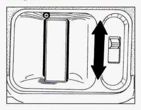
Lock the sliding door from the inside by sliding the manual locking lever down. Unlock it by sliding the lever up.
