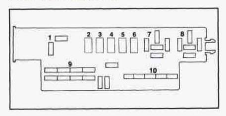
Circuit breakers and relays are located in the circuit breaker/relay panel. This is located behind the panel under the glove box, near the passenger's door.
