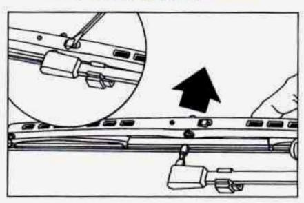
Replacement blades for your vehicle are 24 inches (61 cm) in length. They come in different types and are removed in different ways. Here's how to remove the type with a release clip:
