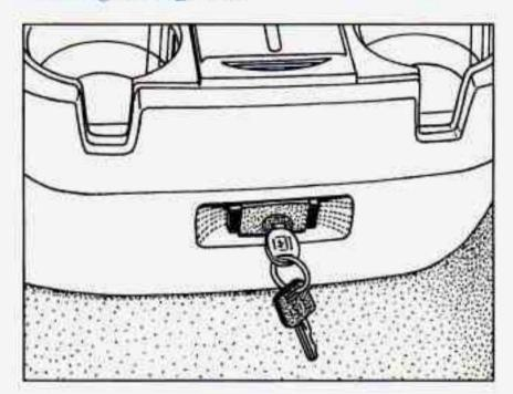
At the base of the center instrument panel console is a storage bin. Use the door key to lock and unlock it. To open the bin, pinch the latch release. Inside the storage bin, you will find a coinholder.
