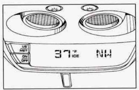
The outside air temperature and the compass are displayed at the front of the overhead console. The control switches are located to the left of the display. Turn the display on or off by pressing the ON/OFF switch. Display the temperature in either degrees Fahrenheit (English) or Celsius (metric) by pressing the US/MET switch.
