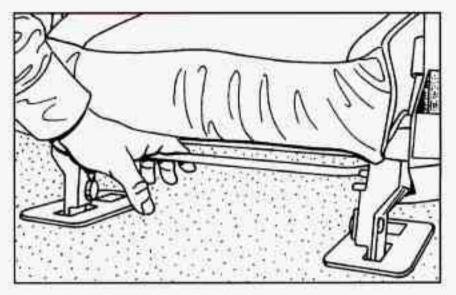
To get out of the third row seats, first lift the upper lever on the seat ahead of you to fold the seatback forward. Push down on the rear release bar under the seat ahead of you to tilt the entire seat forward.
