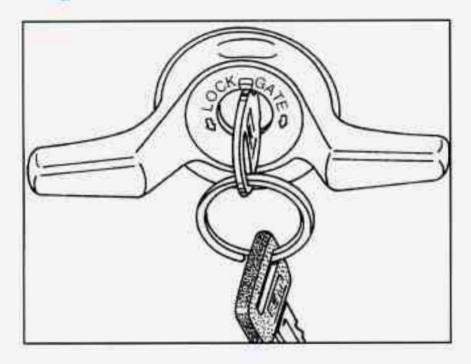
To unlock the liftgate, insert the door key and turn the lock clockwise. The liftgate will automatically lock when you close it.
