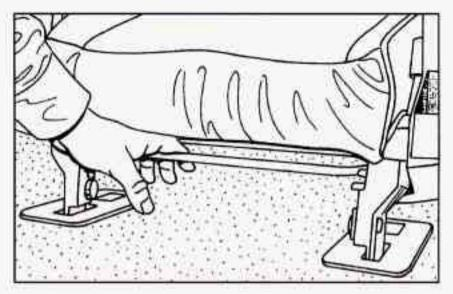
Push down on the rear release bar (located behind the seat) and tilt the entire seat forward.
