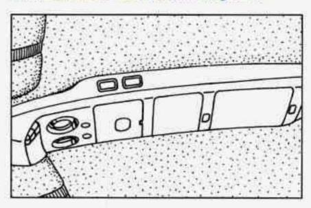
The front overhead console has the front reading lamps, two switches for the optional power sliding door, storage compartments (including one for your garage door opener and one for sunglasses), a compass and an outside temperature display. The features of the overhead console are explained on the following pages.
