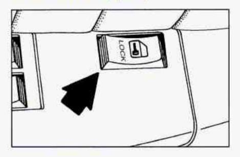
From the inside, press the front of the power door lock switch (on either front door), to unlock all doors and the liftgate.
