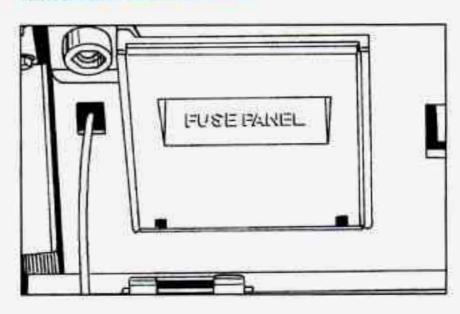
Pull the door open to gain access to the instrument panel fuse block.
