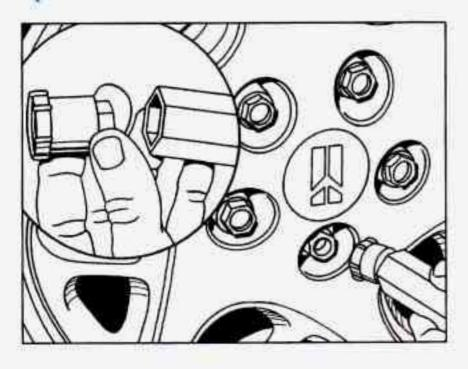
Each wheel nut is covered with a nylon cap. Use the folding wrench to remove the nylon caps from the wheel nuts before you loosen the nuts.
