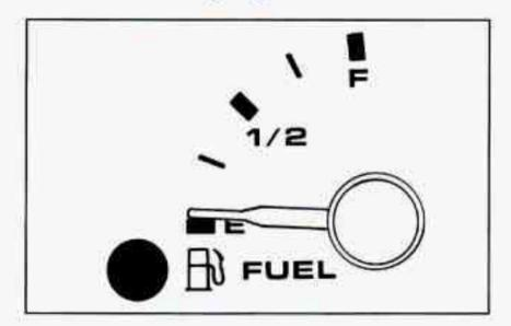
When there is between 3 gallons (11 L) and 0.5 gallon (1.8 L) of fuel left in the tank, the warning light next to the fuel symbol will go on.
