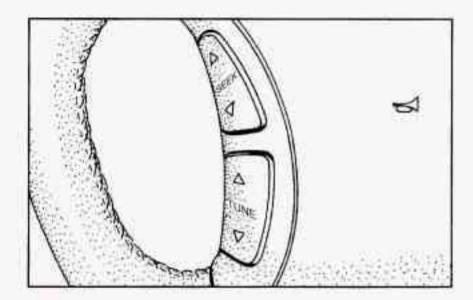
SEEK: Press this button to tune to a higher or lower radio station. The sound will be muted while seeking. When playing a cassette tape or compact disc, press SEEK to hear the next selection.
