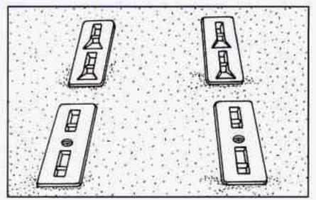
Each rear seat location has two sets of floor pins. Seats equipped with the built-in child restraint option must be secured in the rear set of floor pins. Seats that don't have the built-in child restraint can be secured in either set of floor pins. Move the position of these seats up or back to provide a little more room behind or in front of a seat.
