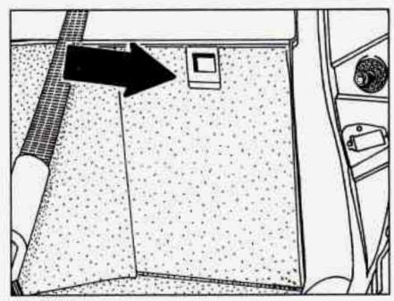
Open the jack storage compartment by sliding the latch down and removing the compartment cover.
