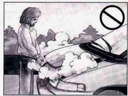
Steam from an overheated engine can burn you badly, even if you just open the hood. Stay away from the engine if you see or hear steam coming from it. Just turn it off and get everyone away from the vehicle until it cools down. Wait until there is no sign of steam or coolant before opening the hood.
