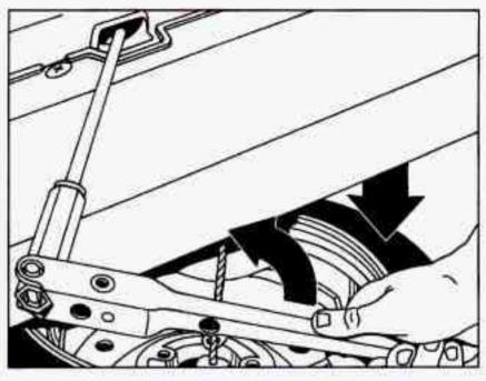
The compact spare tire is located under the vehicle, behind the rear bumper. Insert the narrow end of the shaft into the hole above the rear bumper. Then attach the folding wrench to the shaft.
