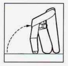
The second and third row bucket seats have been designed to allow them to fold fully upward and forward when the seats are anchored in the rear-most position. This design improves both luggage/cargo capacity and rear seat entry/exit.
