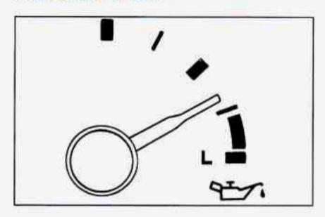
Your vehicle is equipped with an oil pressure indicator. Your oil pressure indicator lets you know when you may have a problem with your engine oil pressure.
