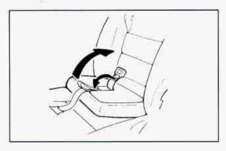
Make sure that the crotch strap is held flush to the child restraint cushion with the fastener strip. Also be sure the shoulder harness adjustment strap (grey) is folded up in the seat. This will allow the cushion to fold completely into the seatback. Raise the cushion.
