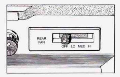
If your vehicle is equipped with seats in the third row, you will have a rear air outlet and a rear fan. To maximize airflow to the rear of your vehicle, place the left bucket seat in the second row in the forward position (see "Adjusting Rear Seats" in the Index). This uncovers the rear air outlet.
