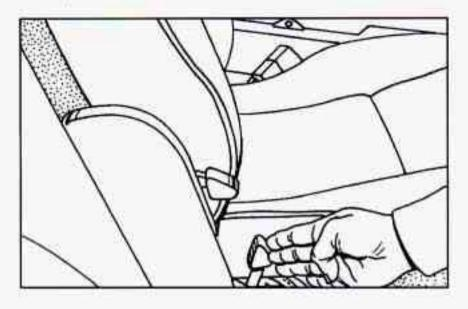
The RIGHT ONLY seats have a lower lever to tilt the seat forward. To get into third row seats, push back the lower lever on the RIGHT ONLY seat (nearest the sliding door) and tilt the seat forward completely. To return the seat to its normal position, pull the seat back, holding the lower lever back. Once the seat is in place, release the lower lever. Push and pull on the seatback to be sure that it is locked.
