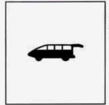
The liftgate ajar symbol on your instrument panel will come on if your liftgate is not completely closed.
