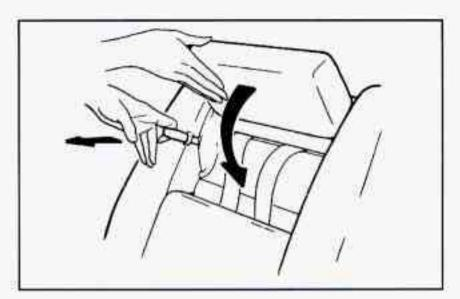
Unlatch the child head restraint by pulling the release strap. Lower the head restraint and press it firmly into the seatback until you hear the latch click.
