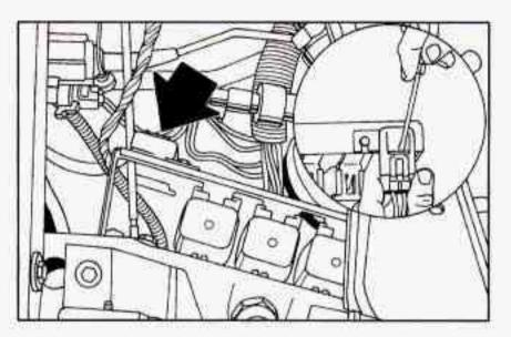
This fuse is located under the hood, on a bracket just behind the passenger's side headlamp. It is mounted on the face of the bracket in the position closest to the passenger's side of the vehicle. The fuse services the injectors, fuel pump, oil pressure sender and fuel pump switch.
