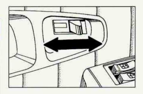
To lock the door from the inside, slide the locking lever rearward.
