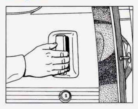
To open the sliding door from outside the vehicle, pull the front of the latch release out and then toward the rear. If you slide the door all the way back, it will latch in the open position.
