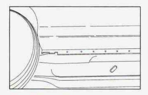
Attach T-hook chains on both sides, in the slotted holes in the frame rails, just ahead of the rear wheels.
