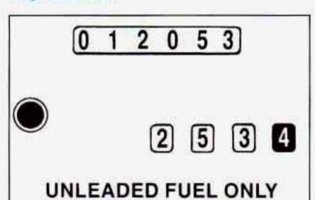
The trip odometer can tell you how far your vehicle has been driven since you last set it to zero. To set it to zero, push the reset button located above the fuel gage.
