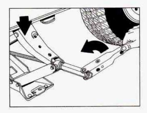
9. Lower the vehicle by attaching the folding wrench to the jack and rotating the wrench counterclockwise. Lower the jack completely.
