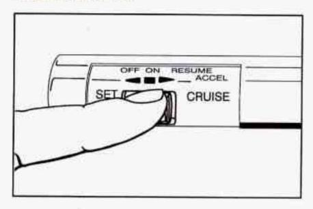
Suppose you set your cruise control at a desired speed and then you apply the brake. This, of course, shuts off the cruise control. But you don't need to reset it. Once you're going about 25 mph (40 km/h) or more, you can move the cruise control switch from ON to RESUME/ACCEL (R/A) for about half a second. You'll go right back up to your chosen speed and stay there.
