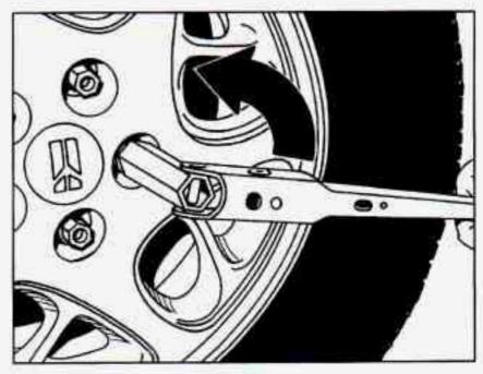
Loosen the wheel nuts — but do not remove them — using the folding wrench.
