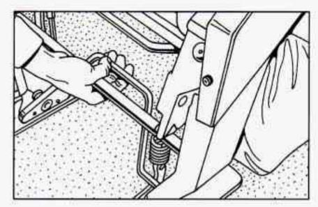
From behind the seat, support the top portion of the seat with one hand as you squeeze the front release bar toward the crossbar. The seat will release from the floor pins.
