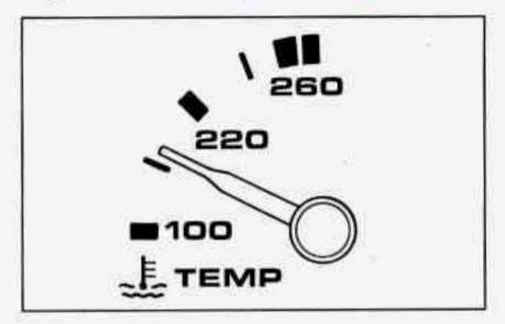
This gage shows the engine coolant temperature. If the gage pointer moves into the red area, your engine is too hot! It means that your engine coolant has overheated. If you have been operating your vehicle under normal driving conditions, you should pull off the road, stop your vehicle and turn off the engine as soon as possible.
