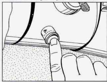
Your hazard warning flashers switch is on the steering column, below the ignition switch. Press the button in to turn on your flashers.
