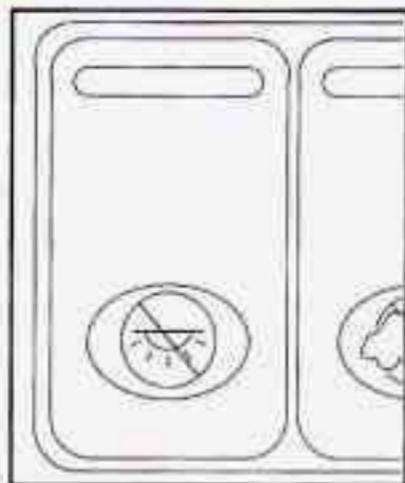
This switch is located in the overhead console switchbank. Press the symbol on the bottom of the rocker switch to override control of the interior lights and turn off power to the courtesy lamps, reading lamps, glove box lamp and underhood lamp.
