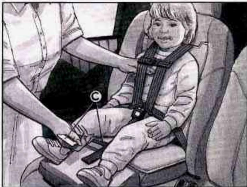
12. Pull the shoulder harness adjustment strap (C) firmly until the harness is snugly adjusted around the child. You should not be able to put more than two fingers between the harness and the child's chest. Make sure the harness and buckle strap are not twisted.
