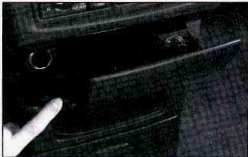
The front power outlet is located next to the ashtray and lighter. Pull the cover down to use the power outlet.
