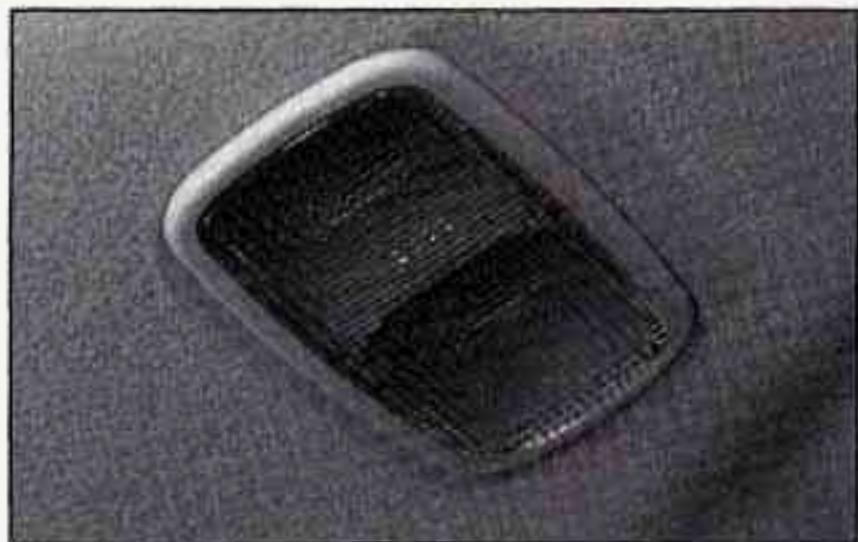
This lamp is located in the center of your vehicle and has no switch of its own. It will go on each time you open the doors, unless you enable the interior lights override.
