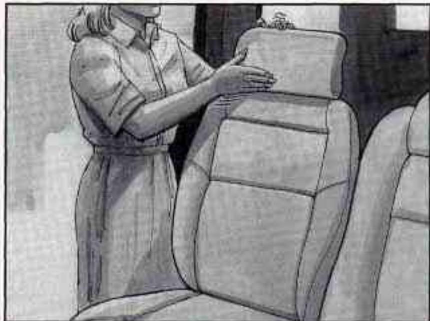
2. Rotate the head restraint rearward until it touches the top of the seatback. Make sure there is no gap between the lower edge of the head restraint and the top of the seatback.
