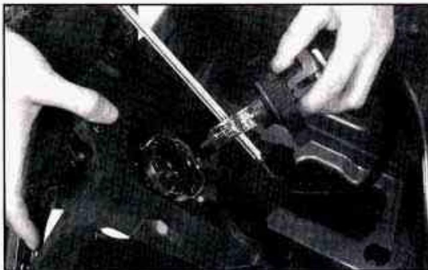
7. Carefully put the bulb assembly back into the lamp housing and tighten the black retainer ring in place. Be careful not to damage the bulb on the headlamp aiming bar.
