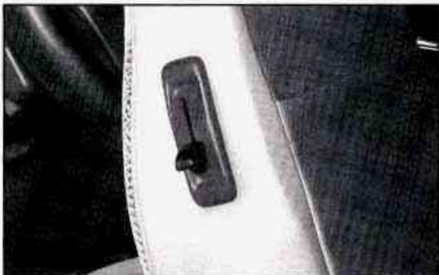
The seatback on the driver's seat folds forward to put items behind the seat. Lift the lever and fold the seatback forward. The seatback will lock into place when you push it back to the upright position.
