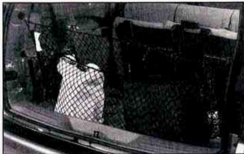
The optional convenience net is designed to help keep small loads, like grocery bags, from falling over during sharp turns or quick stops and starts. Install the convenience net at the rear of your vehicle, just inside the liftgate.
