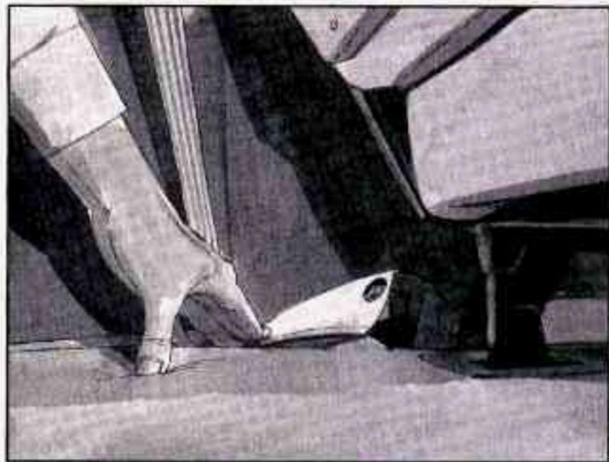
There's a vinyl sleeve there; to get to the bracket, push this vinyl sleeve aside slightly. Anchor the top strap to the bracket. If you need to have an anchor bracket installed for the right-hand side of a 60/40 bench seat, you can ask your Oldsmobile retailer to put it in for you. If you want to install an anchor bracket yourself, your retailer can tell you how to do it.
