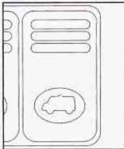
Press the symbol on the bottom of the rocker switch to open the sunroof to the vent position. To close the sunroof from the vent position, press the ribbed top part of the button.
