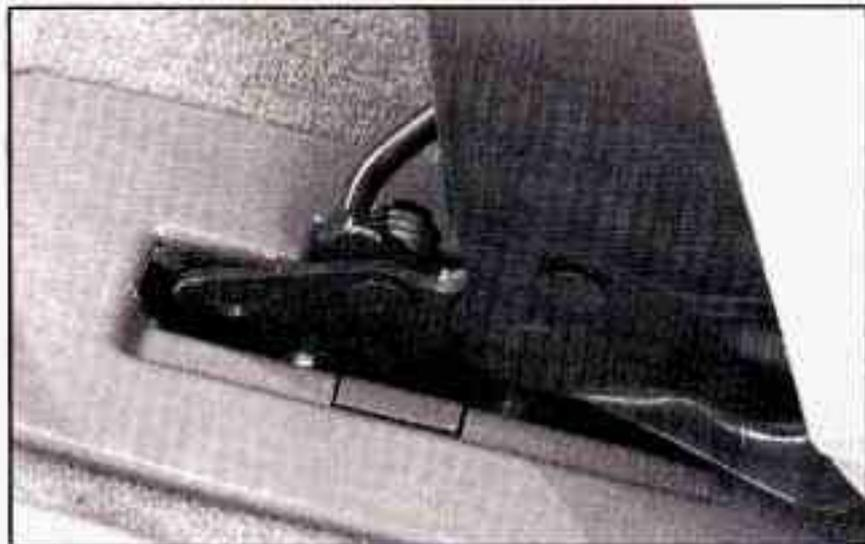
4. If the front latches are not attaching correctly, check that the seat is in the full rear position.
