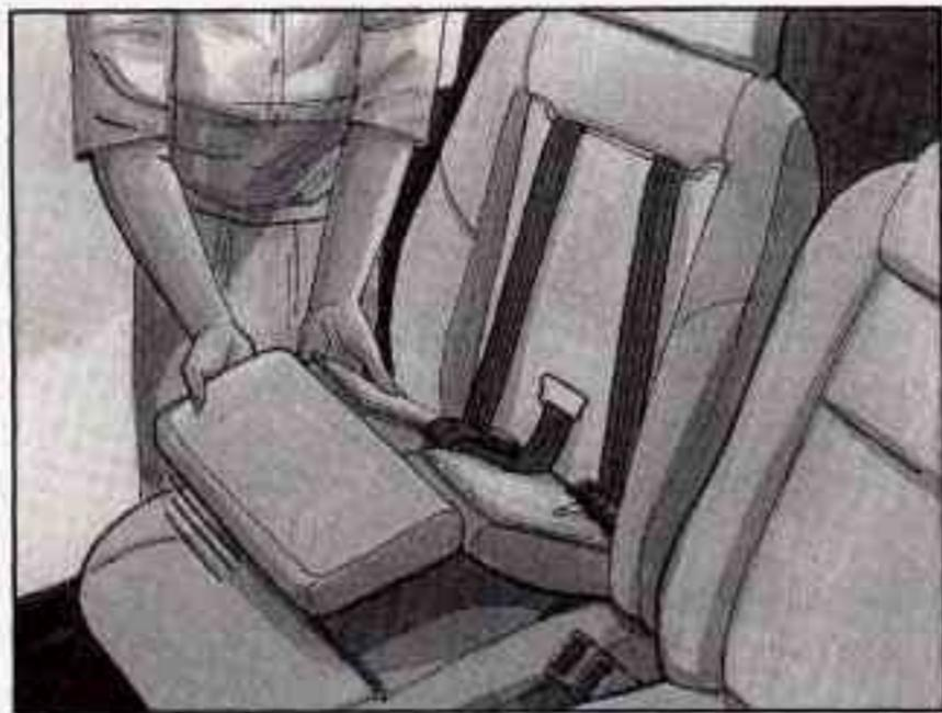
2. Fold the child restraint cushion and leg rest up into the seatback.
