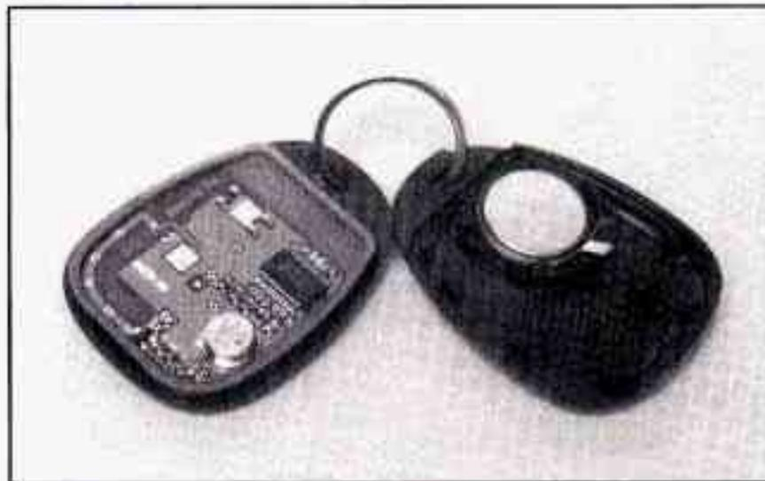
2. Gently pry the battery out of the transmitter. Do not use the metal flanges to "pop out" the battery.
