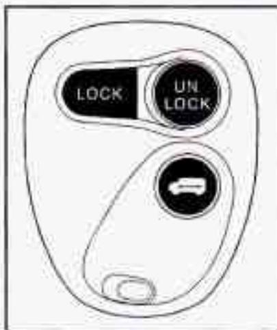
If you have the optional power sliding door (see “Power Sliding Door” later in this section), your remote transmitter will have a button that has a van symbol on it. Press it to open or close the sliding door.
