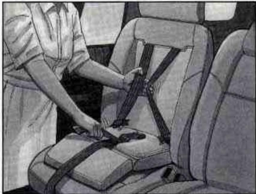
4. Before placing the child in the child restraint, add slack to the shoulder harness. Pull the black shoulder harness release strap firmly. At the same time pull both shoulder harness straps through the slots in the seatback as shown.
