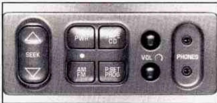
This feature allows rear seat passengers to listen to a different music source than the front seat passengers including AM-FM automatic tone control, cassette tapes or CDs. For example, rear seat passengers may listen to a cassette tape or CD through headphones while the driver listens to the radio through the front speakers. The rear seat passengers have control of the volume for each headphone. Be aware that the front seat audio controls always override the rear seat audio controls.
