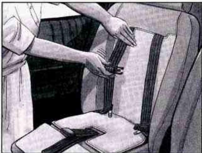
1. Move both latch plates and both sides of the shoulder harness clip to the bottom of the harness straps.
