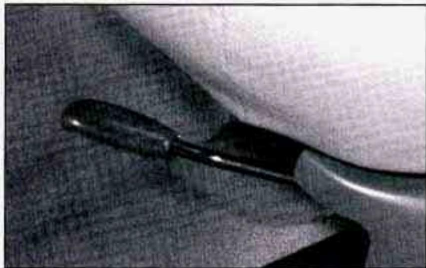
Use the lever on the front left side of the seat to adjust the seat forward or backward. Pull up the lever on the front of the seat to unlock it. Slide the seat to where you want it. To make sure the seat is locked into place, release the lever and try to move the seat with your body.
