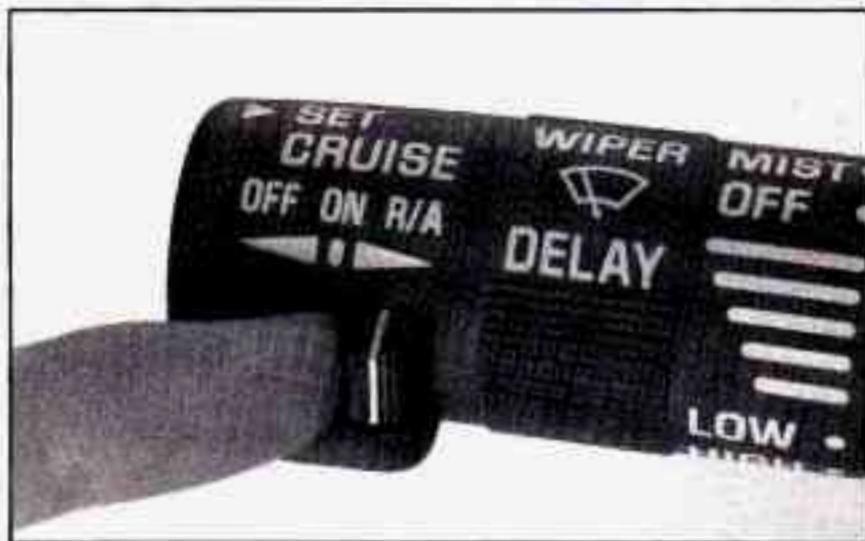
Suppose you set your cruise control at a desired speed and then you apply the brake. This, of course, shuts off the cruise control. But you don't need to reset it. Once you're going about 25 mph (40 km/h) or more, you can move the cruise control switch from ON to RESUME/ACCEL (R/A) for about half a second.
