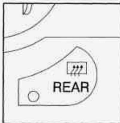
Press REAR (the light will glow) to warm the defogger grid on the rear window.
