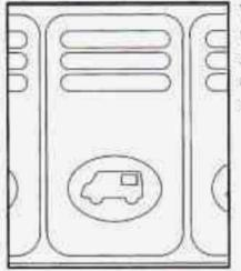
This button, located in the Overhead Console switchbank, is used for opening and closing the rear quarter windows.
