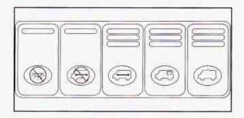
This switchbank is located in the overhead console. The switches that you may find in this switchbank are the Interior Lights Override, Power Sliding Door Override, Power Sliding Door, Power Rear Quarter Windows and Sunroof. If your vehicle does not have some of the options controlled by these switches, there will be a blank button in its place.
