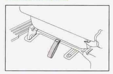
Pull the nylon strap behind the chair to release the rear hooks from the floor pins. The seat can then be lifted off the front floor pins and removed from the vehicle.
