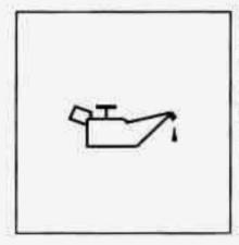
Your vehicle is equipped with an oil pressure warning light. Your oil pressure indicator lets you know when you may have a problem with your engine oil pressure.
