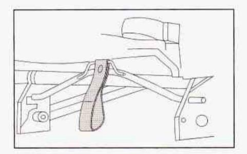
Do not let go of the straps until the seat is folded all the way forward. To unlatch the front latches, squeeze the angled latch release bar towards the straight crossbar.
