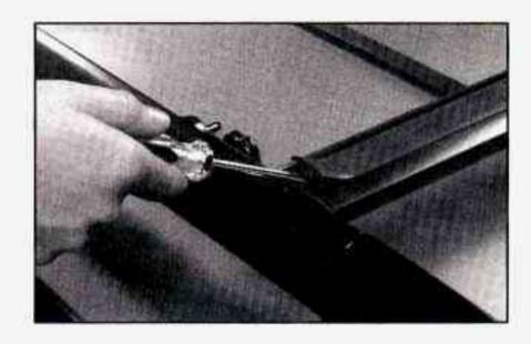
Lift the end of the bumper strip with a flathead screw driver and cut off enough of the strip to access the tapped plates.
