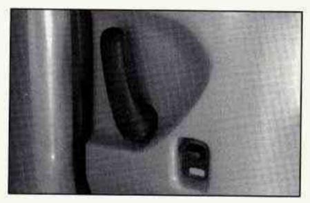
Lock the sliding door from inside the vehicle by moving the manual locking lever down. Unlock it by moving the lever up.
