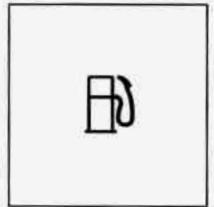
When there is between 3 gallons (11 L) and 1.0 gallon (3.8 L) of fuel left in the tank, the warning light next to the fuel symbol will go on.
