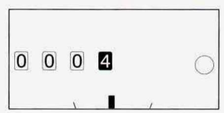
The trip odometer can tell you how far your vehicle has been driven since you last set it to zero. To set it to zero, push the reset button which is located above and to the right of the temperature gage.
