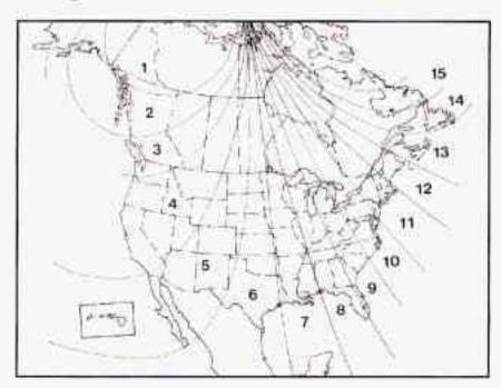
Turn the ignition on and cycle the DIC to the Compass/Temperature mode. Press both the E/M and MODE buttons for approximately five seconds. The last entered variance zone number will be displayed. Press the E/M button until the proper variance number, as shown on the map, is showing. Press the MODE button to set the new variance zone and resume normal operation.
