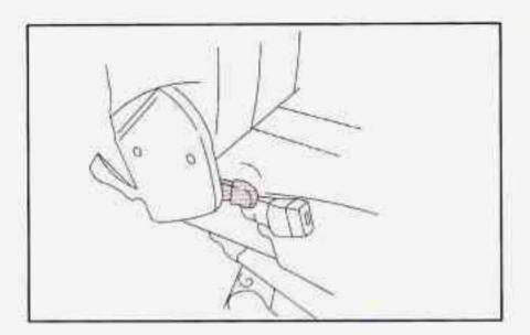
To raise either seatback, pull the nylon strap on the back of the seat while raising the seatback until it locks upright. Push and pull on the seatback to check that it is locked upright.
