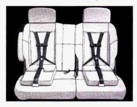
If your vehicle has this option in a 60/40 bench seat, there's a built-in child restraint at each outboard position of the 60/40 bench seat. This bench seat will only fit in the second row of your vehicle.
