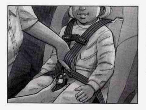
Pull up on both latch plates to make sure they are secure.
