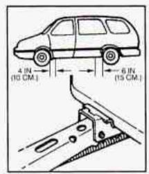
Near each wheel, there is a notch in the vehicle's body. Position the jack and raise the jack head until it fits firmly into the notch in the vehicle's frame nearest the flat tire.
