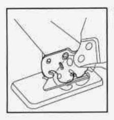
Remove the seat by rocking it slightly towards the rear of the vehicle and then pulling it out. This should be done in one motion.
