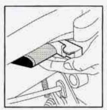
Lift up either lever and slide the seat forward to allow for extra storage behind the seat, or slide the seat back to allow extra room for passengers.
