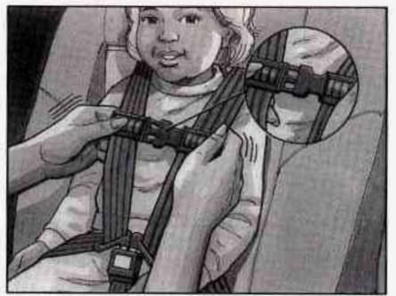
Now fasten the left and right halves of the shoulder harness clip together. The purpose of this clip is to help keep the harness positioned on the child's shoulders.
