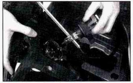
Carefully put the bulb assembly back into the lamp housing and tighten the black retainer ring in place. Be careful not to damage the bulb on the headlamp aiming bar.
