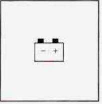
The charging system light will come on when you turn on the ignition as a check to show you it is working. It will remain on as long as the engine is not running.
