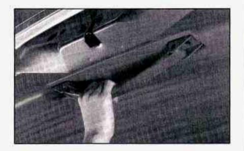
To close the liftgate, pull down on the handle, then firmly shut the liftgate. Don't drive with the liftgate open, even slightly. See "Engine Exhaust" in the Index. A light on your instrument panel will warn you if the liftgate is not completely closed (see "Door Ajar Warning Light" in the Index).
