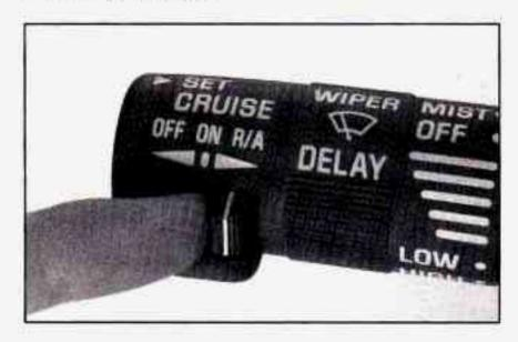
Suppose you set your cruise control at a desired speed and then you apply the brake. This, of course, shuts off the cruise control. But you don't need to reset it. Once you're going about 25 mph (40 km/h) or more, you can move the cruise control switch from ON to RESUME/ACCEL (R/A) for about half a second.
