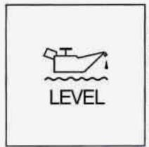
If the Low Oil Level light on the instrument panel comes on, it means you need to check your engine oil level right away. For more information, see "Low Oil Level Light" in the Index. You should check your engine oil level regularly; this is an added reminder. It's a good idea to check your engine oil every time you get fuel. In order to get an accurate reading, the oil must be warm and the vehicle must be on level ground.
