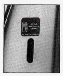
To use the security lock, move the security lock lever all the way up and close the door from the outside.
