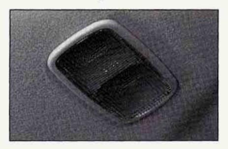
This lamp is located in the center of your vehicle and has no switch of its own. It will go on each time you open the doors, unless you enable the interior lights override.
