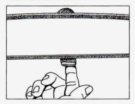
To reduce glare from lights behind you, pull the lever toward you (to the night position). To return the mirror to the day position, push the lever away from you.
