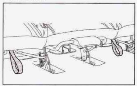
Do not let go of the straps until the seat is folded all the way forward. Unhook the front latches by rolling up the gray handle under the seat until the handle locks.
