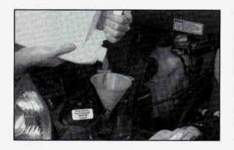
Fill the radiator with the proper DEX-COOL mix, up to the base of the filler neck.
