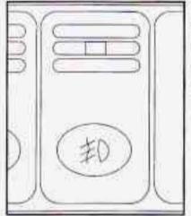
The fog lamps switch is located in the Instrument Panel switchbank.
