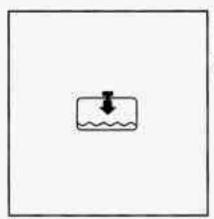
If this light comes on, your system is low on coolant and the engine may overheat.
