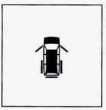
This light will come on if any of the doors or the liftgate are not completely closed and the ignition is turned to RUN or START.
