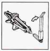
Attach the folding wrench to the jack, and rotate the wrench clockwise to raise the jack head a few inches.
