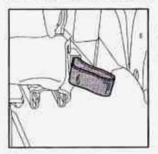
Use the lever on the front of the seatback to raise or lower the seatback to the desired position.
