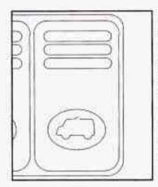
Press the symbol on the bottom of the rocker switch to open the sunroof to the vent position. To close the sunroof from the vent position, press the ribbed top part of the button.
