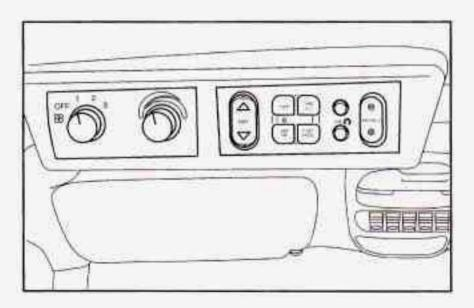
Turn the temperature knob counterclockwise (to the blue area) for cooler air, or clockwise (to the red area) for warmer air.
