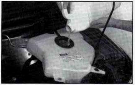
Then fill the coolant recovery tank to the FULL HOT mark.
