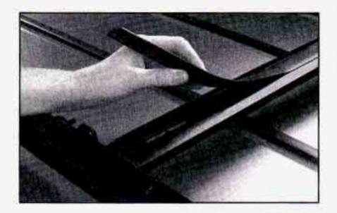
After removing the tiedowns or other equipment, be sure to install the the piece of bumper strip that was cut.
