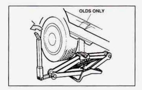
Lower the vehicle by attaching the folding wheel wrench to the jack and rotating the wrench counterclockwise. Lower the jack completely.
