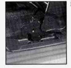
Place the front hooks of the bench seat onto the front two floor pins. To do this, the seat will need to be angled so that the front hooks clear the floor pins.
