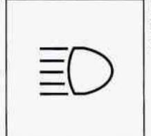
When the high beams are on, this light on the instrument cluster will also be on.
