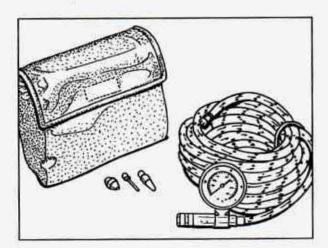
The air inflator kit is stored in the glove box. It includes a 20-foot (6 m) hose with an air pressure gage and nozzle adapters.
