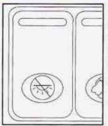
This switch is located in the overhead console switchbank. Press the symbol on the bottom of the rocker switch to override control of the interior lights and turn off power to the courtesy lamps, reading lamps, glove box lamp and underhood lamp.
