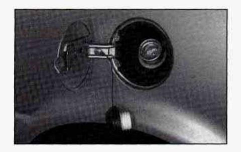
While refueling, hang the cap by the tether from the hook on the filler door hinge.
