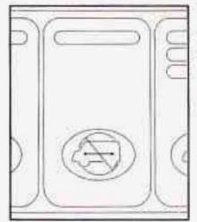
To operate the power sliding door, the power sliding door override switch must be disabled. This switch is located in the overhead console switchbank.
