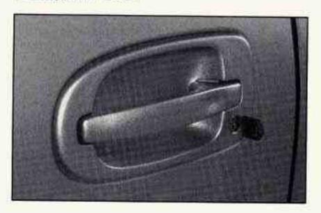
To unlock either sliding door from the outside using your key, insert the key and turn it toward the rear of the vehicle. To lock the sliding door from the outside, turn the key toward the front of the vehicle.
