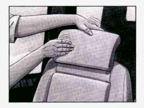
Rotate the head restraint forward and push it all the way down.
