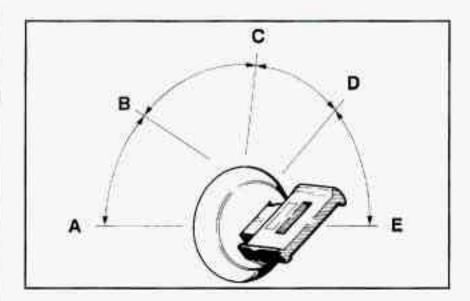
ACCESSORY (A): An on position in which you can operate your electrical power accessories. Press in the ignition switch as you turn the top of it toward you.
