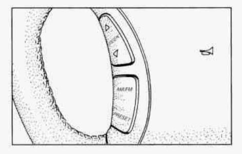
SEEK: Press the up arrow to tune to a higher radio station and the down arrow to tune to a lower radio station. The sound will mute while seeking. When playing a cassette tape or compact disc, press SEEK to hear the next selection. AM-FM: Press this button to choose AM or FM.
