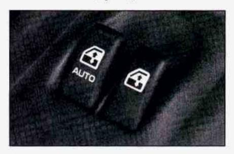
If you have power windows, the switches on the driver's door armrest control the front windows (when the ignition is on). The left switch controls the driver's window. The right switch controls the passenger's window.
