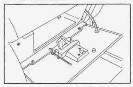
The glove box door has a detent to prevent the door from lowering too far. Open the glove box until the door is partway open, then pull the door down if you need it fully open. To close the glove box, the door must be pushed up past the detent.
