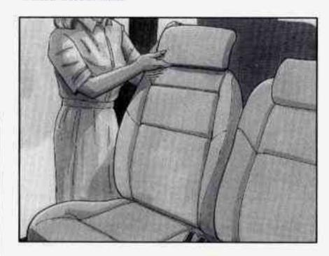
Raise the head restraint until the lower edge of the head restraint is even with the top of the seatback.
