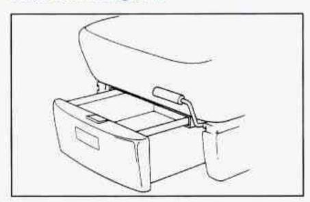
The storage bin is under the manual front passenger's seats. To open the bin, lift the handle and slide the drawer out.
