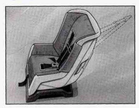
If your child restraint has a top strap, it should be anchored. A child restraint with a top strap should only be used in the second row. Anchor brackets for the second row outside positions are located just above the place where the third row lap-shoulder belts meet the floor.
