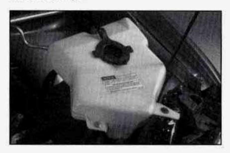
The coolant level should be at or above the FULL HOT mark. If it isn't, you may have a leak in the radiator hoses, heater hoses, radiator, water pump or somewhere else in the cooling system.
