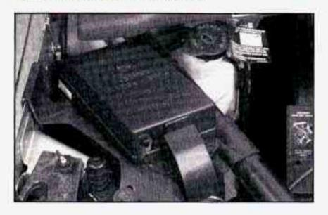
This fuse and relay center is located in the engine compartment, in front of the windshield washer fluid reservoir.
