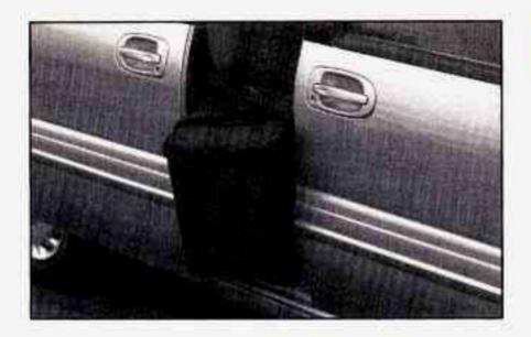
If anything obstructs the power sliding door while it is closing, the door will automatically reverse to the open position, provided it meets sufficient resistance. Resistance must be as strong as the force of the closing door, or stronger. The force of the closing door increases significantly as the door approaches the latch position.
