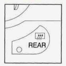
Press REAR (the light will glow) to warm the defogger grid on the rear window.
