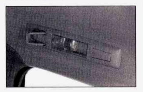
There are two reading lamps in the third row headliner, above the outboard seating positions. If your vehicle does not have dual sliding doors, there is also a reading lamp in the second row on the left side.
