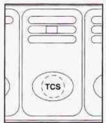
To turn the system off, press the TCS symbol on the bottom of the button in the center console switchbank. The indictor light on the traction control button will go off.
