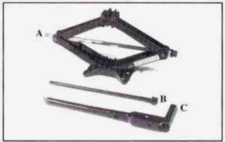
The tools you'll be using include the jack (A), shaft (B) and folding wrench (C).
