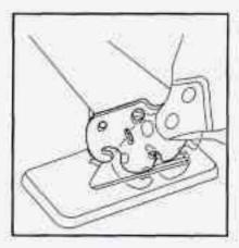
Remove the seat by rocking it slightly towards the rear of the vehicle and then pulling it out.
