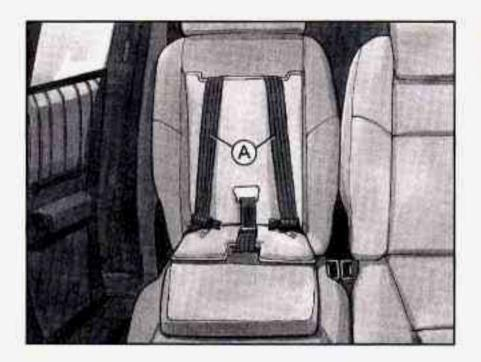
You'll be using the child restraint's harness (A) to secure your child. Don't use the vehicle's safety belts.
