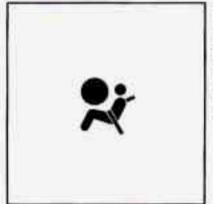
This light will come on when you start your engine, and it will flash for a few seconds. Then the light should go out. This means the system is ready.
