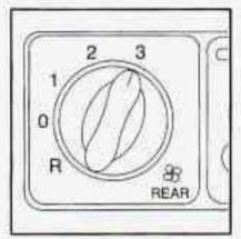
The rear fan control is located below the Climate Control system, in the switchbank.
