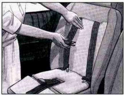
Move both latch plates and both sides of the shoulder harness clip to the bottom of the harness straps.
