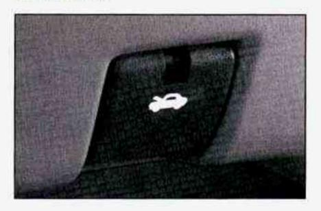
To open the hood, first pull the hood release handle inside the vehicle.
