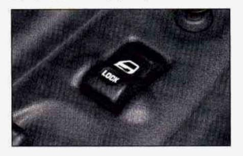
From the inside, press the front of the power door lock switch (on either front door) to unlock all doors and the liftgate. If your vehicle is equipped with the Content Theft Deterrent system, the power door lock switch will not unlock the doors until the system is disarmed. See "Content Theft Deterrent" in the Index for more details.
