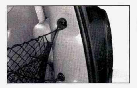
Attach the upper loops to the posts on either side of the liftgate opening (the label on the net should be in the upper left-hand corner).
