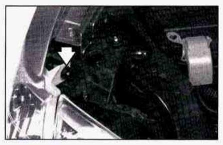
Pull the parking/turn signal lamp assembly away from the body.  Unscrew the bulb sockets from the lamp assembly by pressing the tab while turning counterclockwise.
