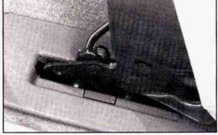
If the front legs are not attached correctly, the rear legs will not attach to the rear set of floor pins.
