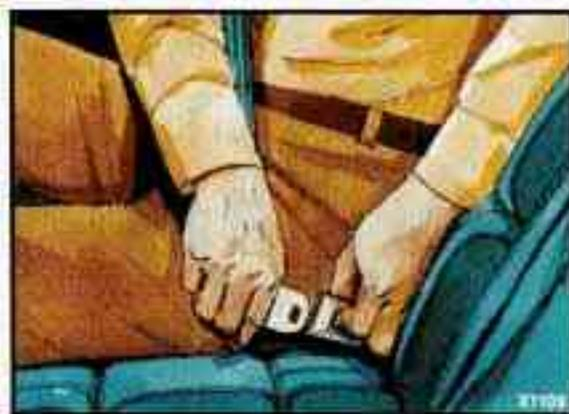
To unclatch the belt, just push the button on the buckle.
