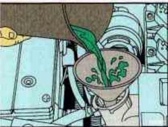
3. Fill the radiator with the proper mix, up to the base of the filler neck.
