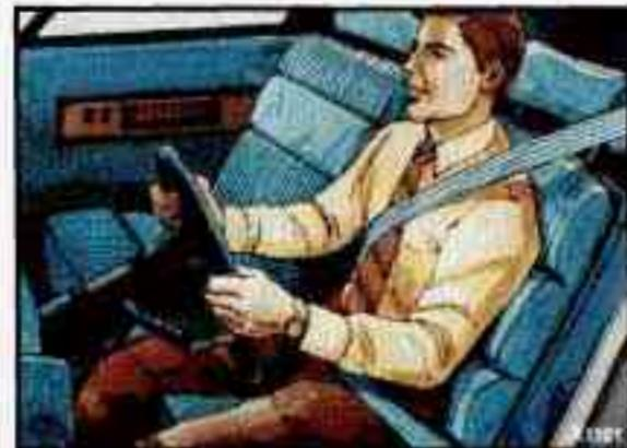
Adjust the height so that the shoulder portion of the belt is properly positioned on your shoulder, away from your face and neck.
