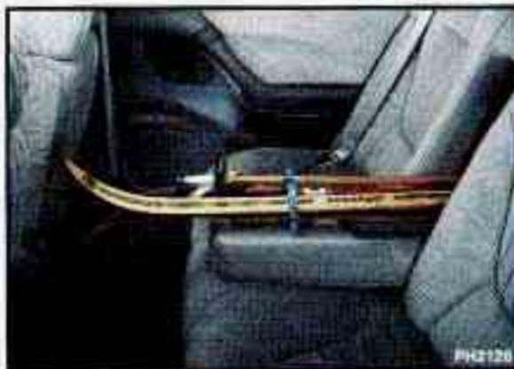
Pull down the interior door to access the trunk for storing long objects.
