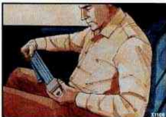
When you sit in a center seating position, you have a lap safety belt, which has no retractor. To make the belt longer, tilt the latch plate and pull it along the belt.
