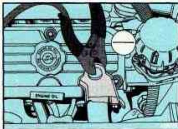
**9.** Attach the cable at least 18 inches (45 cm) away from the dead battery, but not near engine parts that move. The electrical connection is just as good there, but the chance of sparks getting back to the battery is much less.
