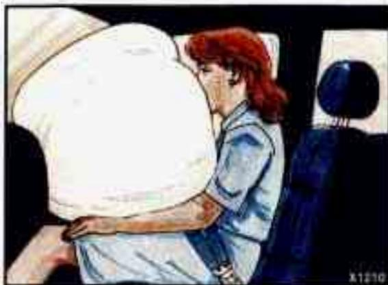
If your vehicle has a right-front passenger air bag, it is located in the instrument panel on the passenger's side.
