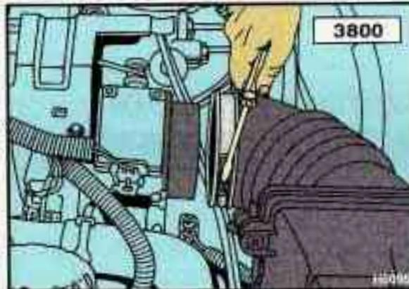
2. Unscrew the clamp on the air intake hose where the hose attaches to the throttle body near the top of the engine. Detach the hose from the throttle body, then pull back the rear of the housing cover.
