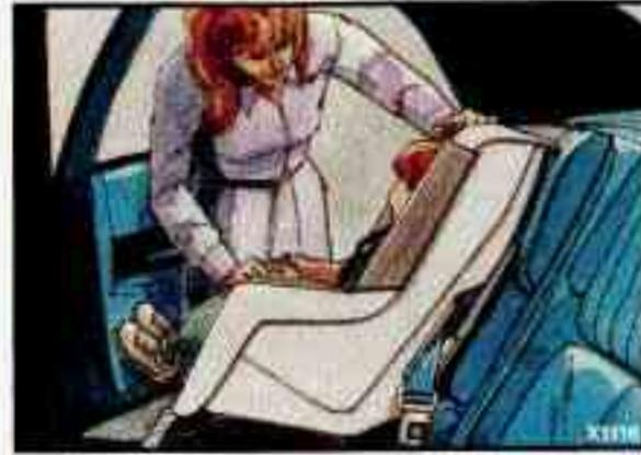
**7.** Push and pull the child restraint in different directions to be sure it is secure.
