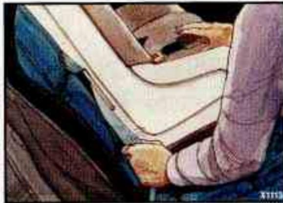
**6.** To tighten the belt, feed it into the retractor while you push down on the child restraint.
