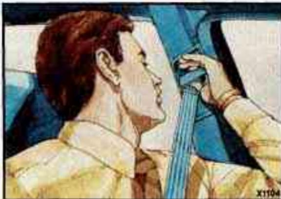
To move it up or down, squeeze the release handle. When you release the handle, try to move it down a little to make sure it has locked into position.
