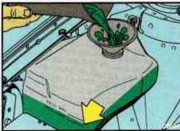
4. Then fill the coolant recovery tank to the **FULL COLD** mark.
